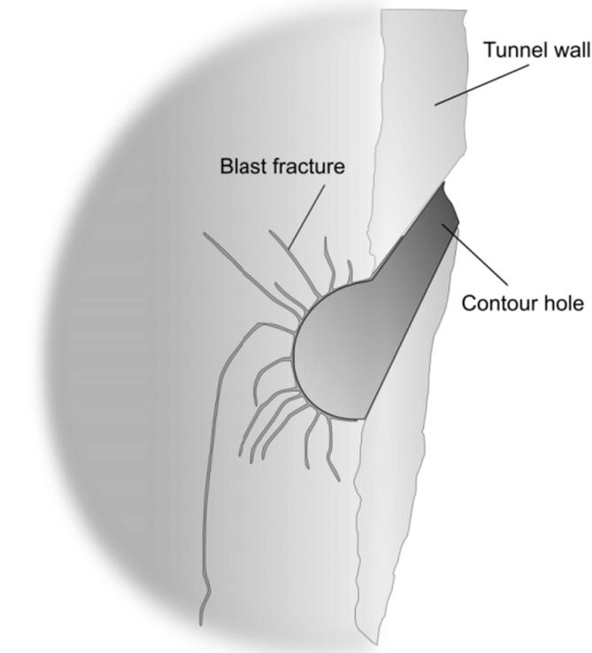
Fig. 3. Part of an investigation slot surface showing blast fractures near a blast hole halfpipe. Hole diameter is 48 mm.
