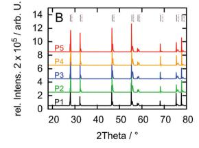
Fig. 6 (A) Diffractograms before the first H<sub>2</sub>O<sub>2</sub> exposure and (B) after the third H<sub>2</sub>O<sub>2</sub> exposure. Y-Axis offset is added for clarity. Indices for  $UO_2$  are shown as gray lines<sup>36</sup> and for  $U_4O_9$  as purple dashed lines.<sup>37</sup>
