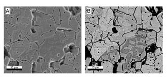
Fig. 5 (A) SE-SEM of P3 after the third exposure to  $\rm H_2O_2$  and (B) BSE-SEM of the same area.
