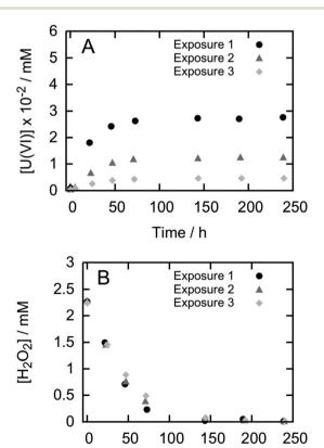
Fig. 1 Uranium release (A) and  $H_2O_2$  consumption (B) from pellet P5 during three consecutive exposures to  $H_2O_2$ .
