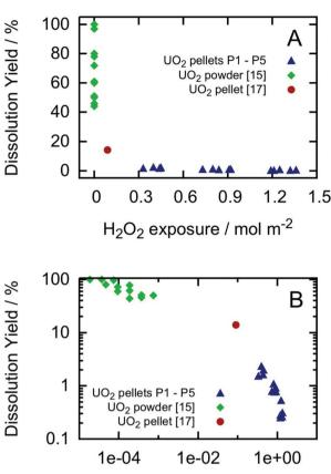
Fig. 3 Dissolution yield vs. accumulated  $H_2O_2$  consumption per  $m^2$  of exposed  $UO_2$ .  $UO_2$  pellets from this study (blue triangles),  $UO_2$  pellets (red dot), as well as powders<sup>18</sup> (green diamonds). (A) Linear axes and (B) logarithmic axes.
