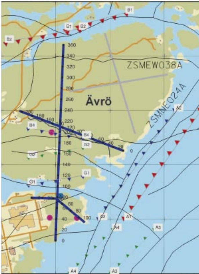
Figure 4-58. Seismic reflector B2 /Juhlin et al. 2004b/ indicates the extension of ZSMEW038A over Ävrö.
