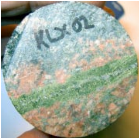
Figure 2-70. Fracture filled with epidote (green) and quartz (grey). Note the red colour of the wall rock due to hydrothermal alteration. Picture from KLX02.
