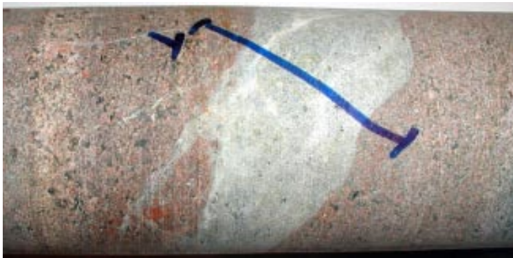
Figure 2-72. Fracture filled with prehnite. Note the red colour of the wall rock due to hydrothermal alteration. From KSH01A.
