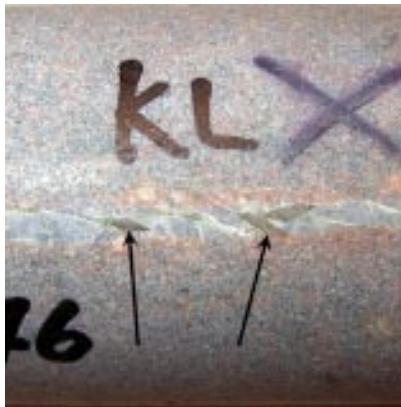
Figure 2-75. Fracture filled with quartz, epidote and titanite (arrows). KLX03.
