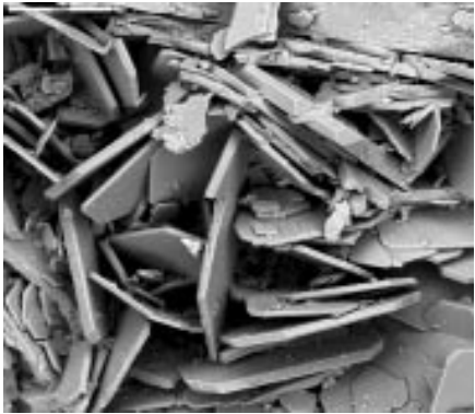
Figure 2-80. SEM-image of apophyllite fracture coating in an open fracture. KLX03. Scale bar is 200 \mu m .
