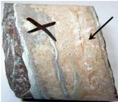
Figure 2-85. Fracture fillings of laumontite (arrow), calcite (white), adularia (red, coating laumontite filled fractures) and hematite-rich cataclasite (red, left). KSH03A.
