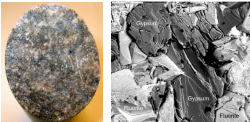
Figure 2-83. Photograph and SEM-image of gypsum and fluorite crystals on a fracture surface. Scale bar (right) is 200 µm. KLX06.
