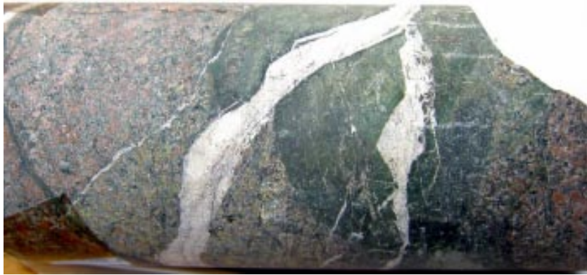
Figure 2-69. Drill-core sample from KSH03 showing fractures filled with calcite (white) cross-cutting a green filling dominated by illite.
