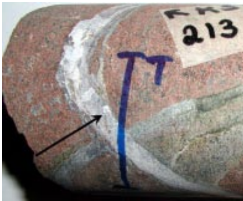
Figure 2-77. Fracture filled with albite (arrow) and calcite (white) is cutting a fracture filled with prehnite. KSH01A.
