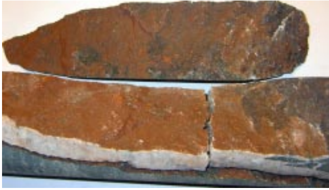
Figure 2-74. Fracture surface covered with hematite. The white fracture filling is earlier formed calcite. KLX04.
