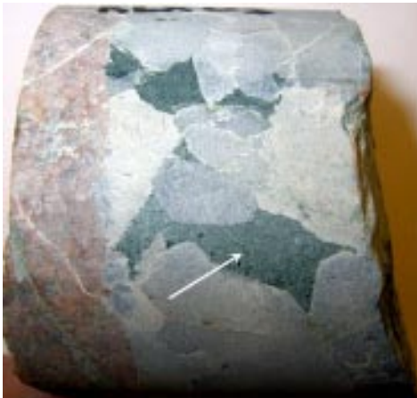
Figure 2-71. Fracture filled with chlorite (arrow), calcite (white) and quartz (grey). KLX03.
