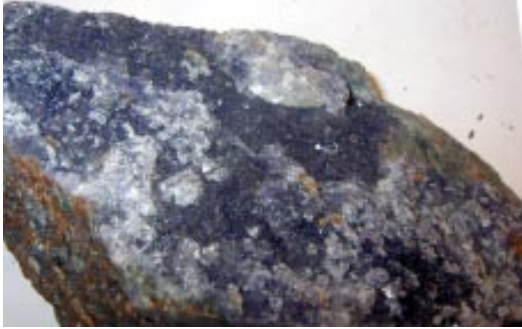
Figure 2-84. Fracture coating of purple fluorite and white calcite. KLX04.
