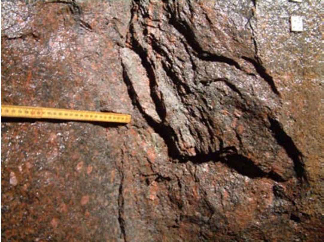
Figure A2e-33. Photograph at depth of approximately 2.5 m showing the right side of the pillar, where almost no slabs could be removed.
