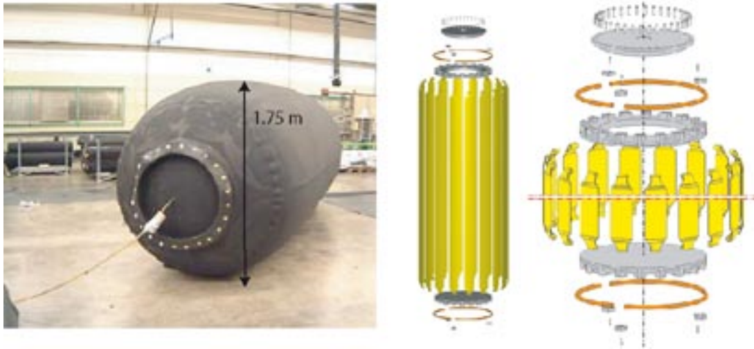
Figure 4-9. The specially constructed rubber bladder and the confining equipment. The vertical textile straps connected to the horizontal steel plates kept the bladder in place as it was expanded by a water pressure.
