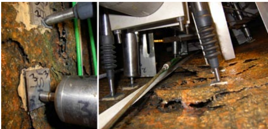
Figure A2e-12. June 8. Photographs of spalling/fracturing at position 3 (2.5 m level) and between positions 9 and 10 at the 3 m level. In the right photograph position 9 is to the left.
