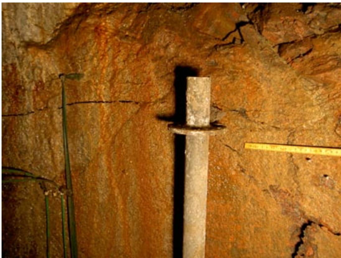
Figure 10-7. Photograph of the horizontal fracture that dilated during de-stress drilling. Note how it ends/begins close to the shear zone.
