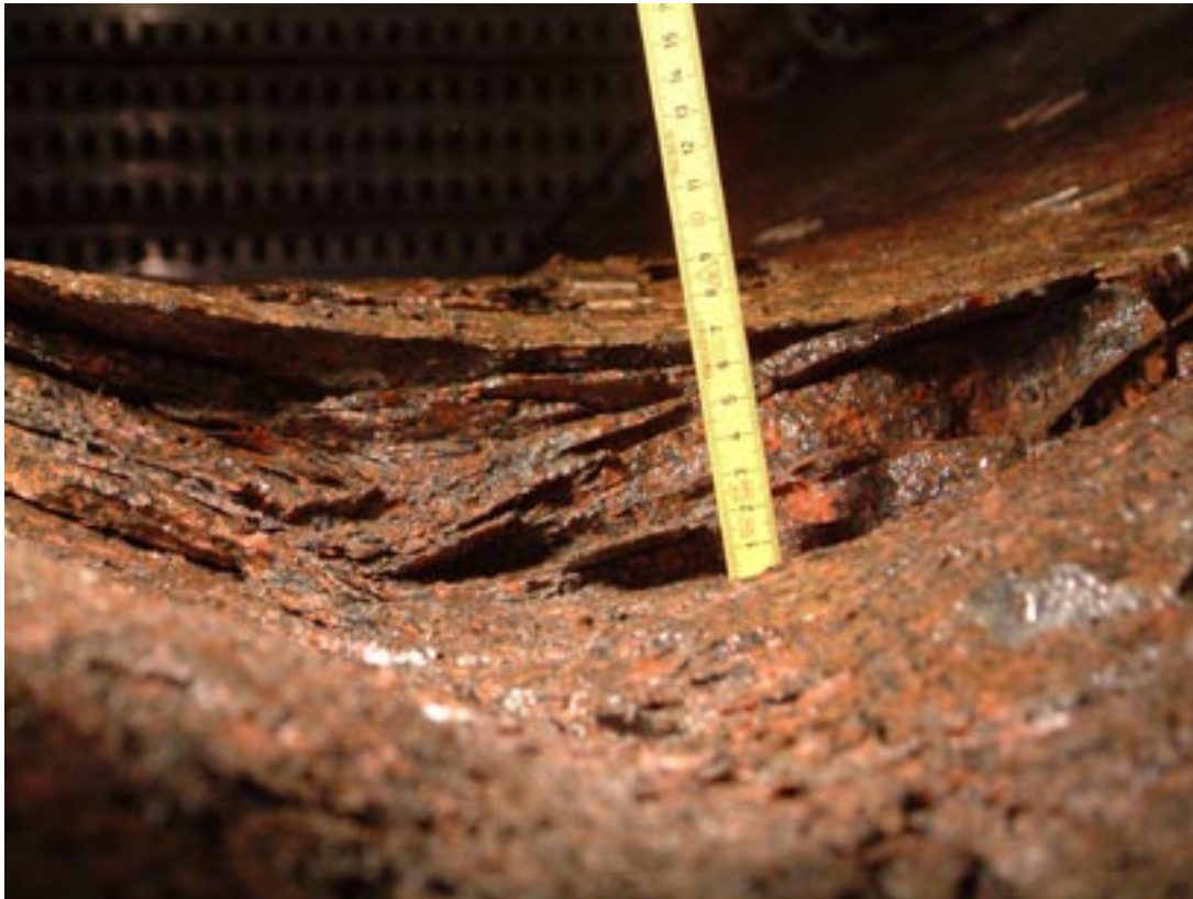
Figure A2e-29. Photograph of the smooth arched notch at a depth of 3.7 m.
