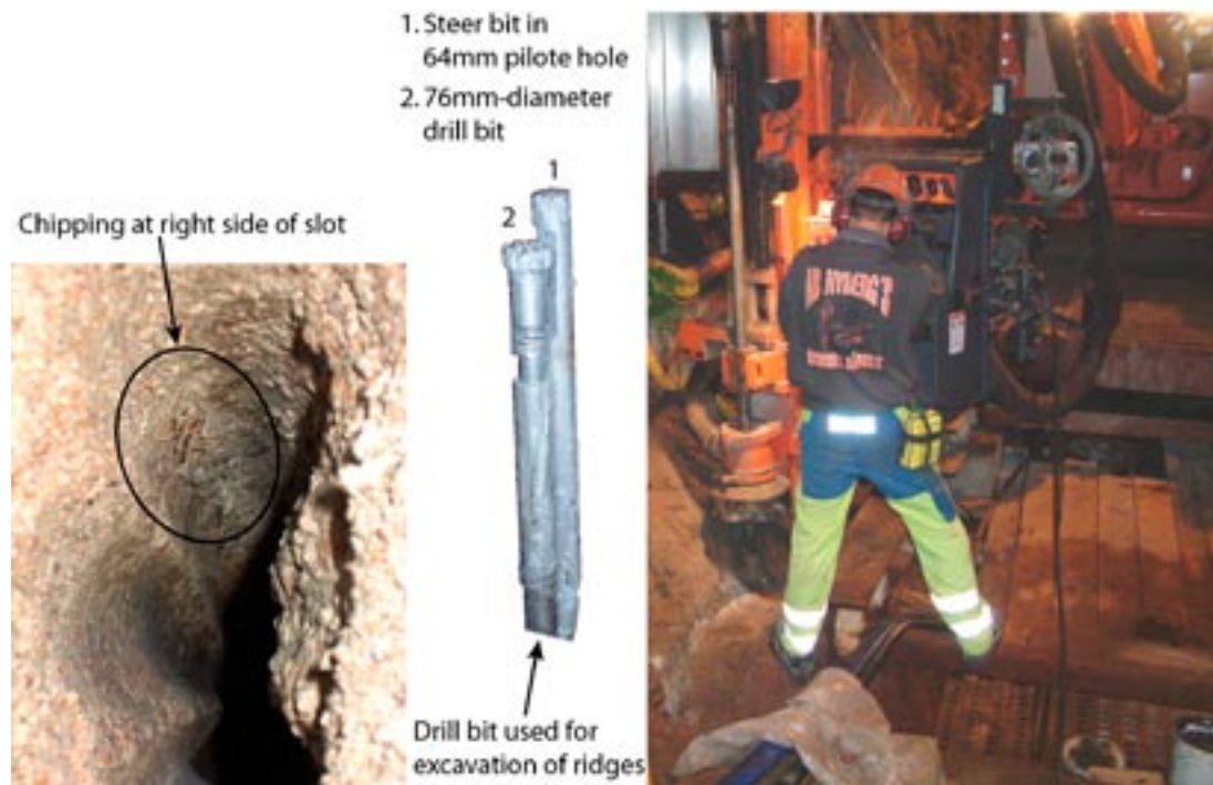
Figure 10-4. Left: chipping initiated from the top of the right part of the notch. Right: photograph of the drilling of the slot.
