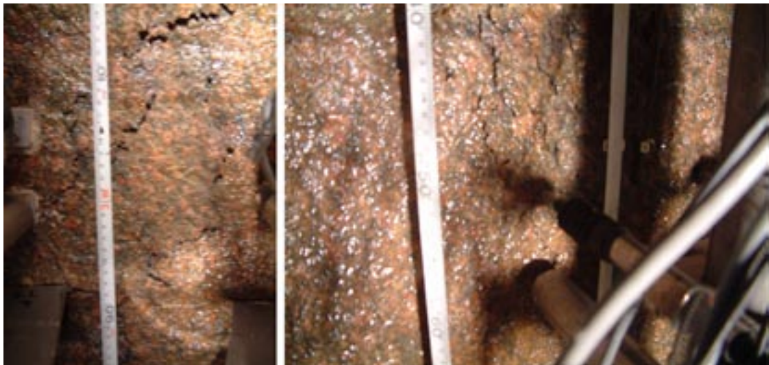
Figure A2e-10. June 2. Photograph of spalling/fracturing at positions 3 (left) and 10 (right).
