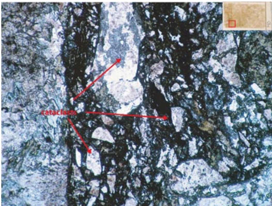
Figure 2-16. Microscope image of sample MD in normal light showing an epidote vein which is actually a microscopic cataclastic shear zone. The image width is 4 mm.
