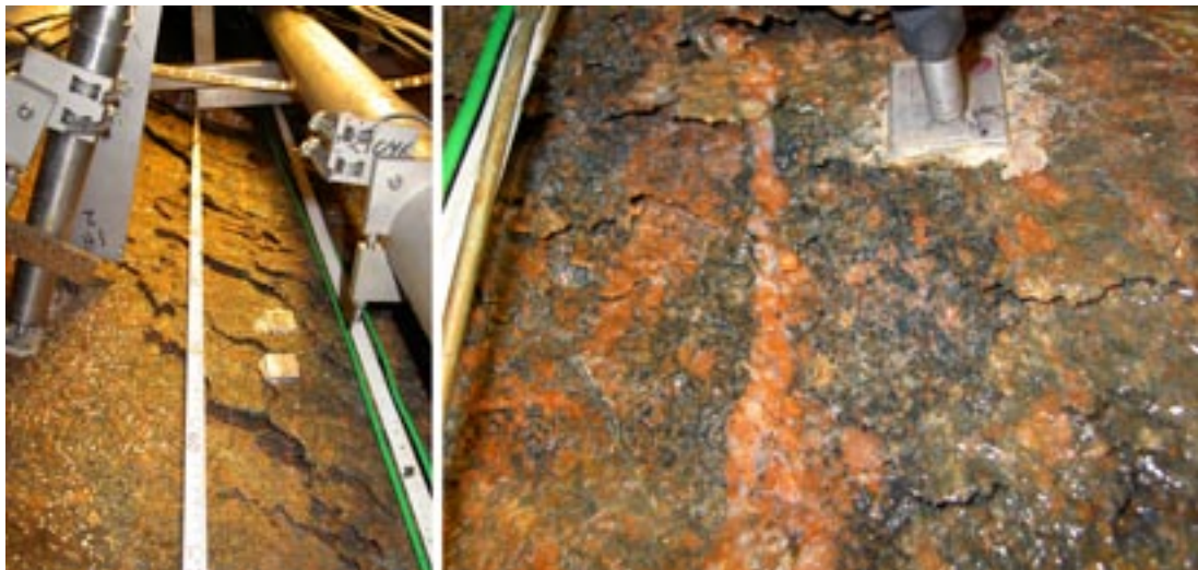
Figure A2e-17. June 23. Photographs of spalling/fracturing at position 3 on the 2.5 m level (left) and at position 10 on the 3 m level (right).
