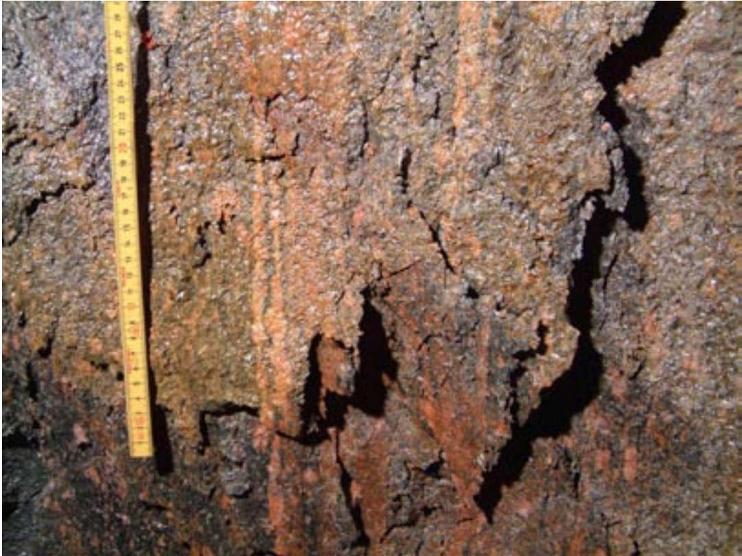
Figure A2e-27. Photograph of rock wall at depth of approximately 4 m. The small cm-scale chips on top of the larger chips are clearly visible.
