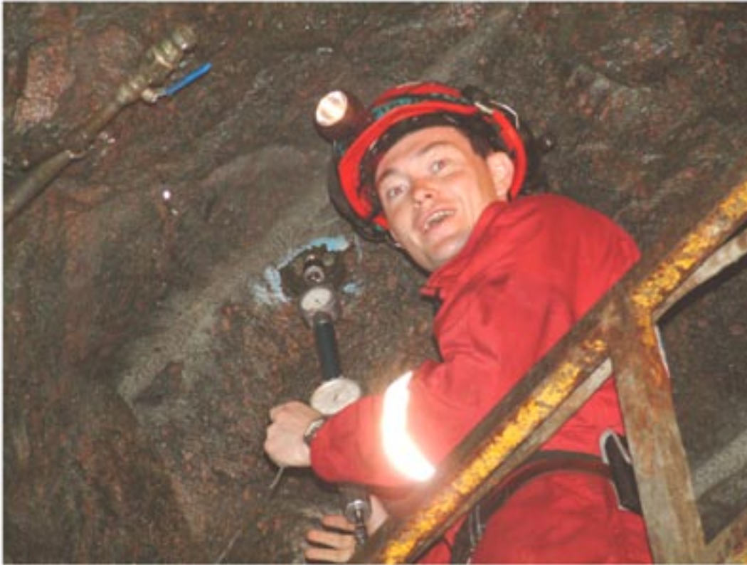
Figure 2-21. The convergence was measured with a Kern Distometer. The convergence pins were installed approximately 0.5 m behind the face.
