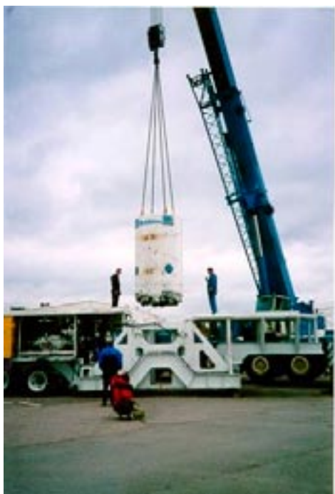
Figure 3-3. Fitting of the cutter head into the frame. The converted TBM machine used for the excavation of the 1.75-m-diameter holes.
