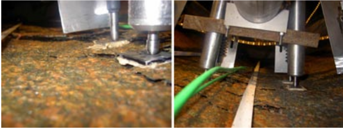
Figure A2e-4. May 18. Photographs of the pillar wall. Left: close-up of position 3 (2.5 m level); the short-range LVDT is the lower one. Right: photograph from below along the centre of the pillar (pos. 3 to the left and pos. 4 right of the pipe).
