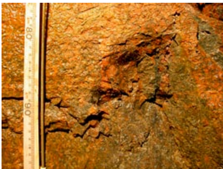
Figure 2-10. The approximate location of sample MD at a depth of 4.9 m. Note the strong oxidation.
