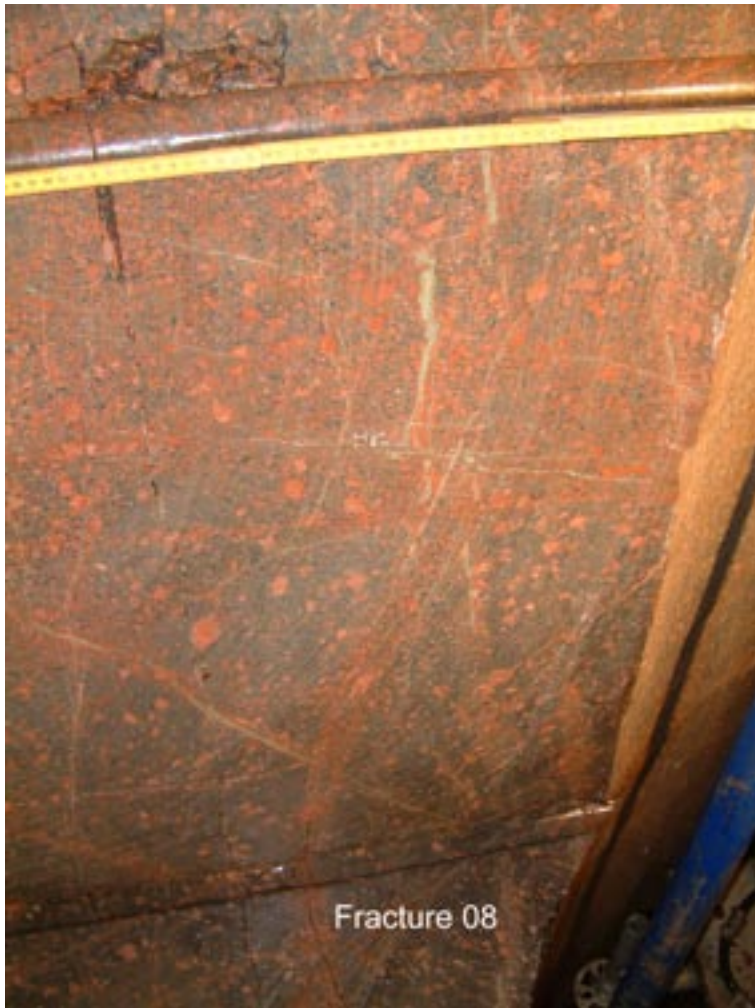
Figure 10-11. Photograph taken of fracture 08 in the remaining left wall. The drill pipe is at a depth of 4 m. The intersection between the failed zone and the pre-existing fracture indicated by the oxidized band is clearly visible.
