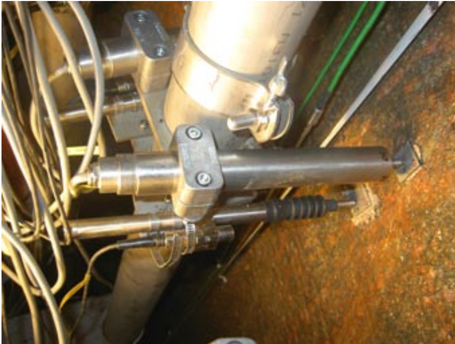
Figure 4-3. LVDTs mounted on a steel pipe in the open hole. The upper LVDT is of the short-range type and the lower of the wide-range type.
