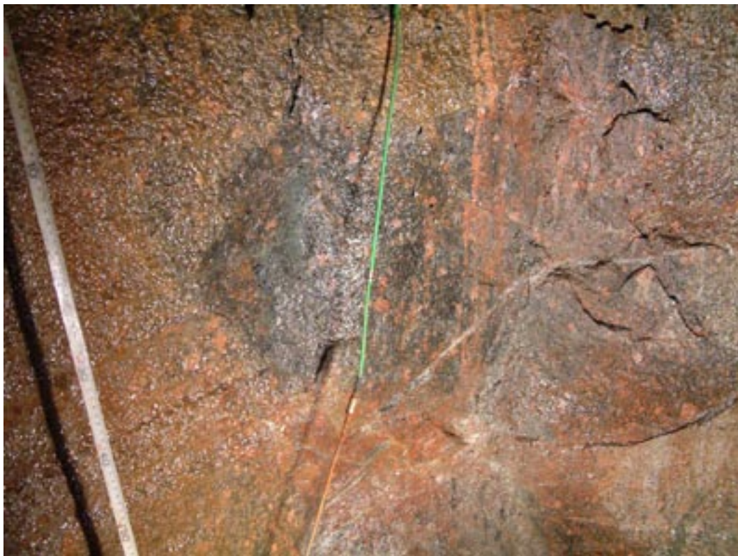
Figure A2e-25. The greenstone body that created a small pit in the rock wall.
