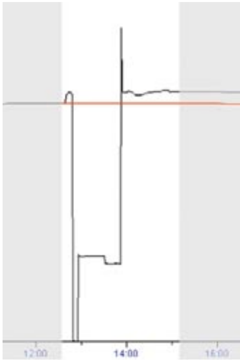
Figure 4-7. Example of the data filtering process. The white area is considered to be disturbed. The black line represents the measurement data from one sensor during the disturbed period. The red line represents the resulting data after filtering. As the figure shows, the filtering application removes the data from the disturbed time interval and the following data are adjusted to make a seamless continuous curve. The result is a data set that shows only the effective displacements during the experiment.
