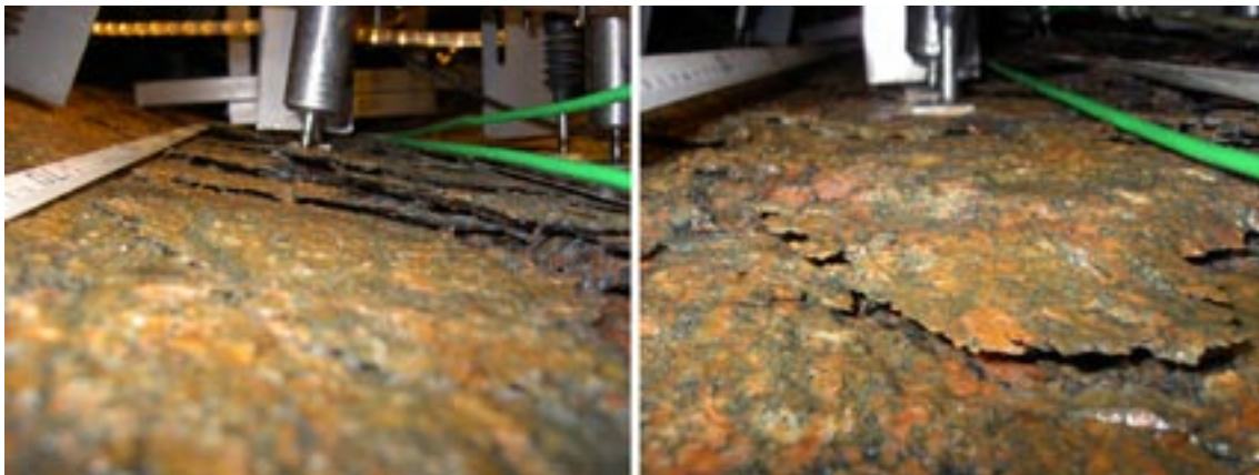
Figure A2e-15. June 16. Photographs of spalling/fracturing at position 3 on the 2.5 m level (left) and at position 9 on the 3 m level (right).
