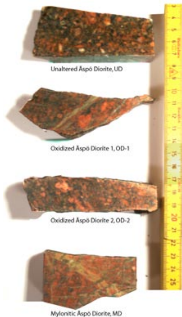
Figure 2-8. Photographs of the rock samples used to make the thin samples.
