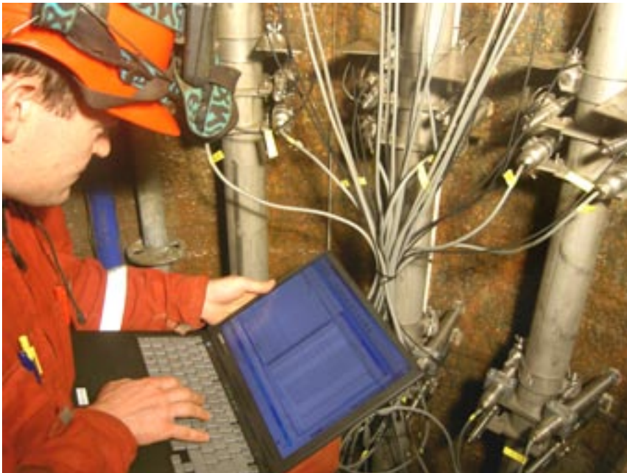
Figure 4-4. Function check of the radially mounted LVDTs after installation. A laptop connected to the Äspö LAN was brought down into the hole for immediate access to the LVDT response during the check.
