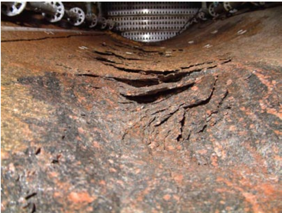
Figure A2e-28. Photograph taken from below of chips at 3.7 m and up. The dilatation and curvature of the slabs can be seen.
