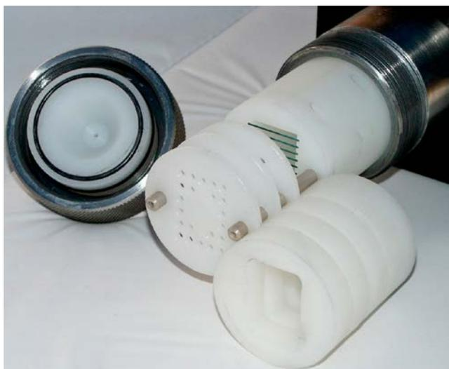
**Figure 2-7.** Mounted pressure-resistant flow cell with glass slides. Three flow diffusers distribute the flow evenly over all test surfaces in the test pile. The steel is not in contact with the groundwater.
