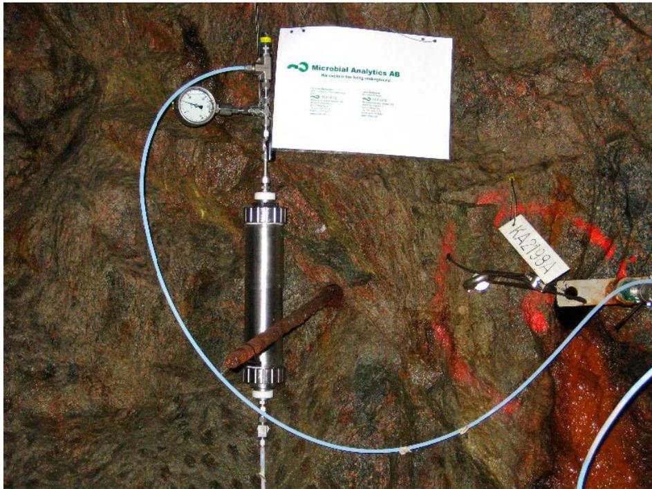
*Figure 2-10. A flow cell connected to the borehole KA2198A in the Äspö Hard Rock Laboratory tunnel, Sweden.*
