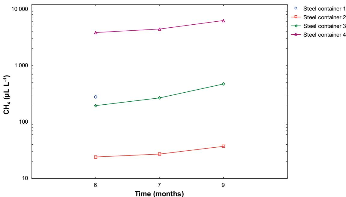
**Figure 3-4.** Methane development over time for all steel containers. For information about steel containers see Table 2-2.
