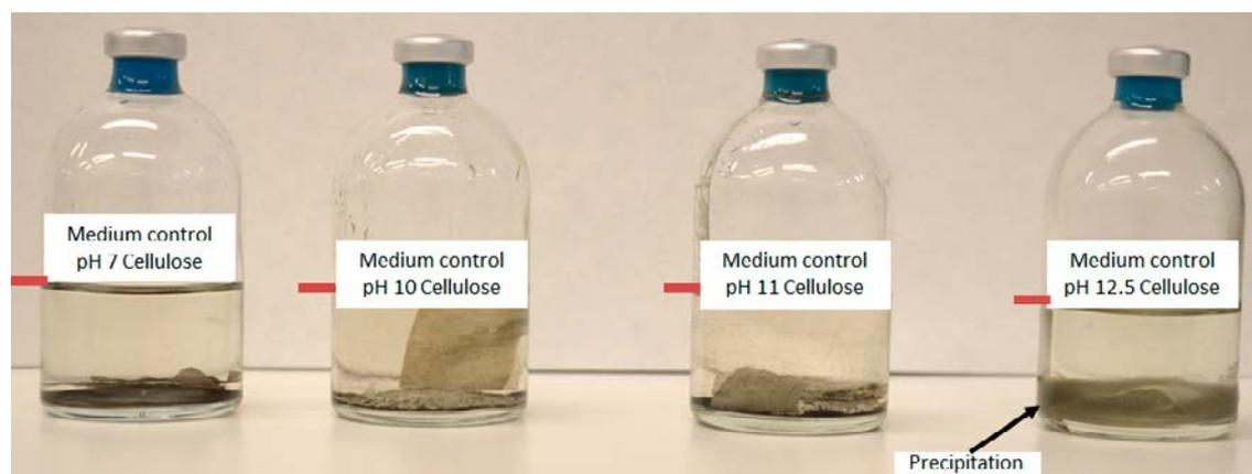
**Figure 3-1.** Serum bottles with cellulose and enrichment medium at different pH. The arrow indicates the precipitation and the red line indicates the media level.
