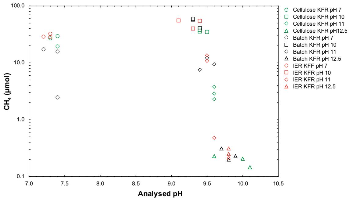
**Figure 3-3.** Analysed methane plotted against analysed pH from serum bottles after 8 weeks of incubation. The serum bottles contained 50 mL enrichment medium and were inoculated with KFR. Additionally, the serum bottles contained material (cellulose or IER). Bottles labelled “Batch” contained only medium (2.2.2). The pH in the name description indicates the expected pH. The detection limit was  $0.04 \mu\text{mol}$ .
