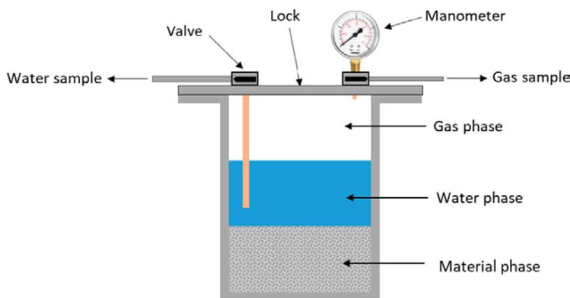
Figure 2-2. Scheme of a steel container.
