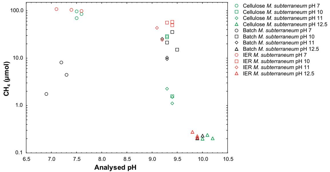
**Figure 3-2.** Analysed methane plotted against analysed pH from serum bottles after 8 weeks of incubation. The serum bottles contained 50 mL enrichment medium and were inoculated with *M. subterraneum*. Additionally, the serum bottles contained material (cellulose or IER). Bottles labelled “Batch” contained only medium (2.2.2). The pH in the name description indicates the expected pH. The detection limit was  $0.04 \mu\text{mol}$ .
