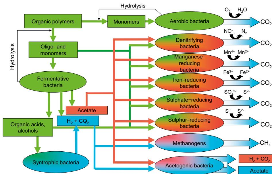
**Figure 1-4.** Possible pathways for the flow of carbon in the subterranean environment. Organic carbon is respired with oxygen, if present, or else fermentation and anaerobic respiration occur with an array of different electron acceptors (Pedersen 2000).
