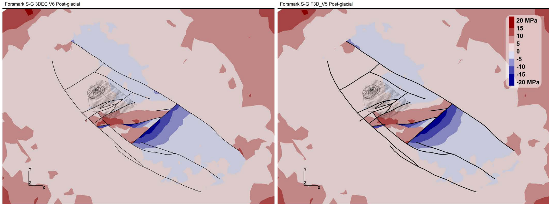
Figure A14-4. Horizontal cross sections at repository depth -470 m of the maximum principal stress magnitude difference to the Martin (2007) interpretation after glaciation in an elastoplastic simulation. The reference value is case-dependent.
