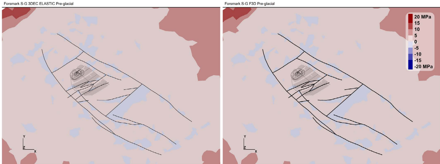
Figure A18-1. Horizontal cross sections at repository depth -470 m of the minimum principal stress magnitude difference to the Martin (2007) interpretation before glaciation in a fully elastic simulation. The reference value is case-dependent.
