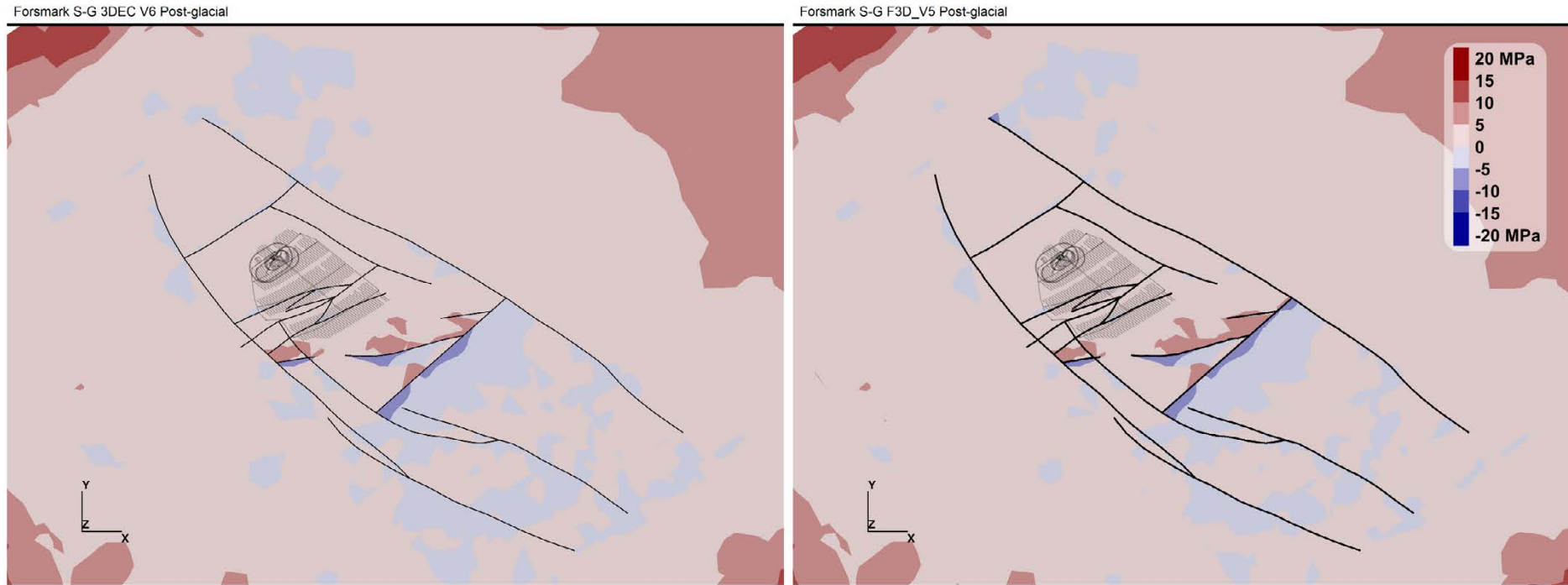
Figure A16-4. Horizontal cross sections at repository depth -470 m of the intermediate principal stress magnitude difference to the Martin (2007) interpretation after glaciation in an elastoplastic simulation. The reference value is case-dependent.
