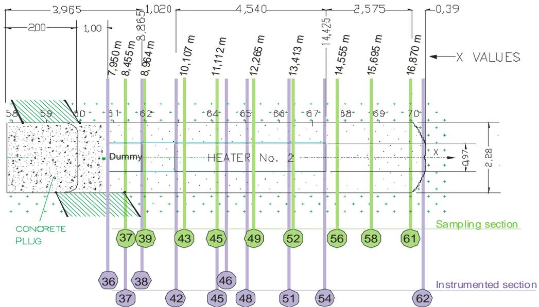
Figure 3: General layout of the *in situ* test during the 2<sup>nd</sup> operational phase and location along the gallery of the sampling sections used for bentonite water content and dry density on-site determinations
