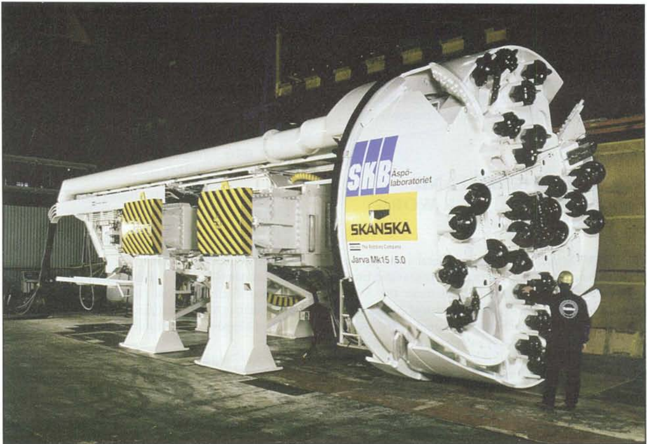
Figure 17-4. The 5m diameter TBM-machine is an ATLAS COPCO Mk 15 with special features for the Äspö application.
