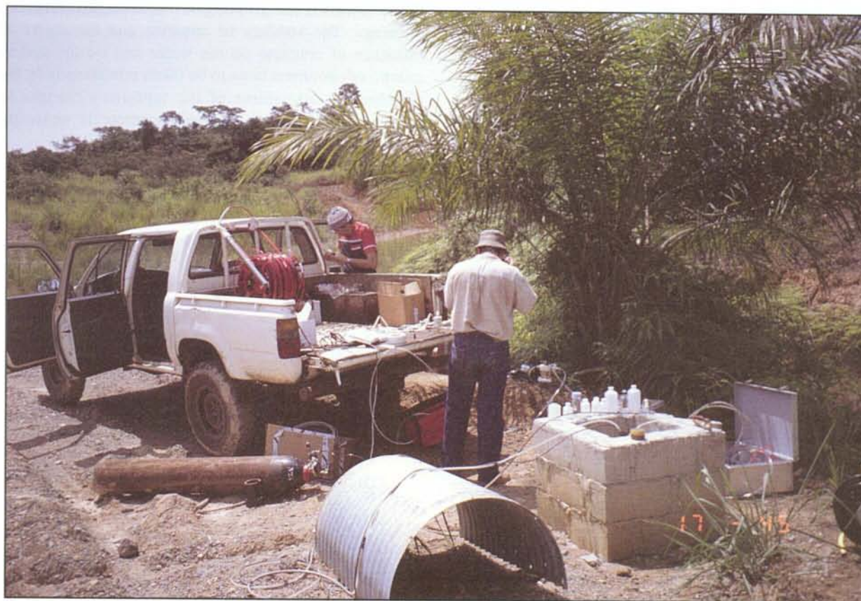
Figure 15.6-3. The Bangombe site. Sampling of groundwater from a packed off section of a vertical borehole.
