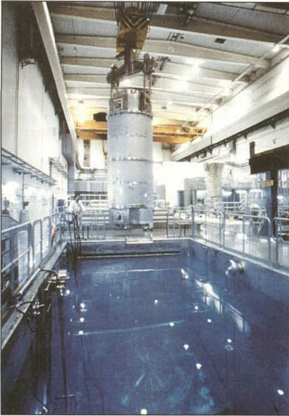
Figure 2-2. Fuel cask with protective shirt being moved from the cooling cell to the unloading pool.
