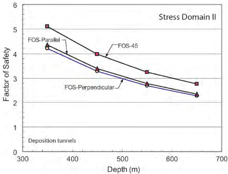
**Figure 4-12.** Factor of safety against spalling for a deposition tunnel in stress domain II as a function of depth, for the three different tunnel orientations ( $0^\circ$ ,  $45^\circ$  and  $90^\circ$  to the maximum horizontal stress direction) /Martin 2005/.
