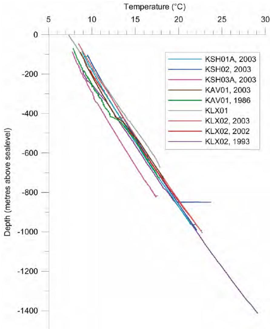
**Figure 4-5.** Measured temperature as a function of depth, from boreholes in the Simpevarp-Laxemar local model area /SKB 2005a/.
