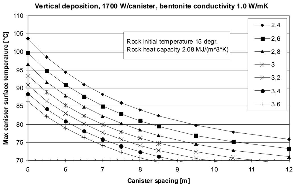
Figure 4-4. Maximum canister surface temperature vs canister spacing for varying values of rock thermal conductivity /SKB 2004a/.
