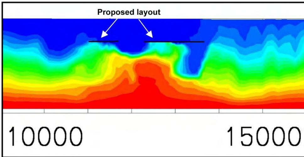
**Figure 7-12.** Salinity distribution in the groundwater- grouting factor 0.1. Vertical profile W-E. Salinity, % Total Dissolved Solids (TDS).
