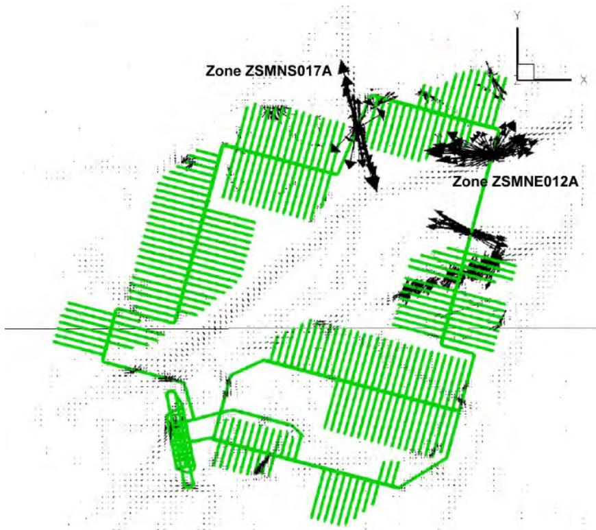
*Figure 7-3. Seepage into the repository at -515 m depth (representative depth for the repository's northern part). Seepage into the tunnels is concentrated at the deformation zone intercepts.*
