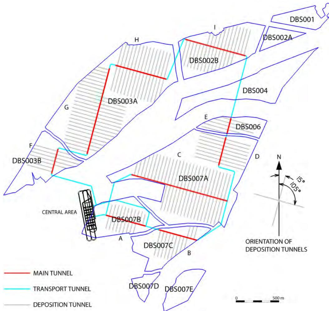
**Figure D4-1.** Originally proposed layout based on deformation zones according to SDM Simpevarp 1.2.
