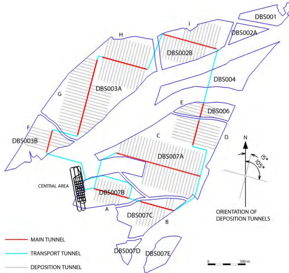
**Figure 5-1. Layout. Level –500 m.**
