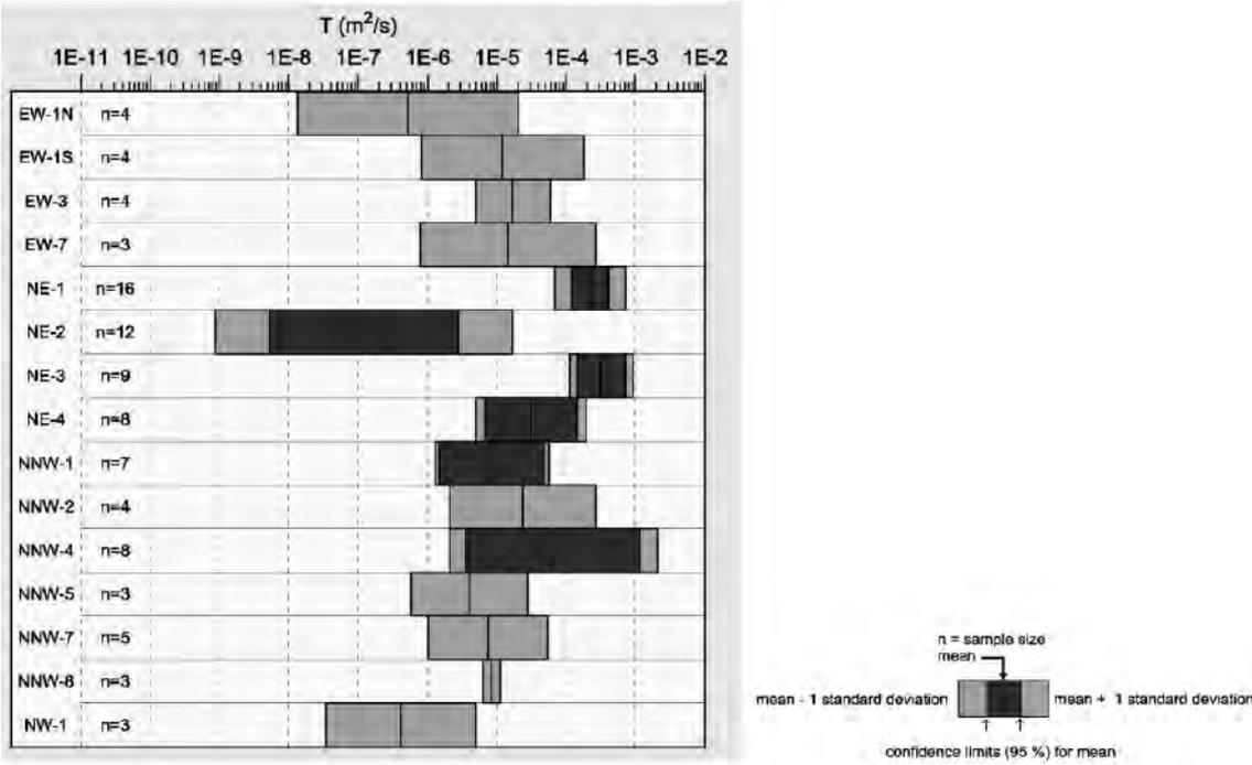
Figure 6-11. Compilation of measured transmissivity values for deformation zones encountered during the excavation of Äspö HRL access tunnel /Rhén et al. 1997/.
