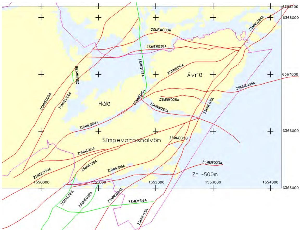
**Figure D2-2.** Deterministically interpreted deformation zones according to SDM Laxemar 1.2. Zones with a high level of confidence are marked with red lines and zones with a medium level of confidence with green lines. Level -500 m /SKB 2006a/.
