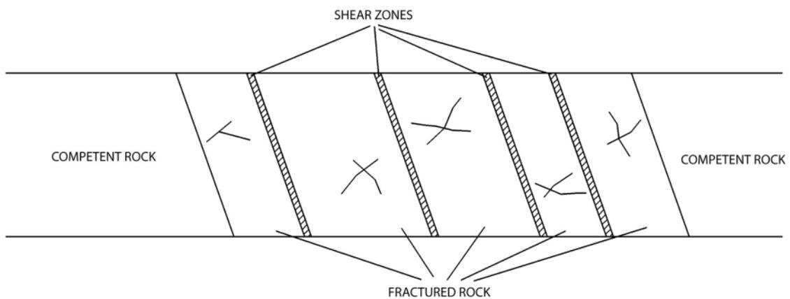
**Figure 6-5.** Schematic figure representing a Type C deformation zone geometry.
