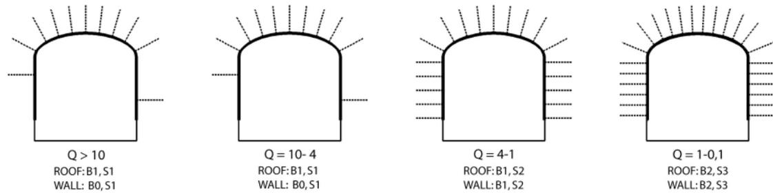
Figure B-3. Principle drawing of support for rock halls.
