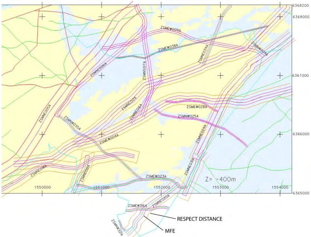
**Figure 3-5.** RD and MFE for deterministic deformation zones lying within the study area. Level -400 m.
