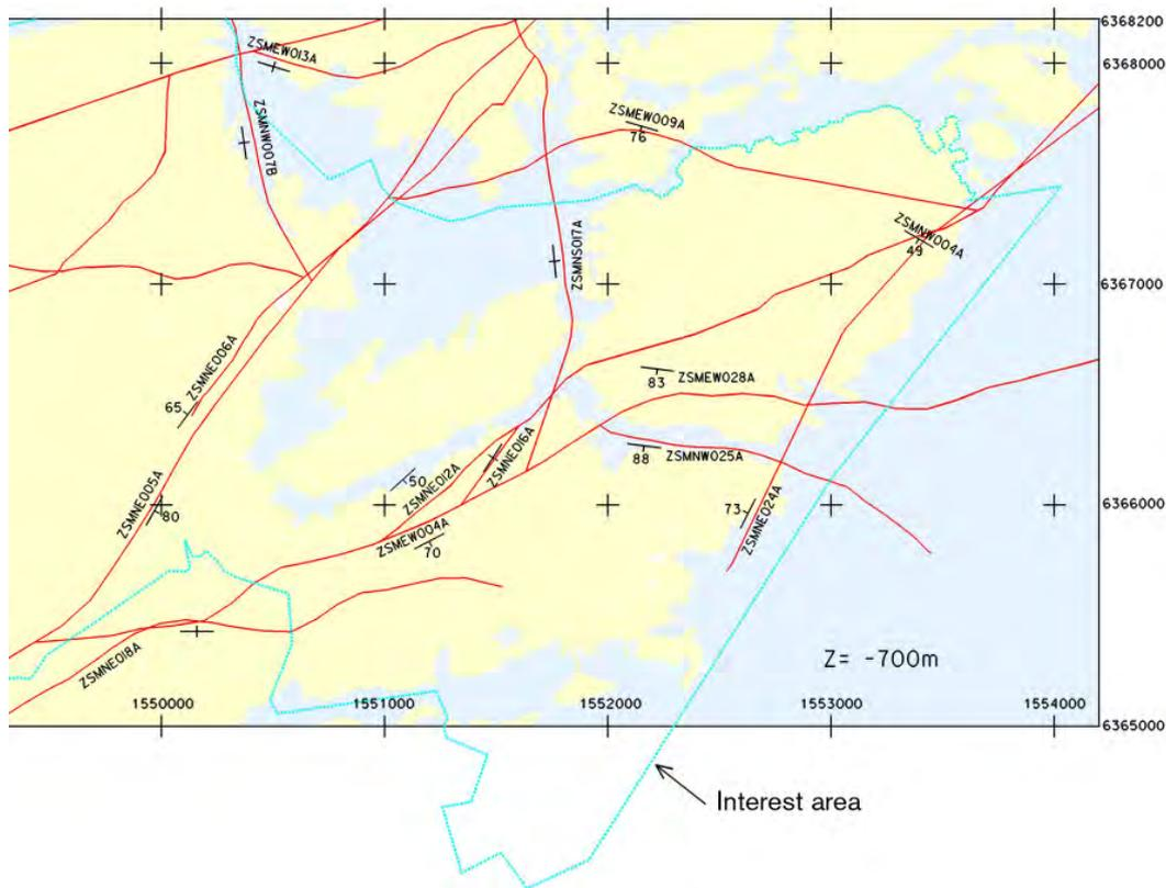
**Figure 3-4.** Deformation zones level  $-700\text{ m}$ . High confidence zones are shown in red, /SKB 2005a/.
