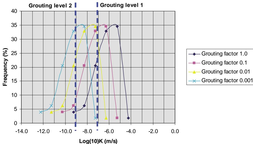
**Figure 7-2.** Distribution of hydraulic conductivity for different grouting factors involving calculation cells that intercept the tunnel geometry.
