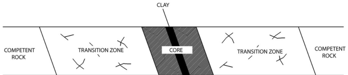
**Figure 6-3.** Schematic figure representing a Type A deformation zone geometry. Modified after /Chang et al. 2005/.
