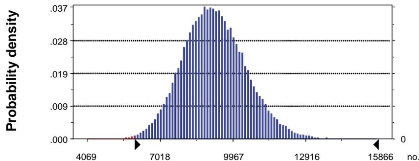
**Figure 10-3.** Forecast: Number of canister positions, Frequency Chart, 100,000 trials. Certainty is 99.75% from 6,000 to +Infinity.
