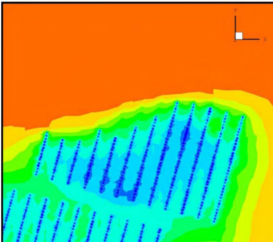
*Figure 7-9. Pressure distribution around the deposition holes for a grouting factor of 0.1. Dark blue represents atmospheric pressure. The figure shows the NE part of the repository at level  $-515$  m.*
