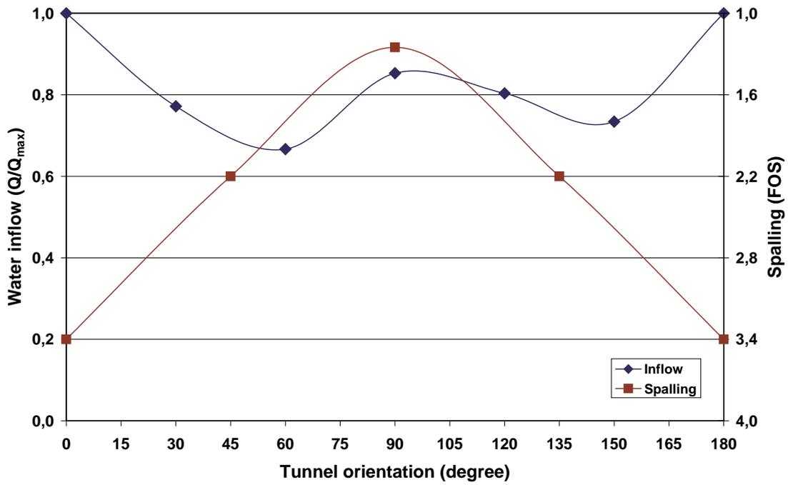
**Figure 4-15.** Compilation of water inflow and spalling risk (FOS = Factor of Safety) for stress domain I at a storage depth -500 m. The tunnel orientation is shown relative to the maximum horizontal stress.
