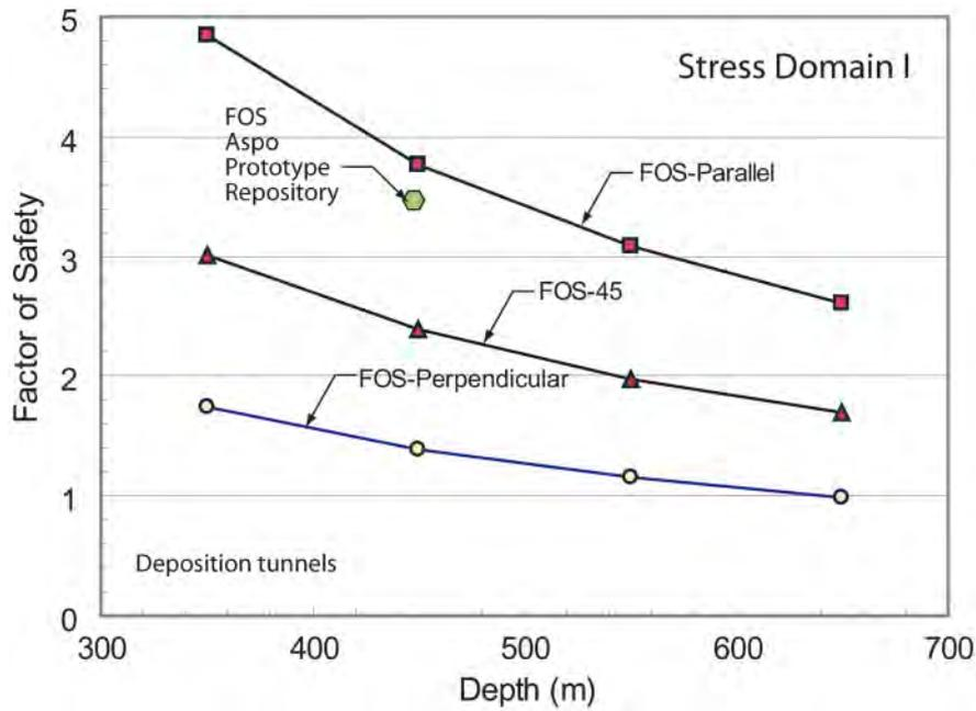
**Figure 4-11.** Factor of safety against spalling for a deposition tunnel in stress domain I as a function of depth, for the three different tunnel orientations ( $0^\circ$ ,  $45^\circ$  and  $90^\circ$  to the maximum horizontal stress direction). Also shown, for reference purposes, is the the TBM tunnel at Äspö at a depth of 450 m. This tunnel is oriented approximately  $30^\circ$  from the maximum horizontal stress. No spalling was observed in the TBM tunnel. /Martin 2005/.
