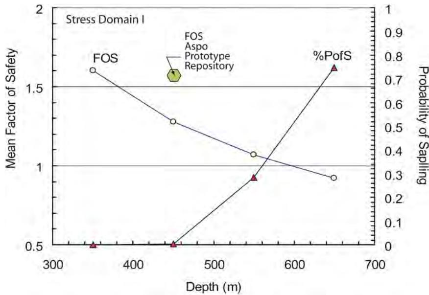
**Figure 4-18.** Factor of safety and probability of spalling in deposition holes in stress domain I. The factor of safety for the deposition hole in the prototype repository in Äspö HRL is shown as a reference. When drilled this hole did not show any signs of spalling /Martin 2005/.
