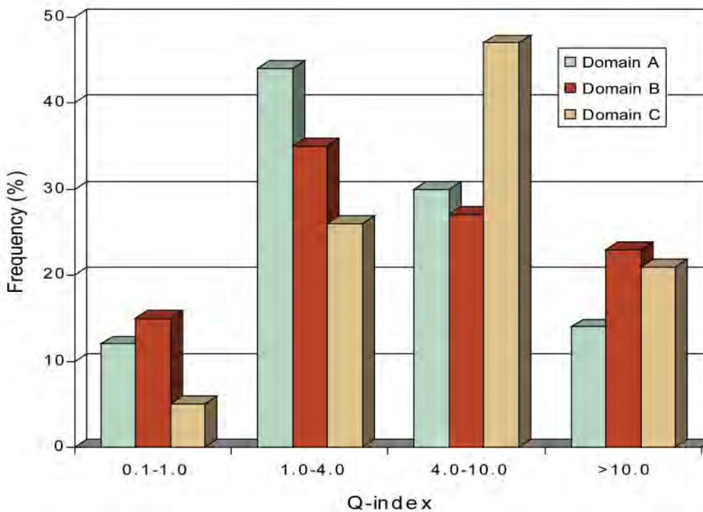
**Figure 9-4.** Estimated rock quality in stochastic deformation zones as a function of frequency and rock domain based on mapping of drill core within the Simpevarp area /Lanaro 2005/.
