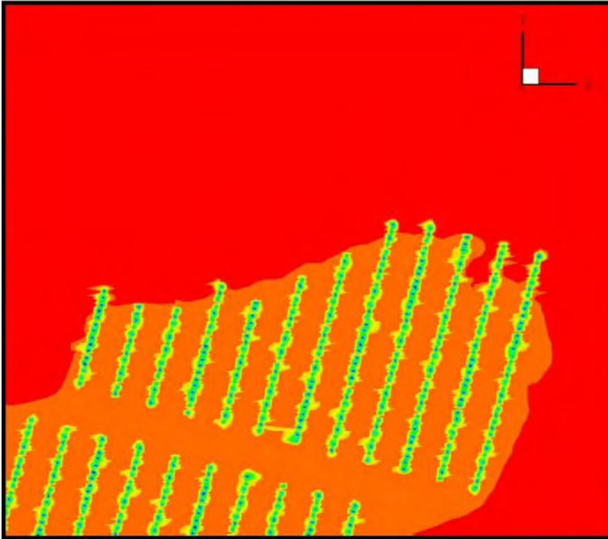
**Figure 7-10.** Pressure distribution around the deposition holes for a grouting factor of 0.001. Dark blue represents atmospheric pressure. The figure shows the NE part of the repository at level -515 m.
