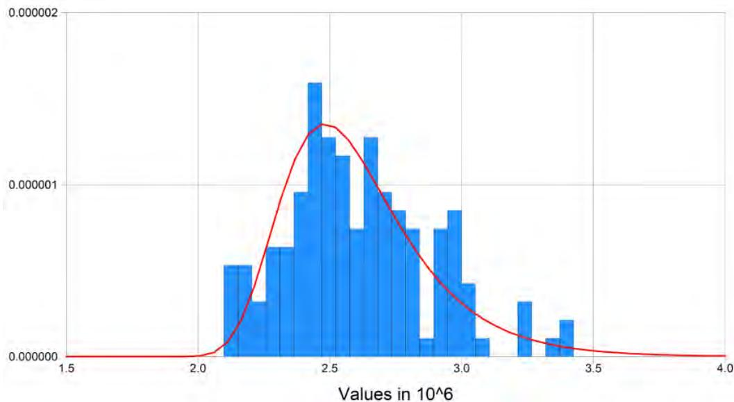
**Figure 10-8.** Forecast: Probability density function of volume of rock spoil from blasting, 6,000 canister positions, Unit:  $t\text{fm}^3$ . Histogram based on 141 values. An adapted extreme value distribution is also shown (Mode  $2.48E+6$ ; Scale  $2.17E+5$ ).
