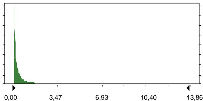
**Figure C-5.** Assumed distribution for percentage loss of deposition holes due to too much in-leaking water.
