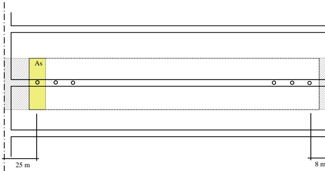
**Figure C-6.** Background for modification factor with regard to end effects in deposition tunnels.
