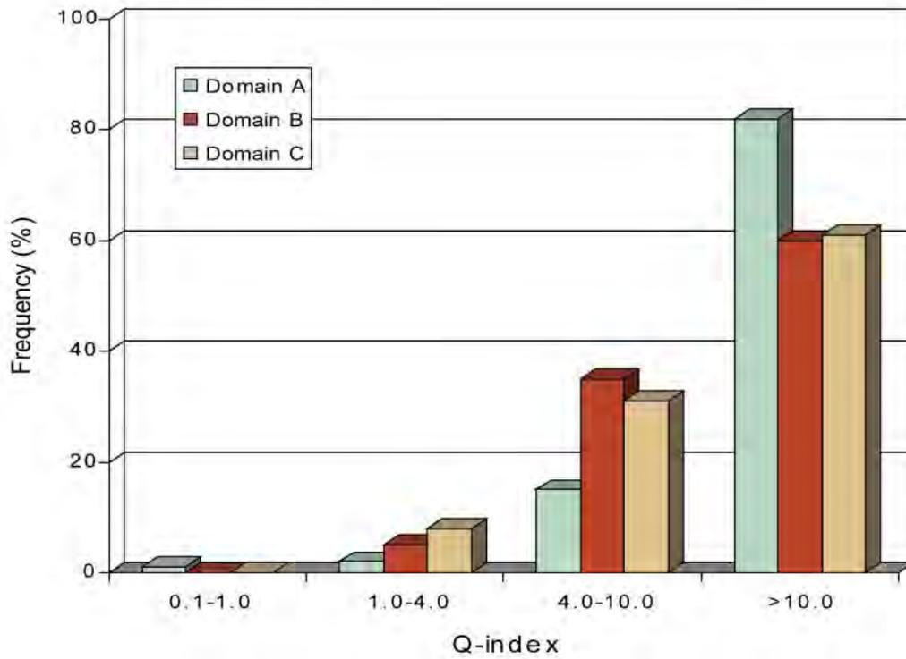
**Figure 9-3.** Estimated rock quality in competent rock as a function of frequency and rock domain based on mapping of drill core within the Simpevarp area /Lanaro 2005/.
