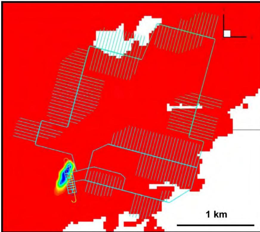
*Figure 7-8. Groundwater level for a grouting factor of 0.01. Horizontal section at level  $-1$  m. Red represents where the groundwater table is at or above level  $-1$  m.*
