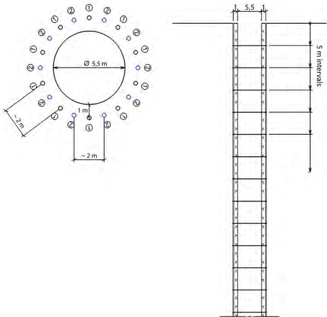
*Figure A-3. Proposed grouting scheme drill hole layout for shafts in rock blocks, grouting level 2.*
