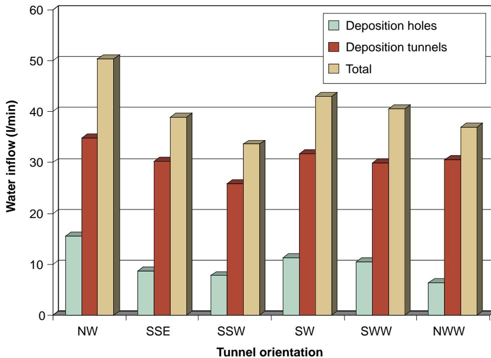
Figure 4-10. Mean water inflow to deposition holes and deposition tunnel as a function of tunnel orientation.
