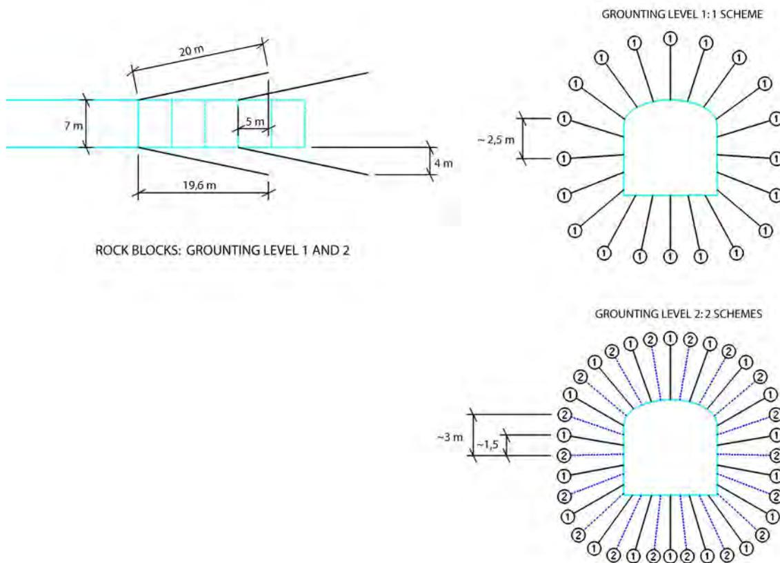
**Figure A-1.** Proposed layout of the grouting scheme for transport tunnels located in rock blocks, grouting levels 1 and 2.
