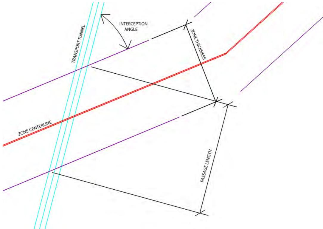
**Figure 6-2.** Definition of zone thickness, interception angle and passage length used in Table 6-1.
