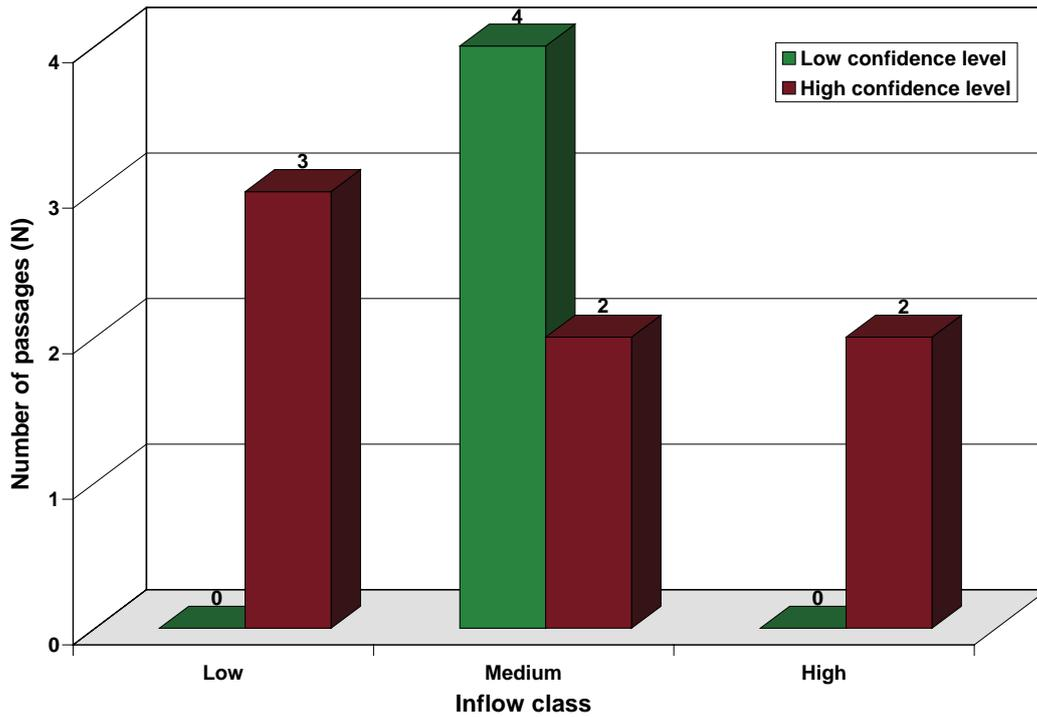
*Figure 6-9. The number of passages as a function of water inflow potential and zone confidence, assuming no grouting.*
