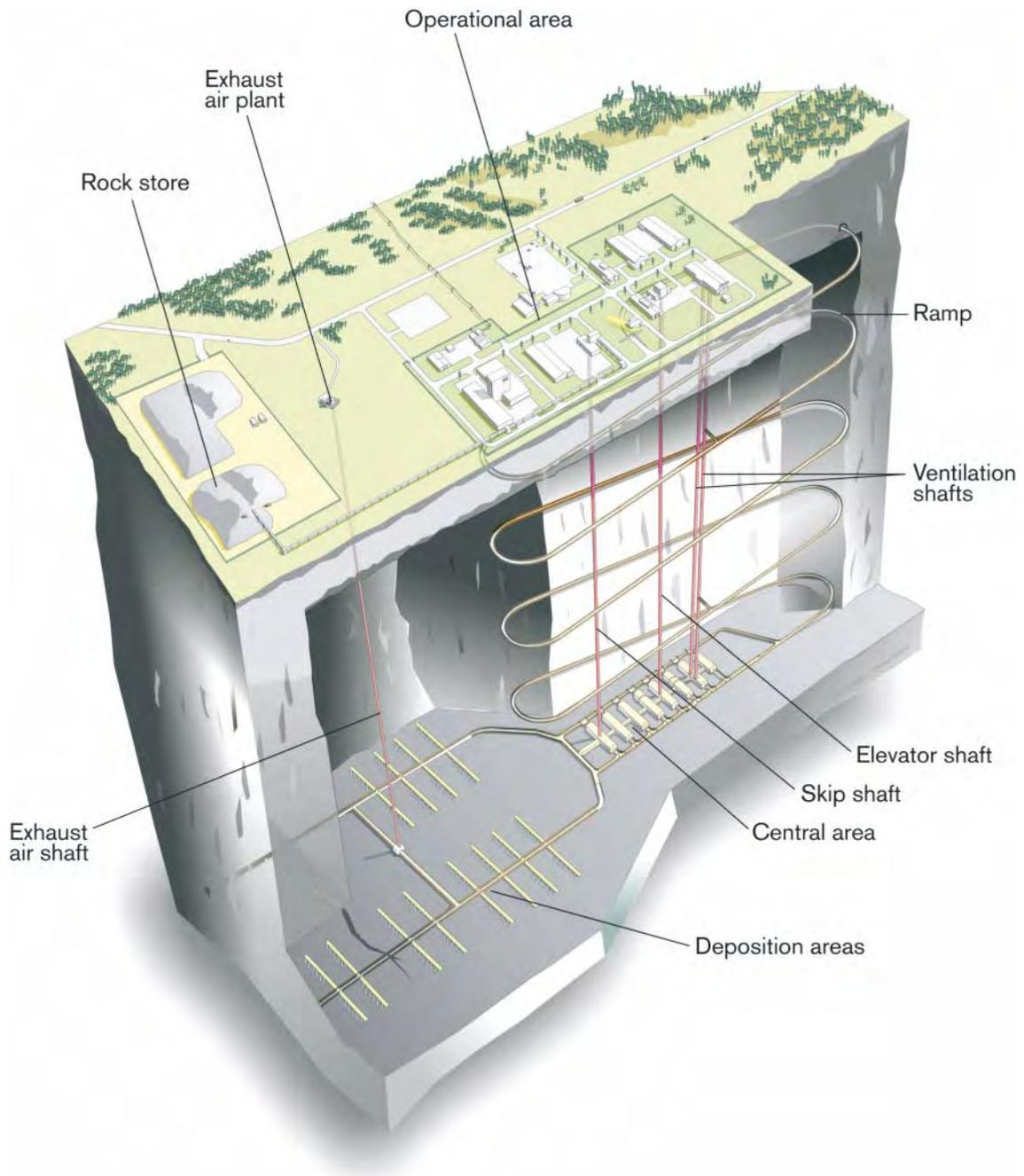
**Figure 1-1.** 3D-illustration of surface and underground facilities.
