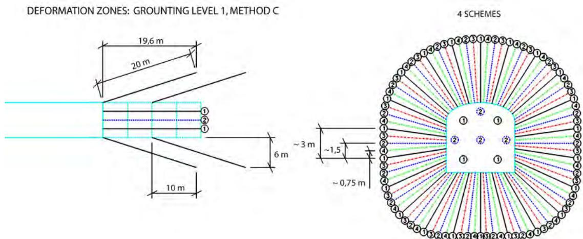
**Figure A-5.** Proposed grouting scheme drill hole layout for transport tunnel-deformation zone intercepts, in accordance with method C and grouting level 1. Four stages of grouting presented.
