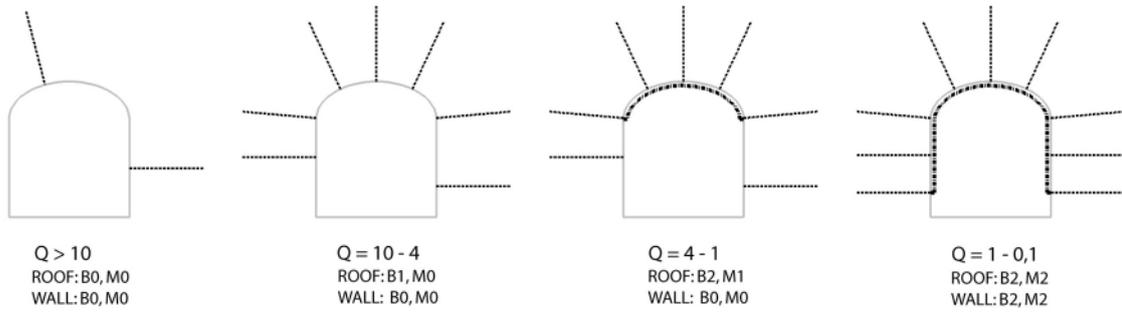
Figure B-1. Principle drawing of support for deposition tunnels.
