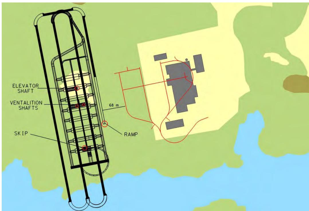
**Figure 5-3.** Layout showing the central area, shafts and ramp along with CLAB's existing surface buildings (grey) and tunnel centre lines (red).
