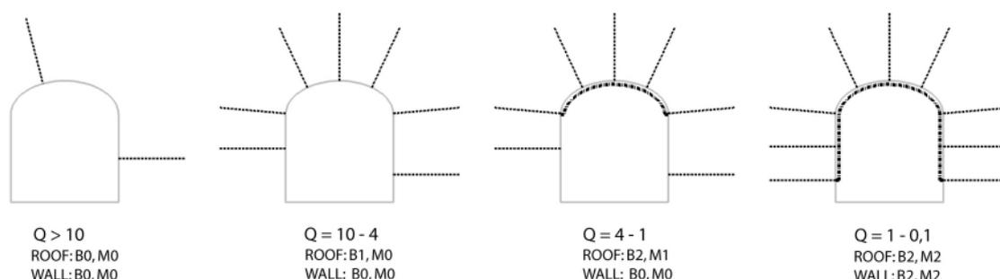
**Figure 9-6. Principle rock support for deposition tunnels.**
