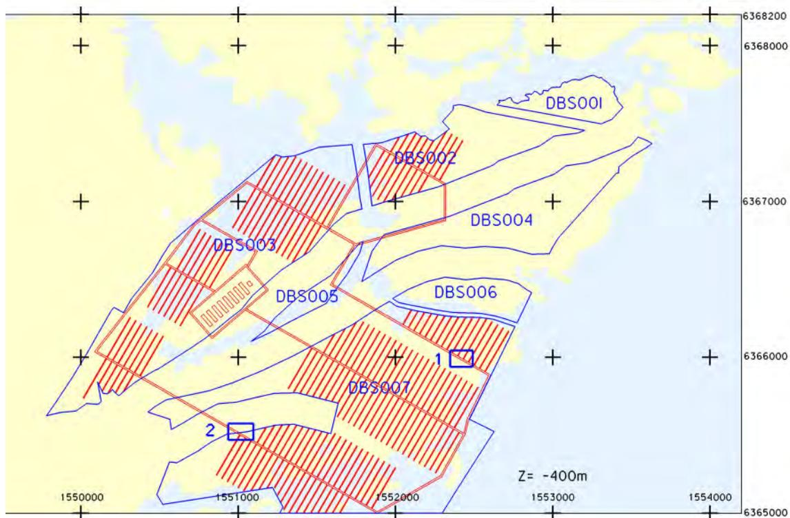
*Figure 5-5. Layout with the central and operational areas located on Hålö. It should be noted that the layout shown was developed during an earlier preliminary design stage. Potential locations for the ventilation shaft and building are marked 1 and 2.*
