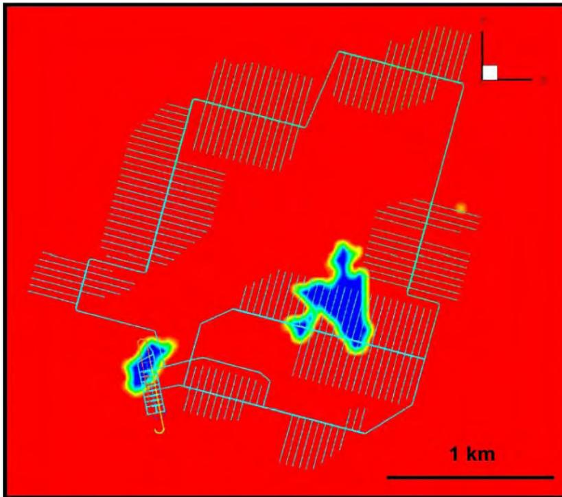
**Figure 7-5.** Groundwater level for grouting factor of 0.1. Horizontal section at level  $-100$  m. Red represents where the groundwater table is at or above level  $-100$  m. Blue represents the drawdown.
