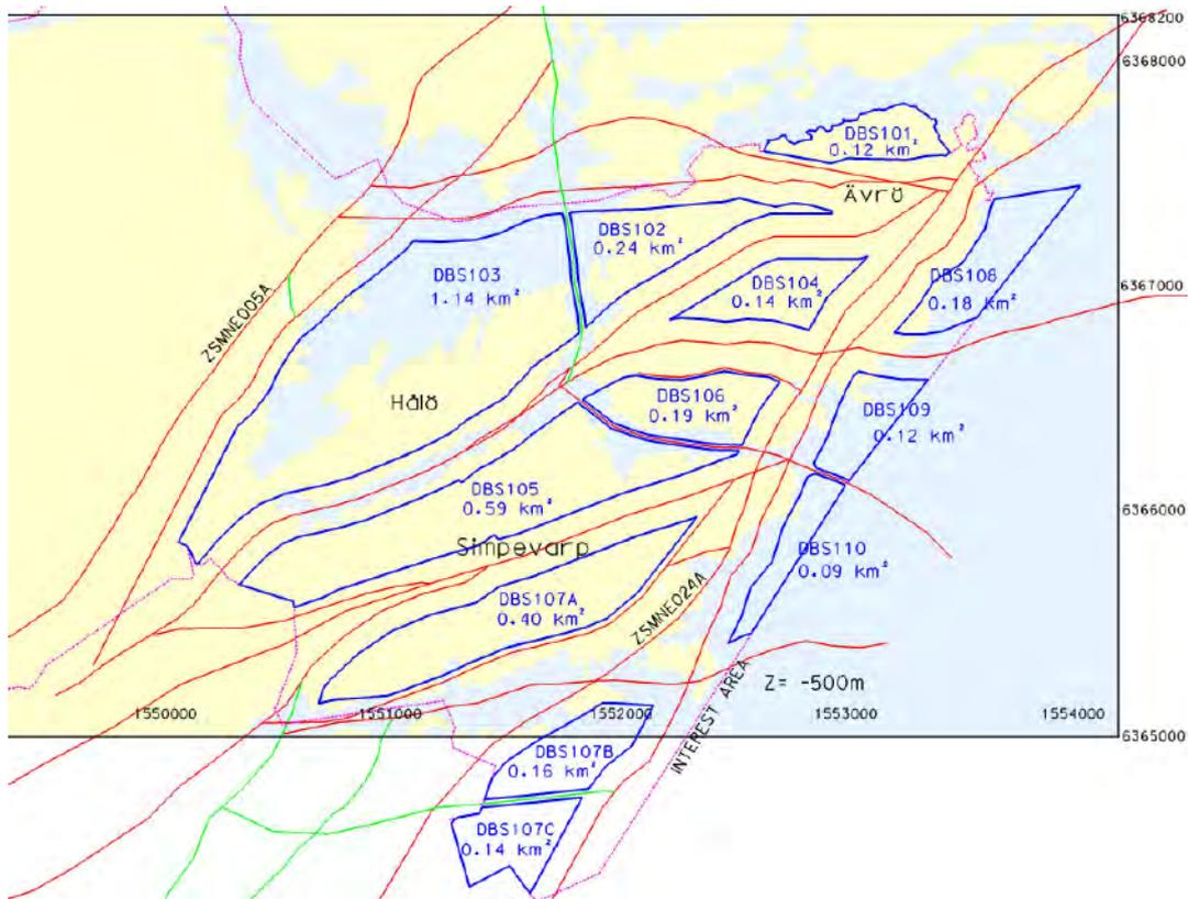
**Figure D2-6.** Areas and shapes of deposition blocks in Simpevarp based on SDM Laxemar 1.2. Zones with a high level of confidence are marked with red lines and zones with a medium level of confidence with green lines. Level -500 m /SKB 2006a/.
