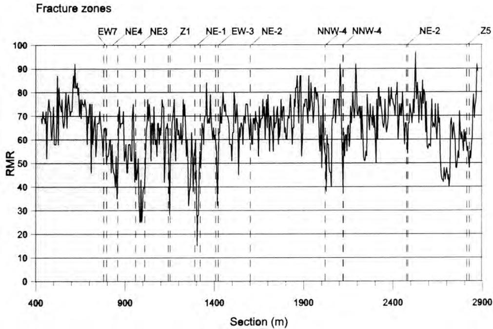
**Figure 6-8.** Compilation of values for  $RMR_{76}$  mapped from the Äspö tunnel change 450–2,875 /Stanfors et al. 1997/.
