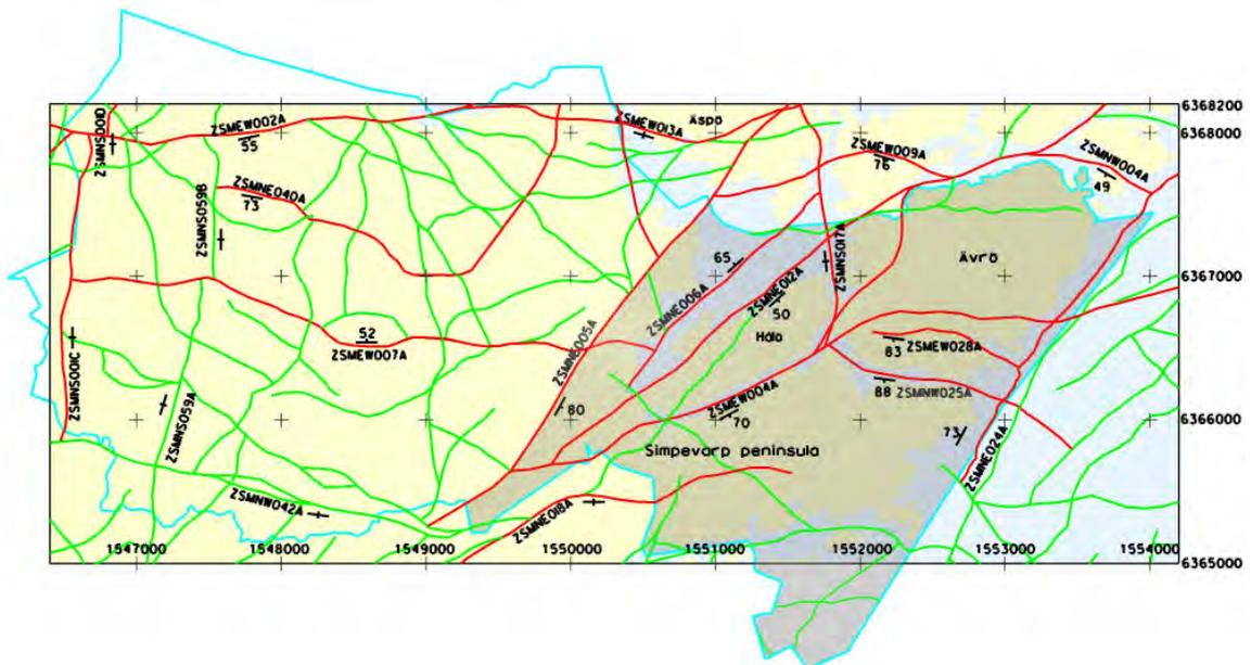
**Figure 3-1.** Local model area Simpevarp v 1.2, Interest area for the storage facility and the current study area shown in grey. The red and green lines represent the deformation zones. (Section level at  $z = 0$  m).
