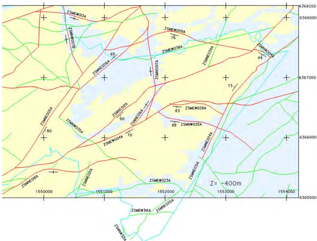
**Figure 3-3.** Deformation zones, level –400 m. High confidence zones are shown in red, “possible” zones in green /SKB 2005a/.
