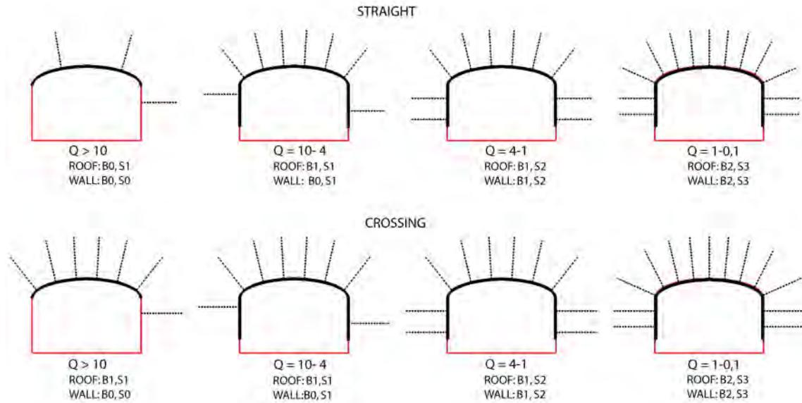
Figure B-2. Principle drawing of support for main tunnels.
