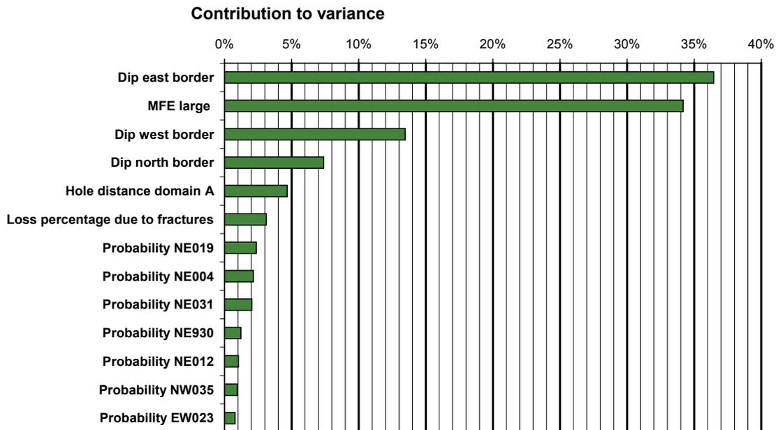
**Figure D5-2.** Factors ranked according to their relative contribution to the uncertainty in the analysis. Refers to the analysis of the number of approved canister positions with eastern border line of ZSMNE024A.
