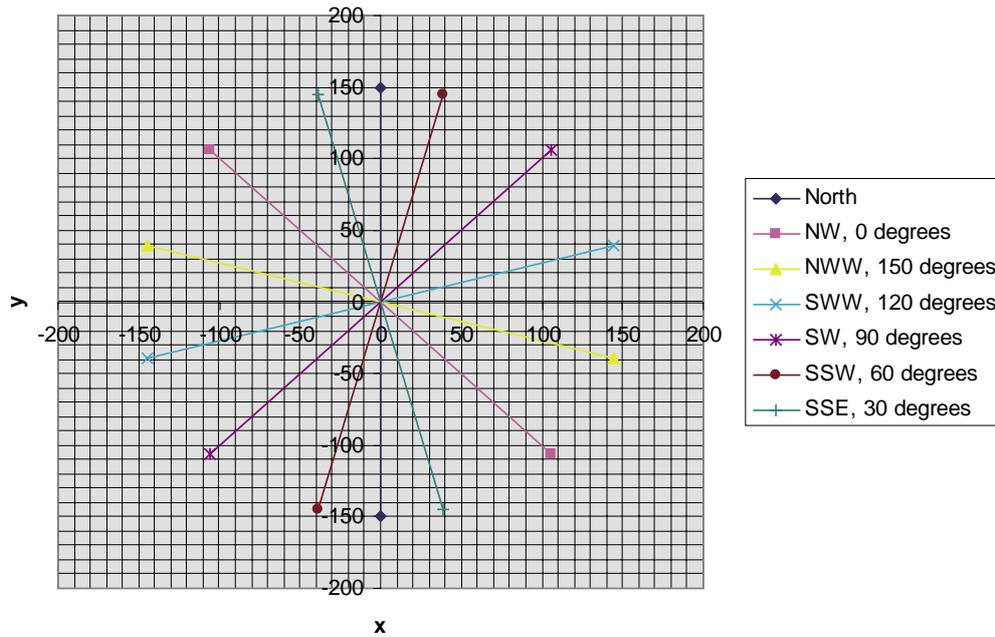
**Figure 4-8.** Tunnel orientations studied in the DFN analysis. The tunnel is rotated clockwise from NW-SE, the orientation of the major horizontal principal stress, in 30° intervals.
