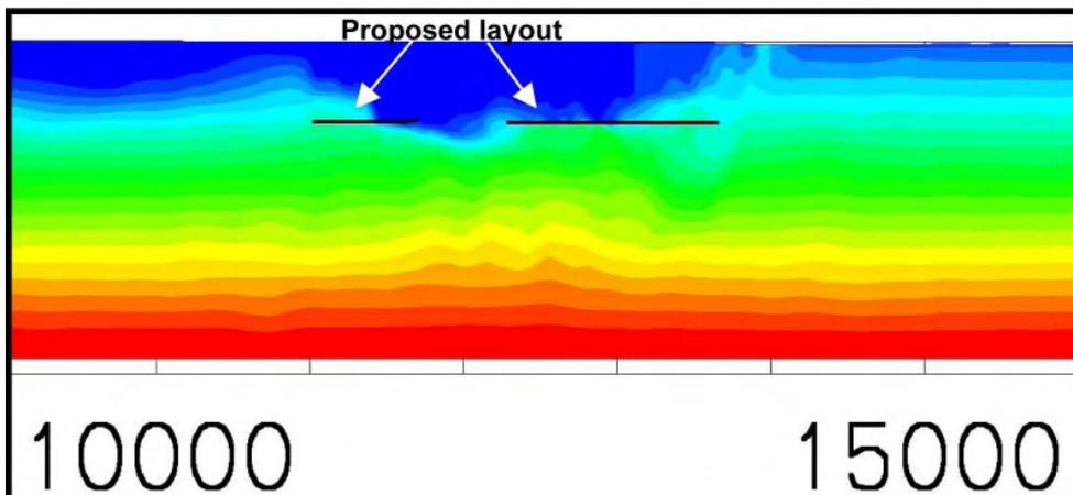
**Figure 7-14.** Salinity distribution in the groundwater- grouting factor 0.001. Vertical profile W-E. Salinity, % Total Dissolved Solids (TDS).
