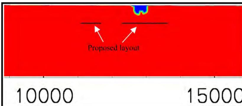
**Figure 7-6.** Vertical section W-E showing the groundwater table drawdown for a grouting factor of 0.1. Maximum drawdown approximately level  $-250$  m.
