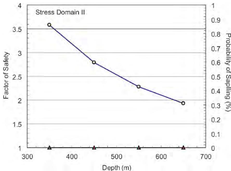
**Figure 4-19.** Factor of safety and probability of spalling in deposition holes in stress domain II /Martin 2005/.
