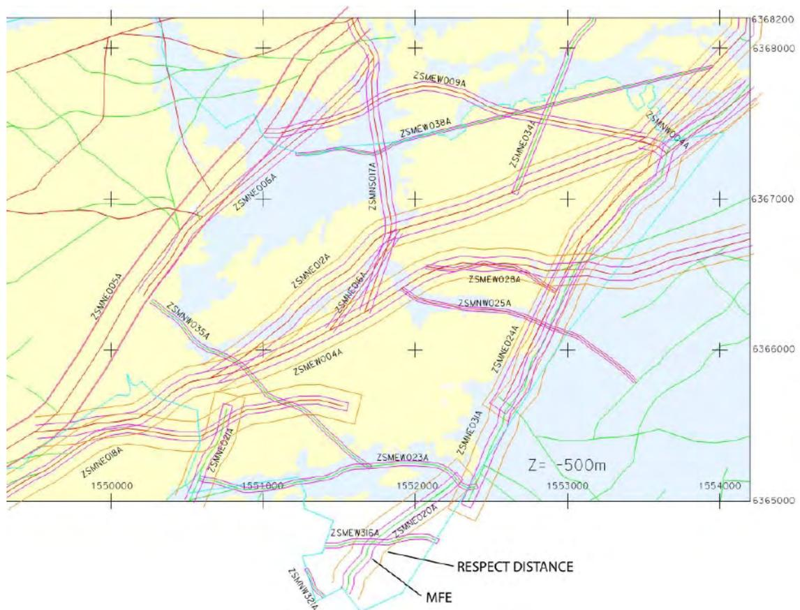
**Figure D2-3.** Representation of RD and MFE for deterministically interpreted zones based on SDM Simpevarp 1.2. Zones with high level of confidence are marked with red lines and possible zones with green lines. Level -500 m /SKB 2005a/.
