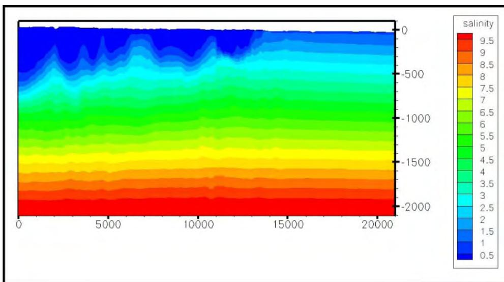
**Figure 7-11.** Salinity distribution in the groundwater- undisturbed natural conditions. Vertical profile W-E. Salinity, % Total Dissolved Solids (TDS).
