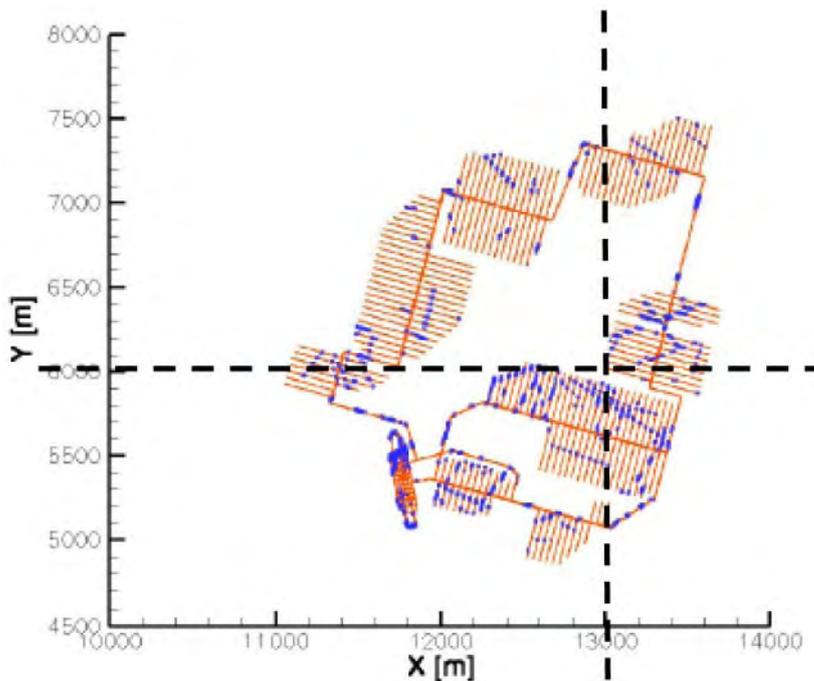
**Figure 7-1.** Results from a single simulation of the proposed repository layout, -500 m level. Blue represents intercepts between the layout geometry and the generated fractures. Dashed lines show vertical section positions.
