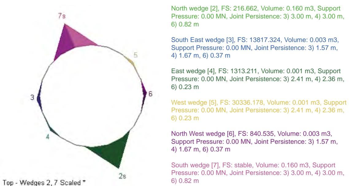
**Figure 4-17.** Result output for fracture combinations 3, 4, 6, judged to be most critical of the different combinations analysed
