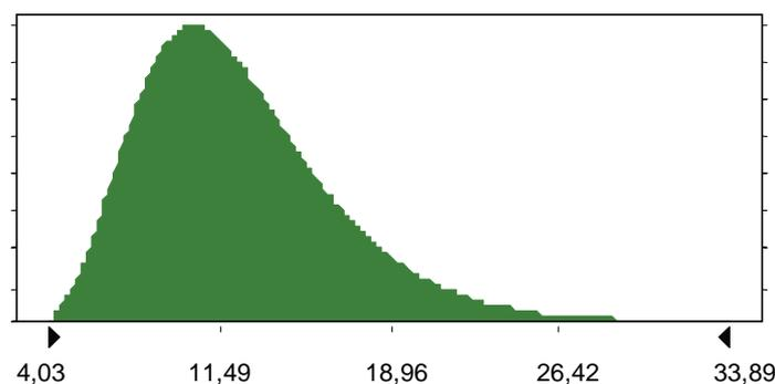
**Figure C-4.** Assumed distribution of percentage loss of deposition holes due to adjacent large fractures.
