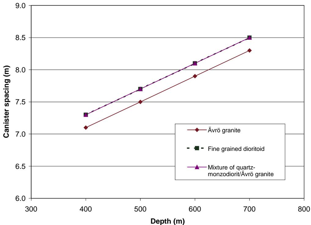
*Figure 4-6. Minimum allowable canister spacing as a function of storage depth, based on mean values of thermal conductivity for each rock domain.*
