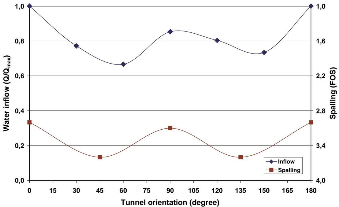
**Figure 4-16.** Compilation of water inflow and spalling risk (FOS = Factor of Safety) for stress domain II at a storage depth -500 m. The tunnel orientation is shown relative to the maximum horizontal stress.
