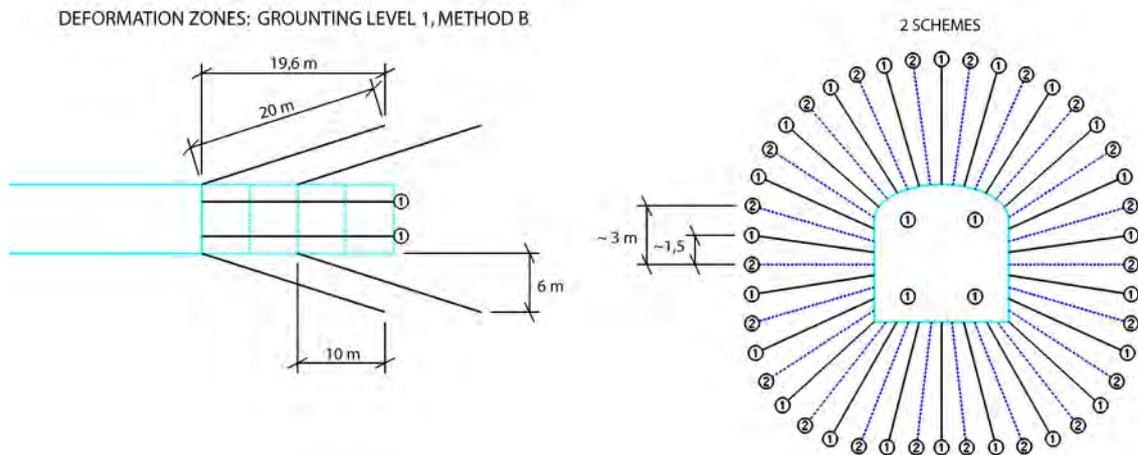
**Figure A-4.** Proposed grouting scheme drill hole layout for transport tunnel-deformation zone intercepts, in accordance with method B and grouting level 1.
