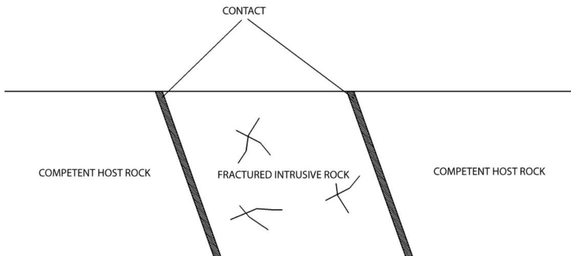
**Figure 6-4.** Schematic figure representing a Type B deformation zone geometry.
