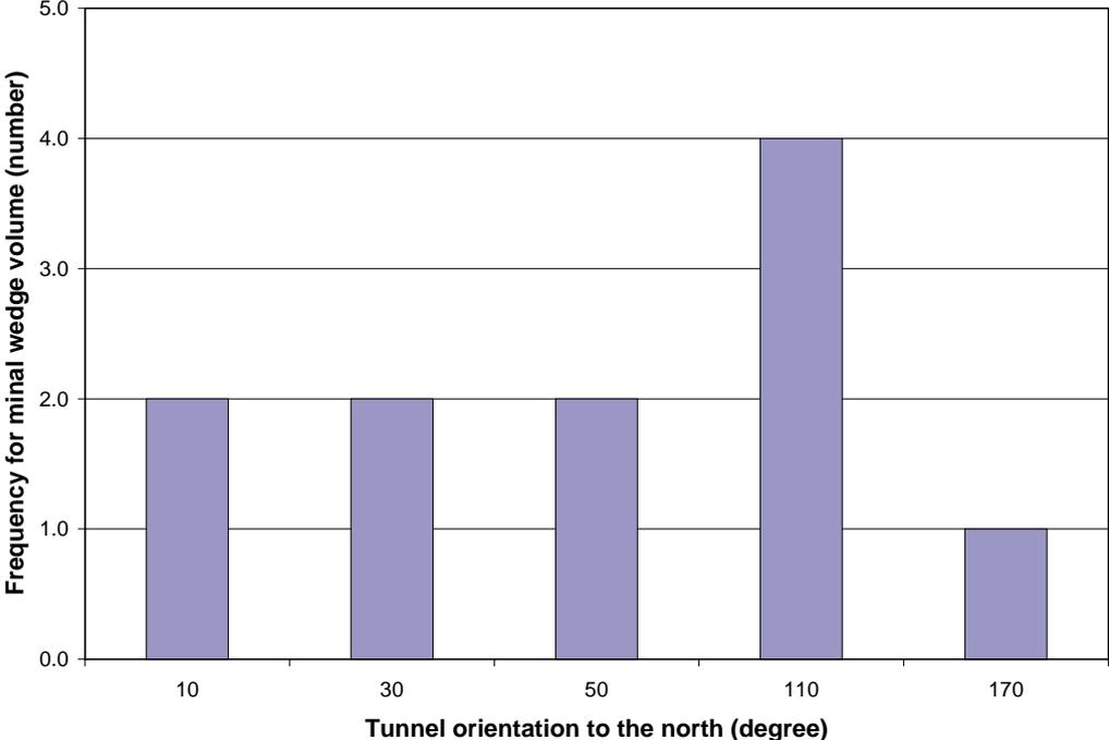
*Figure 4-14. Frequency chart for minimum wedge volume as a function of tunnel orientation, for those fracture combinations that require a support pressure to achieve a factor of safety FOS > 1.5.*
