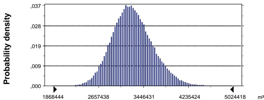
Figure 10-7. Forecast: Volume of rock spoil from blasting, Unit:  $m^3$ . Frequency Chart, 100,000 trials.
