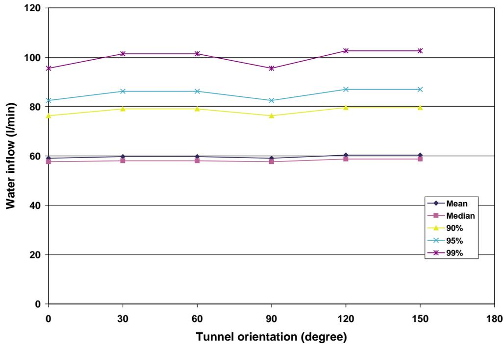
Figure 4-9. Analytically calculated water inflow to the deposition tunnel for storage depth -500 m for six different tunnel orientations related to the major principal stress.
