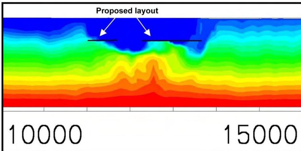
**Figure 7-13.** Salinity distribution in the groundwater- grouting factor 0.01. Vertical profile W-E. Salinity, % Total Dissolved Solids (TDS).
