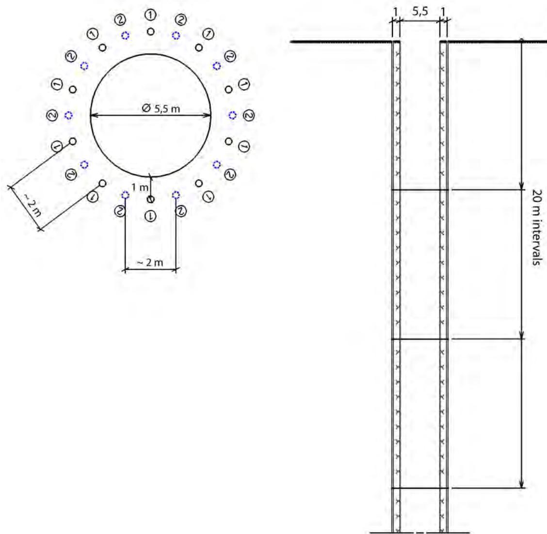
**Figure A-2.** Proposed grouting scheme drill hole layout for shafts in rock blocks, grouting level 1.
