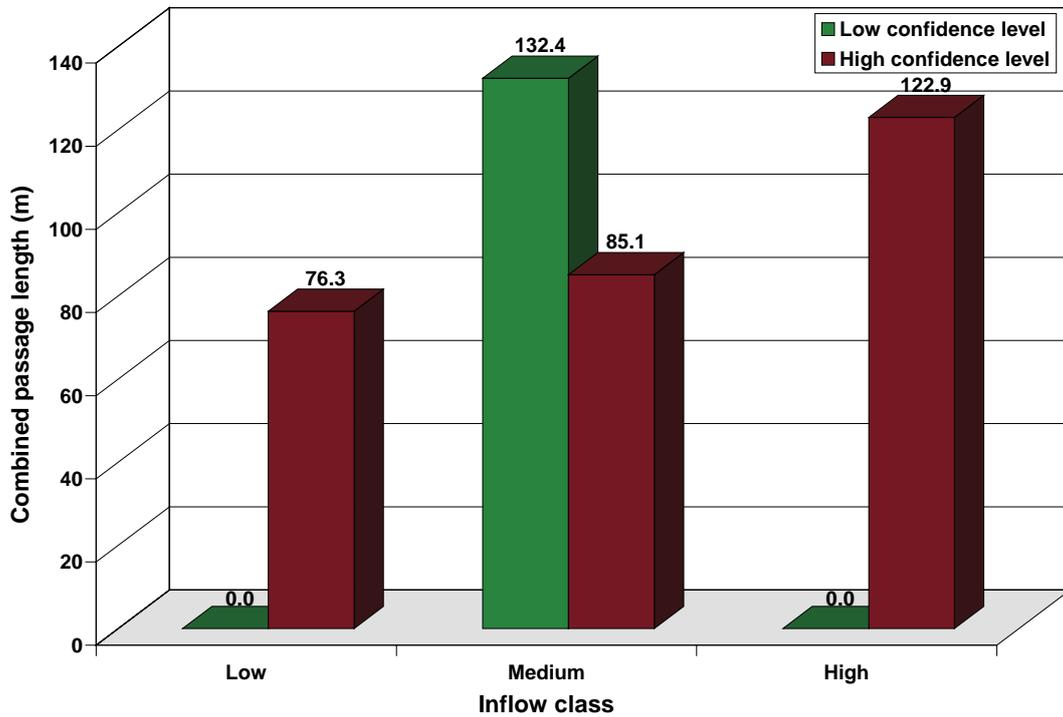
*Figure 6-10. Combined passage length as a function of potential water inflow class and zone confidence assuming no grouting.*
