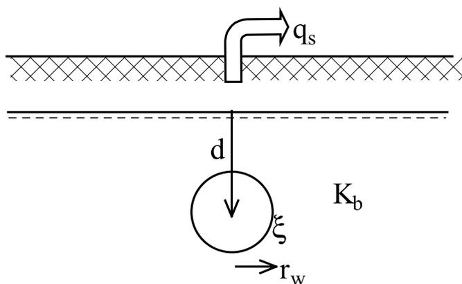
**Figure 4-7.** Analytical model for the deposition tunnels UDP, /SKB 2004a/. See explanation of symbols below Equation 4-1.
