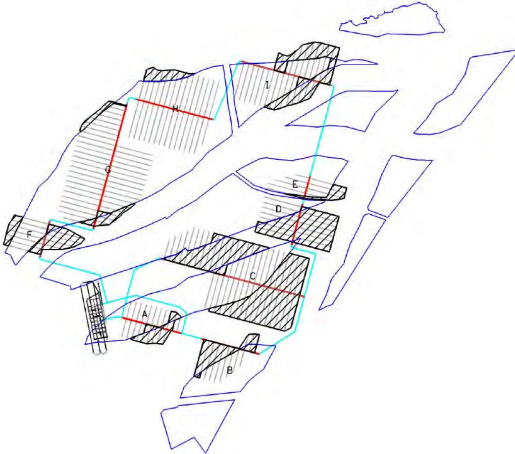
**Figure D4-2.** Proposed layout where areas that are eliminated due to changed interpretation of deformation zones according to SDM Laxemar 1.2 have been highlighted.
