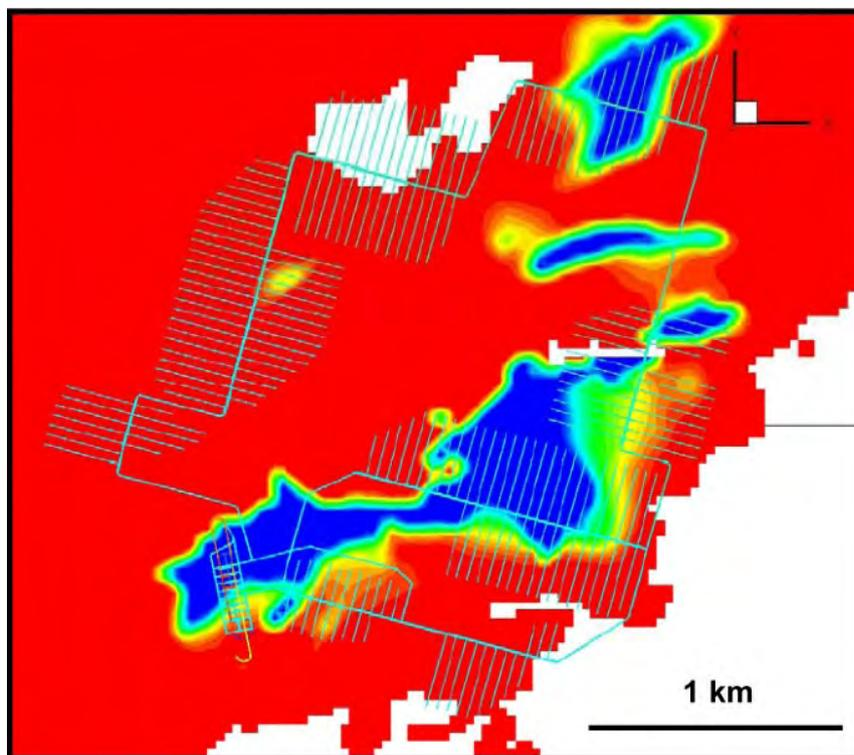
*Figure 7-4. Groundwater table at a grouting factor of 0.1. Horizontal section at level -1 m. Red represents where the groundwater table is at or above level -1 m. Blue represents the drawdown.*
