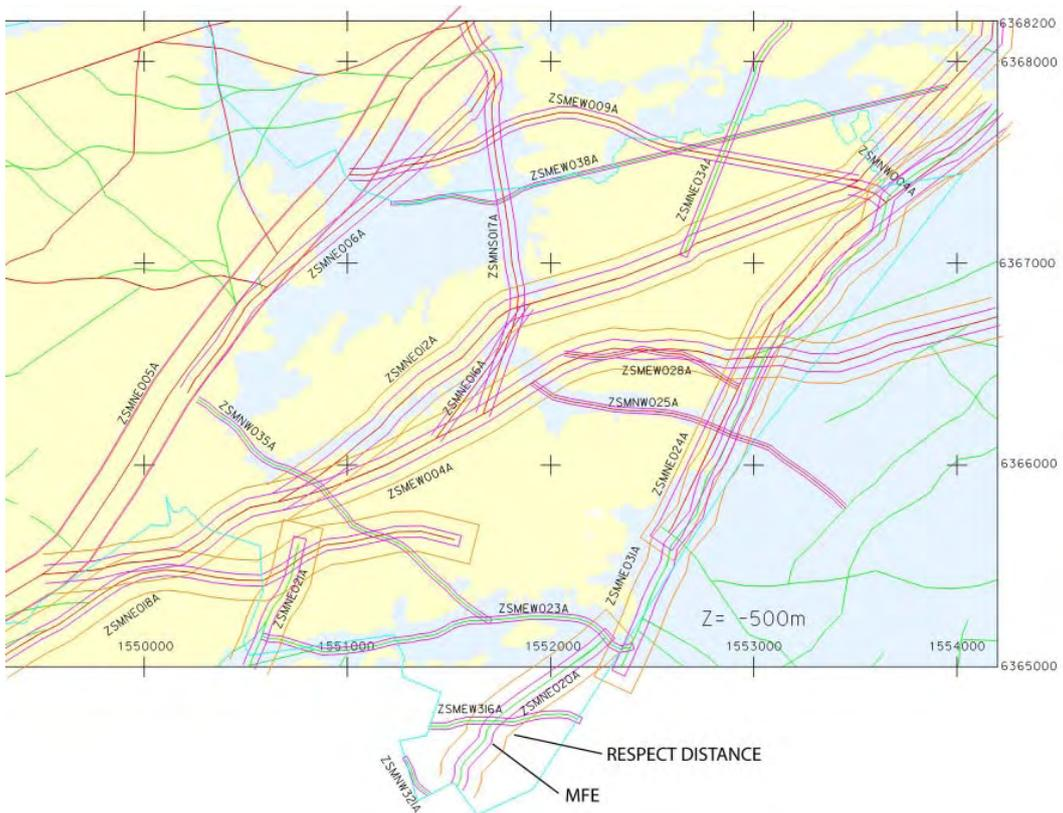
**Figure 3-6.** RD and MFE for deterministic deformation zones lying within the study area. Level -500 m.
