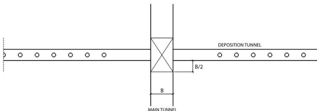
**Figure 9-1.** Area for higher level of rock support at tunnel intersections.
