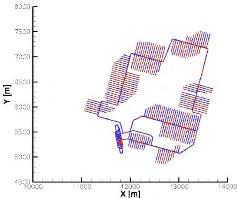
**Figure 7-15.** Contact points (blue) between the tunnel geometry and fractures,  $L > 10$  m.
