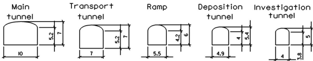
**Figure 4-3.** Tunnel sections. Unit in meters. Revised after /SKB 2002a/.
