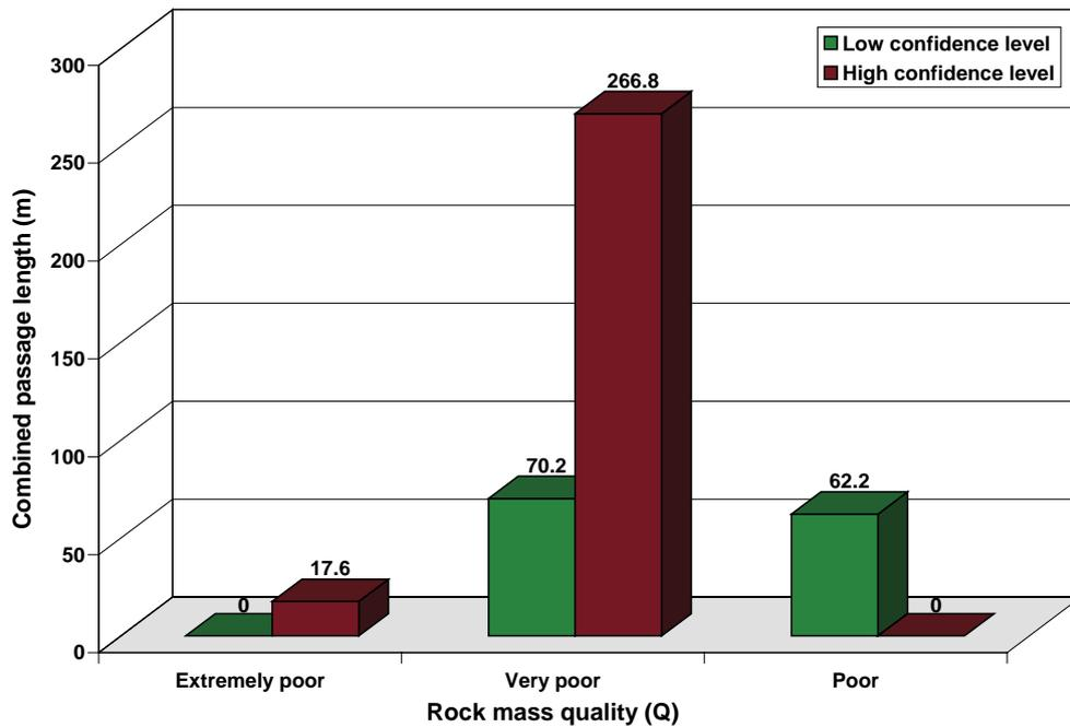
**Figure 6-7.** Combined passage tunnel lengths as a function of rock mass quality and deformation zone confidence level.
