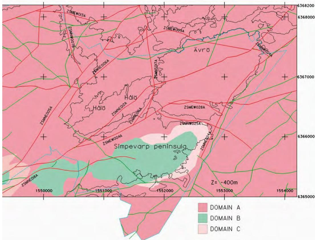
**Figure 3-2.** Map of the bedrock division into rock domains in the Simpevarp subarea on level –400 m. Domain A – Ävrö granite, Domain B – Fine grain dioritoid, Domain C – Mixture of Ävrö granite and quartz monzodiorit. (Modified after SKB, 2005a).
