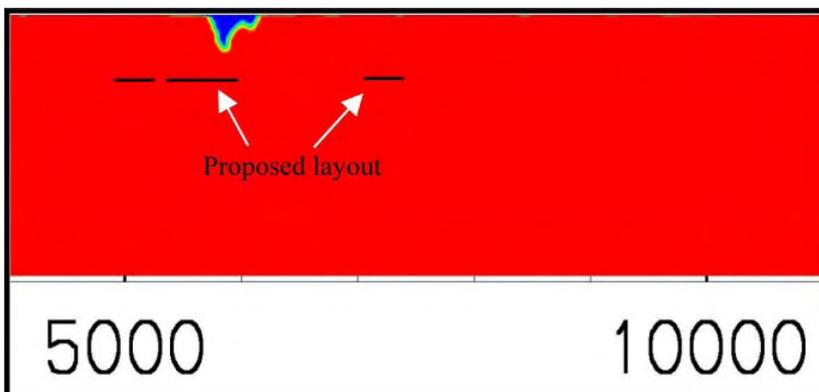
**Figure 7-7.** Vertical section S-N showing the groundwater table drawdown for a grouting factor of 0.1. Maximum drawdown approximately level  $-250$  m.
