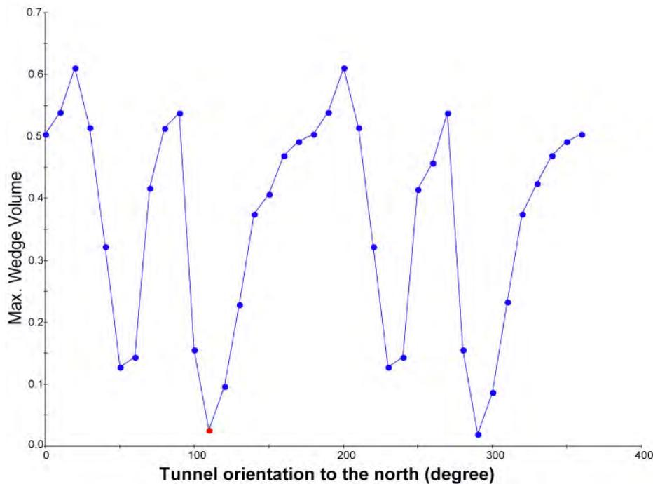
**Figure 4-13.** Maximum wedge volume versus tunnel orientation for fracture combination 4, 5, 6. The wedge volume is minimized with a tunnel orientation of N110.
