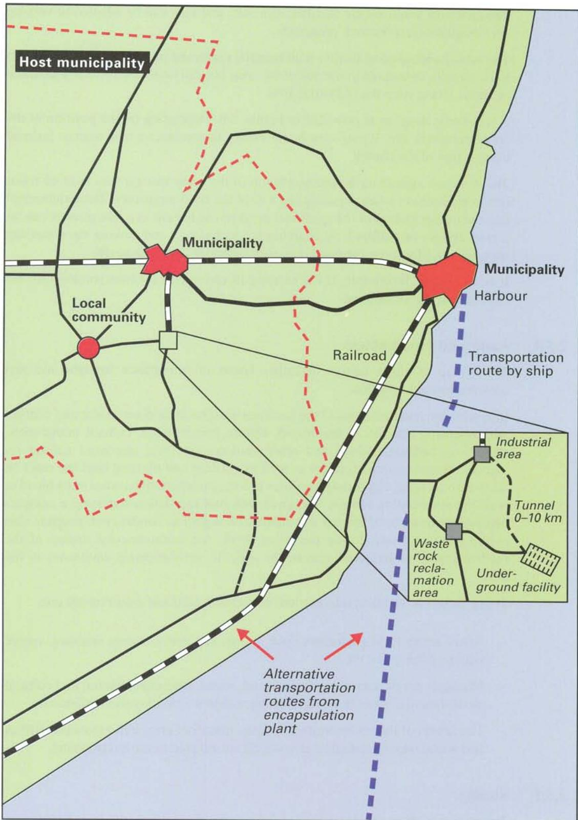
**Figure 2-6.** Schematic diagram of the siting of the industrial area, underground facility and waste rock reclamation area. Not according to scale.
