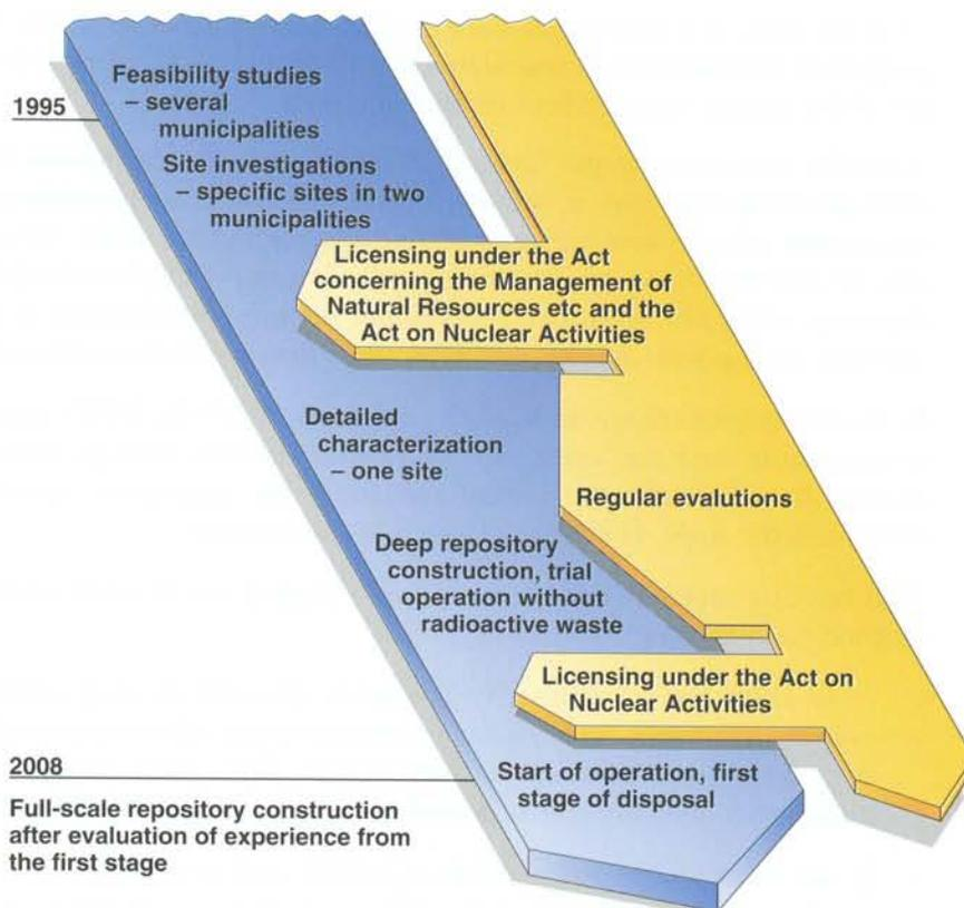
*Figure 2-4. Stages in the work on the siting, construction and commissioning of the deep repository.*
