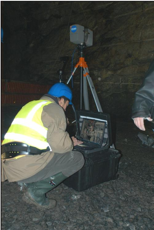
*Figure 13. Laser scanning. The laser scanner is mounted on the tripod and the computer collecting scanning data is placed on the box on the floor.*
