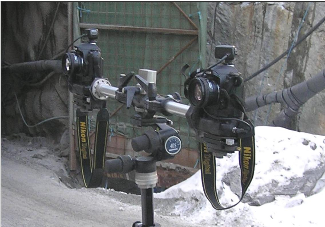
*Figure 11. The use of digital photogrammetry in Onkalo, camera set up.*
