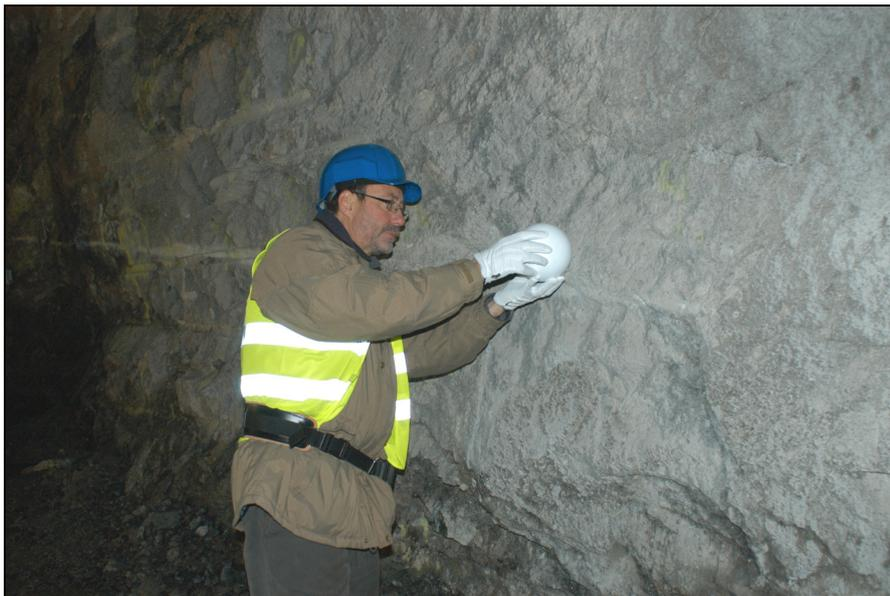
**Figure 18.** A bulb, to be used as one of many reference points during laser scanning, is mounted on the rock wall.
