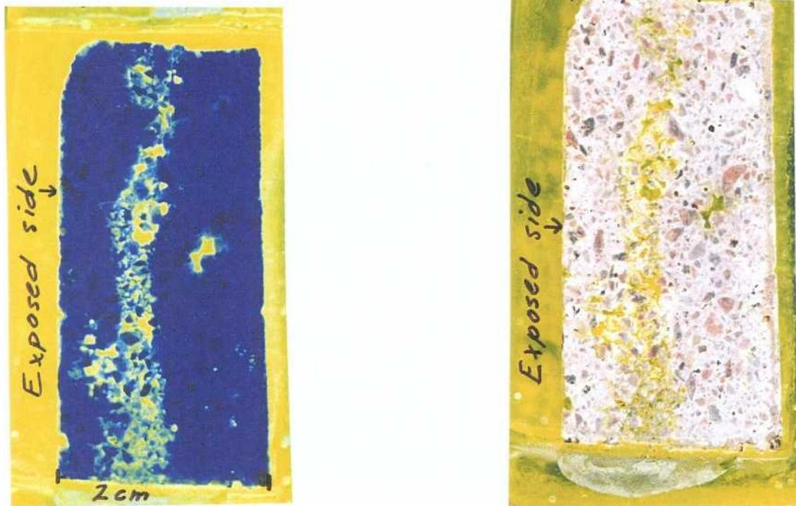
Fig 1. Polished crosssection of the concrete mortar in watertank. The sample is impregnated with epoxy with fluorescent dye which reveals the coarse porosity (yellow patches) under fluorescent light. Thin sections were made from the same piece.
