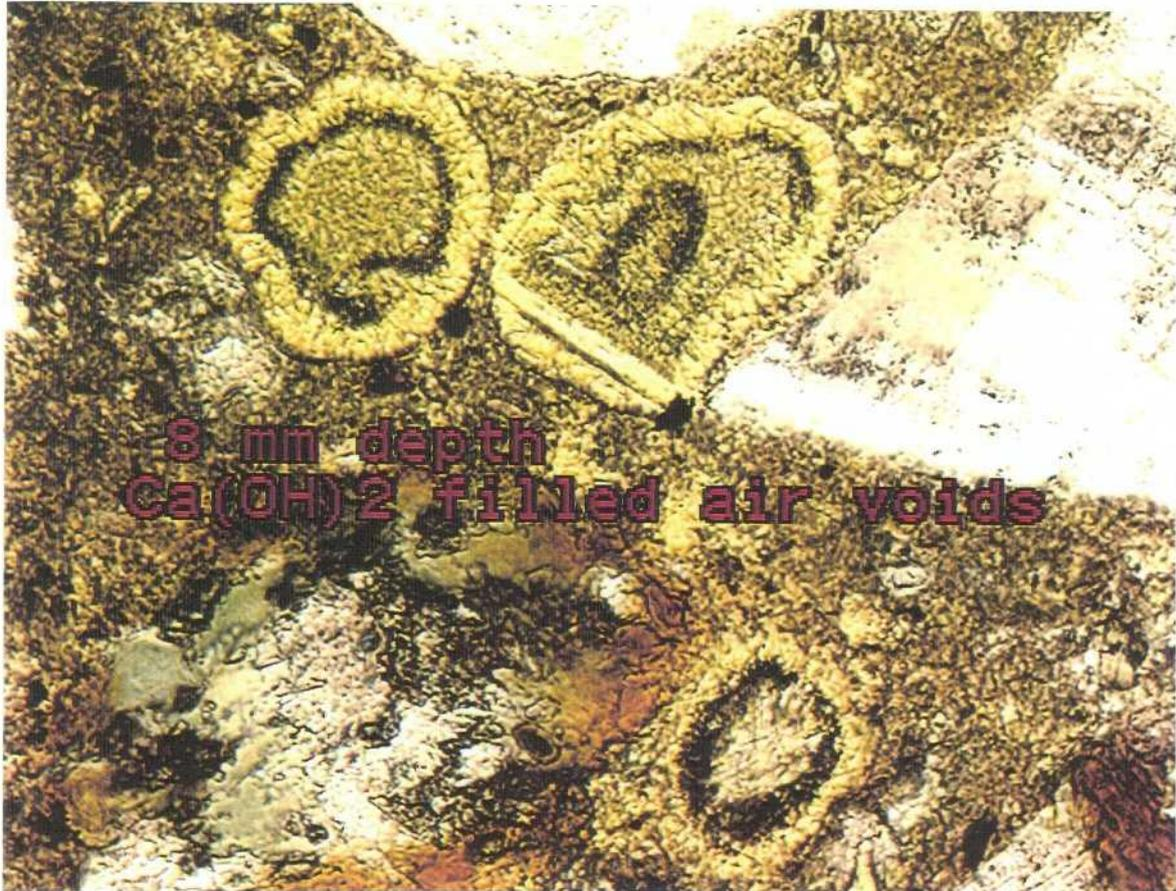
Fig 8. In and just above the zone which is dominated by coarse porosity, numerous portlandite and ettringite-filled air-voids exist. These indicate strong remobilisation of calcium and sulfates. Note the "ring structures" which indicate different episodes of precipitation. Dark rings represent ettringite/monosulfate crystals and light-yellowish rings consist of portlandite.
