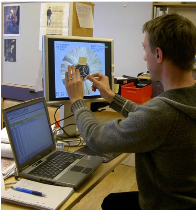
Figure 4-8. The \beta -angle between pointer and bubble is measured on the right screen. The angle, together with an uncertainty value, is documented in an Excel worksheet on the left screen.
