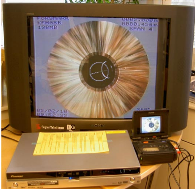
Figure 4-4. BIPS raw data tapes are copied from the Video8-tape player (down to the right) to DVD (down to the left).
