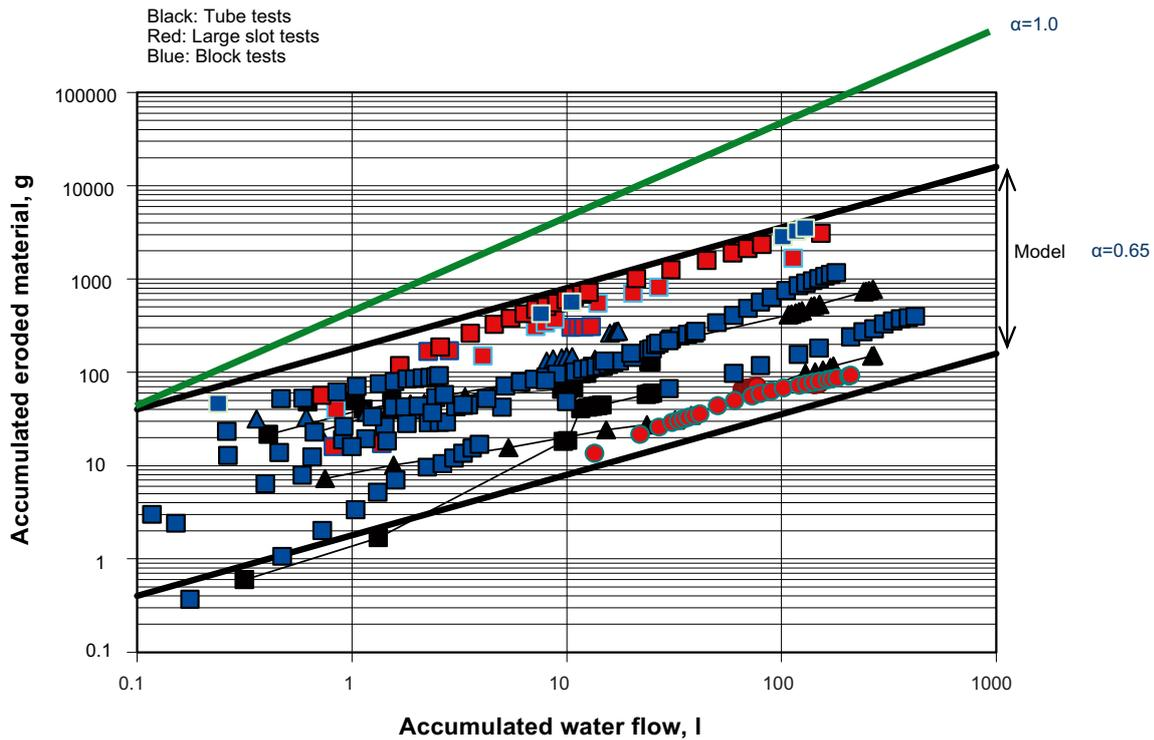
**Figure 7-3.** All erosion results plotted in one diagram. The lower boundary line corresponds to  $\beta = 0.02$  and the upper  $\beta = 2.0$ . The inclination of the boundary lines corresponding to  $\alpha = 0.65$  is motivated by the figure.  $\alpha = 1.0$  (corresponding to constant erosion rate) is also illustrated.
