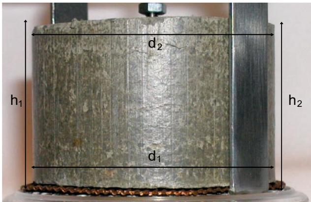
Figure 11-3. Schematic view of specimen height and diameter measurement locations.
