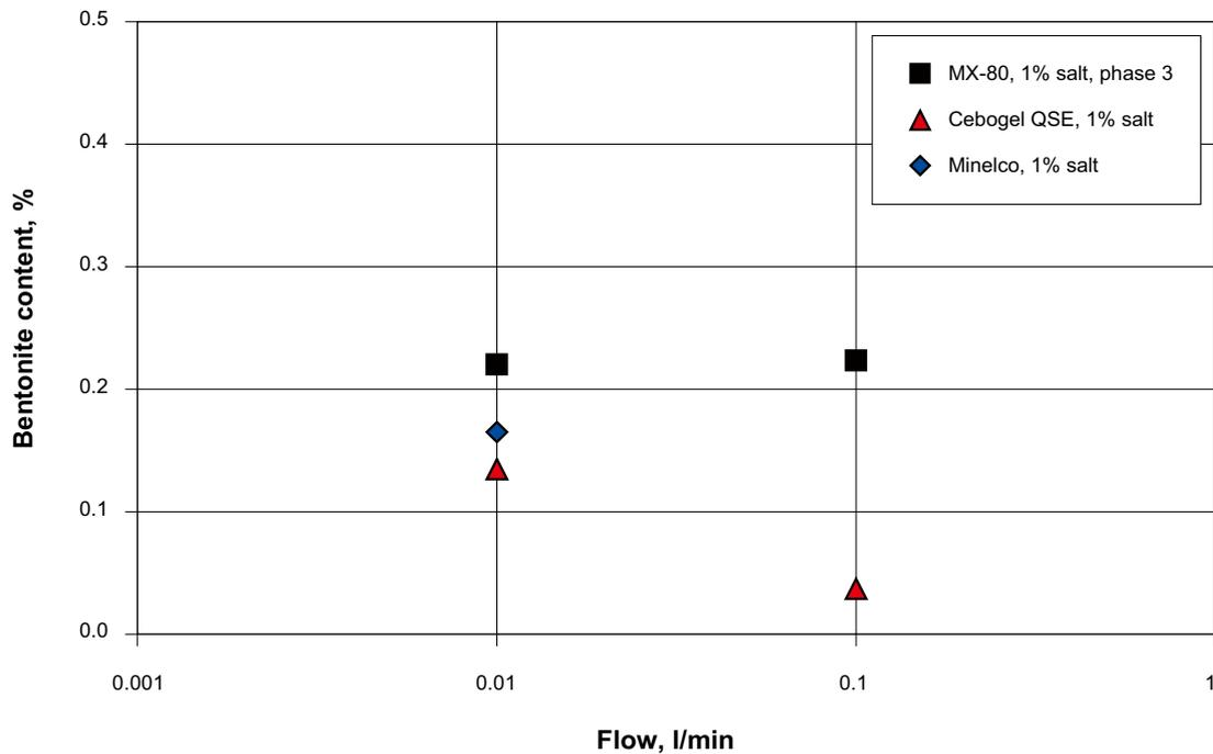
Figure 5-3. The bentonite content in the discharged water in percentage plotted vs. the different water flow rates.
