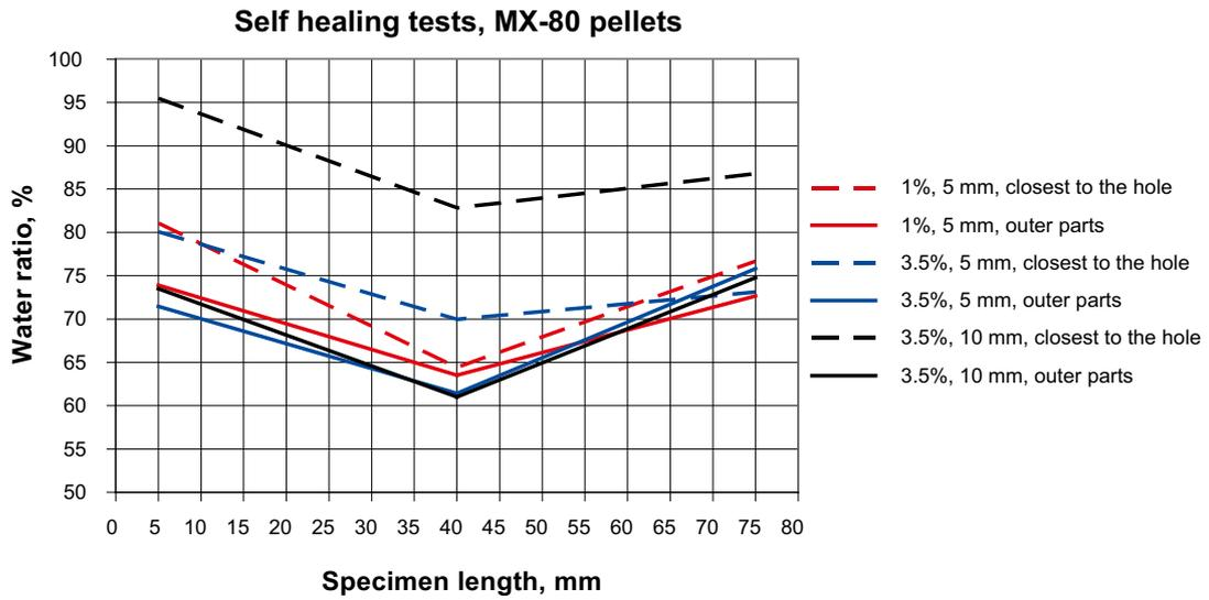
**Figure 10-3.** Water content distribution measured in the three tests performed with MX-80 pellets. (Note the difference in water content between the outer parts and the parts around the pre-drilled hole for the specimens saturated with the higher salt content water (3.5%).)
