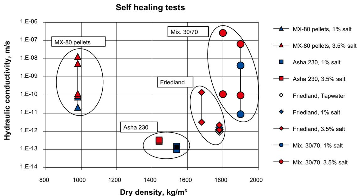
Figure 10-11. Compilation of self healing test results.
