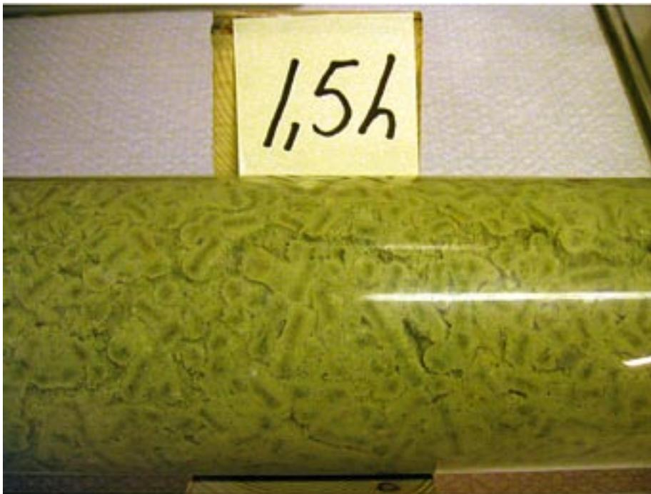
*Figure 5-5. Picture from the test performed with Cebogel pellets, 0.1 l/min and 1% salt in the water. There is no main channel where all water is flowing, like in the tests with MX-80 pellets. The water seems to flow in the voids between the pellets, which can be one reason for the water pressure that was built up during the test.*
