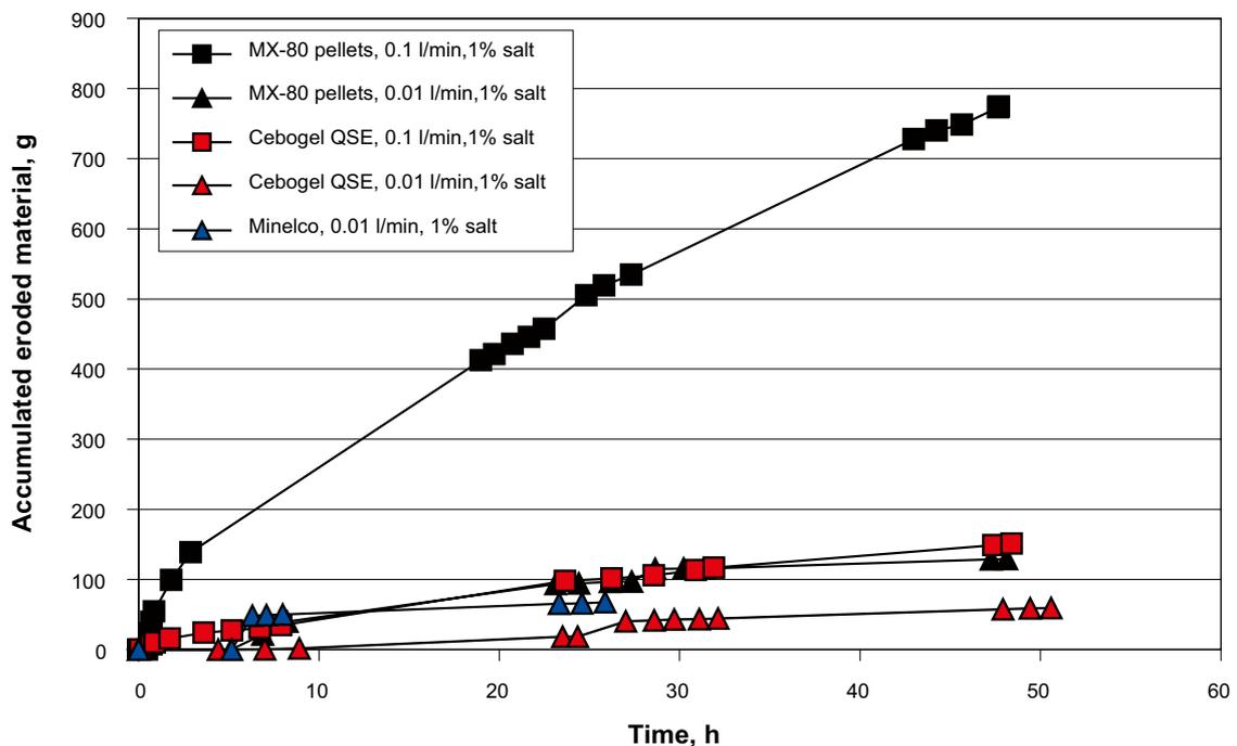
Figure 5-1. The accumulated amount of eroded material plotted vs. time.
