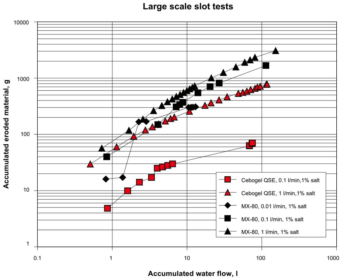
**Figure 6-6.** The accumulated dry weight of eroded material plotted vs. the accumulated water flow. Both the new test results (Cebogel QSE) and the old test results (MX-80) are shown.
