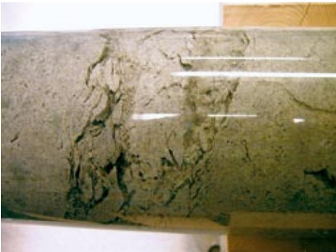
*Figure 4-3.* Picture from the test A:312 (0.01 l/min and 3.5% salt in the water). The material seemed to separate and the water pressure was acting on a surface pushing the bentonite specimen forward.
