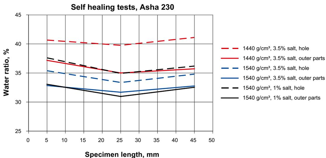
*Figure 10-6. Water content distribution in the three tests performed with Asha 230. There is still a small difference in water content between the central parts and the outer parts. This difference is however too small to influence the hydraulic conductivity more than marginally.*
