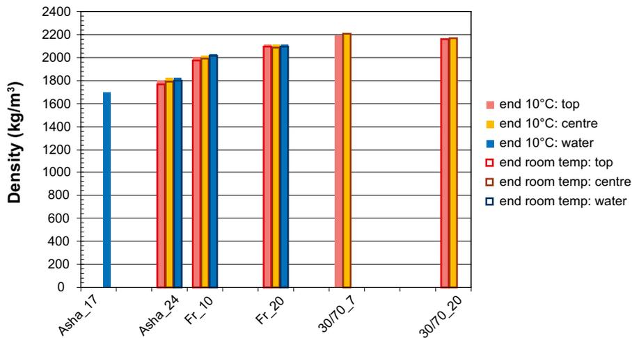
Figure 11-11. Final densities from test series with specimens at 10°C and at room temperature.
