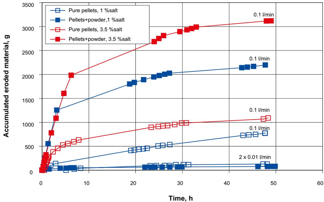
**Figure 4-4.** The accumulated amount of eroded material plotted vs. time for the six tests. In the beginning of the tests the influence of fine material and salt content in the water was strong but after about 24 hours the erosion rate almost was the same in all tests.
