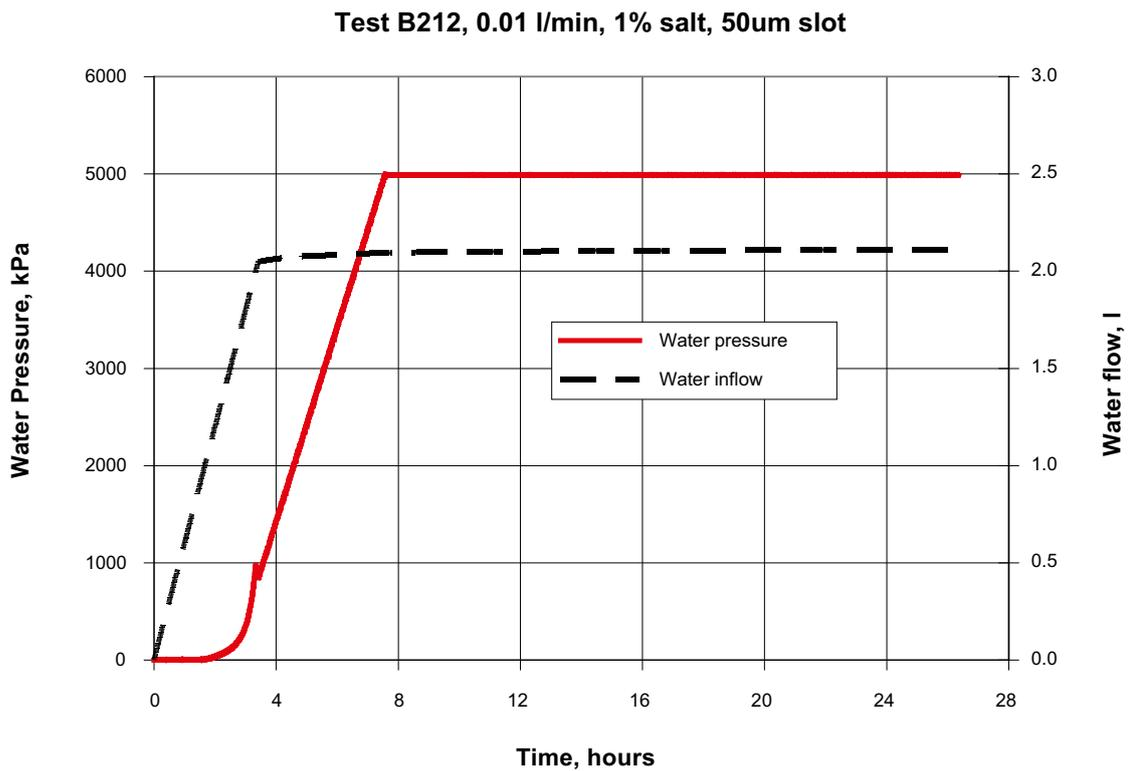
**Figure 9-2.** Results from the test performed with a water flow rate of 0.01 l/min and an aperture of the fracture of 50  $\mu\text{m}$ . The water pressure and the accumulated water flow is plotted vs. time.
