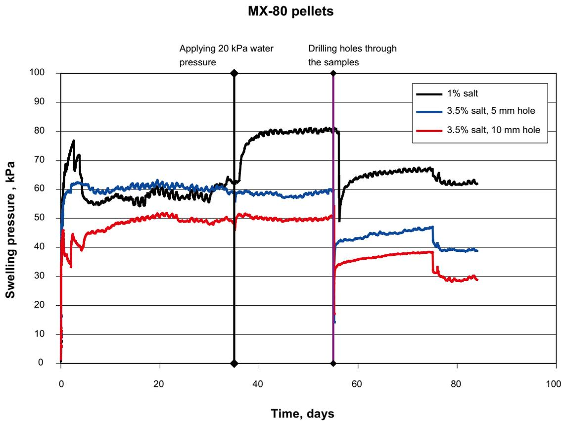
**Figure 10-4.** Development of swelling pressure of MX-80 pellets with time.
