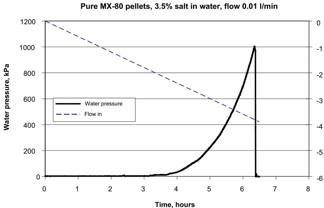
*Figure 4-2.* The water inflow rate and the measured water pressure built up in test A:312. When the pressure reached 1 MPa the test was terminated.
