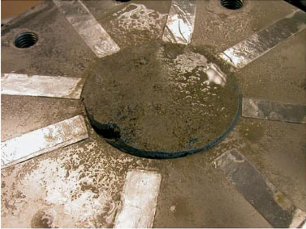
*Figure 9-3. Test performed with 0.01 l/min, 50 um aperture and 1% salt in the water.*
