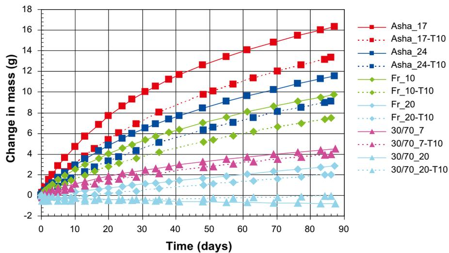
Figure 11-7. Water absorption for test series at 10°C and at room temperature.
