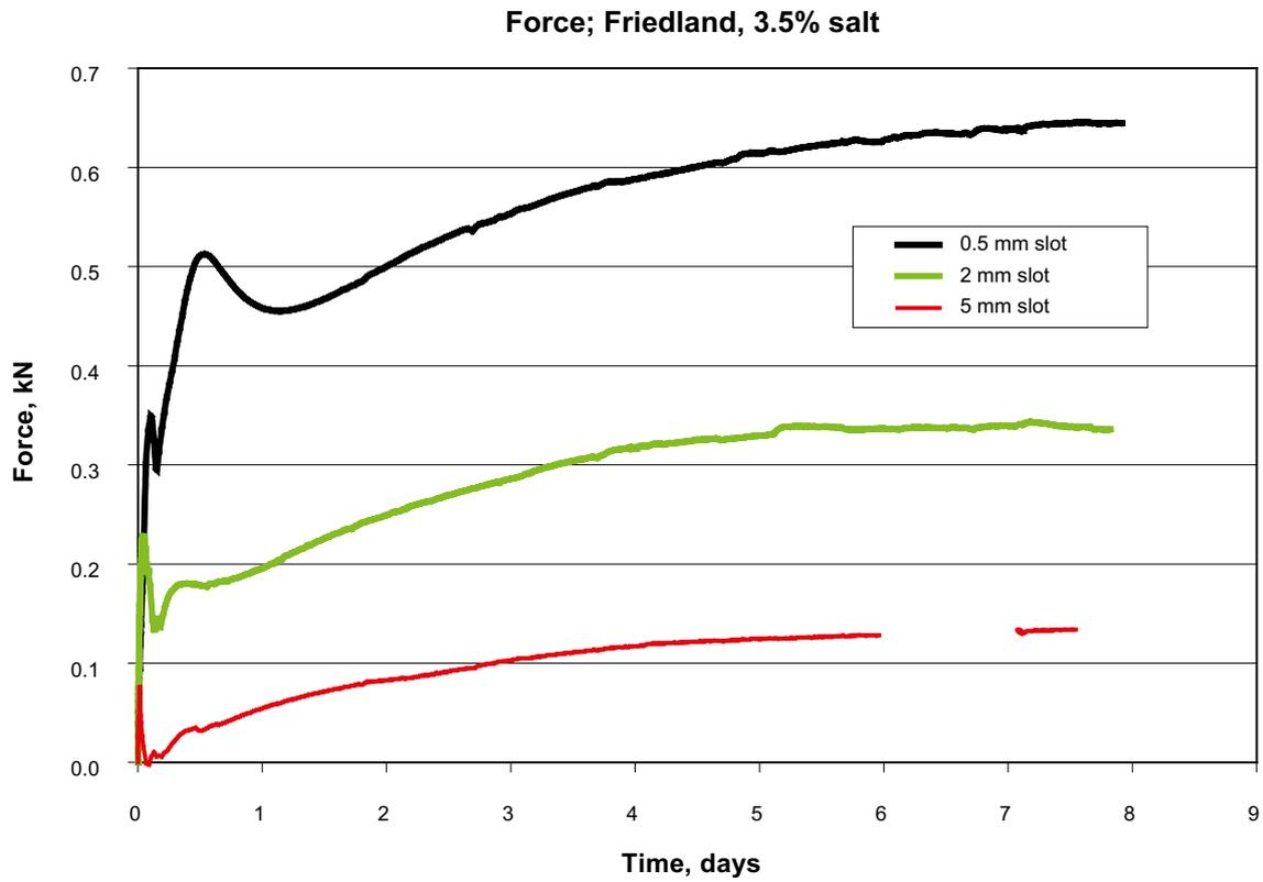
Figure 8-6. The results from the confined tests where force was measured (3.5% salt solution) plotted vs. time.
