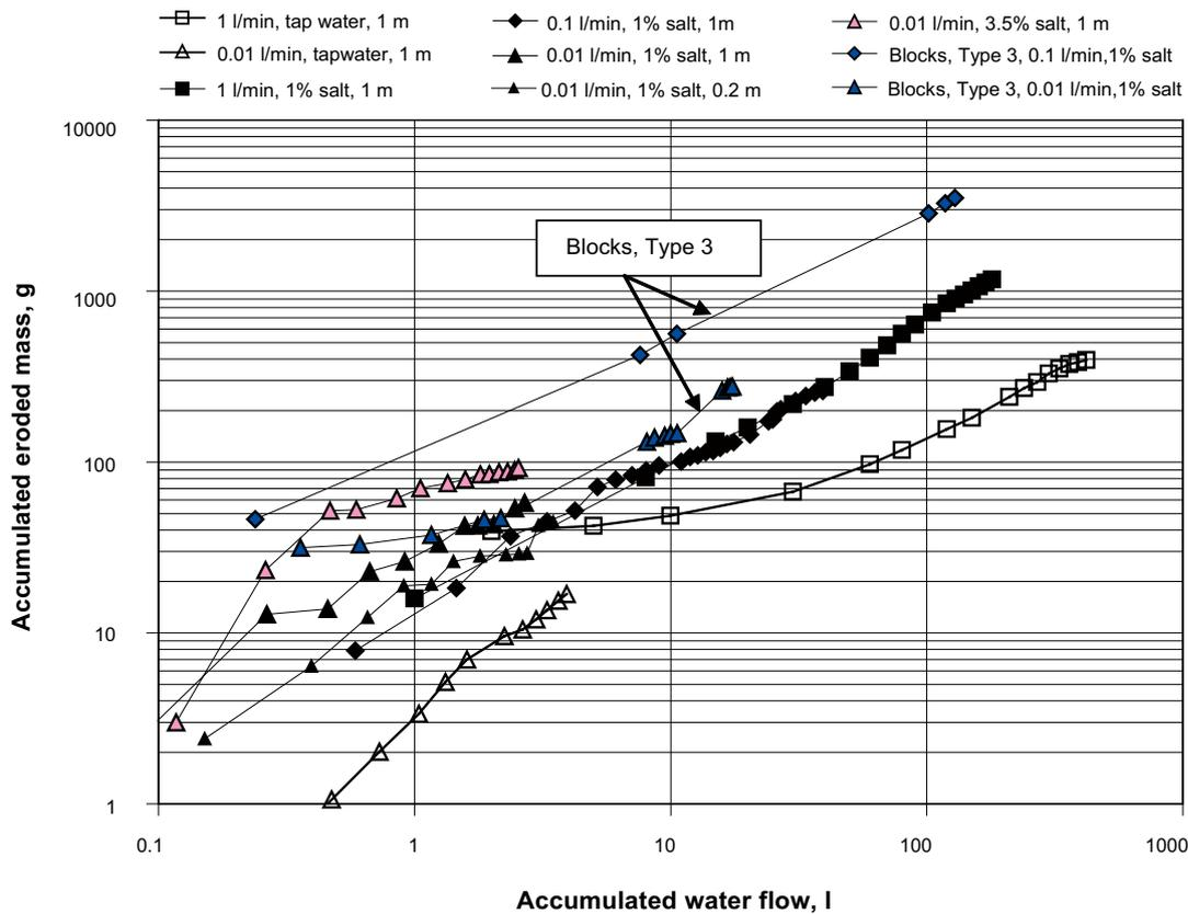
Figure 3-3. Accumulated dry weight of eroded material plotted vs. the accumulated water flow in logarithmic scales.
