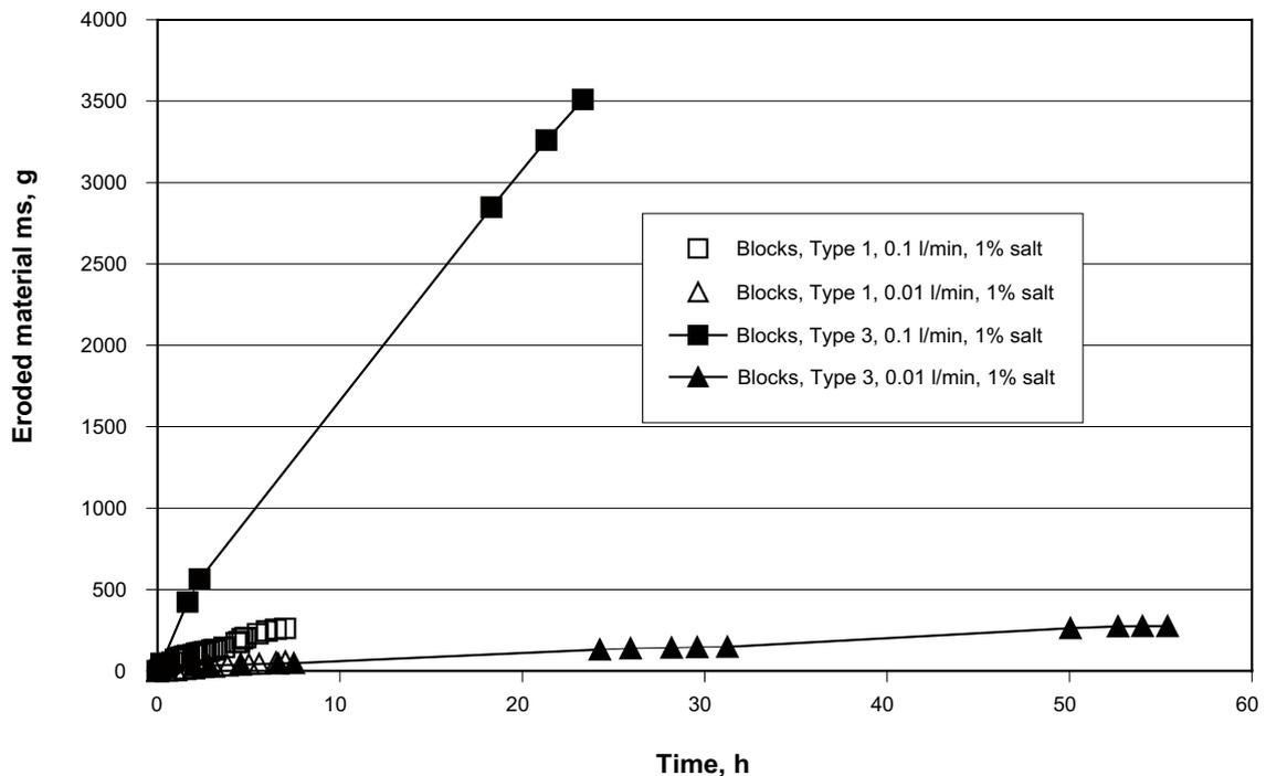
**Figure 3-2.** The accumulated amount of eroded material plotted vs. time. The two test marked with black dots are from the latest tests using Friedland block Type 3, while the two tests with transparent dots are from the tests in Phase 2 using Friedland blocks of Type 1.
