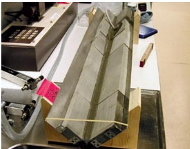
*Figure 3-1. Picture from one of the earlier performed tests. The picture shows a 1m long steel profile filled with blocks of compacted bentonite. A constant water flow was applied in one end and the amount of eroded material in the other end was measured.*
