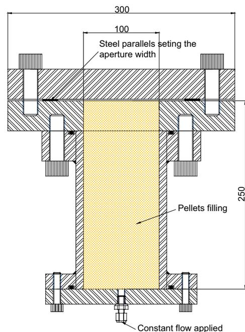
**Figure 9-1.** *Left:* Picture from the laboratory showing the assembled equipment just before test start. *Right:* Schematic drawing of the test equipment.
