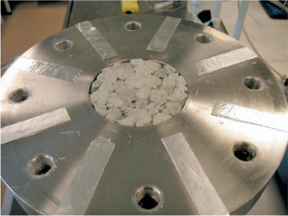
*Figure 9-4. Test performed with 0.01 l/min, 100 um aperture and 1% salt in the water.*
