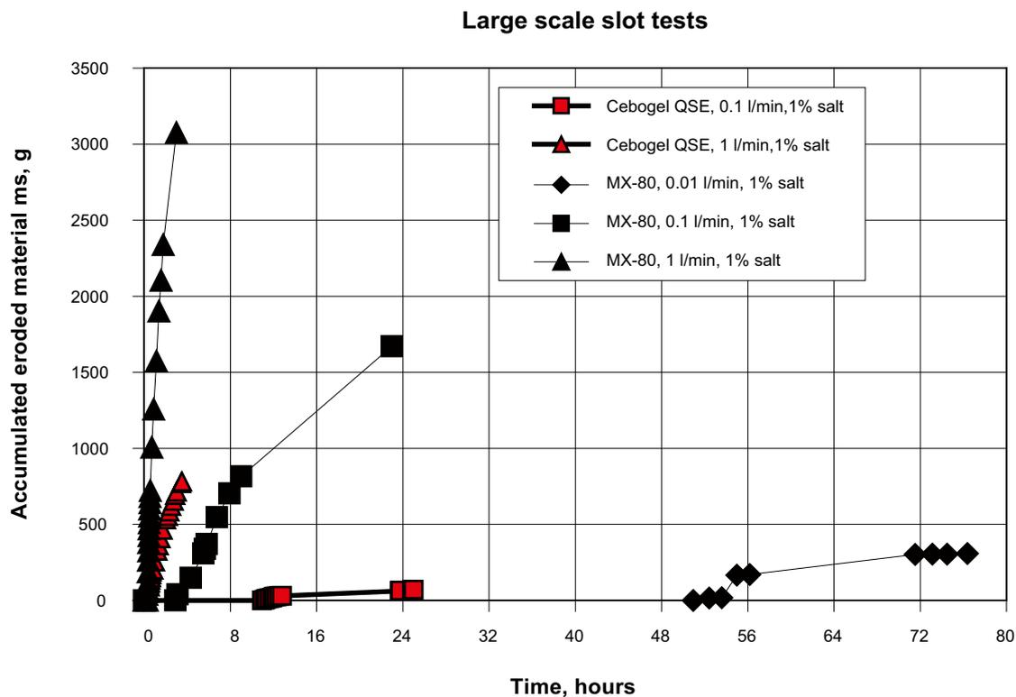
*Figure 6-5. The accumulated dry weight of eroded material plotted vs. time. Both the new test results (Cebogel QSE) and the old test results (MX-80) are shown.*
