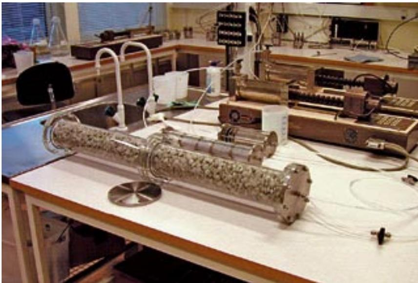
*Figure 4-1. Picture showing the test equipment. The picture shows a Plexiglas tube filled with Mx-80 pellets. A constant water flow was applied in one end and the discharging water was collected in the other end.*
