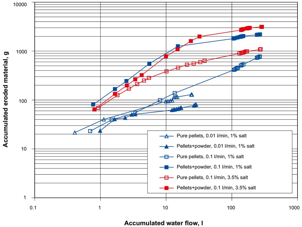
Figure 4-5. The accumulated amount of eroded material plotted vs. the accumulated water flow in logarithmic scales.
