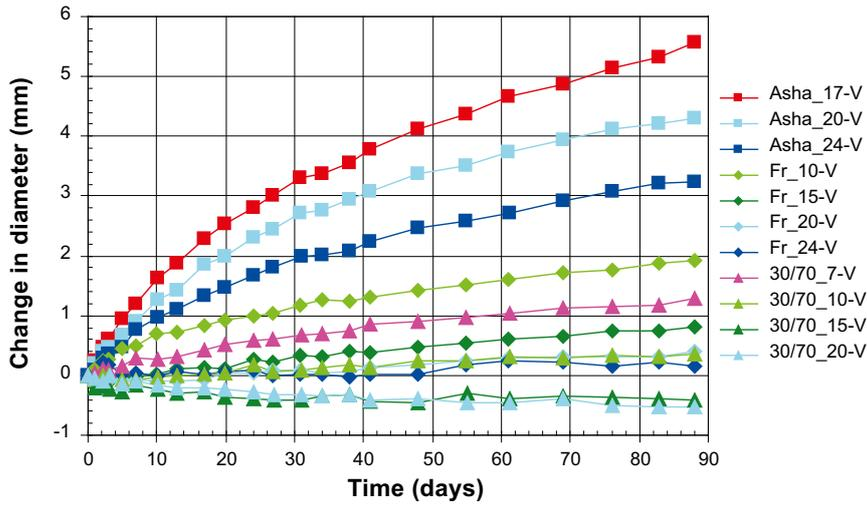
Figure 11-9. Change in specimen diameter as result of water uptake. (The diagram shows the average of the measurements taken at each time.)
