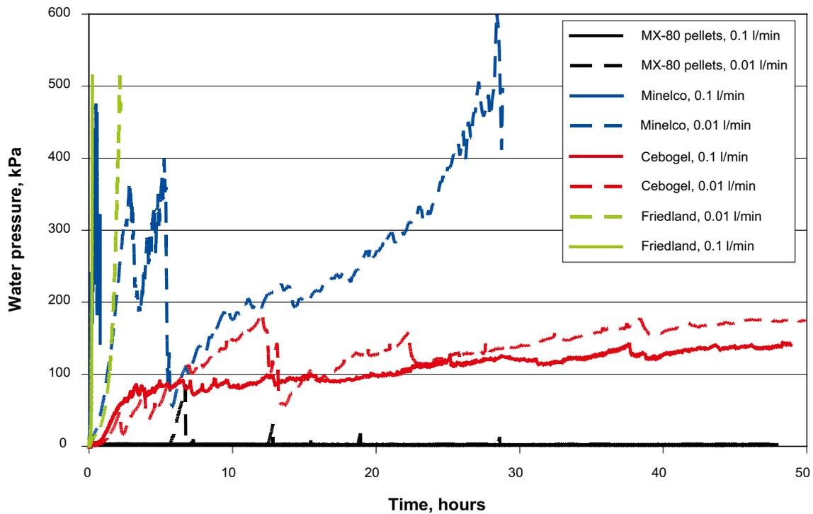
*Figure 5-4. Diagram showing the resistance to water inflow built up during the test time for the different materials and applied water flows plotted vs. time. The behavior seems to be very different for the different materials.*
