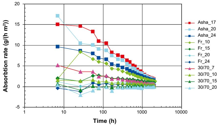
Figure 11-5. Water absorption rate for the specimens presented in Figure 11-4.
