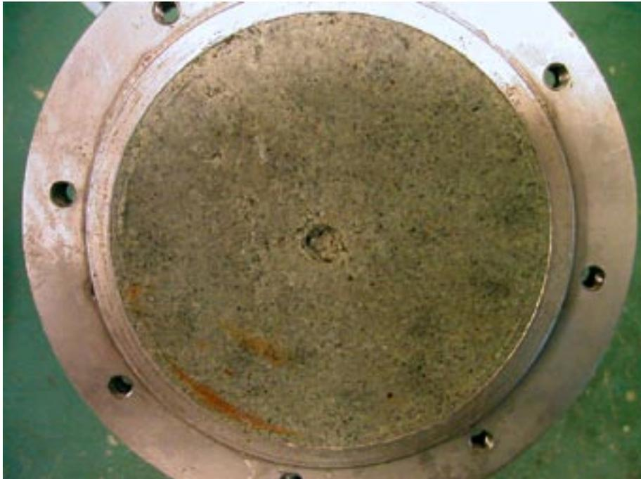
*Figure 10-2. Picture from specimen SH103 (10 mm hole in MX-80 pellets) at the termination of the test. The drilled hole can still be seen very clearly. The hole is filled with gel with a higher water content than the surroundings.*
