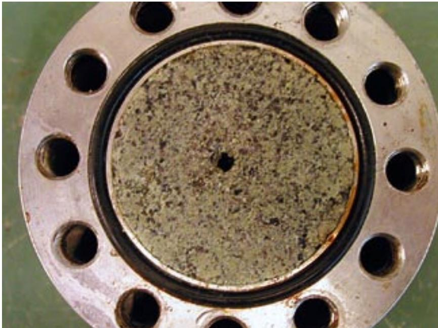
**Figure 10-9.** Picture from specimen SH603 (30/70 mixture) at termination of the test. The drilled hole is still open. No healing had occurred in any of the 30/70 samples.
