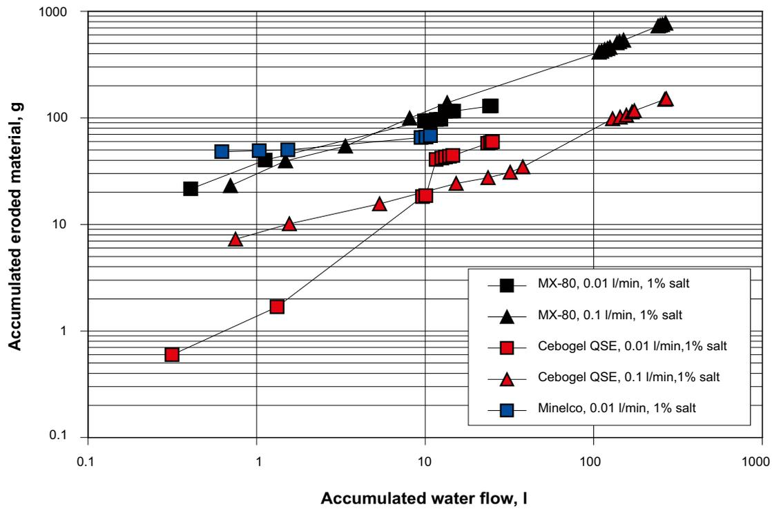
Figure 5-2. The accumulated amount of eroded material plotted vs. the accumulated water flow in log scales.
