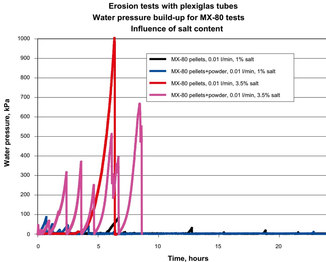
*Figure 4-7. The water pressure built up during tests plotted vs. time. The results are from tests performed with a constant water flow of 0.01 l/min and with different salt content in the water.*
