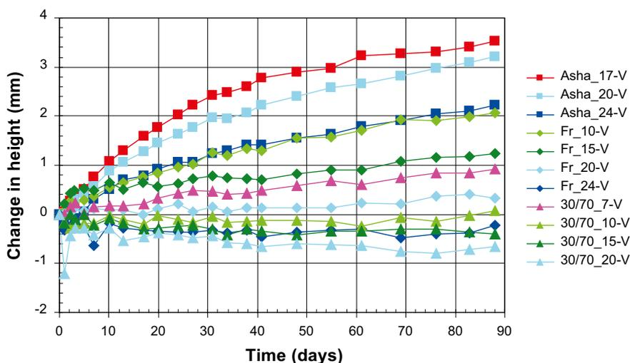
*Figure 11-8. Change in specimen height as result of water adsorption. (The diagram shows the average of the measurements taken at each time.)*
