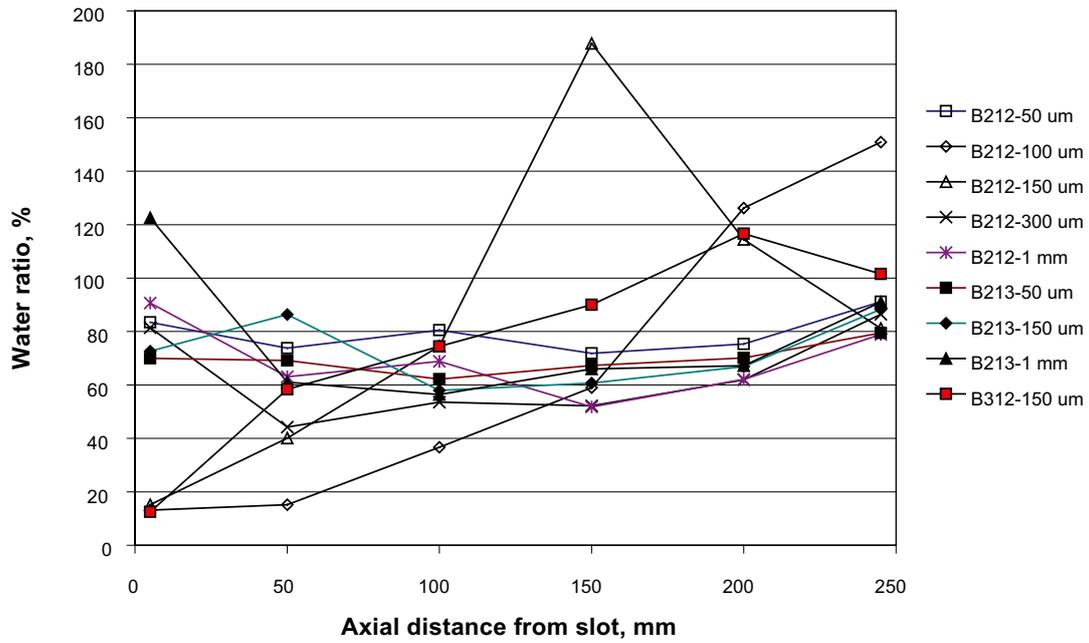
Figure 9-5. Water content distribution in the pellets filling after termination. The water content is plotted vs. the axial distance from the slot.
