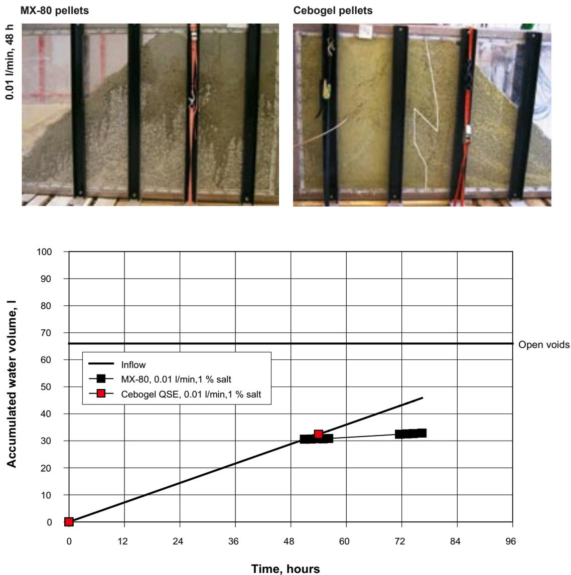
Figure 6-2. Upper: Pictures from the two tests performed with a water inflow rate of 0.01 l/min taken after 48 hours. Lower: The total inflow and the difference between inflow and outflow plotted vs. time.
