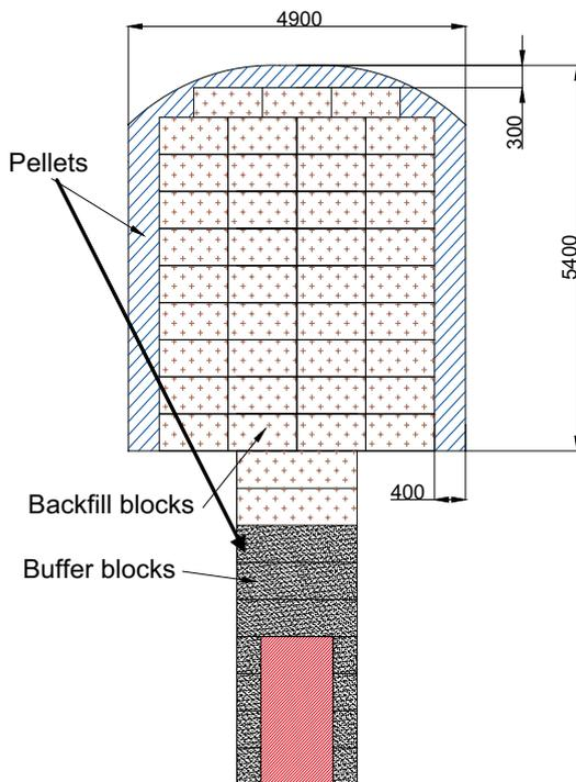
**Figure 7-1.** The rock surface in both the deposition tunnel and the deposition holes is in direct contact with pellets filling.
