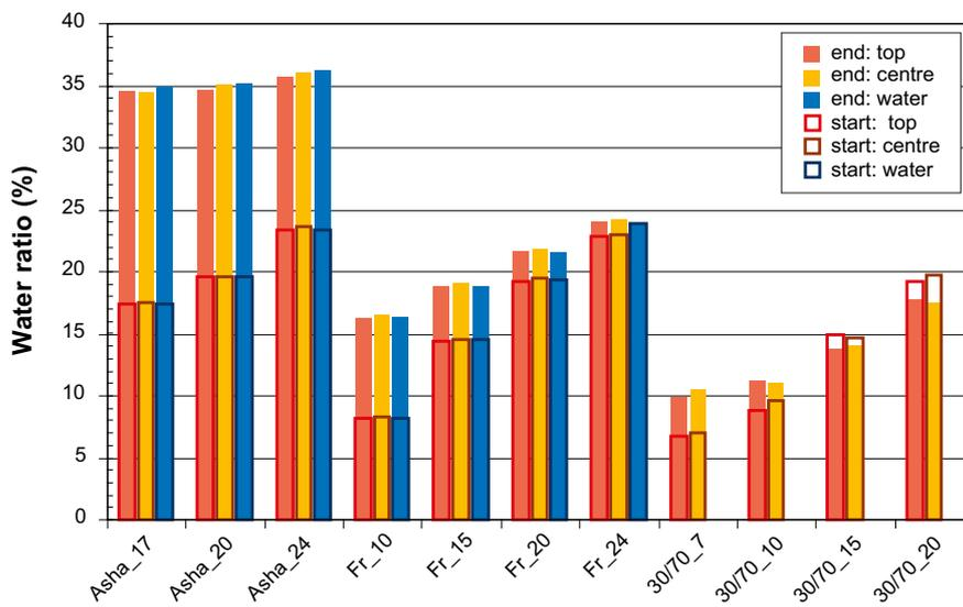
Figure 11-6. Measured water contents at start and at the end of the test for one of the test series.
