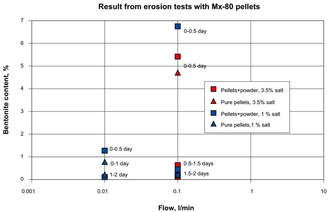
Figure 4-6. The bentonite content in the discharged water (after different times) plotted vs. different water flow rates. The influence of time is very strong. After 1 day the bentonite content in the water is about 0.1–0.3% for all tests.
