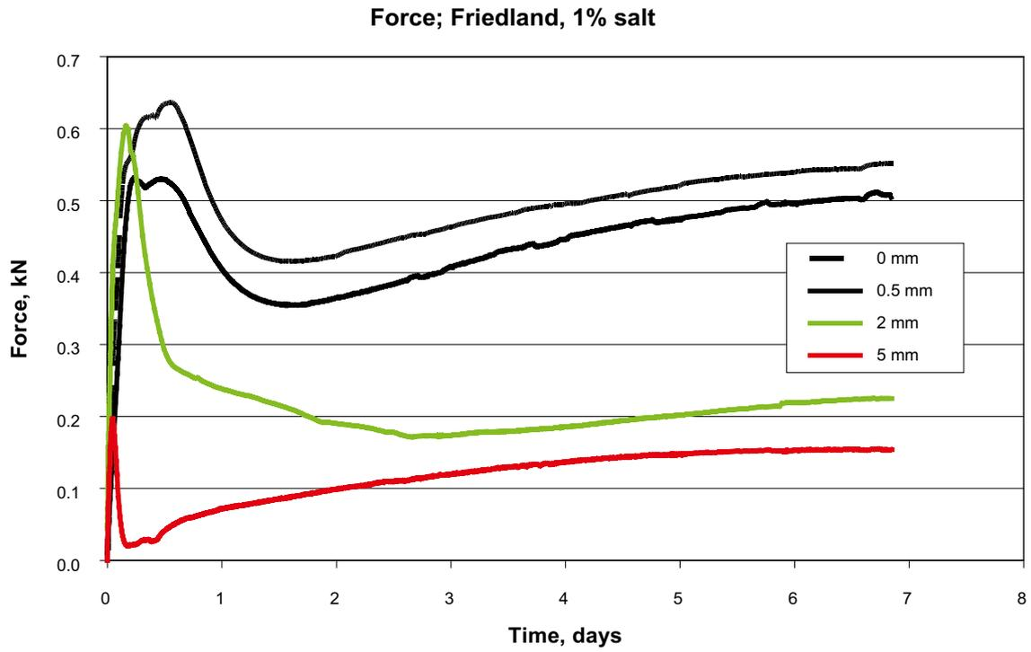
Figure 8-5. The results from the confined tests where force was measured (1% salt solution) plotted vs. time.
