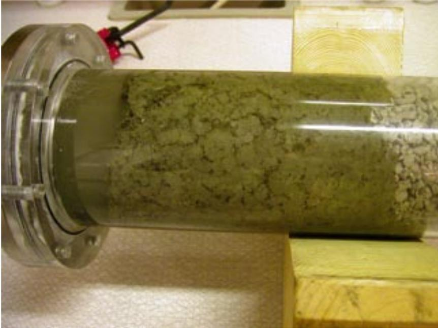
*Figure 5-6. Pictures from the test performed with Friedland granules, 0.1 l/min and 1% salt in the water. The material sealed and the water pressure could act on a surface pushing the material forward.*
