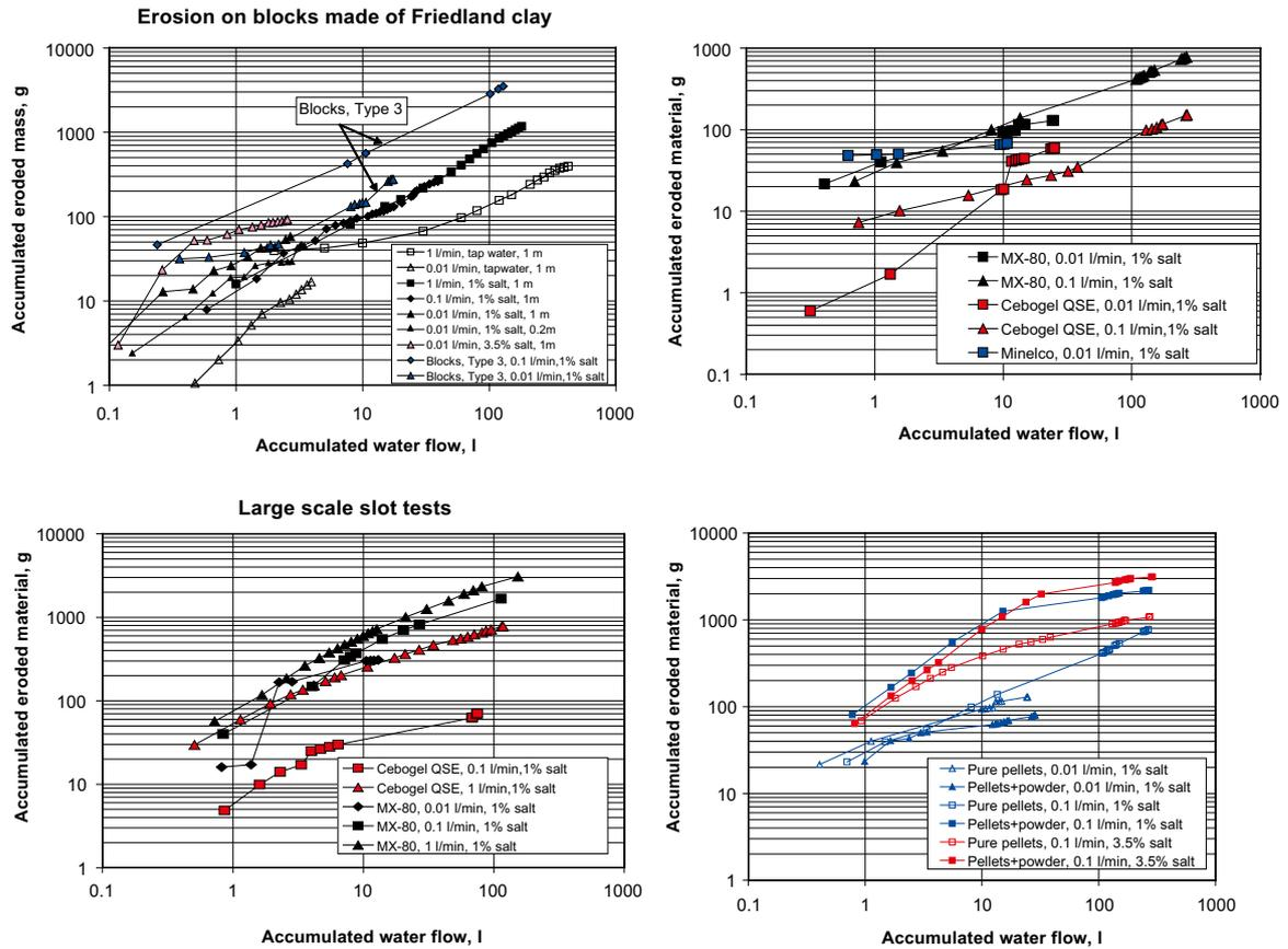
**Figure 7-2.** Results of erosion tests plotted as accumulated dry mass of eroded material as a function of accumulated water flow in double logarithmic diagrams (diagrams of larger size are available, see Figure 3-3, 4-5 and 6-6). **Upper left:** Friedland clay blocks. **Upper right:** Tube tests of different pellet materials. **Lower left:** Slot tests of different pellet materials. **Lower right:** Tube tests of pellets mixed with 50% powder.
