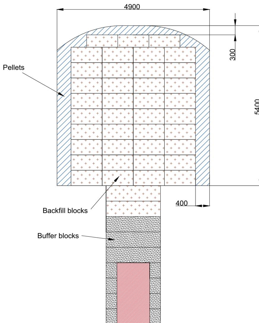
**Figure 2-1.** Schematic drawing showing an example of the geometry of a deposition tunnel backfilled with blocks and pellets.
