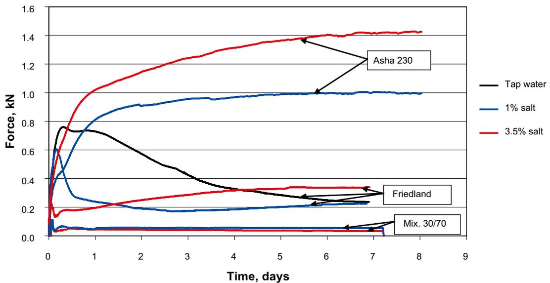
Figure 8-8. The results from the confined tests measuring the force. The tests are performed with different materials, different waters and with an initial slot of 2 mm.
