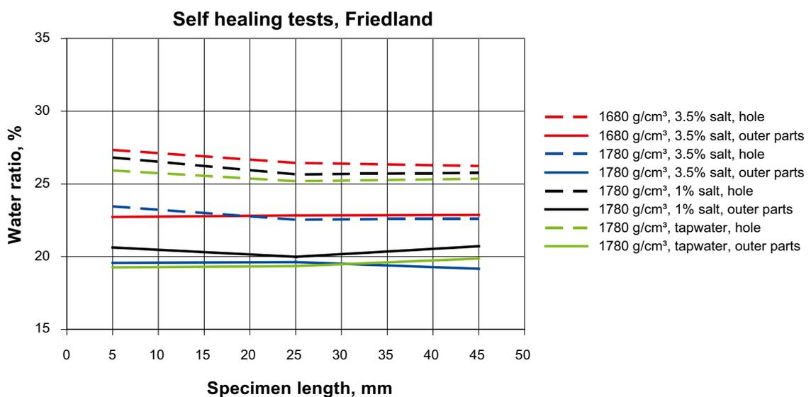
Figure 10-8. Diagram showing the water content determination for the three tests performed with Friedland clay.
