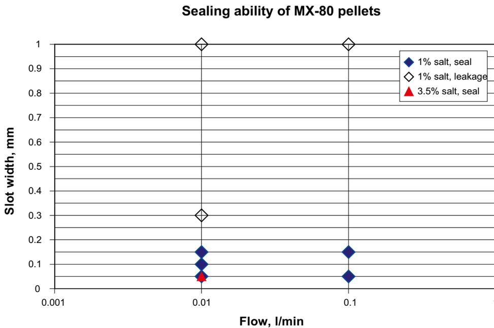
Figure 9-6. Compilation of the test results. The different slot widths are plotted vs. different water flow rates. The tests indicate that the maximum slot width that the MX-80 material could seal was 0.15 mm for the tested flow rates.
