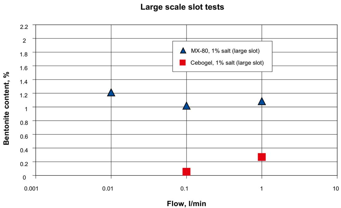
**Figure 6-7.** The dry weight of eroded bentonite in percentage in the discharged water plotted vs. the different water flow rates. In the diagram is both the new test results (Cebogel QSE) and the old test results (MX-80) shown.
