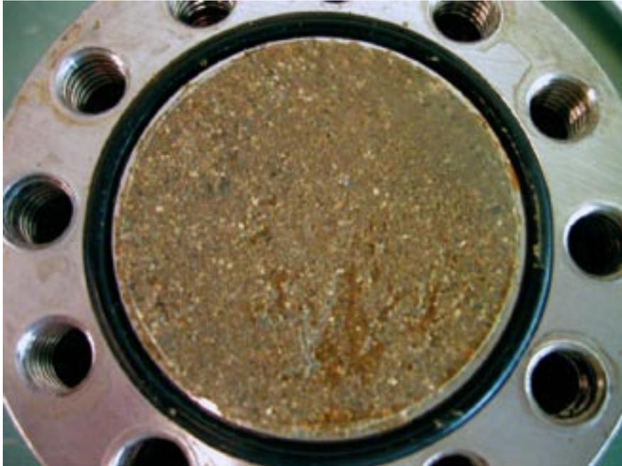
*Figure 10-5. Picture from specimen SH203 at the termination of the test. The drilled hole has healed completely.*
