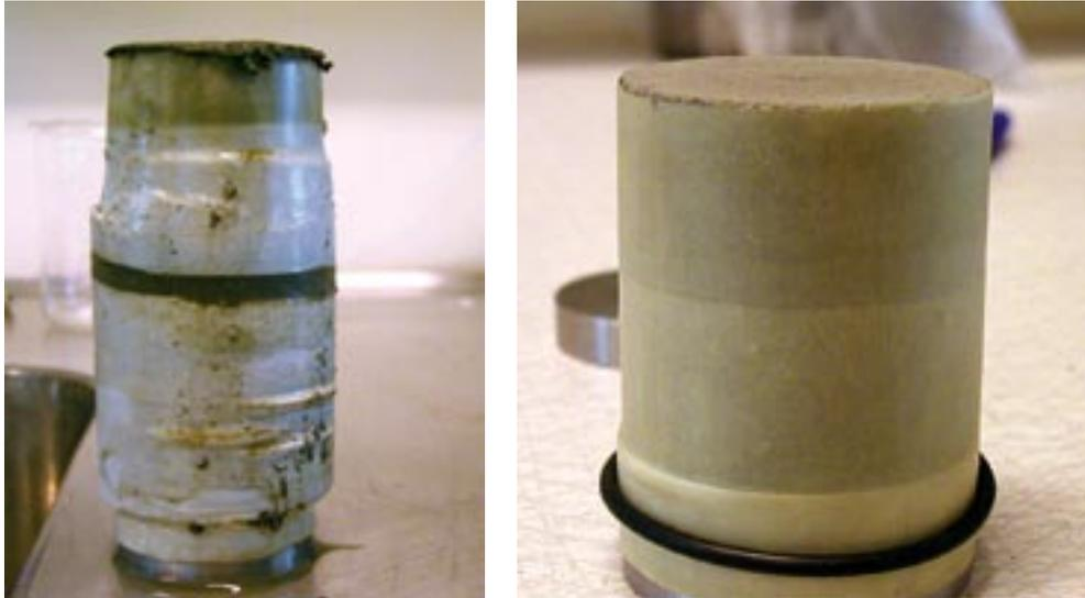
*Figure 8-2. Picture showing a Friedland specimen before (left) and after (right) testing.*
