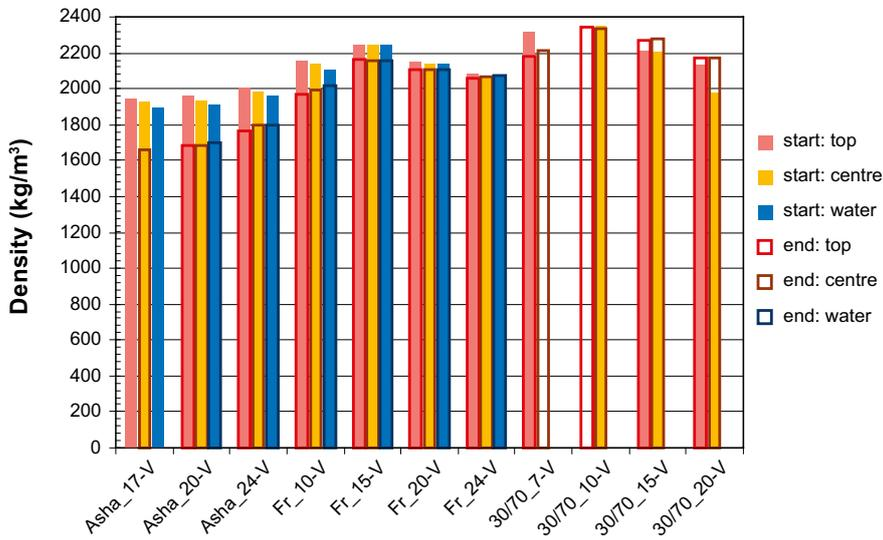
Figure 11-10. Initial densities compared with the corresponding densities at the end of the test for one of the test series.
