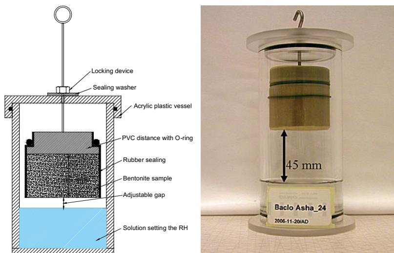
**Figure 11-1.** Schematic view showing the test equipment to the left and the equipment used for measuring water absorption rate to the right.
