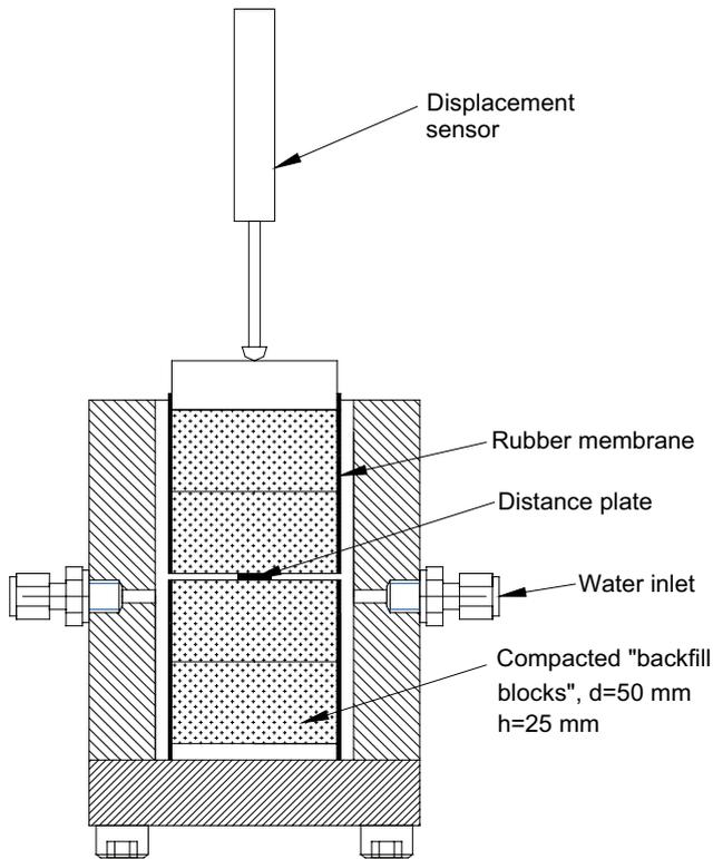
*Figure 8-1. Schematic drawing of the test equipment used.*
