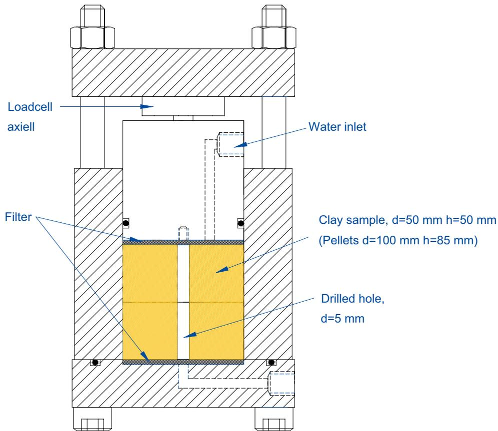
**Figure 10-1.** Schematic drawing of the test equipment used in self-healing tests. In the tests with MX-80 pellets a larger test cell was used (inner diameter= 101 mm, height= 85 mm).
