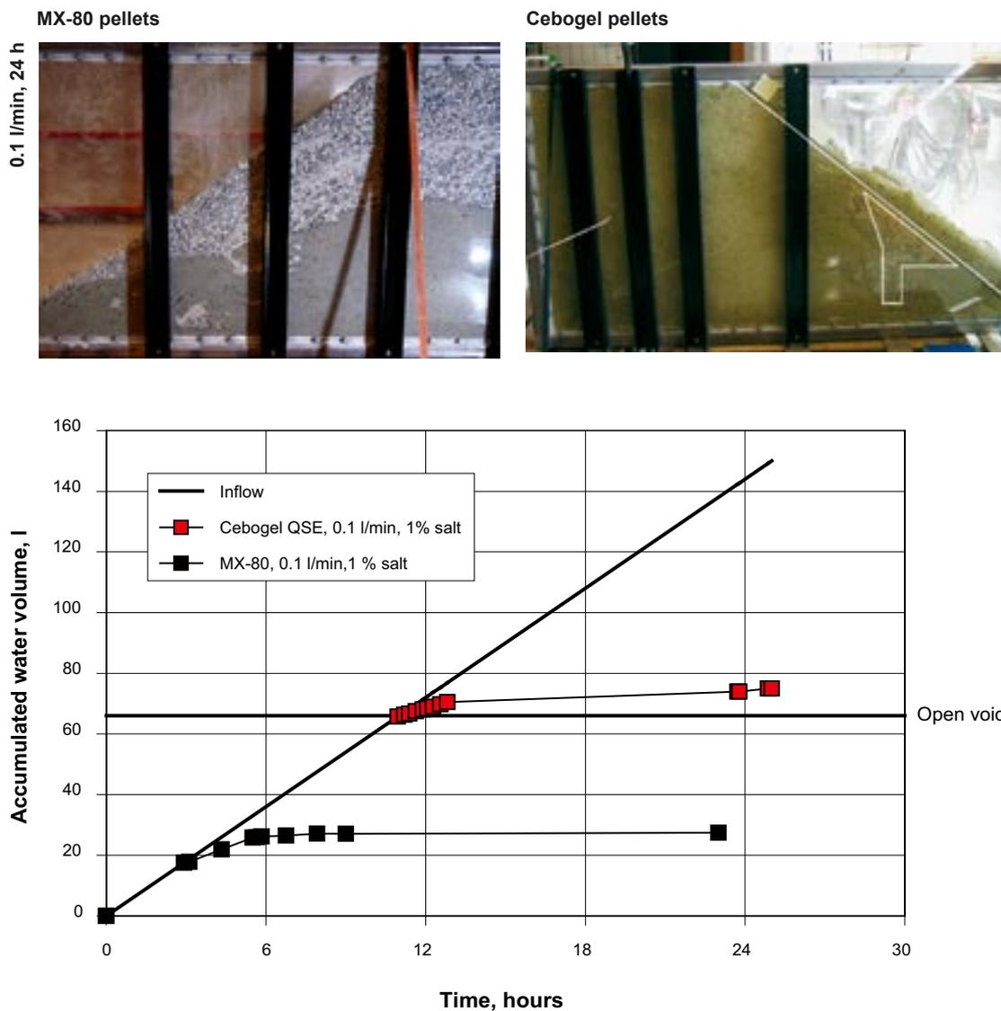
**Figure 6-3.** Upper: Pictures from the two tests performed with a water inflow rate of 0.1 l/min taken after 24 hours. Lower: The total inflow and the difference between inflow and outflow for the two tests plotted vs. time.
