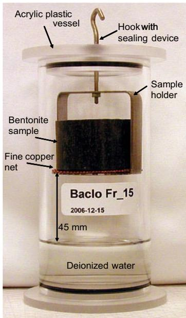
Figure 11-2. Equipment used for measuring swelling and studying cracking.
