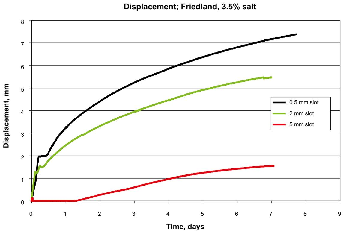
**Figure 8-4.** The results from the unconfined tests where displacement was measured (3.5% salt solution) plotted vs. time.
