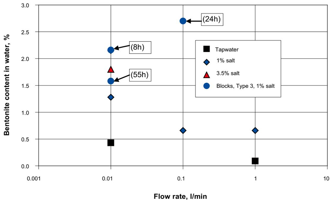
Figure 3-4. Compilation of all erosion measurements with Friedland blocks in laboratory. The average bentonite content in samples taken from the discharging water plotted vs. different flow rates. The circular blue dots show the values from the latest tests using Type 3 Friedland blocks, while the other test results are from Baclo Phase 2 tests where Type 1 Friedland blocks were used.
