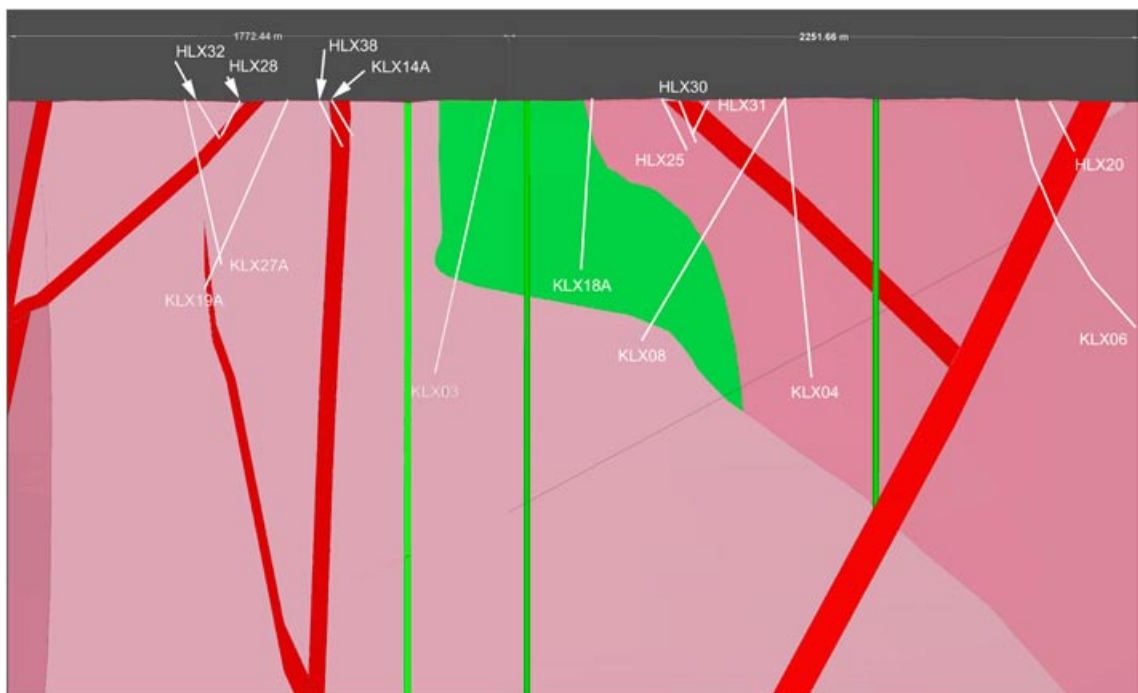
Figure 2-13. NW-SSE/W-E 2D cross-section from the western margin of the Laxemar subarea, through the central part and towards the eastern margin in the direction of (but not including) the Simpevarp subarea (cross-section #5 in Figure 2-11). Indicated are the major rock domains, the major deformation zones and the projected positions of the cored and percussion boreholes. The varying widths of the deformation zones reflect their orientation relative to the cross-sectional cut, (cross-section length = 4,024 metres; vertical thickness of section = 2,000 metres).
