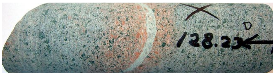
Figure 2-15. Red stained, hydrothermally altered rock adjacent to a fracture filled with prehnite. Sample KSH03A:128.08–123.23 m borehole length. Drill core diameter is approximately 5 cm.
