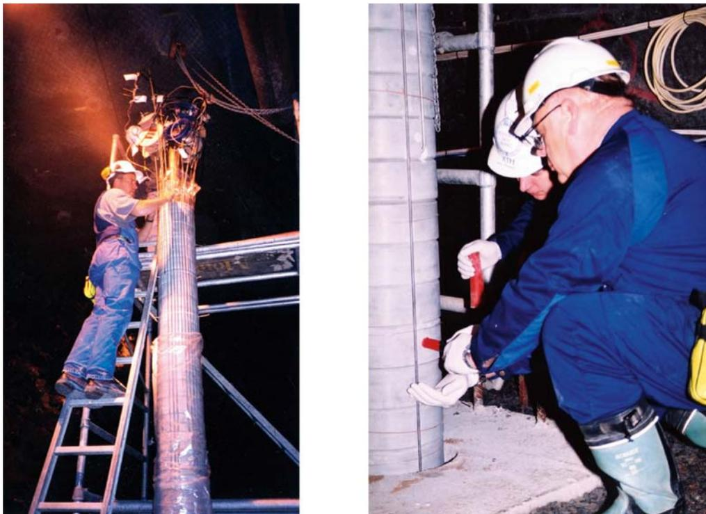
**Figure 4-1.** Left: Finalizing the construction of the A2 parcel at test site, note the large number of wire protecting tubes from sensors. Right: Insertion of the plug containing  $^{60}\text{Co}$  during lowering the parcel into the test hole. Note the limited amount of tubes in the lower hot section.
