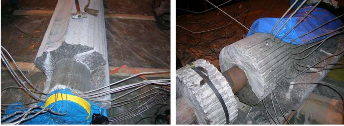
*Figure 4-8. Left: Photo taken just after the removal of the first piece of rock from the upper part of the parcel. Note the well covered sensor wire protecting tubes and the tight interface between bentonite and the covering rock. Right: Sawing cuts were made approximately at the original block interfaces and the released blocks were successively removed from the copper tube.*
