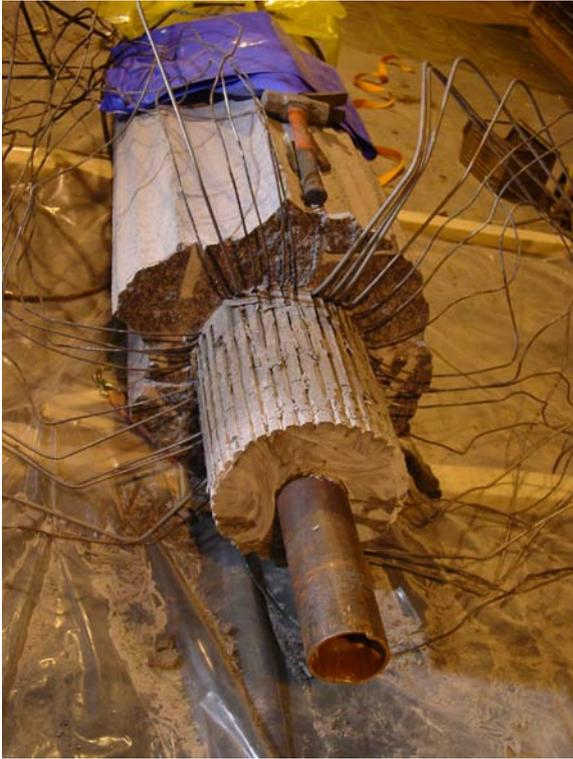
**Figure A8-4.** The lower part of the LOT parcel A2. The diameter of the bentonite blocks is 30 cm, stacked on the central copper tube. Sensor wires are located along the outside of the bentonite blocks (peeled back before dissection). The deep end is still contained within a rind of granite.
