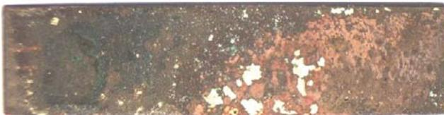
*Figure A3-1d. Distribution of the blue-green corrosion products (almost white in the picture) on side 2 of copper coupon A230G.*
