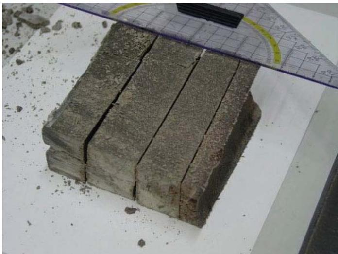
**Figure A8-16.** Cut profile from block 13. The heater was in contact along the right side (curved surface), and the contact to granite was along the left side. The lower edge represents the base of block 13.
