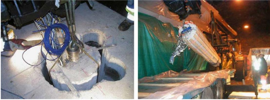
*Figure 4-7. Left: Top part of the parcel with attached lifting device. Note the surrounding slot made by overlapping percussion drill holes and the larger core drilled holes. Right: Entire A2 test parcel with rock-cover being placed on a lorry for transport.*
