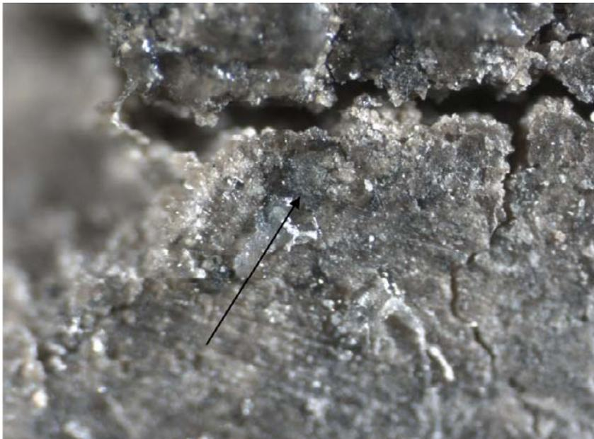
*Figure A7-15. Light microscopy image of the bentonite-Cu tube contact surface (image width appr. 4 cm).*
