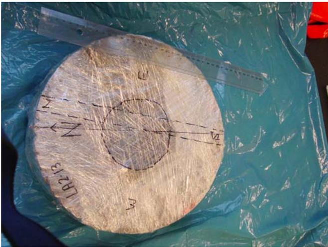
**Figure A8-12.** Sample block 13 (LA2-13) wrapped in plastic foil marked and ready for cutting. The top surface is oriented up in the experiment, and the radial orientation is relative to North. Two radial slabs were first cut, labelled N and S.
