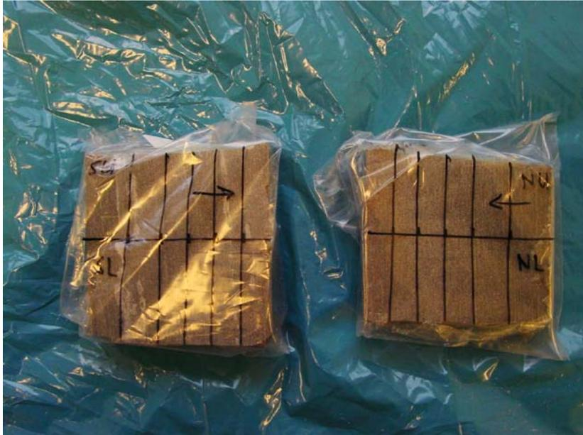
**Figure A8-14.** Two slabs marked for cutting 4 radial profiles for the measurement of water content. The profiles are labelled NU (North, upper profile), NL (North, lower profile), SU (South, upper profile), and SL (South, lower profile). The lines marking the cuts for the segments are only approximate
