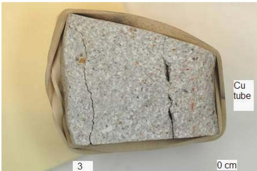
**Figure 9-1.** The section 0–3 cm of block 11 from the LOT A2 parcel. Note the brick-red “grains” occurring in the innermost 2 cm of the block. Fissures formed during storage.
