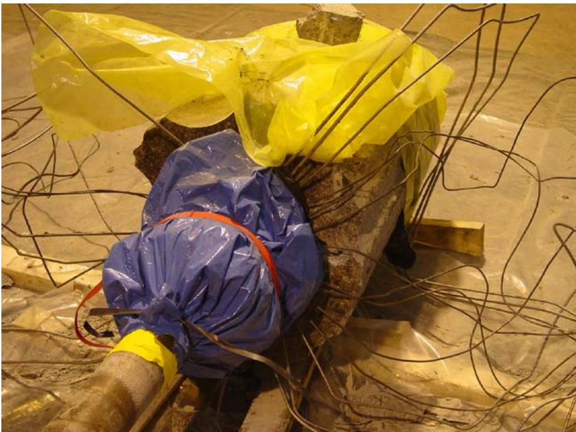
**Figure A8-5.** Protection of the bentonite section from drying out between the 1<sup>st</sup> and 2<sup>nd</sup> day of sampling.
