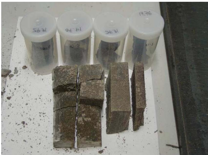
**Figure A8-17.** Cut profile from block 13 after subsampling. The larger pieces were processed to perform the CEC, ion selectivity and XRD analyses. Some reference samples were kept sealed and refrigerated (for water content, density).
