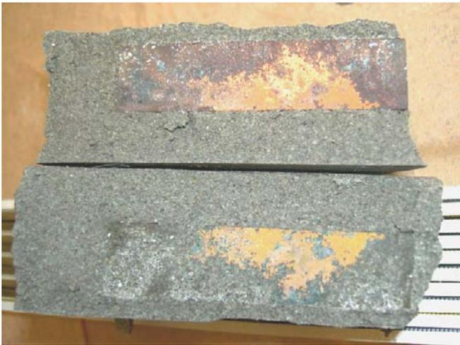
**Figure A3-1a.** Corrosion products seen on the adjacent bentonite after breaking loose copper coupon A230H. (The copper coupon is in place in the upper bentonite piece.)
