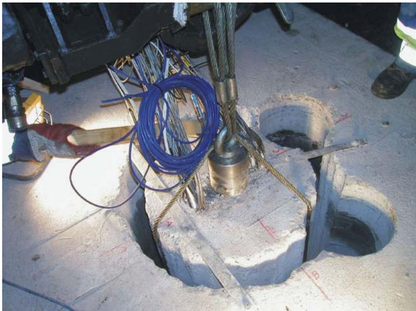
**Figure A8-3.** LOT parcel A2 ready to be lifted. The stack of bentonite blocks is completely contained in an outer rind of granite (image from O. Karnland, *Clay Technology*).
