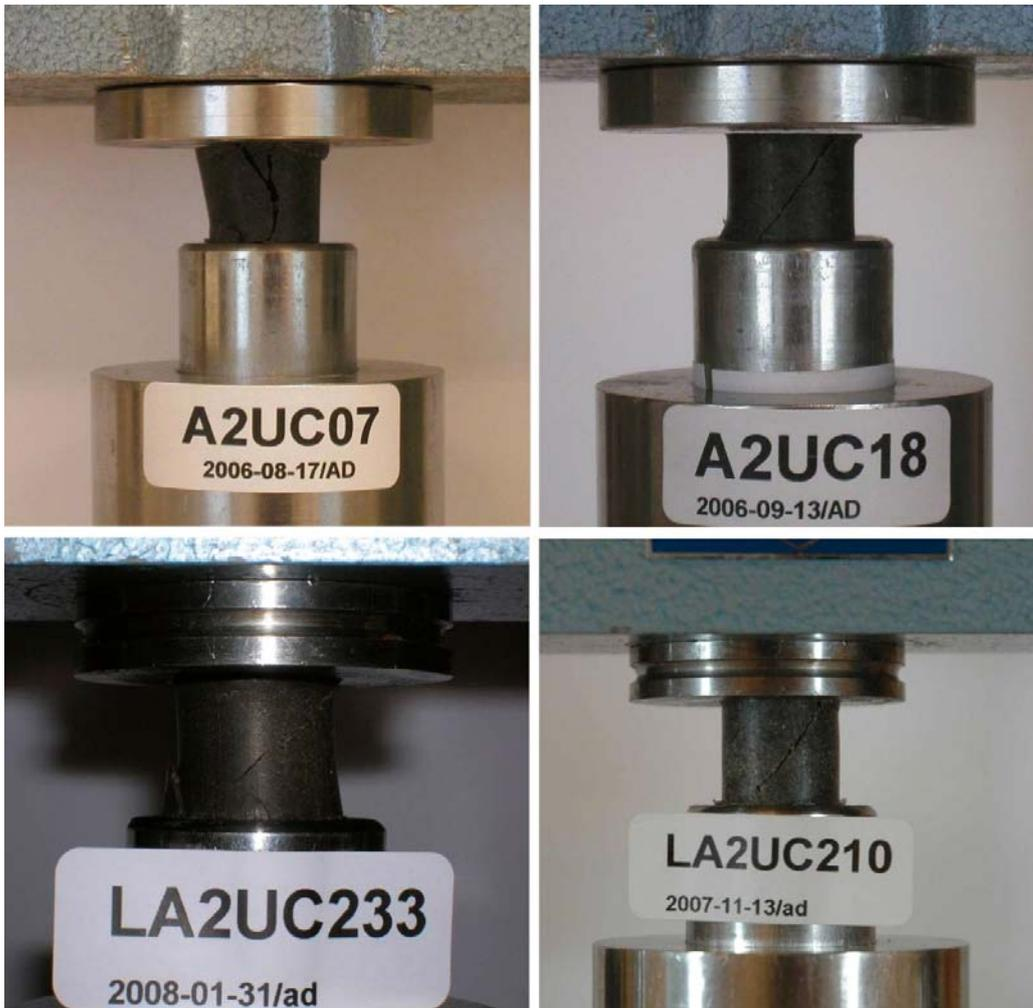
**Figure 8-12.** Photos of selected specimens after failure. The specimens represent block 09 position 1 cm (upper left), block 33 position 1 cm (upper right), air dried, milled and re-compacted material from block 11 position 1 cm (lower left) and compacted specimen exposed to 150°C in an oven in the laboratory (lower right).
