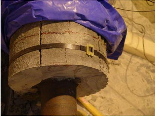
*Figure A8-6. Block 13 secured with a supporting nylon strap, and marked for cutting. The thickness of a block is 10 cm, the outer diameter 30 cm, and the inner diameter 11 cm. The radial width is 9.5 cm.*
