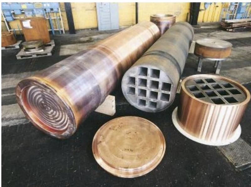
**Figure 1-1.** Nuclear waste disposal canisters of the Swedish design. (SKB).
