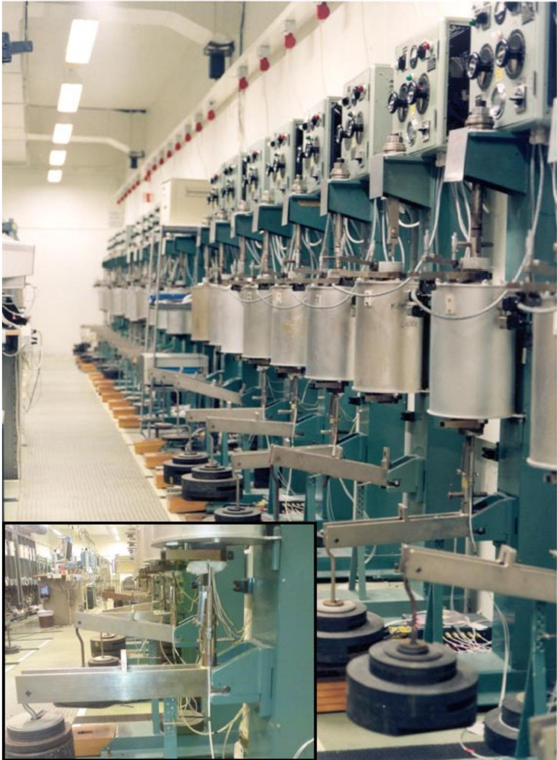
*Figure 3-4. The creep laboratory with creep rigs visible. Insert: a close-up on the lever arm.*
