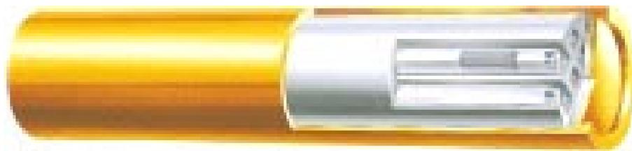
**Figure 11-1.** Copper canister and cast iron insert. The canister is 4,835 mm long, 1,050 mm in diameter and 50 mm in wall thickness.
