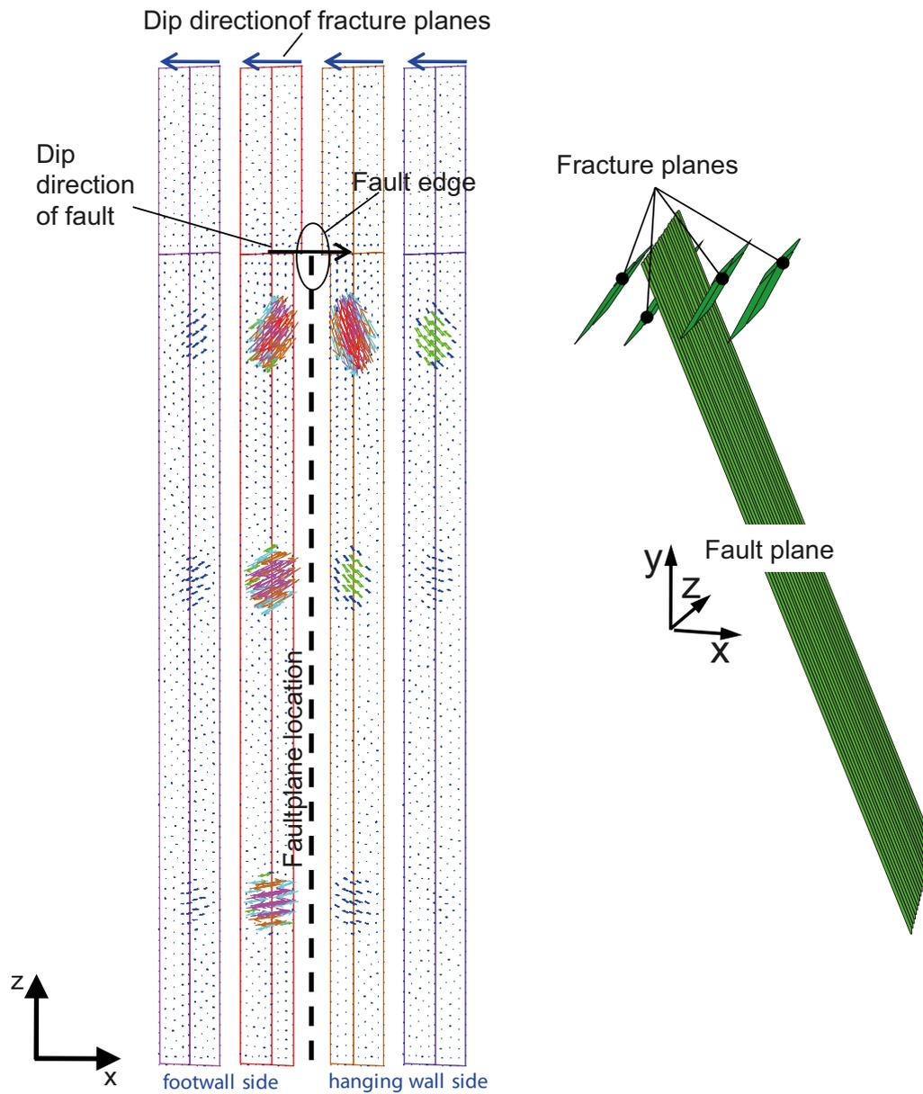
**Figure 5-34.** Left: Vector plot showing induced fracture shear displacements in fractures with opposite dip direction to the fault in the M6\_Str1\_tfBASE\_rt05 model. The fracture planes are viewed from above. The black and blue arrows indicate dip directions of fault and fracture planes, respectively. Right: Locations and orientations of fracture planes.
