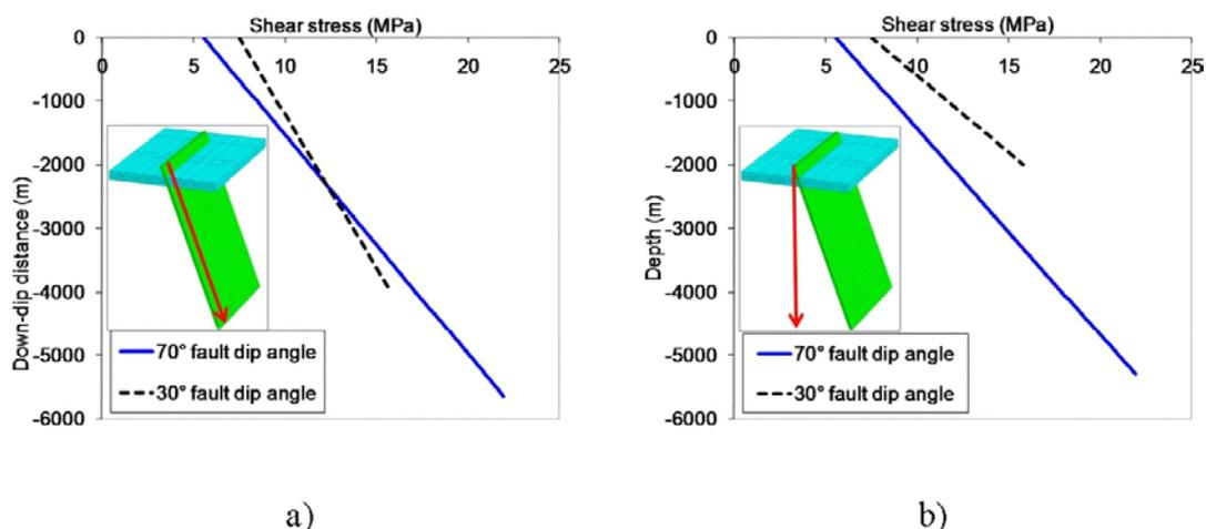
**Figure 4-10.** Initial fault shear stresses as function of a) down-dip distance and of b) depth in the  $M_w$  5.5 and  $M_w$  6.2 models. The meanings of down-dip distance and depth are illustrated by the insets.
