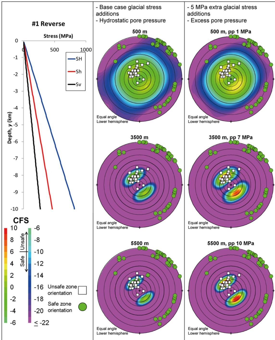
**Figure 7-11.** Contours of CFS values at three depths plotted along with the poles of Forsmark deformation zones. The colours of the plot symbols indicate zone orientations considered safe or unsafe according to the legend. Positive CFS values indicate instability. Circles denote 10° dip intervals. Upper left: The assumed *in situ* stress field. Middle: Hydrostatic pore pressure and stress additions only. Right: Excess pore pressure and 5 MPa extra glacial stress addition.
