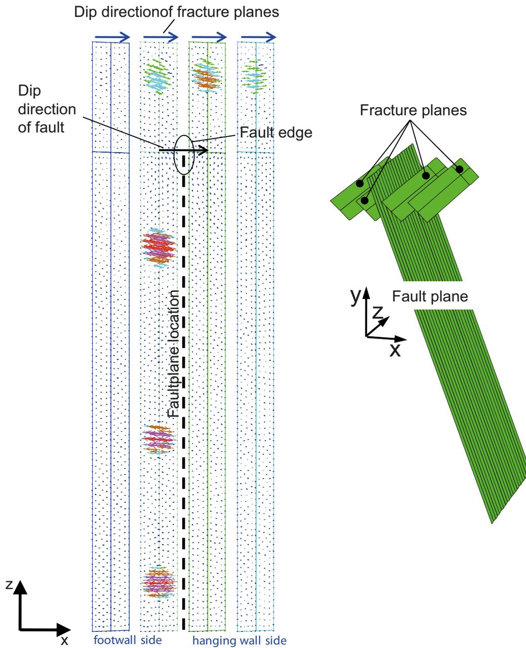
**Figure 5-33.** Left: Vector plot showing induced fracture shear displacements in fractures with same dip direction as the fault in the M6\_Str1\_tfBASE\_r105 model. The fracture planes are viewed from above. The black and blue arrows indicate dip directions of fault and fracture planes, respectively. Right: Locations and orientations of fracture planes.
