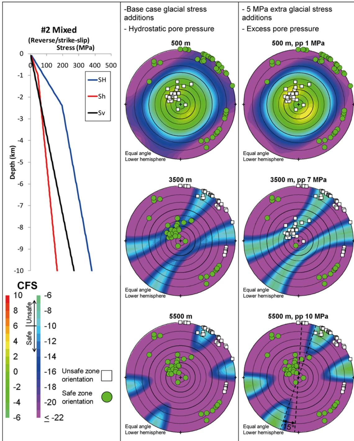
**Figure 7-12.** Contours of CFS values at three depths plotted along with the poles of Forsmark deformation zones. The colours of the plot symbols indicate zone orientations considered safe or unsafe according to the legend. Positive CFS values indicate instability. Circles denote 10° dip intervals. Upper left: The assumed in situ stress field. Middle: Hydrostatic pore pressure and stress additions only. Right: Excess pore pressure and 5 MPa extra glacial stress addition.
