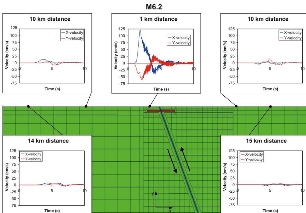
**Figure 6-9.** Velocities at the ground surface in M6\_str1\_tfBASE\_rt05. The distances that are given are with respect to the surface break of the fault.
