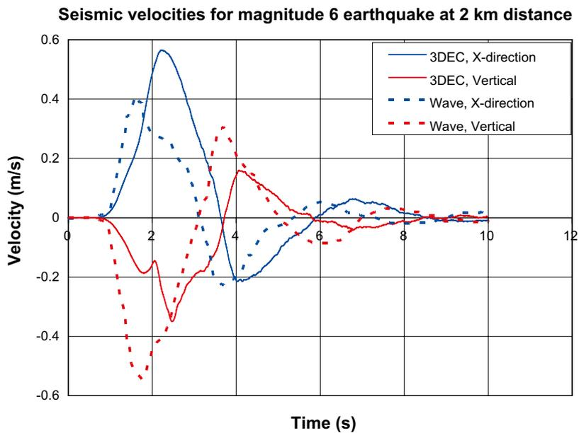
*Figure 6-18. Comparison between velocity records from the 3DEC model and WAVE model. The 3DEC results were taken from the footwall side (recording point 2).*
