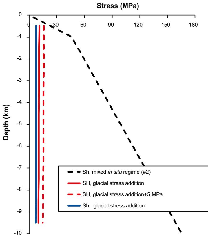
**Figure 7-10.** Comparison between the minor horizontal stress component in the mixed *in situ* stress model and the glacial stress addition components at 11 ka BP /Lund et al. 2009/. The diagram shows that the glacial stress additions are relatively low compared to the *in situ* stresses and that they are relatively insensitive to the depth. This means that their relative importance decreases with depth.
