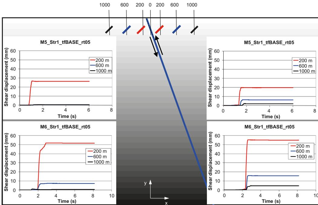
**Figure 5-16.** Temporal development of induced target fracture shear displacements at three horizontal distances from the primary fault in the *M5\_Str1\_tfBASE\_rt05* and *M6\_Str1\_tfBASE\_rt05* models. Dip direction: opposite to fault dip direction. Left diagrams: footwall side. Right diagrams: hangingwall side.
