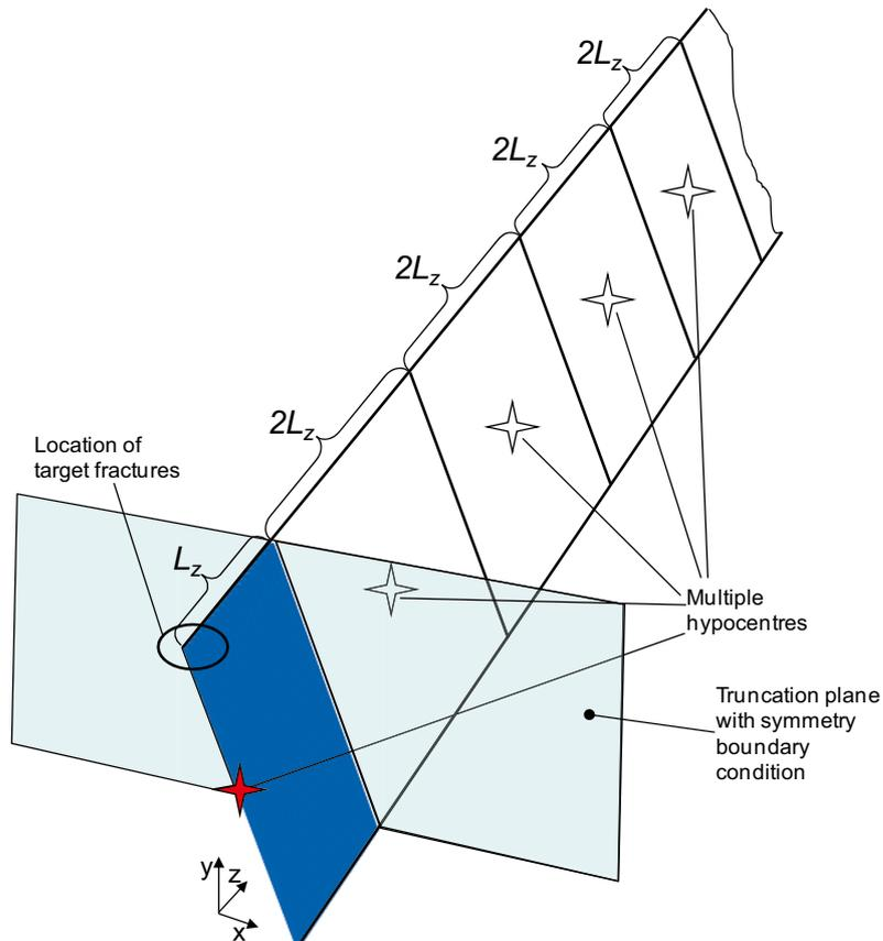
**Figure 4-14.** Having symmetry boundary condition at the truncation plane means that the truncated model simulates a fault of infinite length and with an infinite number of hypocentres.
