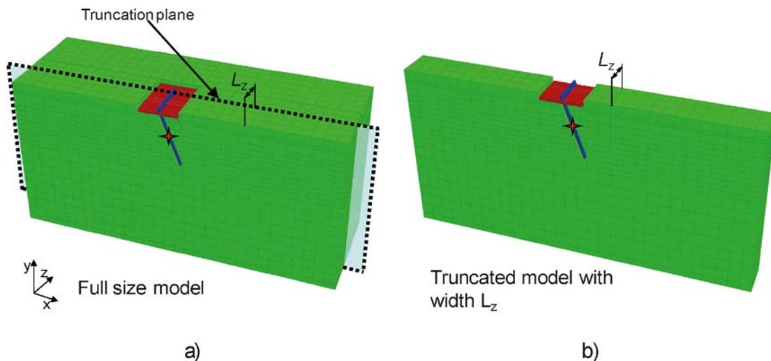
**Figure 4-13.** The principle for truncation of model. Left: Full size model that includes the entire fault plane. Used to model  $M_w$  5.5 and  $M_w$  6.2 events. Right: Truncated model in which the fault plane is cut at the truncation plane. Used to model  $M_w$  7.5 events.
