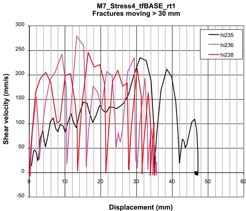
*Figure 5-26. Target fracture shear velocity versus displacement in the fractures with displacements > 30 mm in the M7\_Str4\_tfBASE\_rt1 model.*
