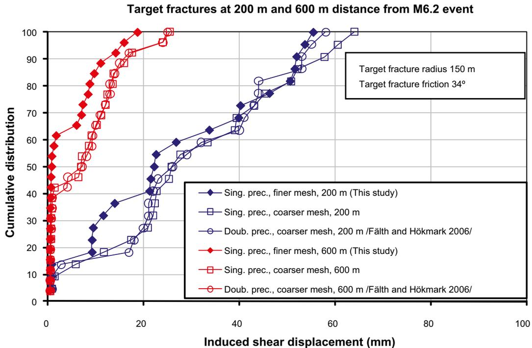
**Figure 6-15.** Cumulative distribution of induced target fracture shear displacements. The results from three models are shown: (1) Double precision model, coarser discretisation /Fälth and Hökmark 2006/, (2) Single precision model, coarser discretisation, (3) Single precision model, finer discretisation (this study).
