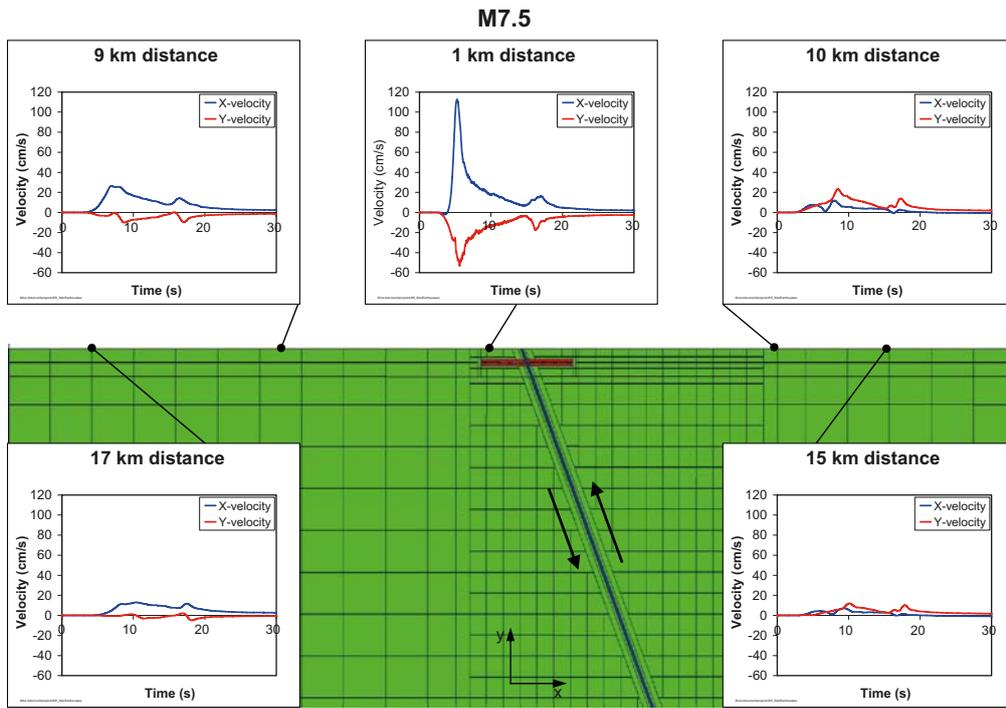
**Figure 6-10.** Velocities at the ground surface in *M7\_str4\_tfBASE\_rt1*. The distances that are given are with respect to the surface break of the fault. The wave passing after 17–18 s is due to reflections at the truncation boundary. This does not have any importance for the results.
