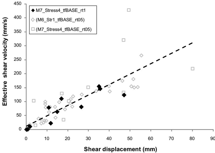
**Figure 5-29.** Effective target fracture shear velocity plotted versus corresponding maximum fracture shear displacement. Results compiled from the models discussed in this section (cf. Table 5-2). Two of the models are discarded in the final assessment (Section 7.1). These are represented by the unfilled plot symbols. The dashed line is a linear regression line.
