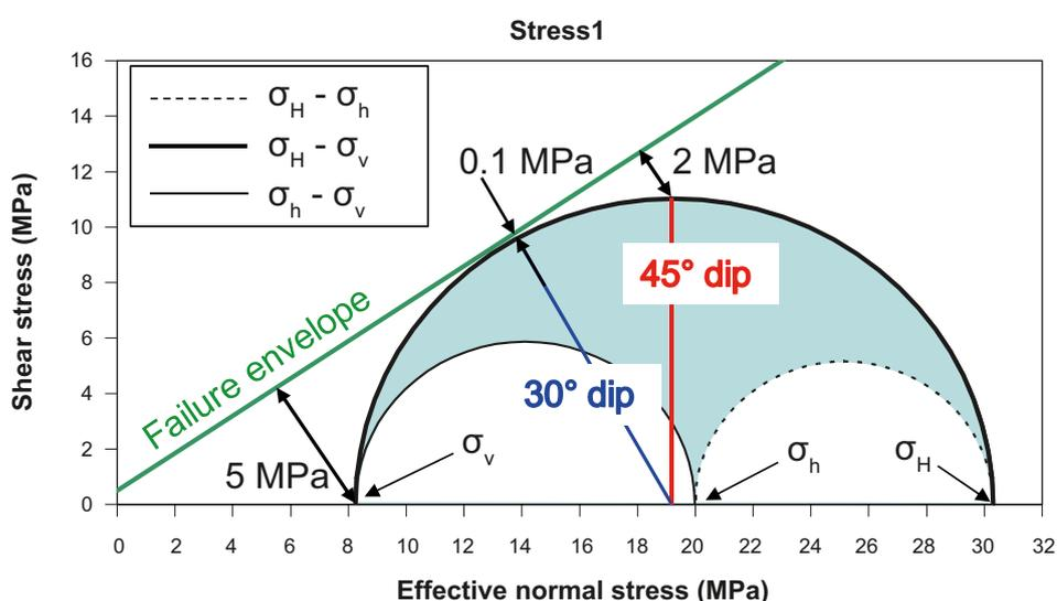
**Figure 4-11.** Mohr's circle diagram illustrating the Stress1 initial stresses at 500 m depth. The green line is the failure envelope for the target fractures. The numbers indicate the stability margins for horizontal fractures and for fractures dipping 30° and 45° in the  $\sigma_H - \sigma_v$  plane.
