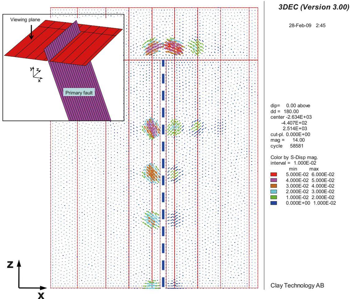
**Figure 5-35.** View from above of resulting shear displacement vectors in horizontal target fractures in the M6\_Str1\_tfBASE\_rt05 model. The dashed blue line indicates the intersection between the fault plane and the repository horizon. The colour code gives displacements in metres according to the colour legend. Text above the colour legend is 3DEC plot information (relating to orientation and position of viewing plane) and runtime information.
