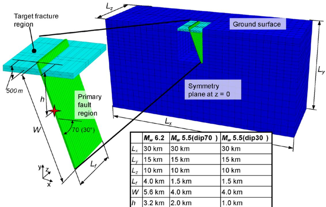
**Figure 4-6.** Outlines and dimensions of the  $M_w$  5.5 and  $M_w$  6.2 models. There are two sets of  $M_w$  5.5 models with 70° and 30° primary fault dip angles, respectively. Note that parts of the model geometry have been hidden for illustrative purposes.
