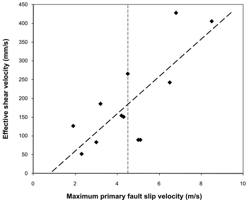
**Figure 5-30.** Effective target fracture shear velocity plotted versus maximum primary fault slip velocity. Results compiled from  $M_w$  5.5,  $M_w$  6.2 and  $M_w$  7.5 models. The highest target fracture effective shear velocity in each model is plotted. The dashed line is a linear regression line.
