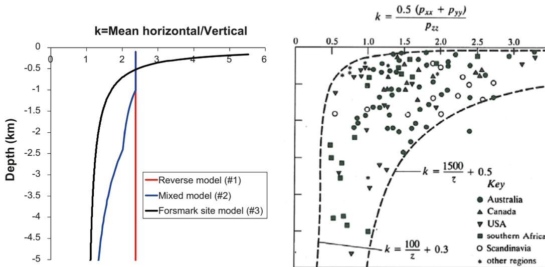
Figure 7-8. Ratio between mean horizontal stress and vertical stress. Left: The stress models considered here. Right: Measured data, worldwide (After /Brown and Hoek 1978/; note that max depth is 3 km).
