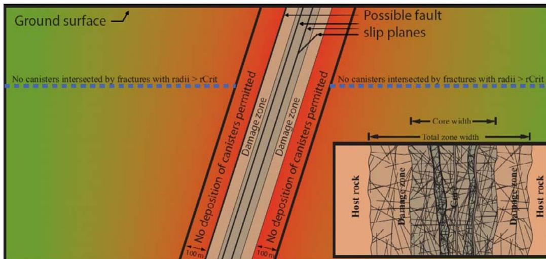
**Figure 1-8.** Respect distance rules, layout D2. The critical fracture radii,  $r_{Crit}$  (the size of the fractures that determine whether intersected canister positions should be accepted or rejected) will vary with distance from the closest potential slip plane.
