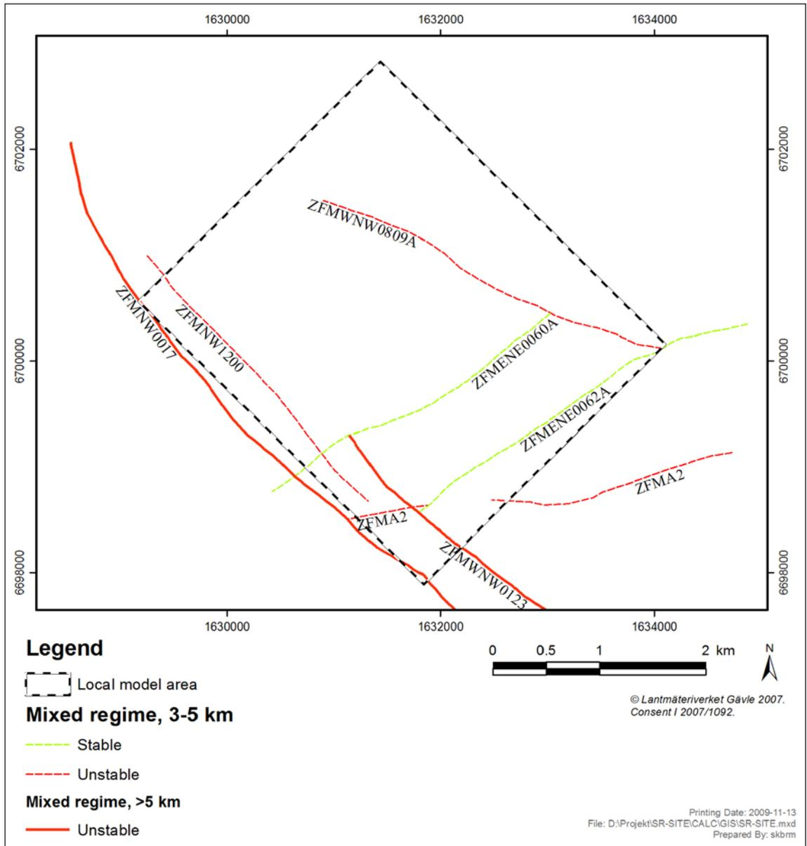
**Figure 7-15.** Map of deformation zones at repository depth<sup>6</sup>, -470 m /Stephens et al. 2008/. Zones with trace lengths > 3 km are shown. Zones within 600 m distance from any canister are coded with respect to their stability at 3.5 km depth according to the (#2) mixed stress regime assumptions applied in Figure 7-12. Stable zones are green and unstable are red.
