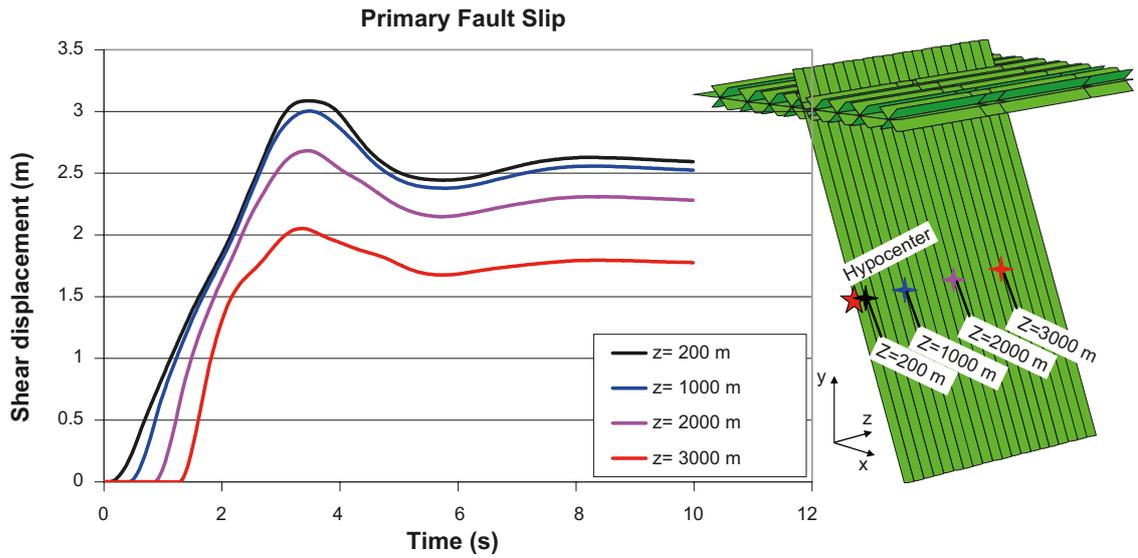
Figure 5-4. Temporal development of primary fault slip at four points at hypocentre depth in the M6\_Str1\_tfBASE\_rt05 model. The points are located at different distances from the hypocentre.
