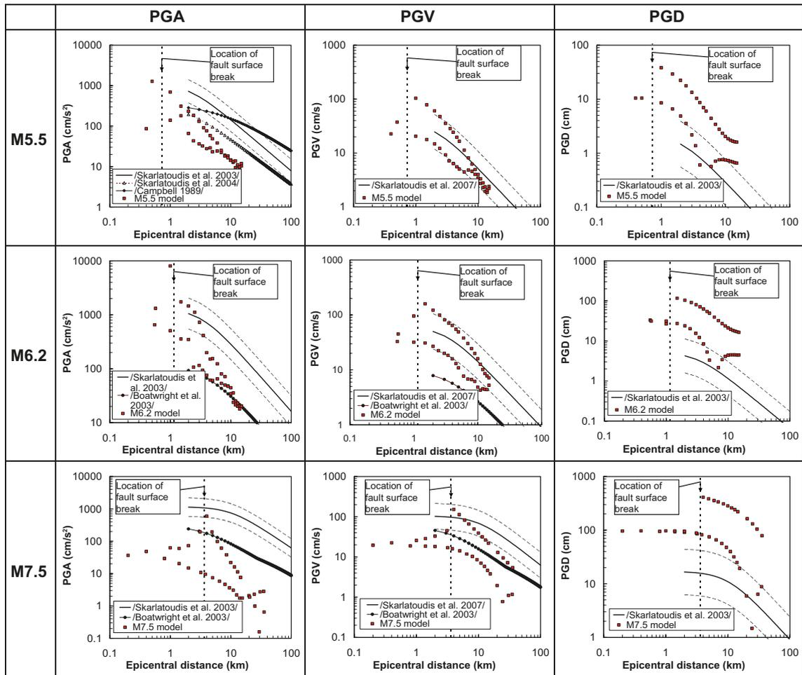
**Figure 6-12.** Comparison of PGA, PGV and PGD in (upper)  $M_w$  5.5 models, (middle)  $M_w$  6.2 models and (bottom)  $M_w$  7.5 models with empirical attenuation relations from /Campbell 1989, Skarlatoudis et al. 2003, 2004, 2007, Boatwright et al. 2003/ scaled to the actual earthquake magnitude. The  $\pm 1\sigma$ -curves are from /Skarlatoudis et al. 2003, 2007/. The location of the fault surface break is also indicated.
