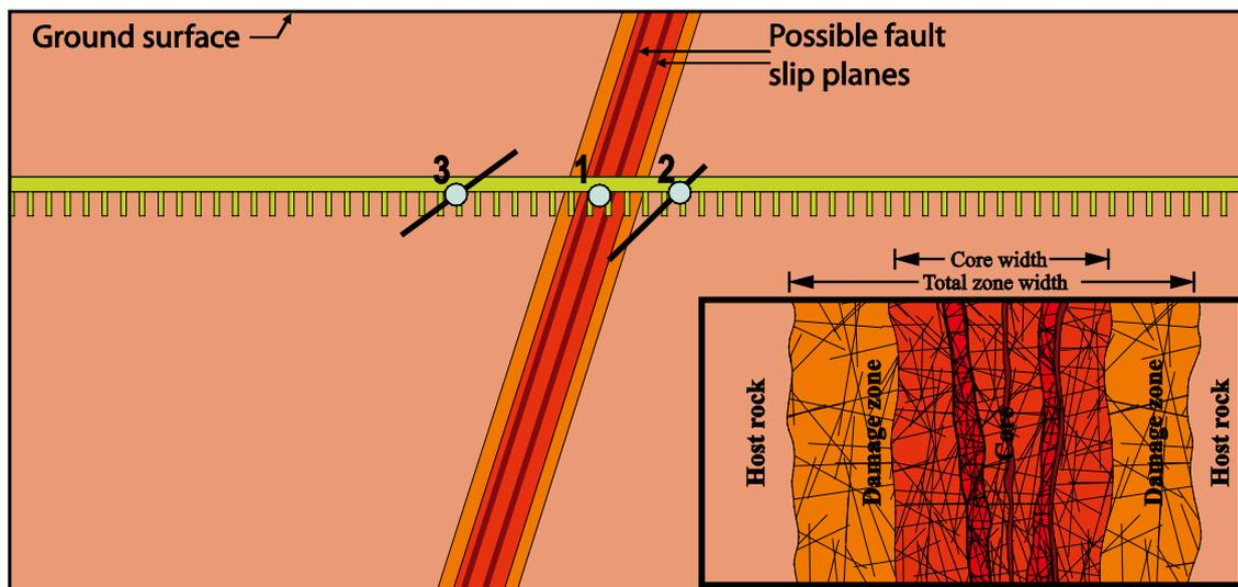
**Figure 1-5.** Shear displacements across a deposition hole can potentially occur because the deposition hole intersects 1) a slipping earthquake fault, 2) a fracture that is mechanically connected to a slipping earthquake fault, 3) a fracture that is remotely reactivated by a slipping earthquake fault. Inset shows deformation zone components, cf. /Munier and Hökmark 2004/.
