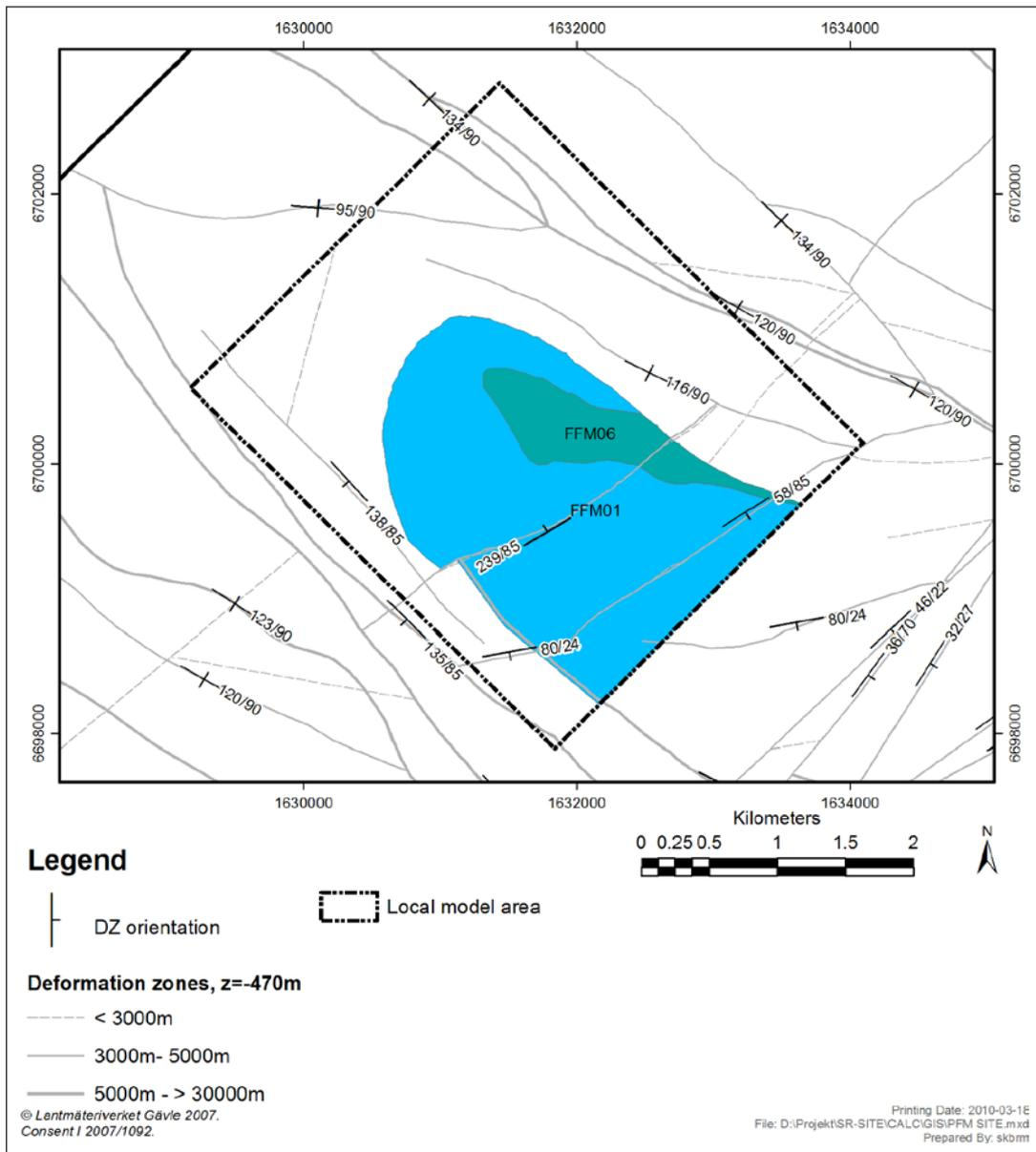
**Figure 1-9.** Map showing deformation zones at repository depth within the Forsmark local model area.<sup>1</sup> The numbers indicate strike/dip. /Stephens et al. 2008/.
