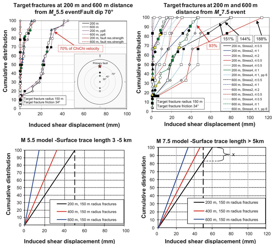
**Figure 7-1.** Upper: Modelling results for  $M_w$  5.5 and  $M_w$  7.5 earthquakes. Red arrows denote the results selected for the continued processing. Lower: schematic representation with linear slip distributions. “x” (lower, right) denotes the percentage of 150 m radius fractures that would slip more than the 50 mm canister damage threshold.
