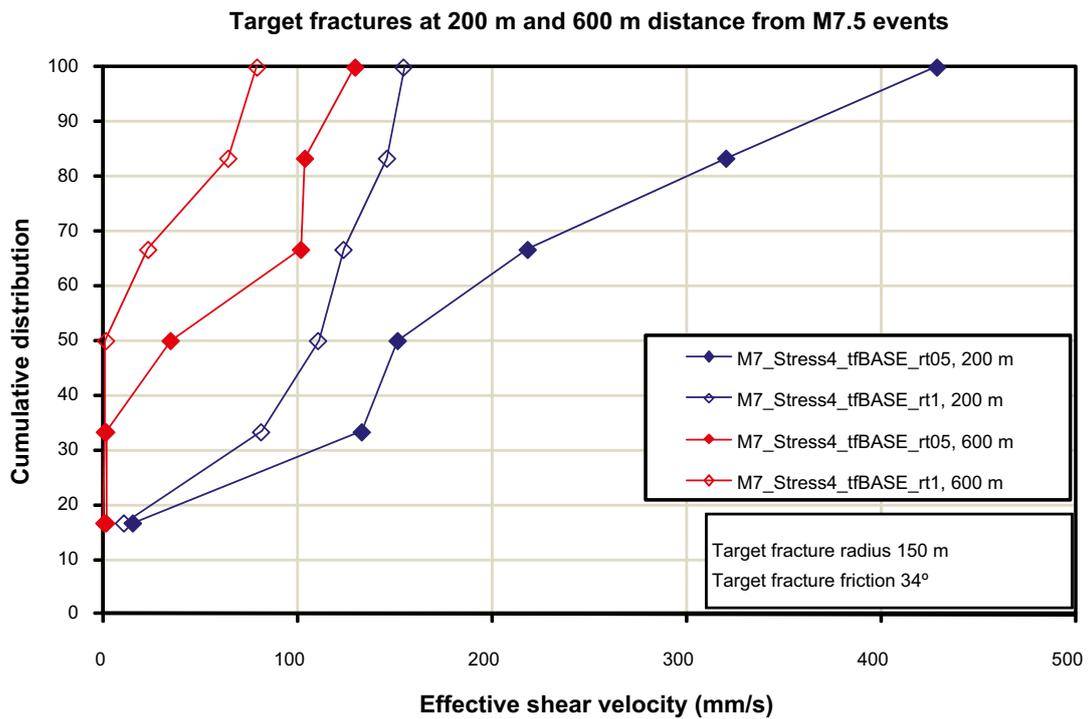
*Figure 5-28. Cumulative distribution of effective shear velocities in the two  $M_w$  7.5 models. Results at 200 m and at 600 m distance from the primary fault are shown.*
