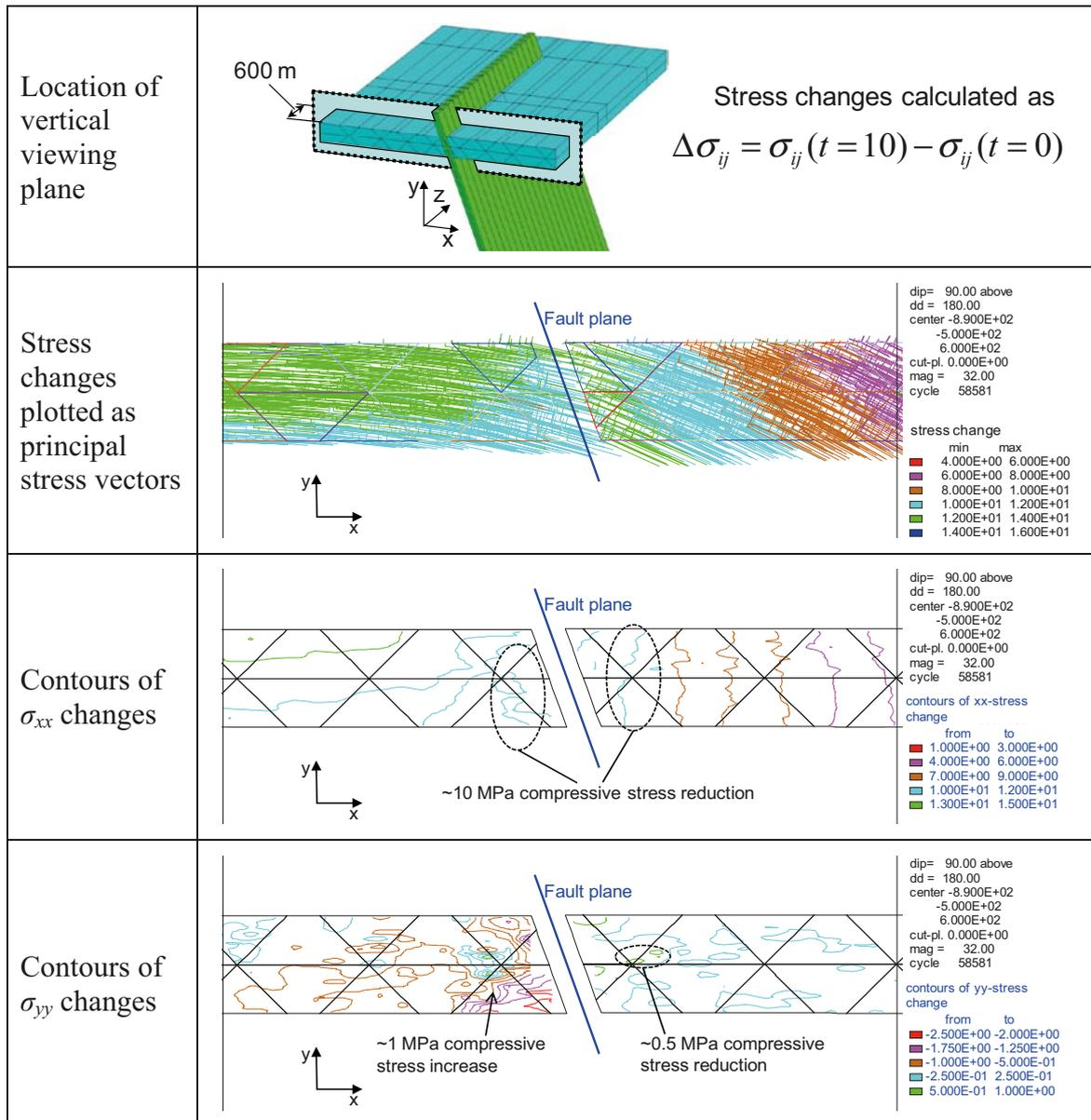
**Figure 5-9.** Stress changes at 500 m depth in M6\_str1\_tfBASE\_rt05 calculated as the difference between the stresses at  $t = 0$  s and  $t = 10$  s. The vertical viewing plane is located at  $z = 600$  m, i.e. between target fractures. Positive values indicate compressive stress reduction (stress relaxation) and negative values indicate compressive stress increase.
