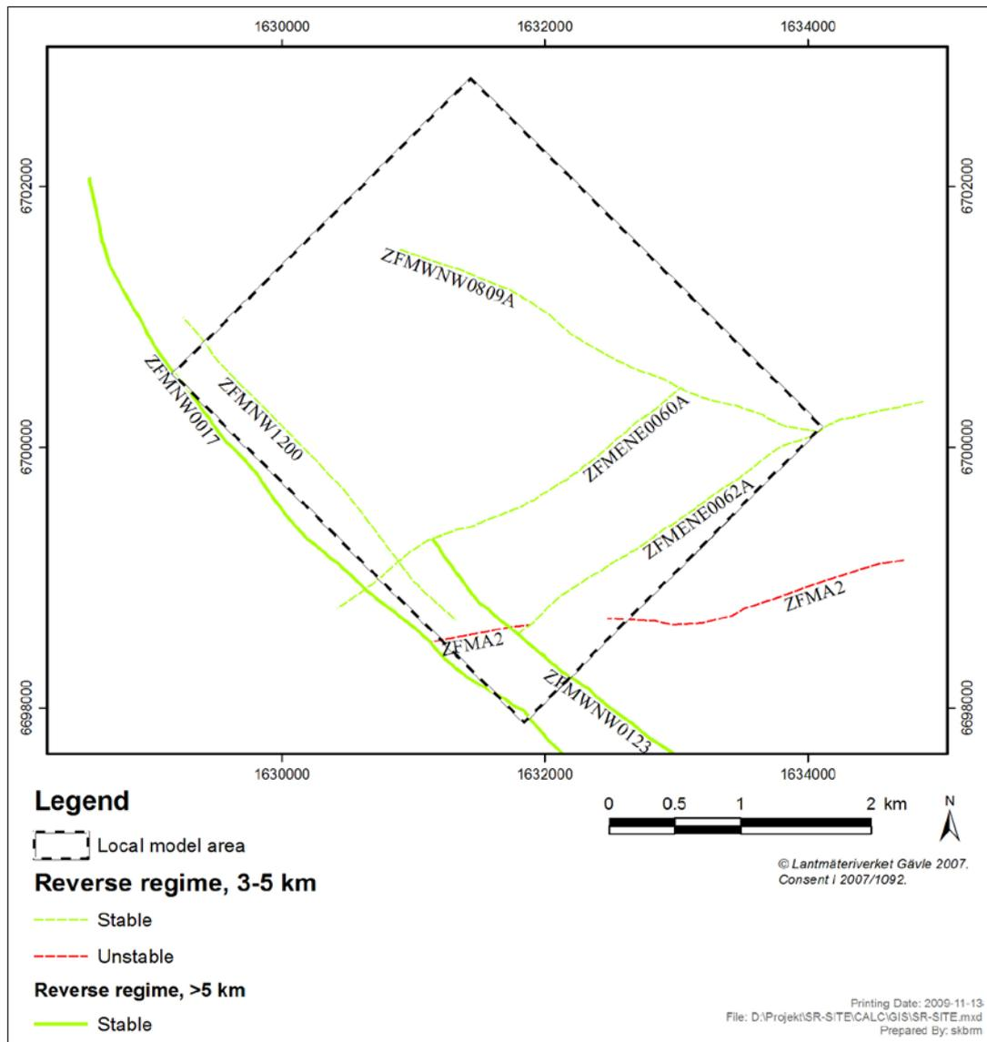
**Figure 7-14.** Map of deformation zones<sup>5</sup> at repository depth, -470 m /Stephens et al. 2008/. Zones with trace lengths > 3 km are shown. Zones within 600 m distance from any canister are coded with respect to their stability at 3.5 km depth according to the (#1) reverse stress regime assumptions applied in Figure 7-11. Stable zones are green and unstable are red.
