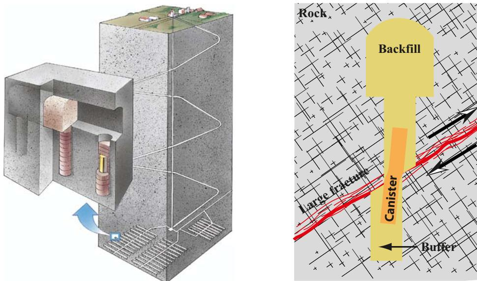
**Figure 1-4.** Left: Schematic of KBS-3 repository with ramp, system of horizontal tunnels and vertical deposition holes. Right: Shear displacement across deposition hole.
