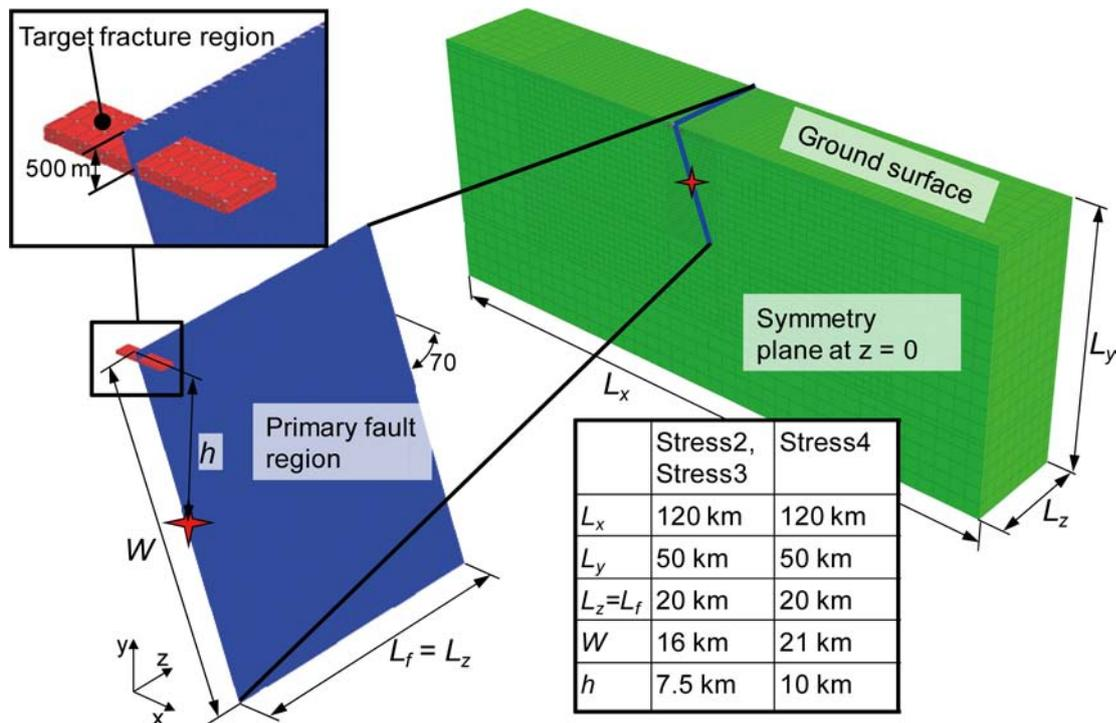
**Figure 4-2.** Geometric outlines of  $M_w$  7.5 models. Parts of the model geometry are hidden in the figure in order to show the primary fault and the target fracture region. The system of orthogonal planes is a set of construction planes used to define the geometry and to facilitate the discretisation of the continuum. Note that the fault length,  $L_f$ , is equal to the model width,  $L_z$ .
