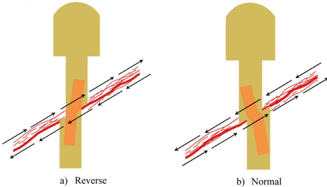
**Figure 5-31.** Sense of fracture shear displacement: a) Reverse shearing. All significant target fracture displacements found in the 3DEC models are of this type. b) Normal shearing.
