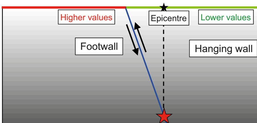
**Figure 6-13.** The models give in general higher values of PGA, PGV and PGD on the footwall side.
