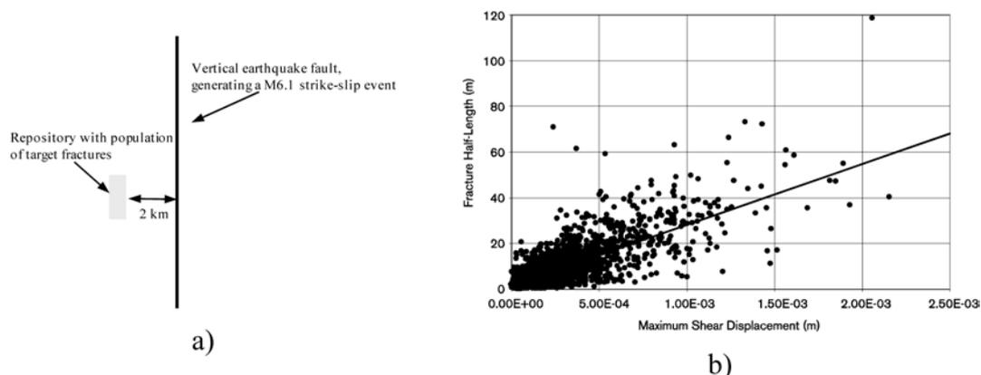
**Figure 2-1.** a) Schematic plan view of repository volume and earthquake fault. b) Relation between induced displacement and fracture size for frictionless fractures. From /Munier and Hökmark 2004, Figures 3-3 and 3-4/ based on /La Pointe et al. 1997/.
