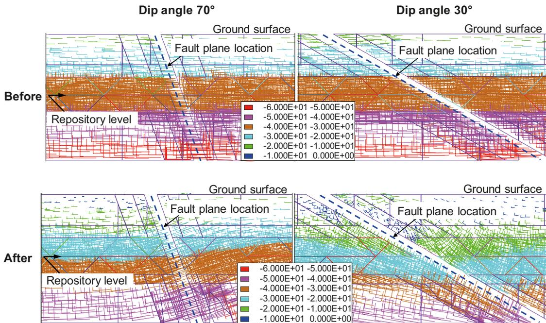
Figure 6-7. 3DEC principal stress vector plots in vertical sections in  $M5.5$  models with fault dip angle  $70^\circ$  (left) and with fault dip angle  $30^\circ$  (right). The vectors are coloured according to the magnitude of the major principal stress. Top: Before earthquake. Bottom: After earthquake. Note that compressive stresses are negative in 3DEC.
