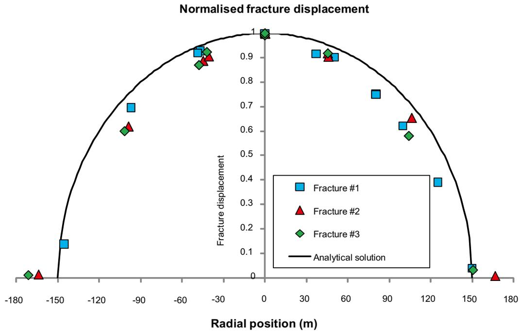
**Figure 5-37.** Normalised fracture displacement distribution as function of radial position. Analytical results and results from the M6\_Str1\_tfBASE\_rt05 model.
