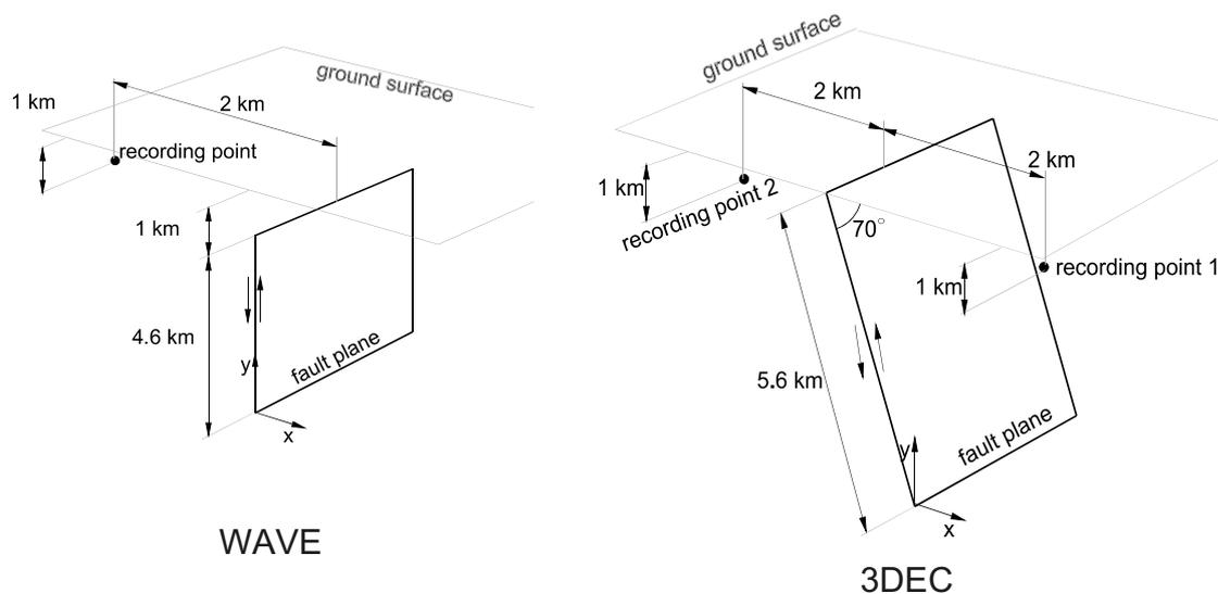
**Figure 6-16.** Conceptual geometries of the models and location of recording points. Left: *WAVE* model. Right: *3DEC* model.
