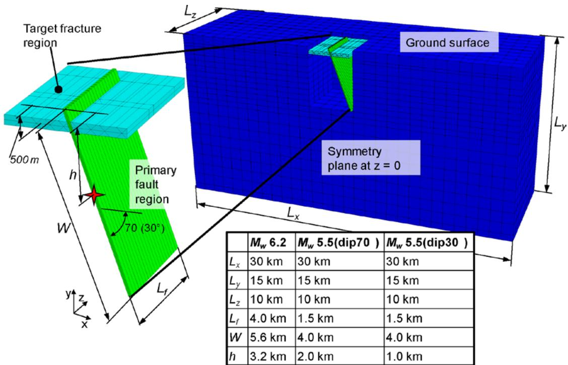
**Figure 4-1.** Geometric outlines of  $M_w$  5.5 and  $M_w$  6.5 models. Parts of the model geometry are hidden in the figure in order to show the primary fault and the target fracture region. The system of orthogonal planes is a set of construction planes used to define the geometry and to facilitate the discretisation of the continuum.
