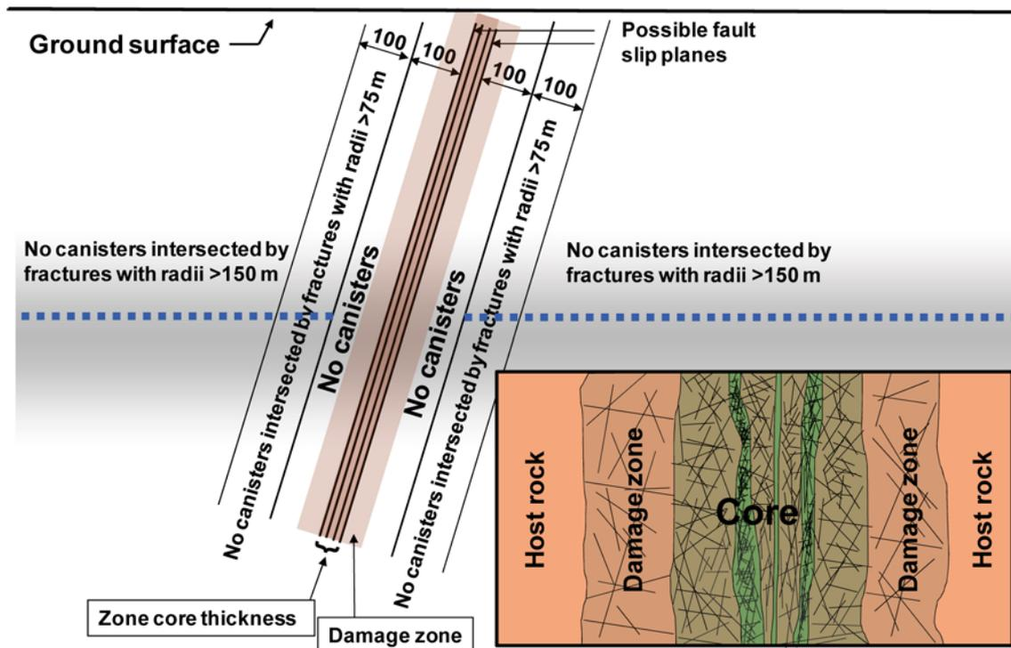
**Figure 1-7.** Schematic of respect distances applied in layout D1. All planes within the core of the deformation zone are regarded as potential slip planes. Inset shows deformation zone components, cf. /Munier and Hökmark 2004/. The total thickness of deformation zones (core + damage zone) at the Forsmark site is estimated to be in the range 10–100 m /Stephens et al. 2007/.
