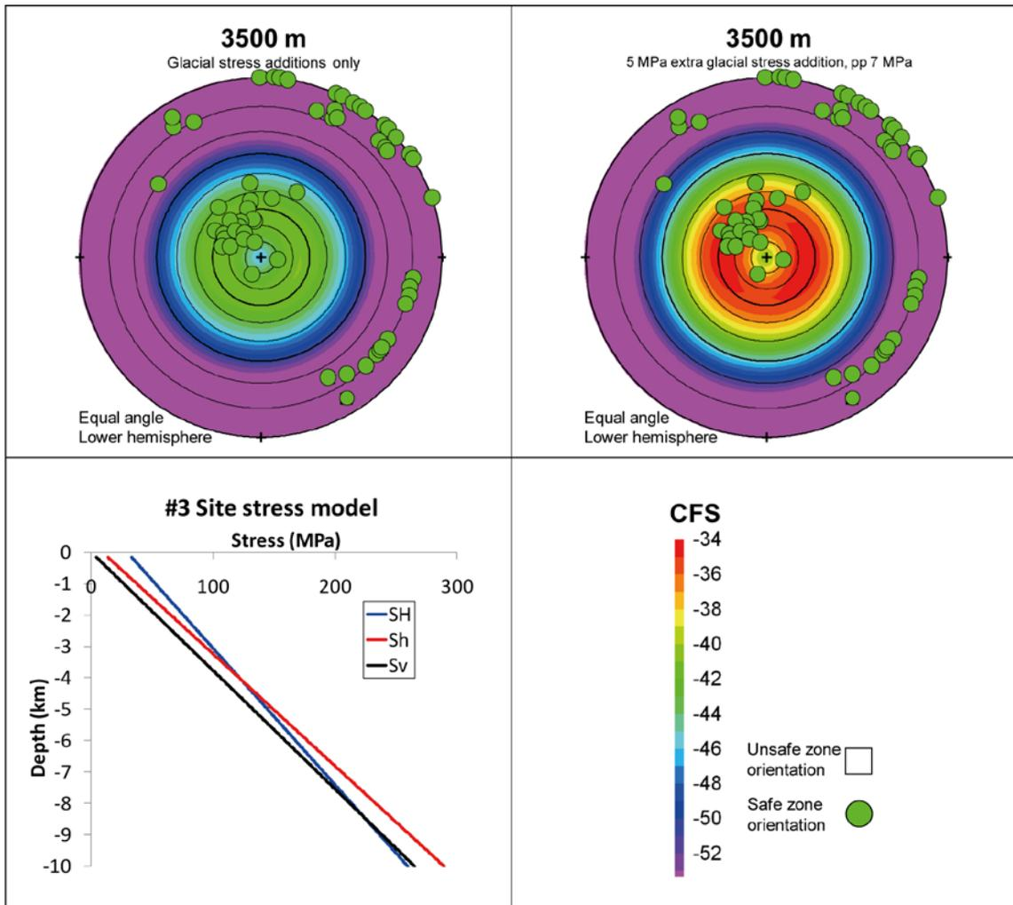
**Figure 7-13.** Contours of CFS values at 3,500 m depth plotted along with the poles of Forsmark deformations zones. The colours of the plot symbols indicate zone orientations considered safe or unsafe according to the legend. Positive CFS values indicate instability. Circles denote 10° dip intervals. Upper left: Hydrostatic pore pressure and stress additions only. Upper right: Excess pore pressure and 5 MPa extra glacial stress addition. Lower left: The assumed in situ stress field.
