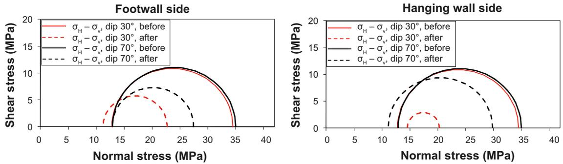
Figure 6-6. Mohr's circle diagrams illustrating stress states before and after earthquake in  $M_w$  5.5 models with fault dip angles  $30^\circ$  and  $70^\circ$ .
