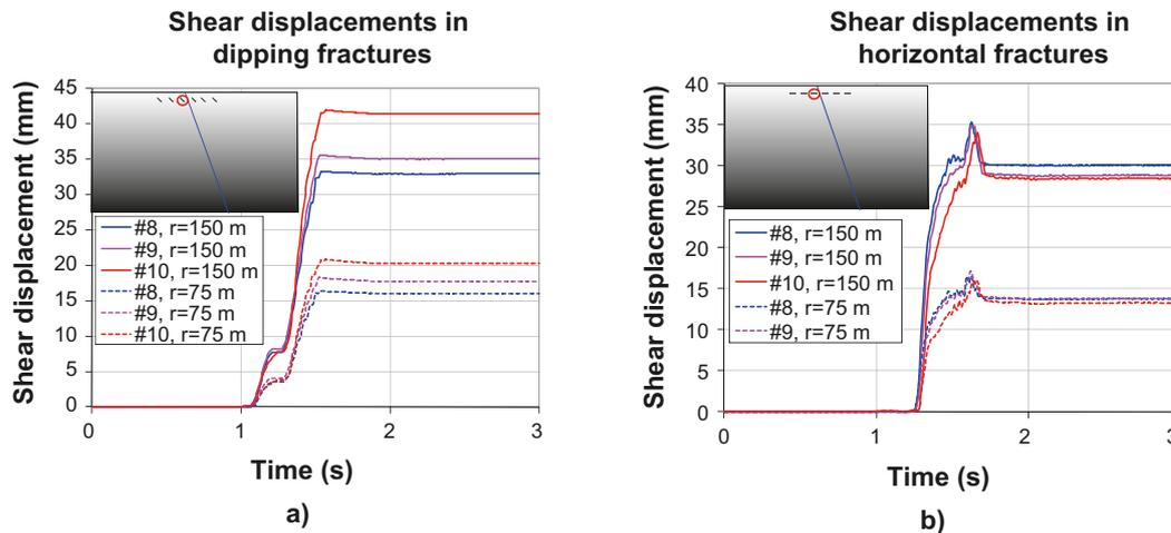
**Figure 5-36.** Induced shear displacements in test models. a) Dipping fractures and b) horizontal fractures. The results indicate that both displacements and velocities scale linearly with fracture size.
