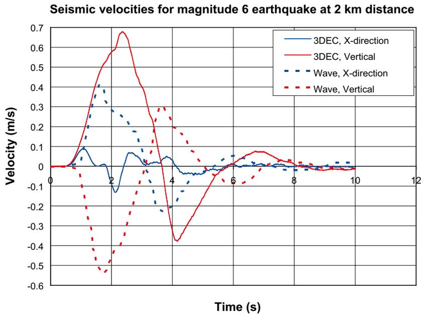
*Figure 6-17. Comparison between velocity records from the 3DEC model and WAVE model. The 3DEC results were taken from the hanging wall side (recording point 1).*
