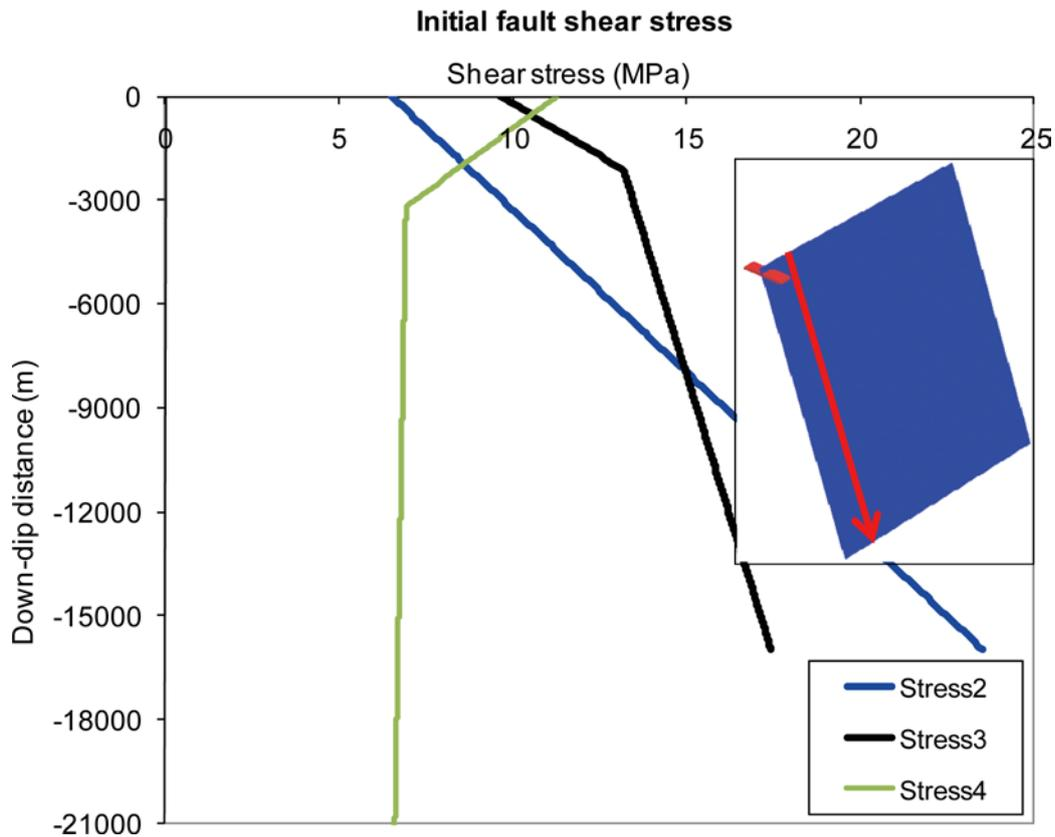
**Figure 4-19.** Initial fault shear stresses as function of down-dip distance in the  $M_w$  7.5 models. The meaning of down-dip distance is illustrated by the inset.
