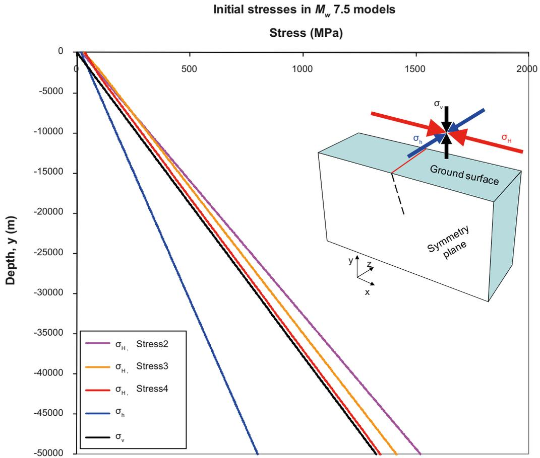
**Figure 4-18.** *In situ* stress directions and variations with depth,  $y$ , in the  $M_w$  7.5 models. Note that  $y$  is zero at the ground surface (upper boundary of model) and negative at depth.
