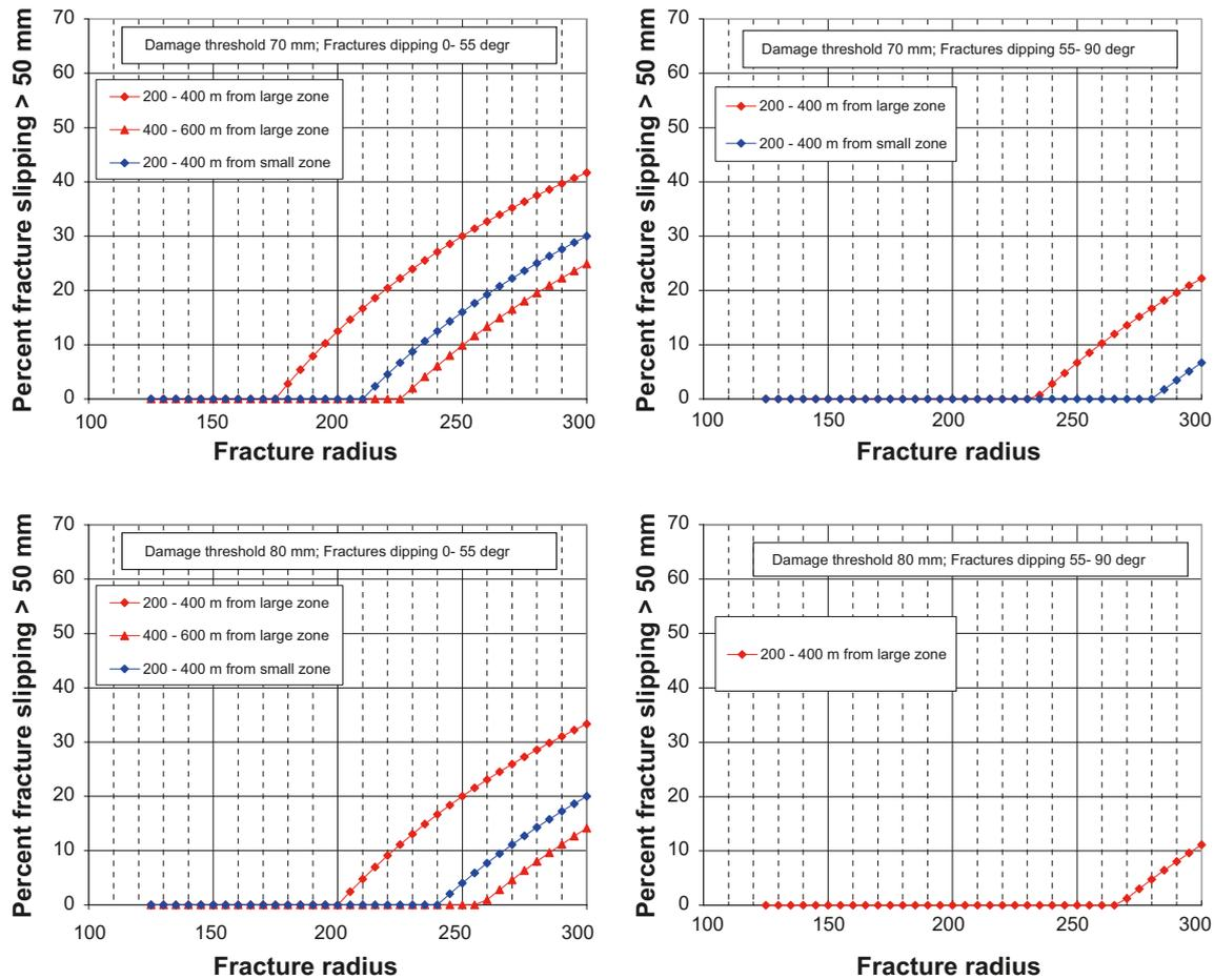
*Figure 7-4. Percentage of horizontal and gently-dipping (left) and steeply-dipping (right) fractures that will slip more than 70 mm (upper) and 80 mm (lower) as function of fracture radius. Red: fracture outside large zones. Blue: fractures outside small zones.*
