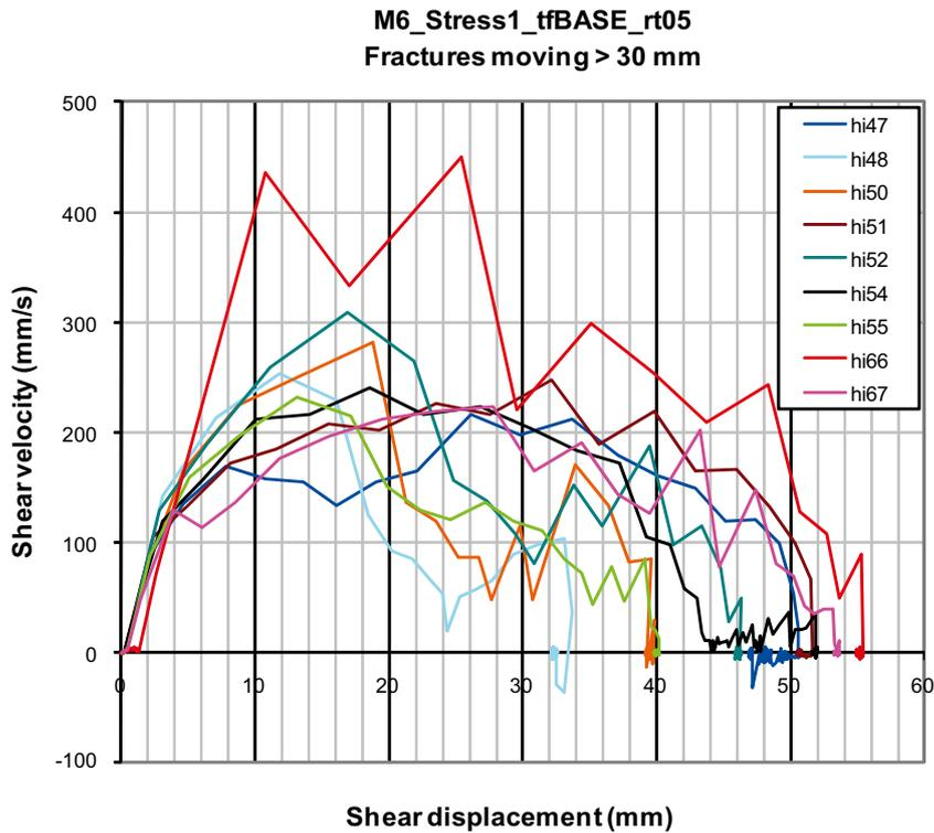
*Figure 5-25. Target fracture shear velocity versus displacement in the fractures with displacements > 30 mm in the M6\_Str1\_tfBASE\_rt05 model. For the fracture with the highest peak velocity (hi66) the velocity is higher than 400 mm/s during about 7 mm of the 50 mm total displacement.*
