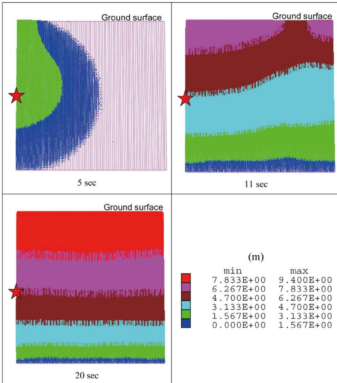
**Figure 5-3.** Vector plots showing primary fault slip at three instances of time in the M7\_Str4\_tfBASE\_rt05 model. The vectors are coloured according to their magnitudes. The star indicates the hypocentre.
