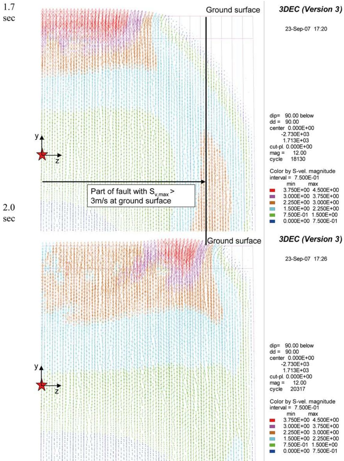
**Figure 6-5.** Upper: Primary fault slip velocity vectors after 1.7 s. Lower: Primary fault slip velocity vectors after 2.0 s. Results from the M6\_Str1\_tfBASE\_rt05 model with strength reduction time 0.5 s. The hypocentre is indicated with a red star. Note: The lower part of the fault plane is hidden in the plots.
