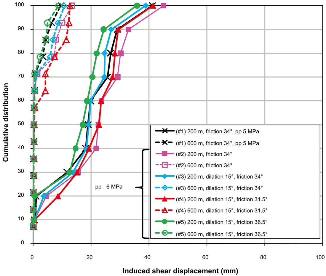
Figure 5-38. Cumulative distribution of induced target fracture shear displacements at different distances from the primary fault in  $M_w$  5.5 models. The colours denote models with different fracture strength parameter values. Each plot symbol represents the result of one particular fracture.
