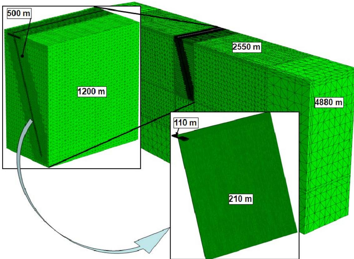
Figure 4-17. The finite-difference mesh in the  $M_w$  7.5 model. The numbers indicate the maximum zone edge lengths used in the different regions.
