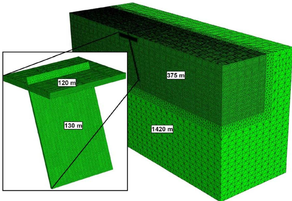
**Figure 4-7.** Outline of the finite-difference mesh in the  $M_w$  5.5 and  $M_w$  6.2 models. The numbers indicate the maximum zone edge lengths in the different parts of the models.
