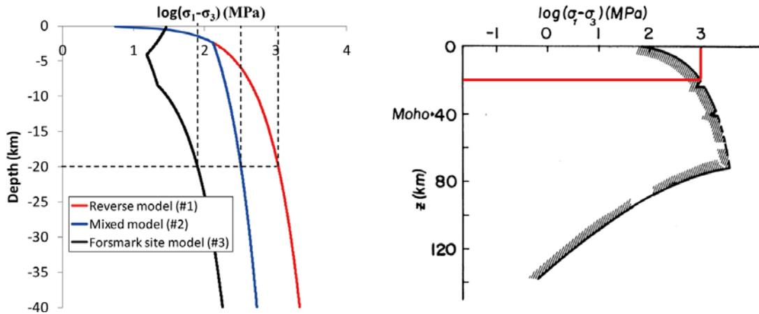
Figure 7-7. Left. Maximum principal stress difference as function of depth for the reverse and mixed stress models. Right: Maximum principal stress difference redrawn from /Milnes et al. 1998/
