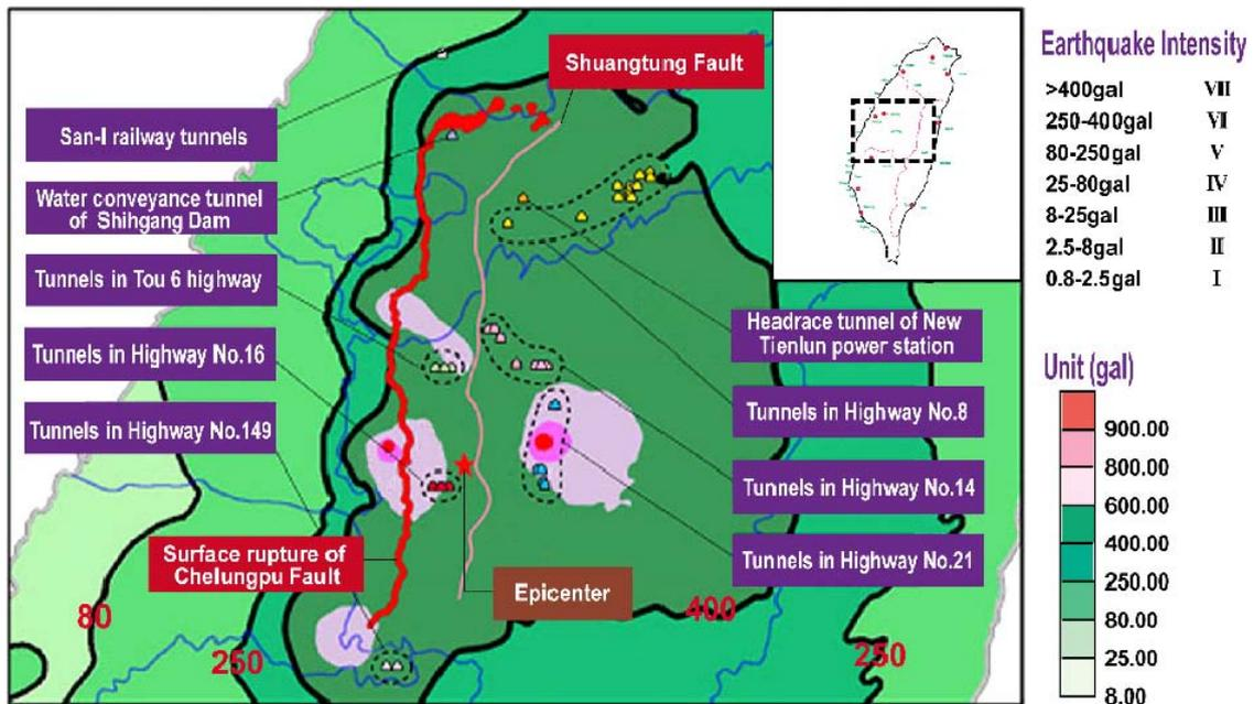
**Figure 3-3.** Intensity (Chinese Intensity Scale) and peak ground acceleration in gal (1 Galileo is  $1 \text{ cm/s}^2$ , 1000 gal is  $10 \text{ m/s}^2 \sim 1.02 \text{ g}$ ) due to the Chi-Chi earthquake (T T Wang 2001, Personal communication).
