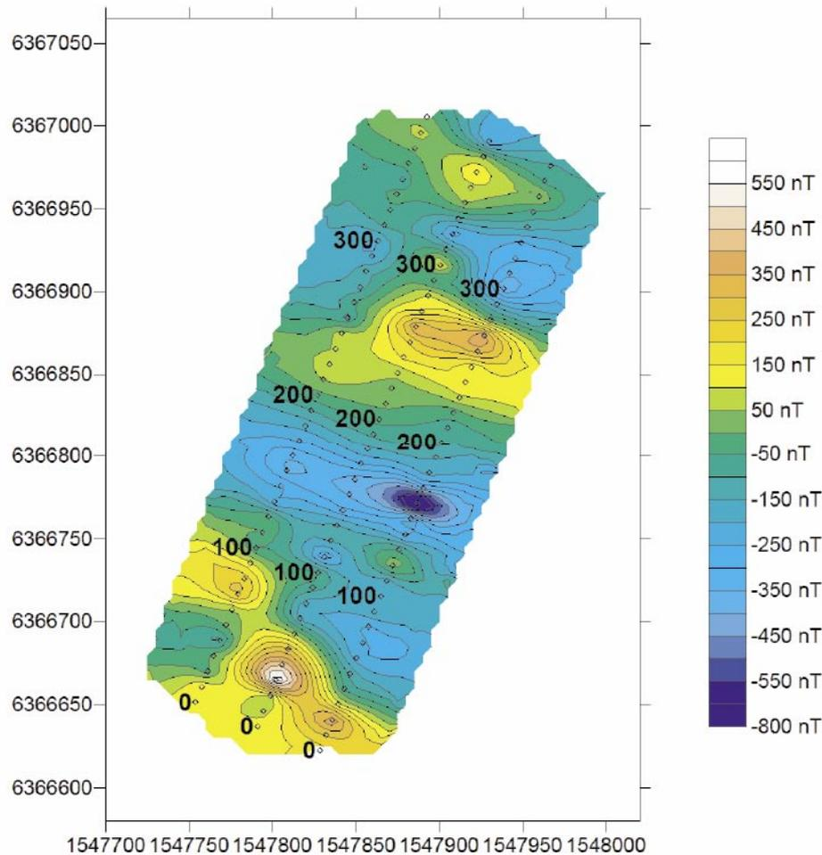
**Figure 4-10.** Contour map of ground magnetic data from profile group 4. Measurement stations are shown with symbols. Labels indicate local line-coordinates.
