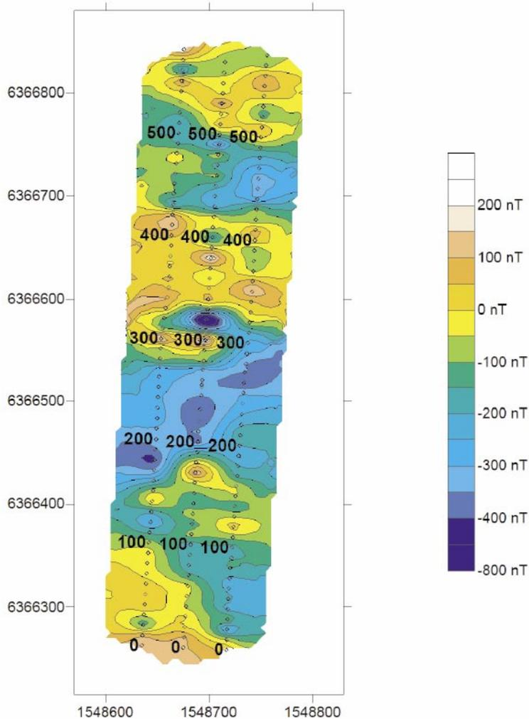
**Figure 4-13.** Contour map of ground magnetic data from profile group 5. Measurement stations are shown with symbols. Labels indicate local line-coordinates.
