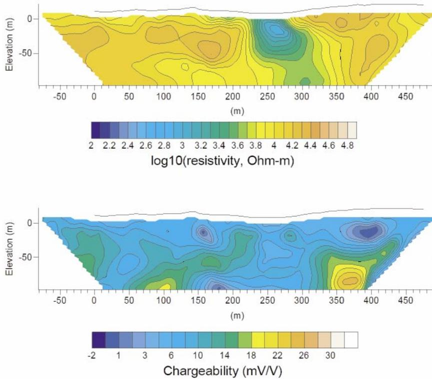
**Figure 4-17.** Inverted resistivity (top) and chargeability (bottom) sections for the central profile of the profile group 6 (LSM000281). The black lines show elevation data along the profile.
