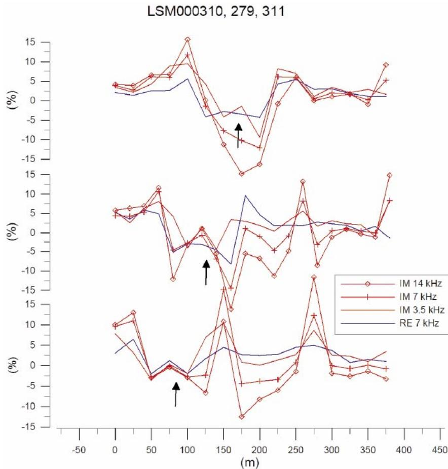
**Figure 4-12.** Slingram data for profile group 4 (LSM000310 top, LSM000279 centre, LSM000311 bottom). The arrows indicate the position of a telephone line according to the field notes.
