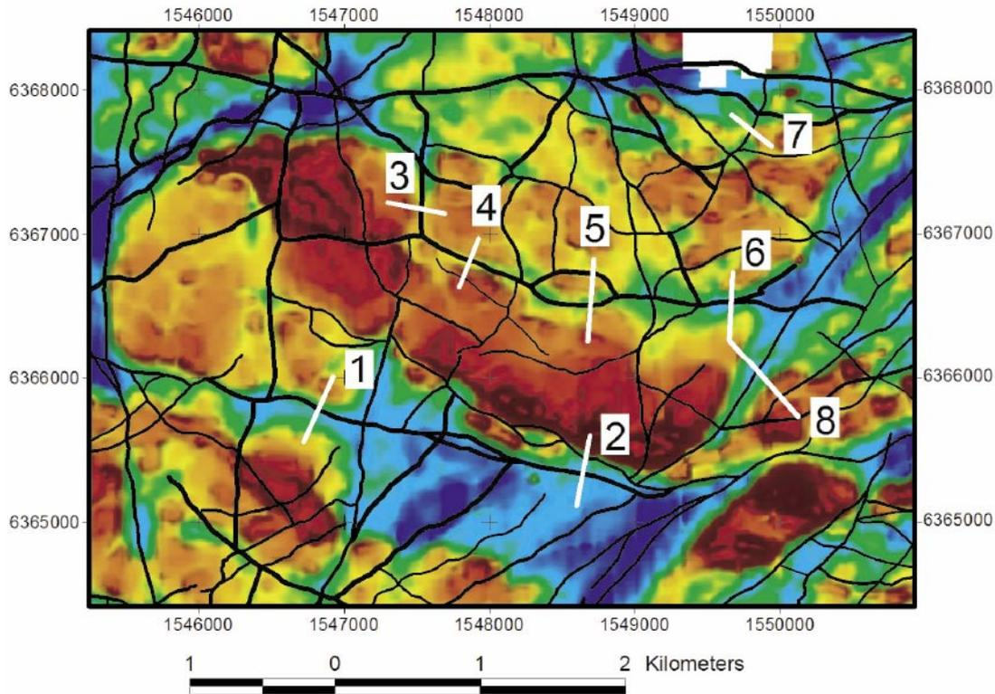
**Figure 4-2.** High-pass filtered, reduced-to-the-pole aeromagnetic map of the Laxemar area. Linked lineaments /1/ are shown in black where the line thickness is proportional to the “weight” /1/ of the lineament. The central profile of each group of profiles in the investigation is shown with a white labelled line. Label 1 to 8 correspond to LSM000276 to LSM000283.
