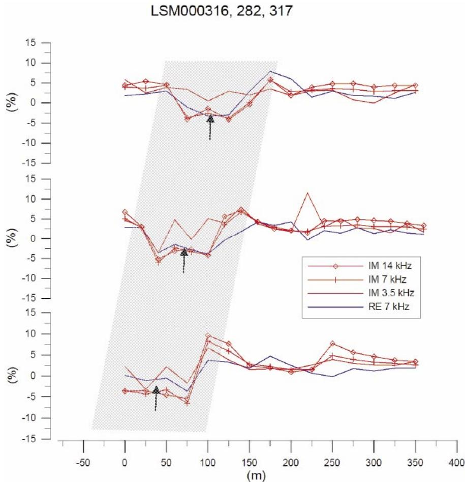
**Figure 4-21.** Slingram data for the profile group 7 (LSM000316 top, LSM000282 centre, LSM000317 bottom). The arrows indicate the position of cultural features according to the field notes. The shaded area indicates those data that have been severely affected by the cultural features. Note that the coordinate 0 starts in south-east.
