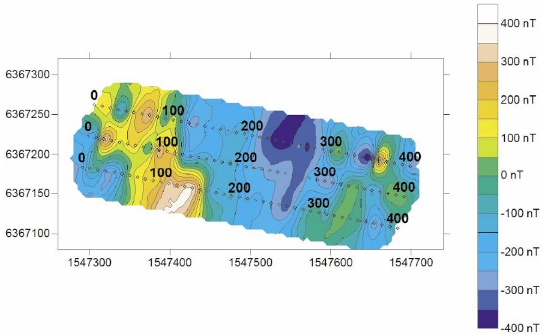
**Figure 4-7.** Contour map of ground magnetic data from profile group 3. Measurement stations are shown with symbols. Labels indicate local line-coordinates.
