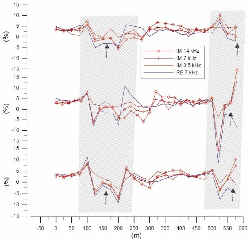
**Figure 4-15.** Slingram data for profile group 5 (LSM000312 top, LSM000280 centre, LSM000313 bottom). The arrows indicate the position of telephone lines according to the field notes. The shaded areas indicate those data that have been severely affected by the telephone lines.
