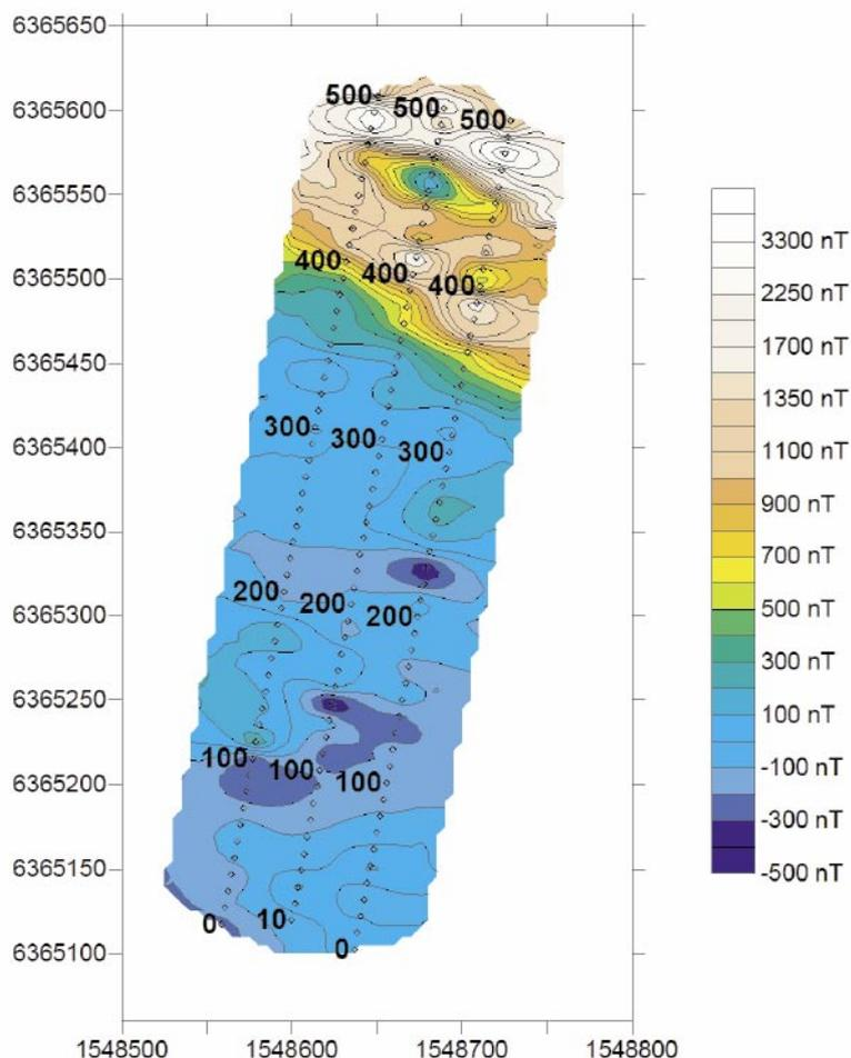
**Figure 4-5.** Contour map of ground magnetic data from profile group 2. Measurement stations are shown with symbols. Labels indicate local line-coordinates.
