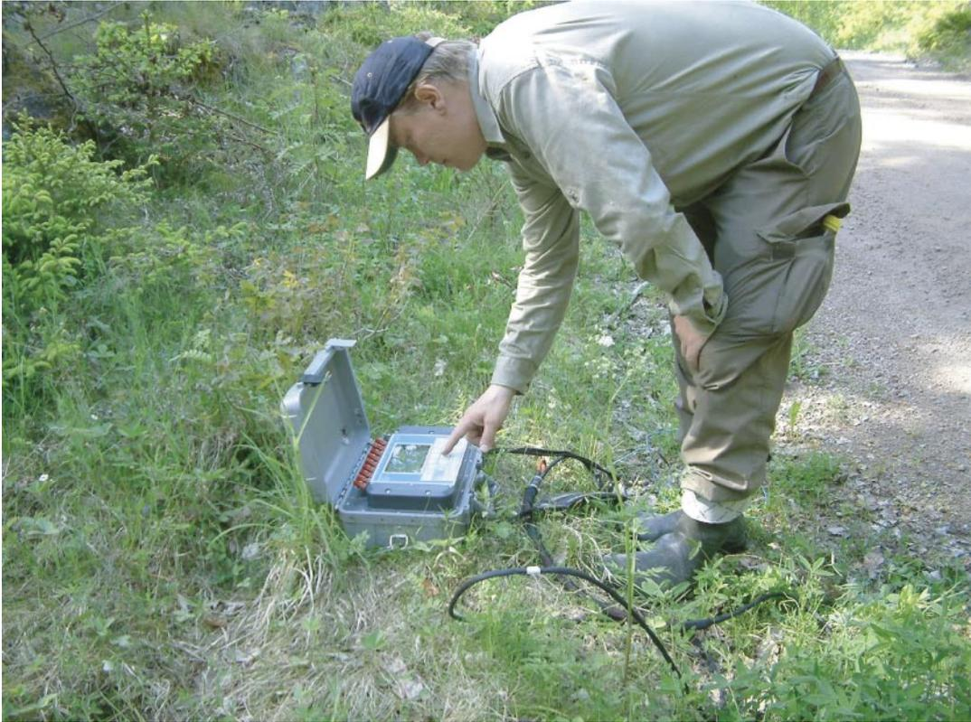
*Figure 3-1. Scintrex IPR-12 receiver for electric resistivity measurements.*
