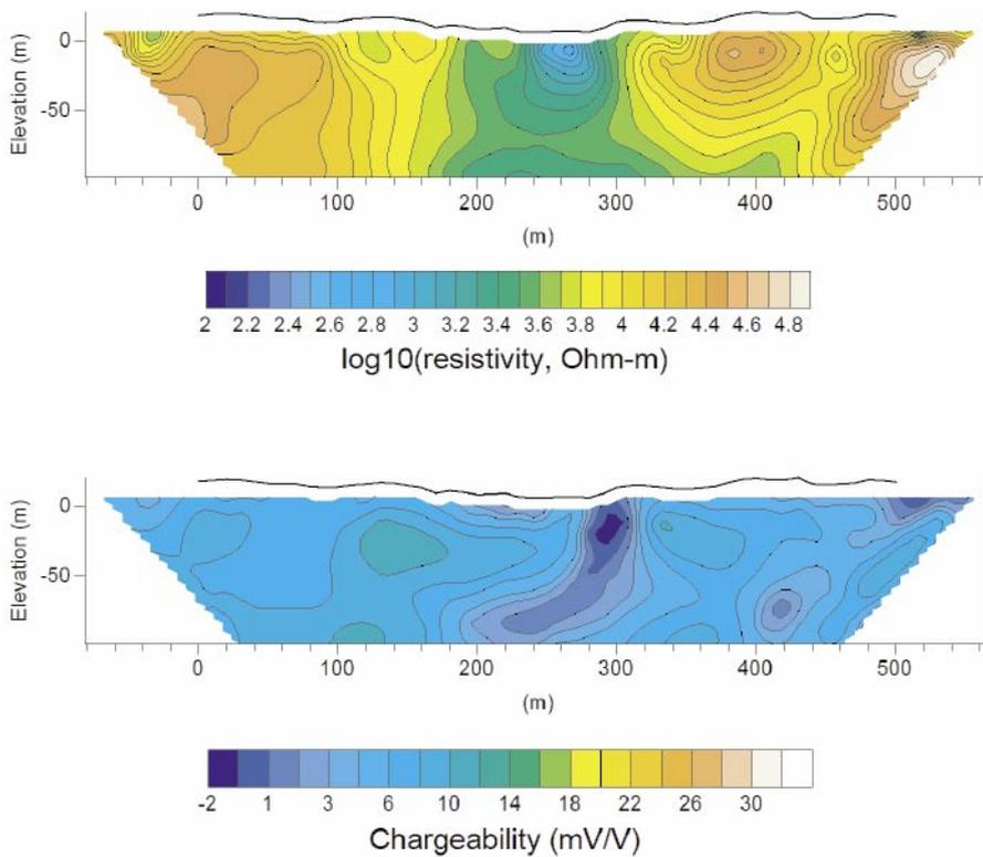
**Figure 4-4.** Inverted resistivity (top) and chargeability (bottom) sections for the central profile of profile group 1 (LSM000276). The black lines show elevation data along the profile.
