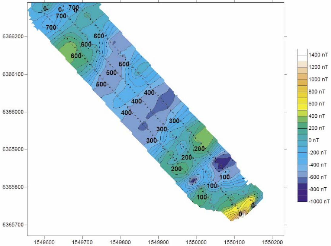
**Figure 4-22.** Contour map of ground magnetic data from the group of profiles no 8. Measurement stations are shown with symbols. Labels indicate local line-coordinates.
