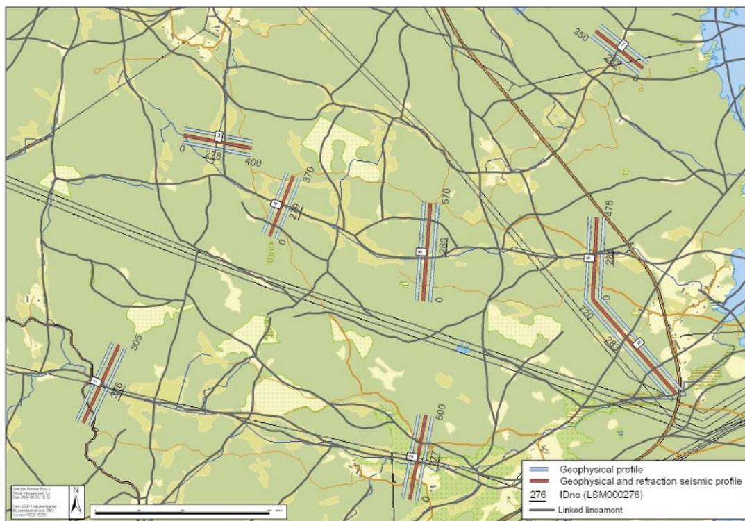
**Figure 1-1.** Location of geophysical profiles for ground geophysical measurements over interpreted lineaments in the Laxemar area /1/. Along the red profiles refraction seismic measurements were also performed /2/.
