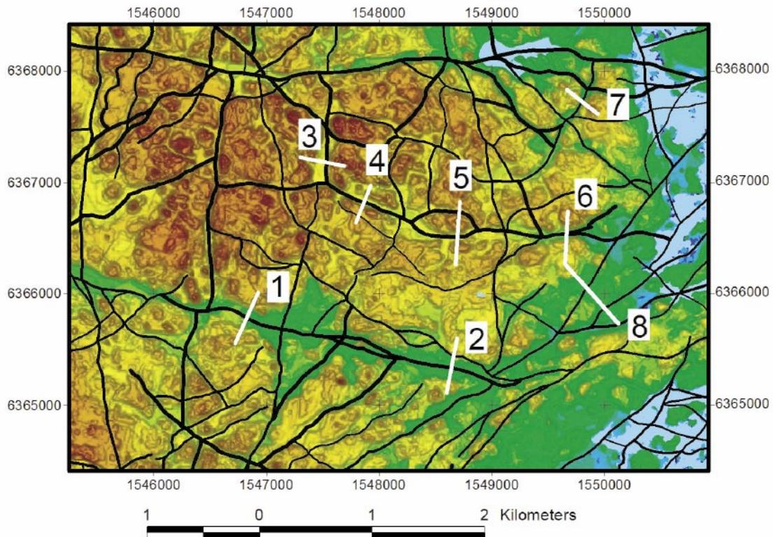
**Figure 4-1.** Shaded relief elevation map of the Laxemar area. Linked lineaments /1/ are shown in black where the line thickness is proportional to the “weight” /1/ of the lineament. The central profile of each group of profiles in the investigation is shown with a white labelled line. Label 1 to 8 correspond to LSM000276 to LSM000283.
