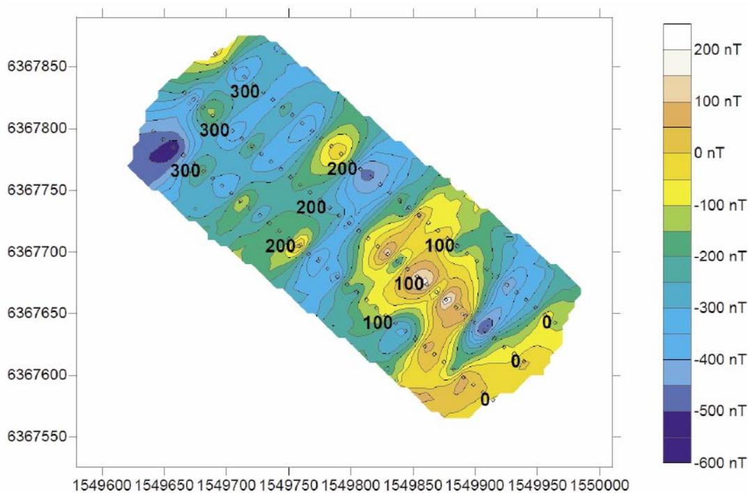
**Figure 4-19.** Contour map of ground magnetic data from the profile group 7. Measurement stations are shown with symbols. Labels indicate local line-coordinates.
