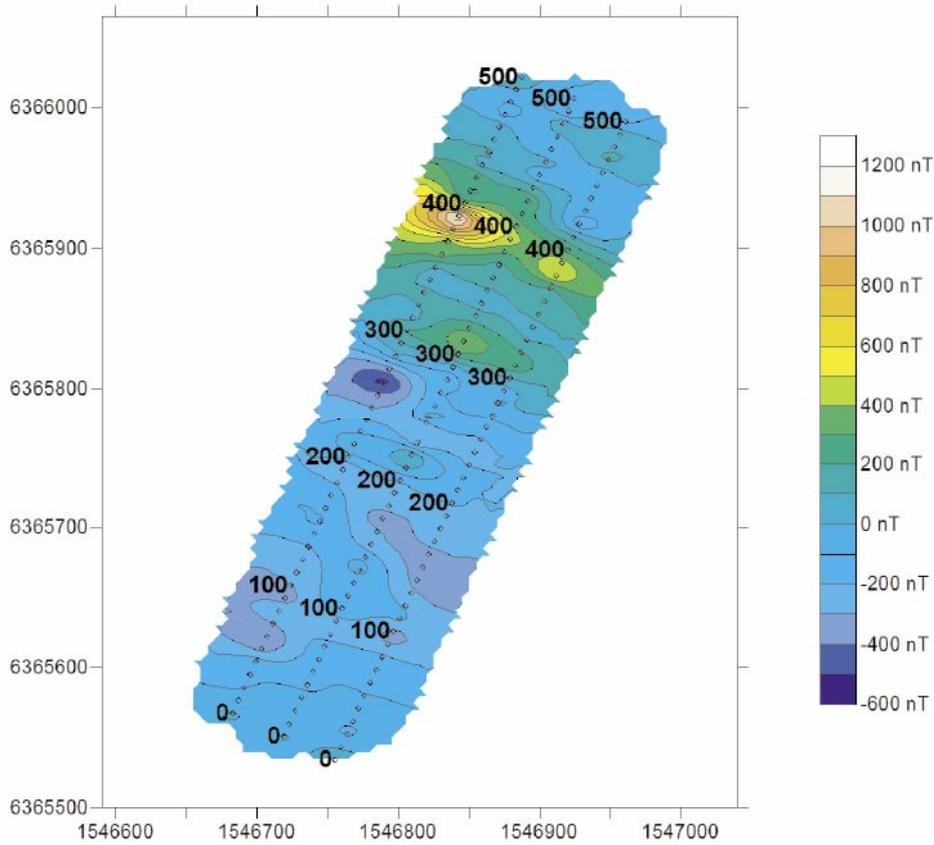
**Figure 4-3.** Contour map of ground magnetic data from profile group 1. Measurement stations are shown with symbols. Labels indicate local line-coordinates.
