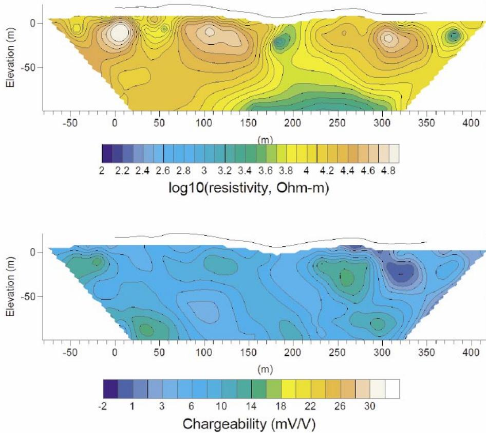
**Figure 4-20.** Inverted resistivity (top) and chargeability (bottom) sections for the central profile of the profile group 7 (LSM000282). The black lines show elevation data along the profile. Note that the coordinate 0 starts in south-east.
