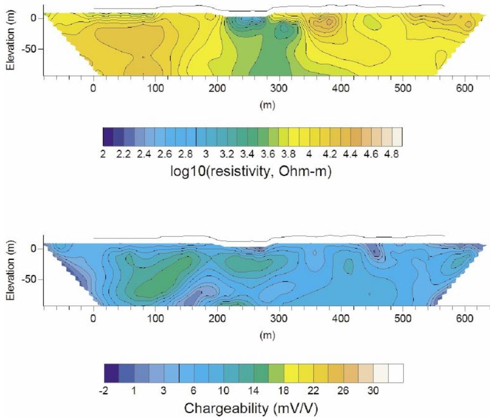
**Figure 4-14.** Inverted resistivity (top) and chargeability (bottom) sections for the central profile of profile group 5 (LSM000280). The black lines show elevation data along the profile.
