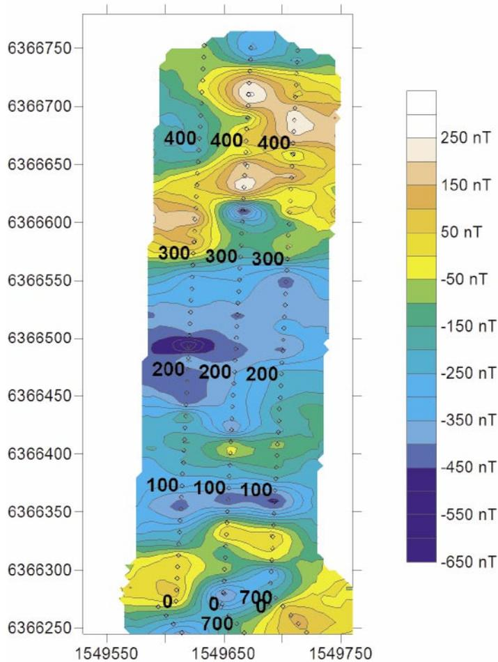
**Figure 4-16.** Contour map of ground magnetic data from the profile group 6. Measurement stations are shown with symbols. Labels indicate local line-coordinates. The northern end of group 8 can be seen in the southern part of the map.
