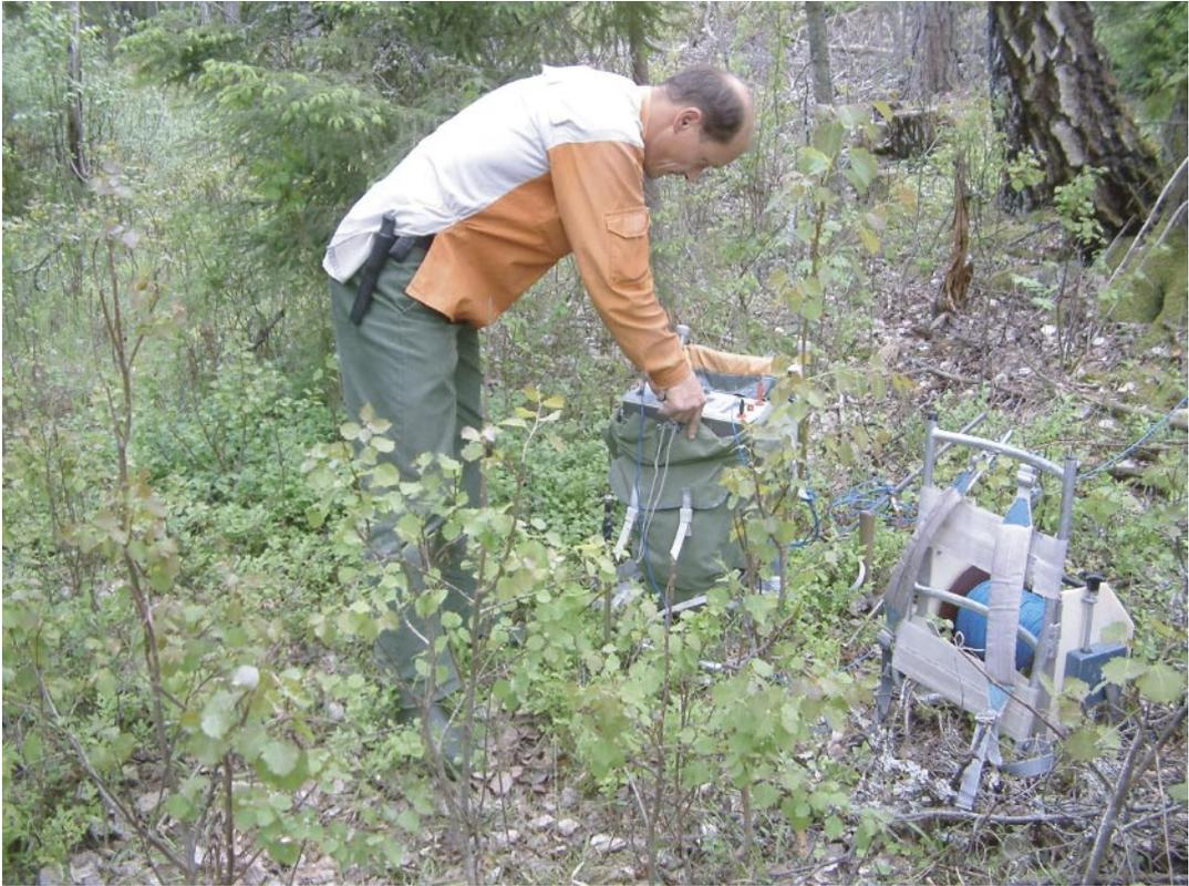
*Figure 3-2. Scintrex IPC-8 250W transmitter for electric resistivity measurements.*
