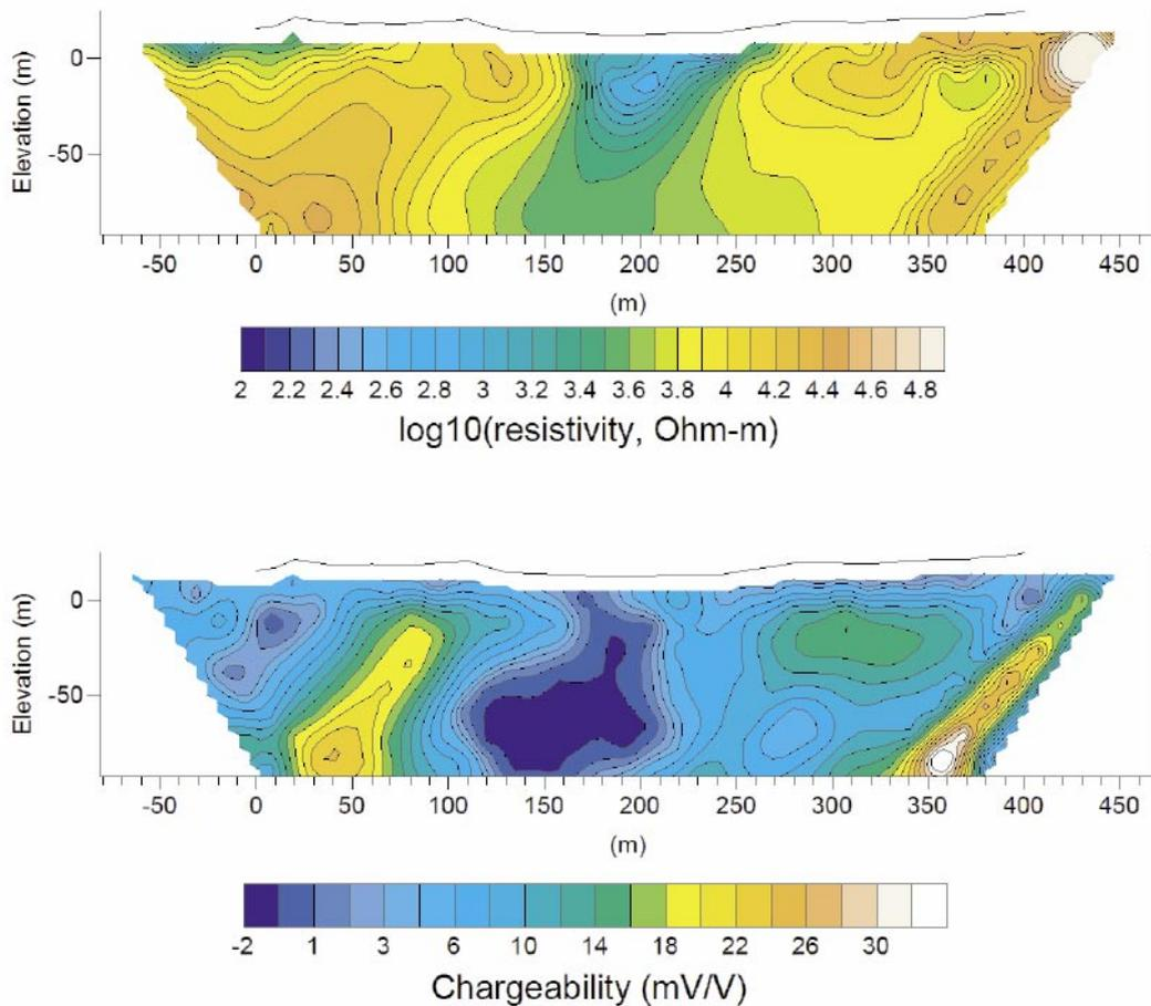
**Figure 4-8.** Inverted resistivity (top) and chargeability (bottom) sections for the central profile of profile group 3 (LSM000278). The black lines show elevation data along the profile.
