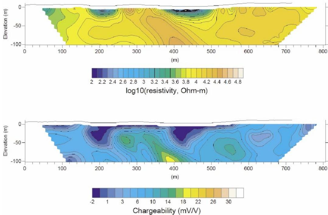
**Figure 4-23.** Inverted resistivity (top) and chargeability (bottom) sections for the central profile of the group of profiles no8 (LSM000283). The black lines show elevation data along the profile. Note that the coordinate 0 starts in south-east.
