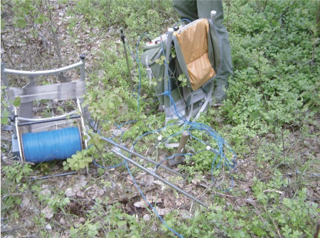
*Figure 3-3. Current electrodes for resistivity measurements.*
