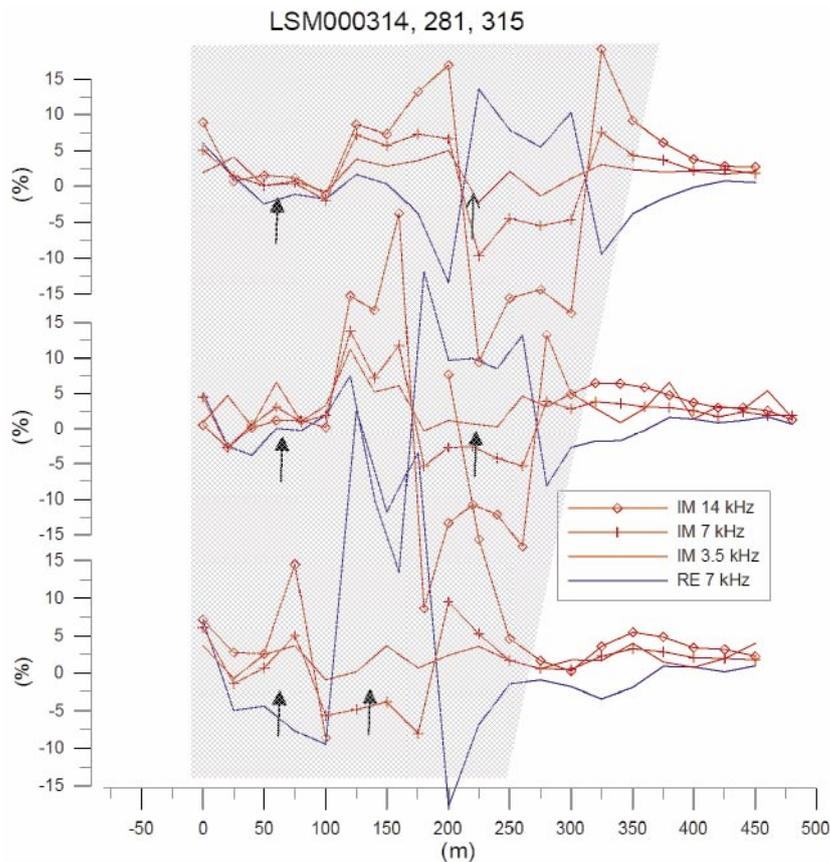
**Figure 4-18.** Slingram data for the profile group 6 (LSM000314 top, LSM000281 centre, LSM000315 bottom). The arrows indicate the position of cultural features according to the field notes. The shaded area indicates those data that have been severely affected by the cultural features.
