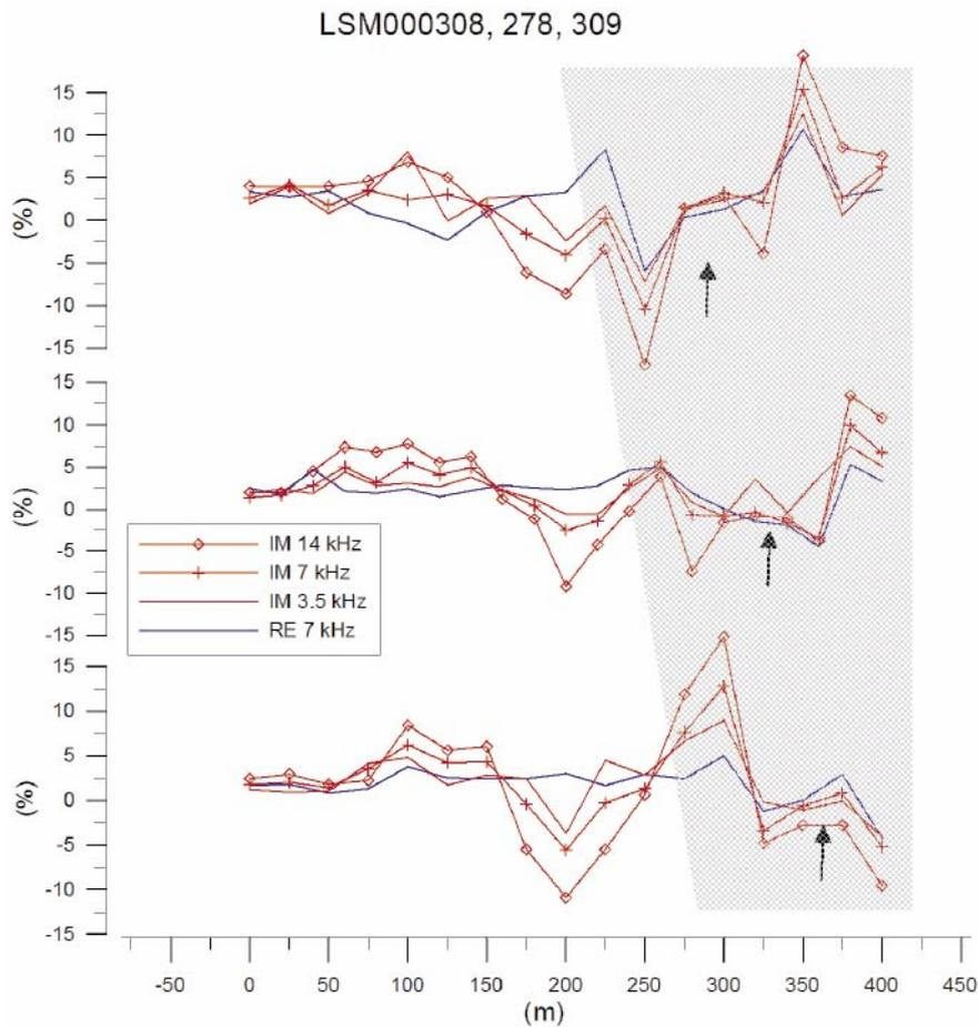
**Figure 4-9.** Slingram data for profile group 3 (LSM000308 top, LSM000278 centre, LSM000309 bottom). The arrows indicate the position of a telephone line according to the field notes. The shaded area indicates those data that have been severely affected by the telephone line.
