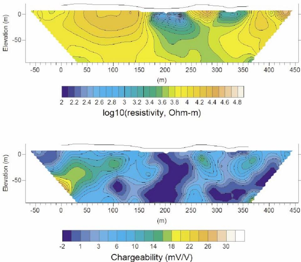
**Figure 4-11.** Inverted resistivity (top) and chargeability (bottom) sections for the central profile of profile group 4 (LSM000279). The black lines show elevation data along the profile.
