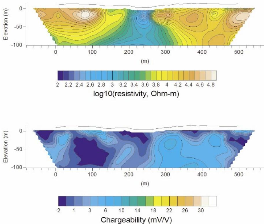
**Figure 4-6.** Inverted resistivity (top) and chargeability (bottom) sections for the central profile of profile group 2 (LSM000277). The black lines show elevation data along the profile.
