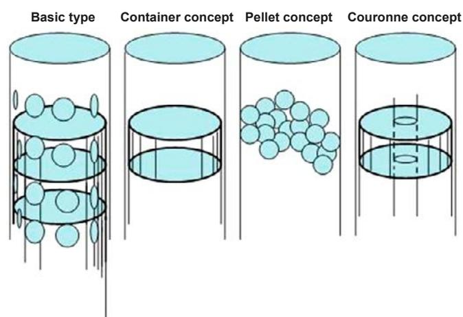
**Figure 2-3.** Clay plug concepts. Left: “Basic” type with dense clay blocks confined in perforated copper tubes. Second left: “Container” plug with blocks in a cylinder attached to drilling rods and released in the desired position. Third left: Dense, clay pellets poured into the hole. Right: “Couronne” plug with rings of dense clay around jointed copper rods (Pusch and Ramqvist 2006a).
