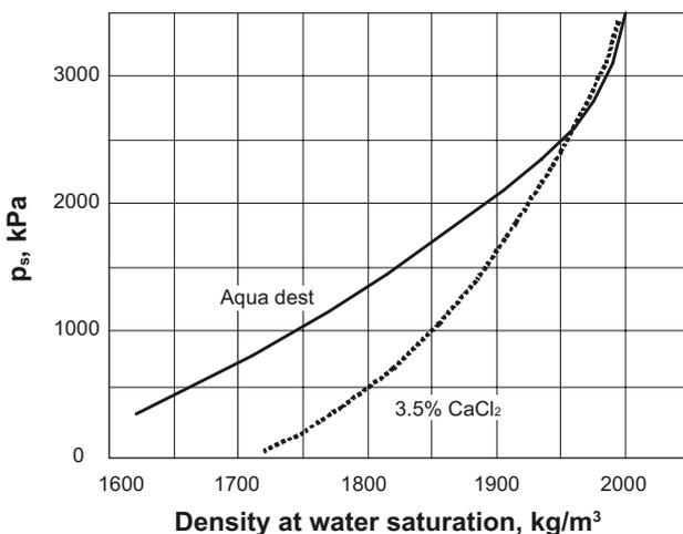
**Figure 5-6.** Approximate relationship between density at water saturation and swelling pressure of smectite-rich clay (Pusch and Yong 2006).
