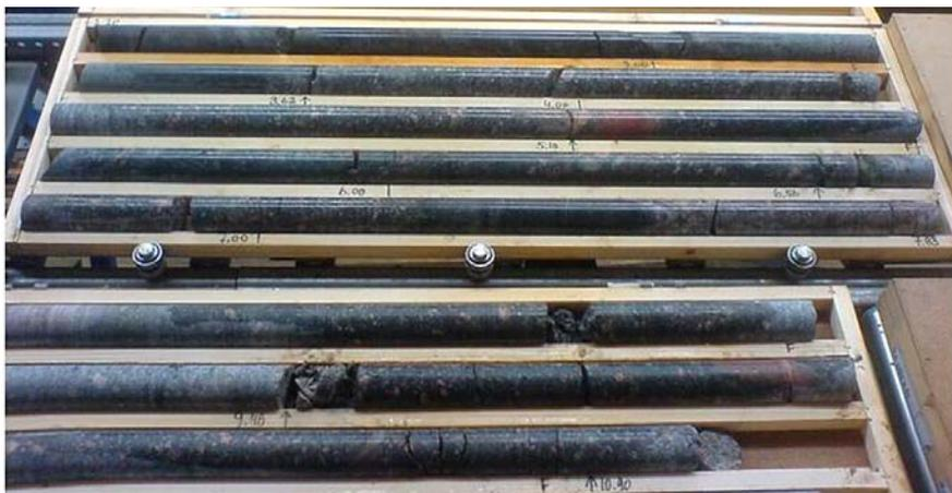
Figure 2-16. Borehole KA3386A01. Small fracture zones or fracture assemblies can be seen at 8.70 and 9.50 m borehole length.
