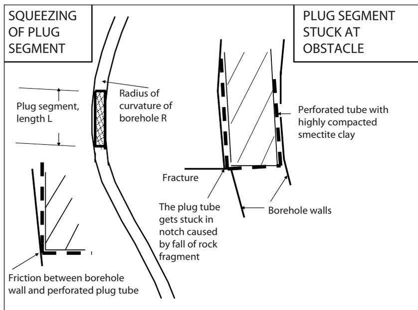
*Figure 2-5. The length of borehole plug must be limited for avoiding problems at placement.*
