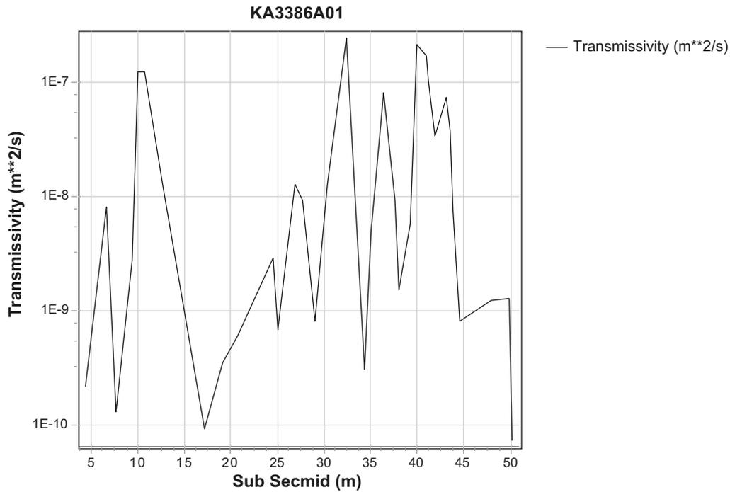
Figure 2-15. Borehole KA3386A01 – hydraulic transmissivity along the borehole.
