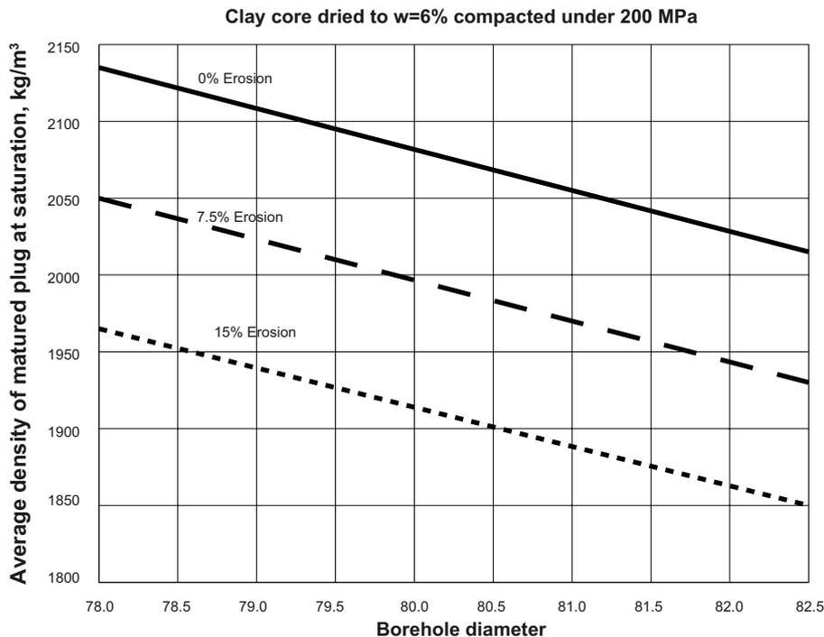
**Figure 2-10.** Theoretically derived relation between borehole diameter and ultimate density at water saturation of “Basic” type clay plugs for three erosion scenarios (SKB IPR-06-28).
