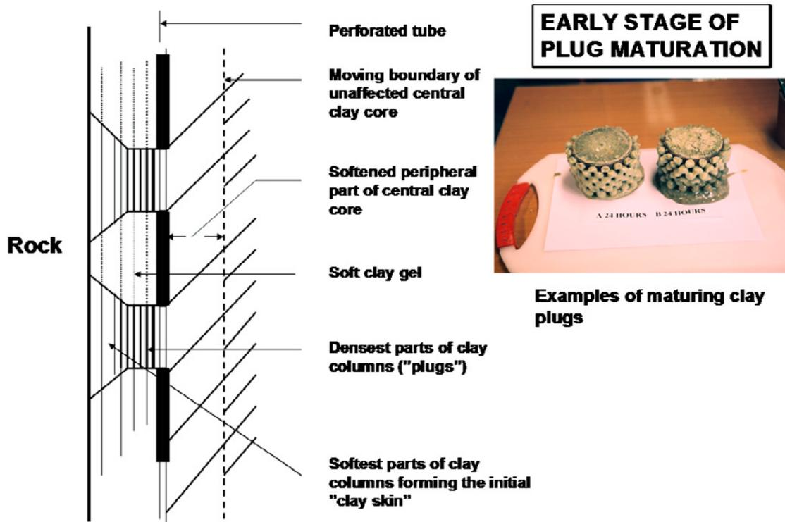
Figure 2-7. Schematic view and photos of the earliest stage of a maturing clay plug.
