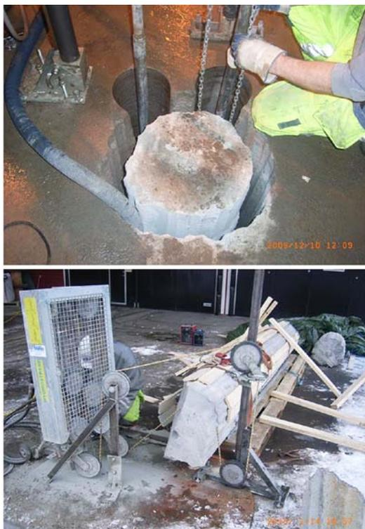
**Figure 5-3.** The rock column containing the plugged borehole KA 1621 G02. Upper: Slot drilling. Lower: Wire sawing to produce 100 mm thick discs.
