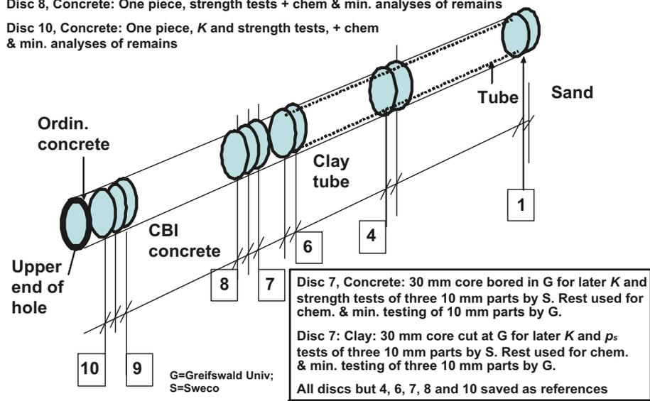
Figure 5-4. Schematic view of the plugs in the hole. Disc 1 served as reference. Discs 2,3 and 5 were saved for information. The other ones were analyzed.
