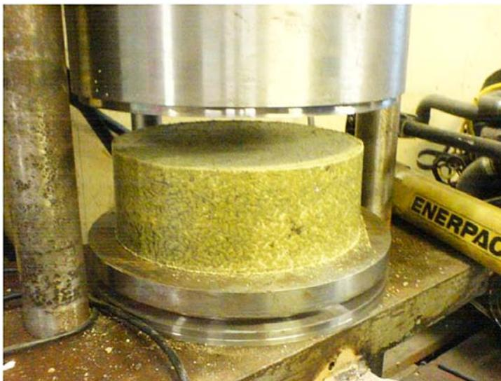
**Figure 4-4. Compaction of blocks. CEBOGEL bentonite block with 285 mm diameter and 100 mm height. Density 2,060 kg/m<sup>3</sup>.**
