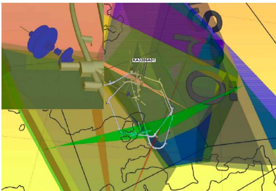
**Figure 2-13.** Detailed view of the Äspö structure model, the Äspö tunnel and borehole KA3386A01. It demonstrates that the borehole does not penetrate any of the major fracture zones (Bockgård 2011).
