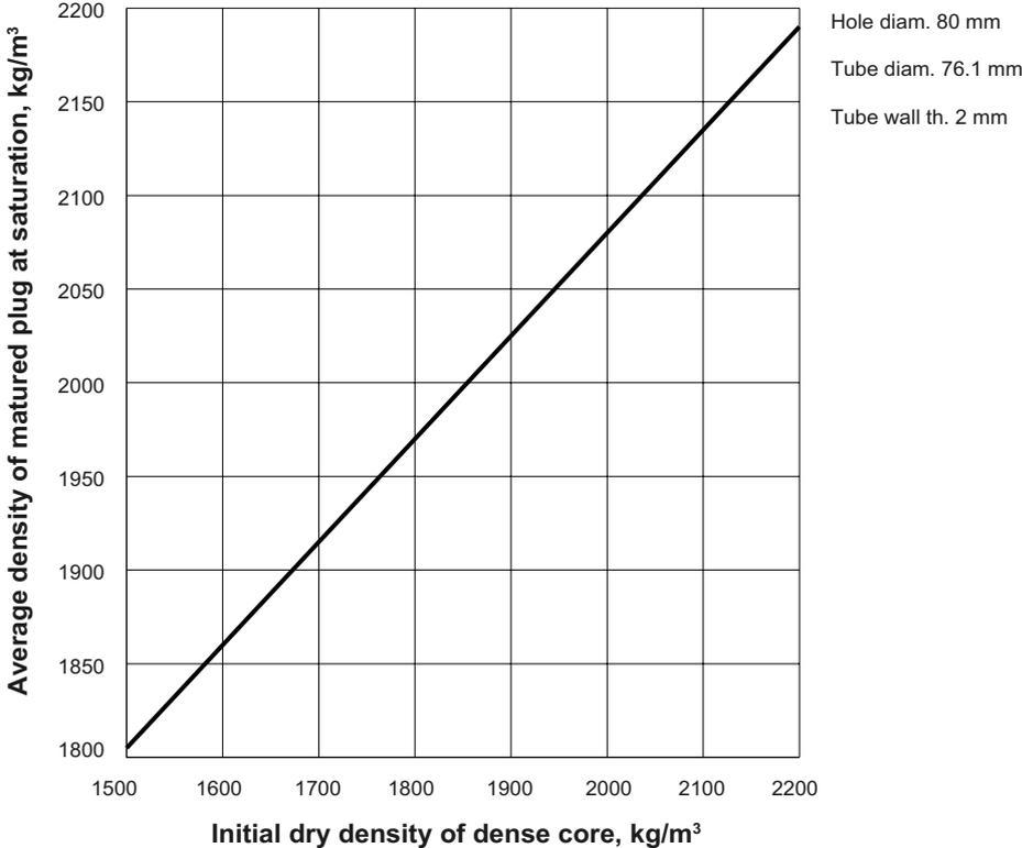
**Figure 2-9.** Relation between initial dry density of the dense core in the tube and the theoretical average density at water saturation of the entire clay plug.
