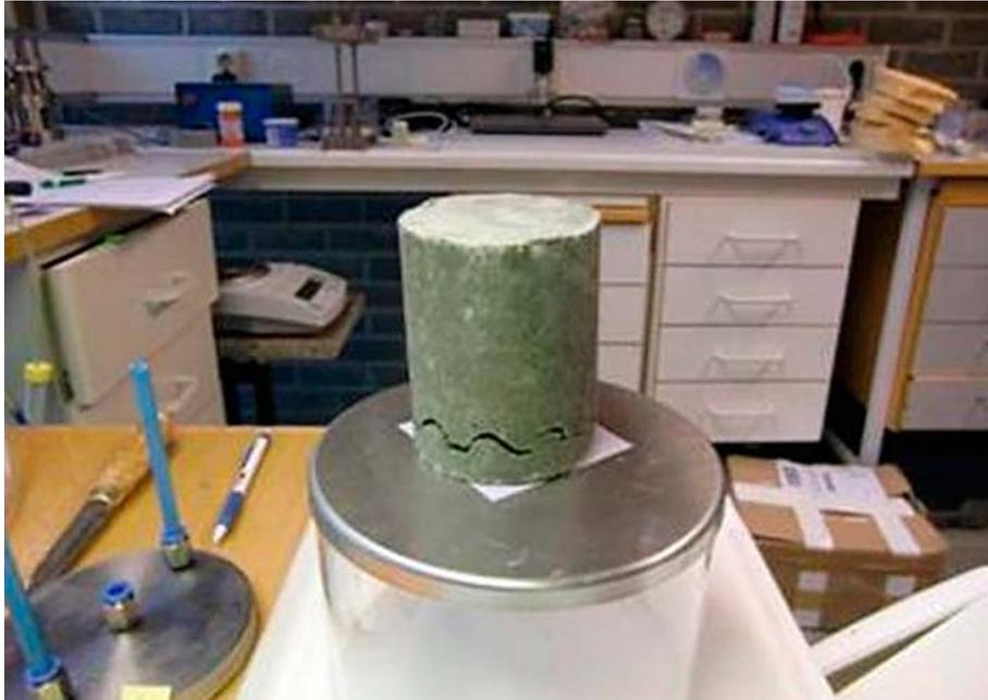
*Figure 5-7. The clay plug (turned upside down) released from Disc 6. The wavy fracture was caused at the disassembling and occurred at the contact of a tube-confined part and one where only clay blocks had been placed in the hole.*
