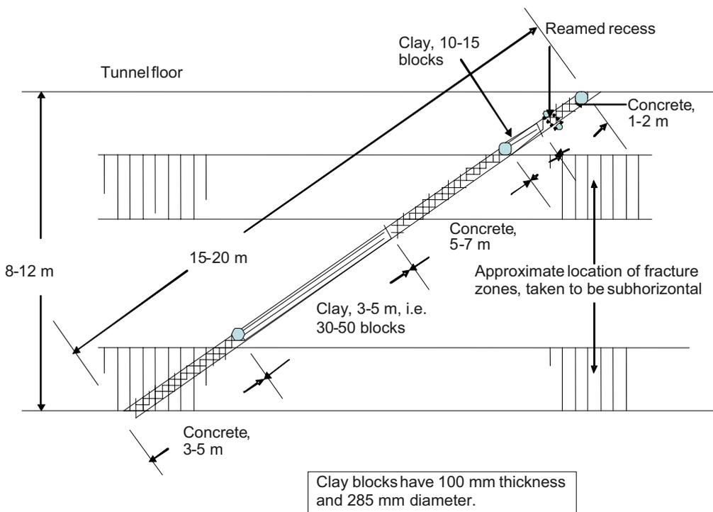
Figure 4-3. The selected sealing principle using on-site cast CBI concrete and prefabricated clay plugs of “Basic” type.
