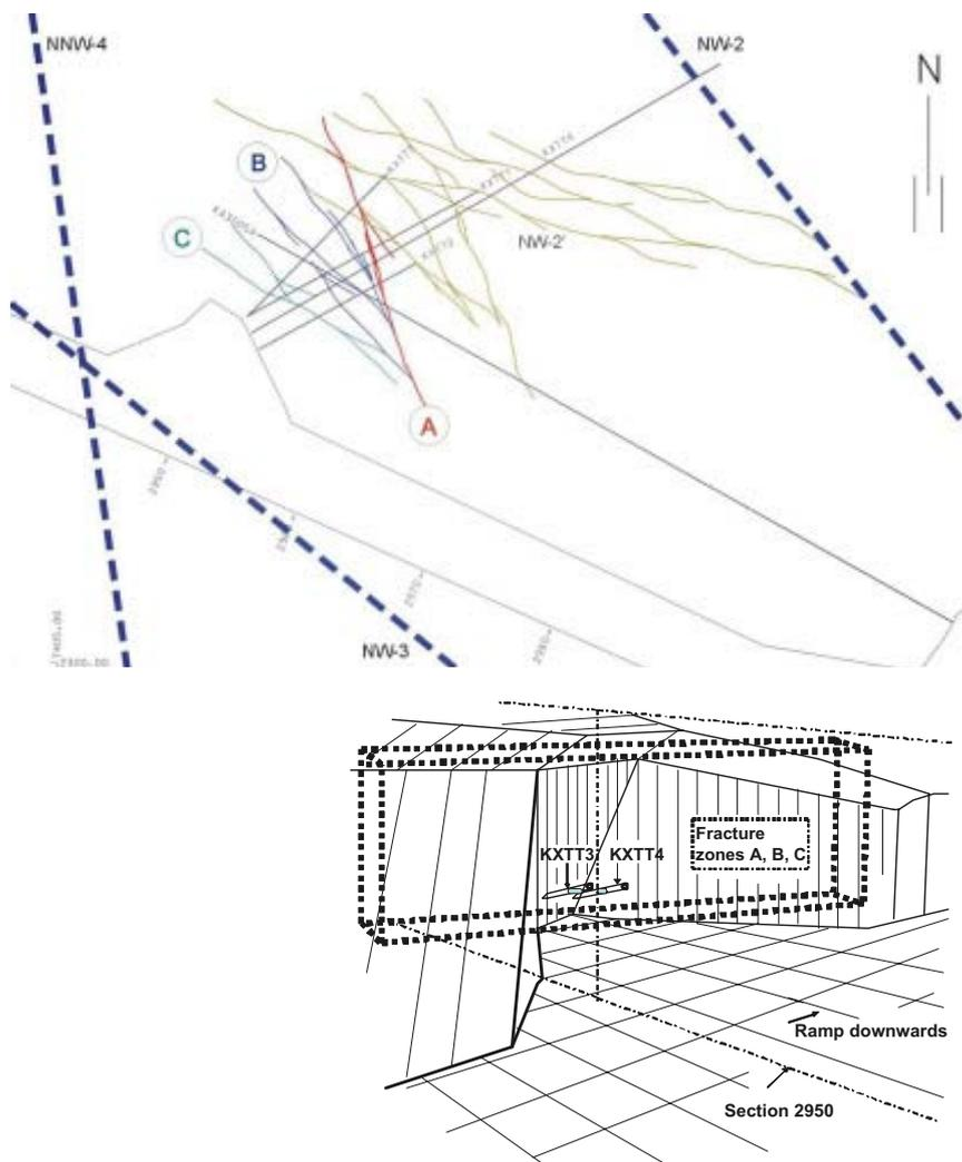
*Figure 4-1. Upper: Horizontal section at Z = -400 showing structural model based on identified conductive geological structures in the TRUE-1 volume (Winberg et al. 2000). Lower: Perspective view.*
