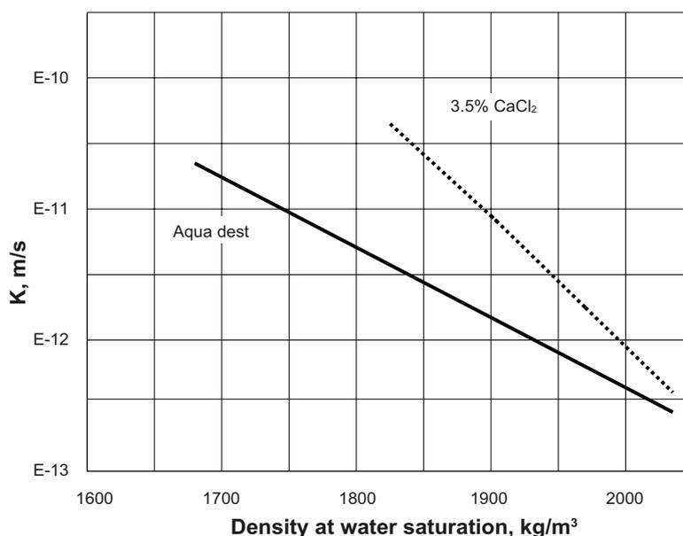
Figure 2-8. Approximate relationship between density and hydraulic conductivity of smectite-rich clay. (Pusch and Yong 2006)
