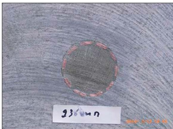
Figure 5-5. The sectioned clay plug with the perforated copper tube embedded in dense clay.
