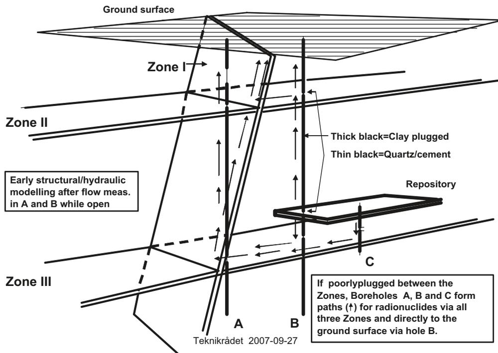
Figure 3-2. Short-circuiting of fracture zones by open or inadequately sealed or leaching boreholes.
