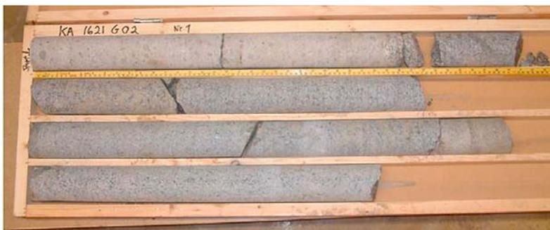
**Figure 5-2.** Hole KA 1621 G02. The core from the 80 mm-diameter hole representing the uppermost 3 metres of the hole has at least 5 water-bearing fractures.
