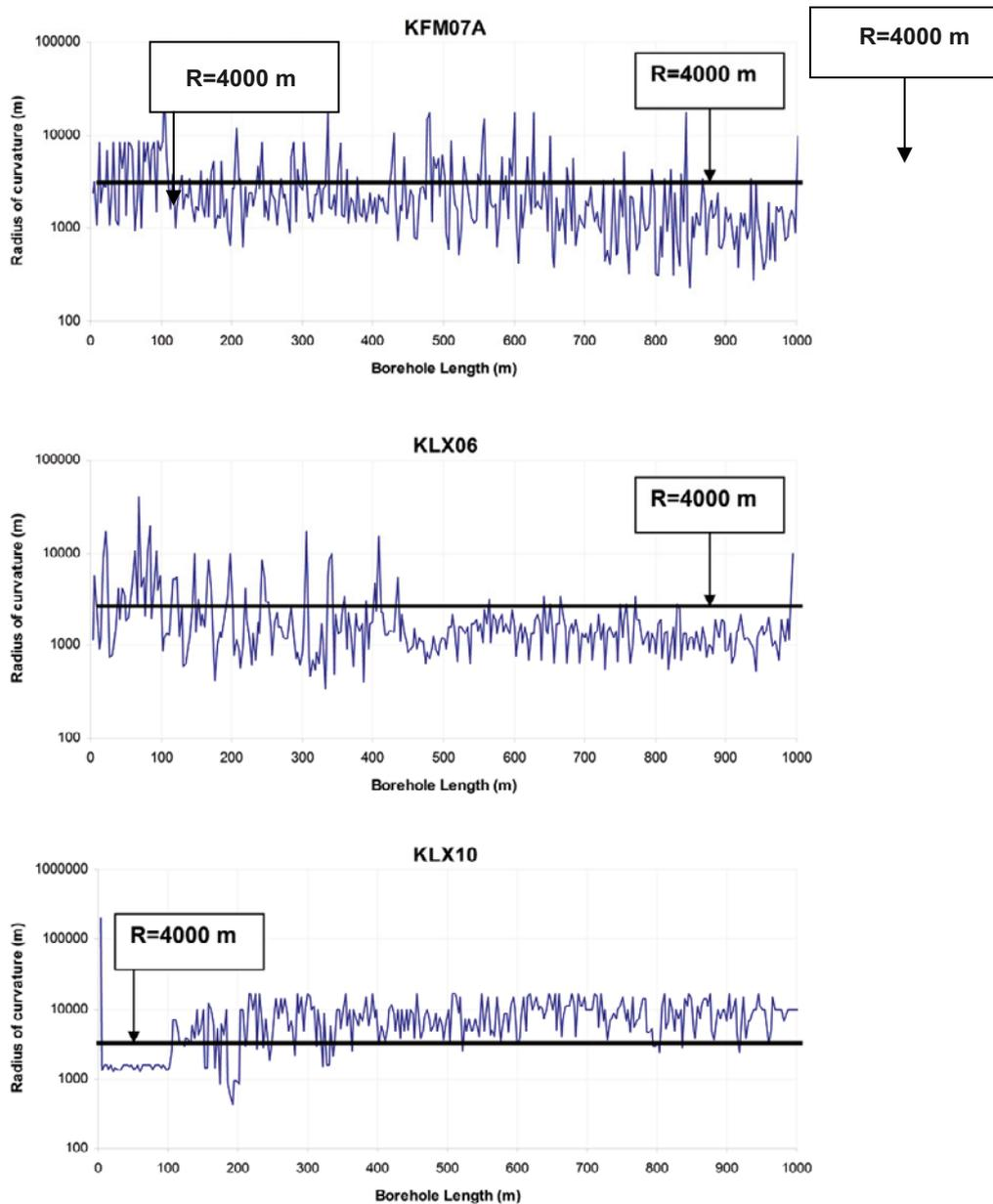
**Figure 2-6.** Examples of rather small radii of curvature (upper two diagrams) and rather large radii (lowest) (Nilsson and Nissen 2007).
