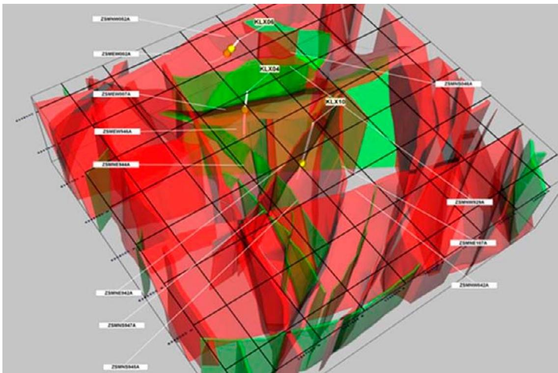
**Figure 2-2.** Perspective view of Laxemar with the three boreholes KLX04, KLX06 and KXL10. The boreholes intersect a number of steeply oriented fracture zones: 19 zones by KLX04, 4 zones by KLX06, and 10 zones by KXL10. The spheres indicate the upper ends of the holes.
