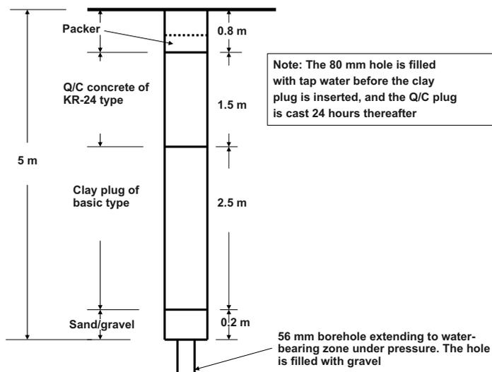
**Figure 5-1.** Schematic view of the two 5 m boreholes (actual depths 6.00 and 5.90 m) with 80 mm diameter for testing of the interaction of quartz/cement and clay. The upper part of the hole was filled with CBI concrete over a clay plug of “Basic” type resting on sand gravel.
