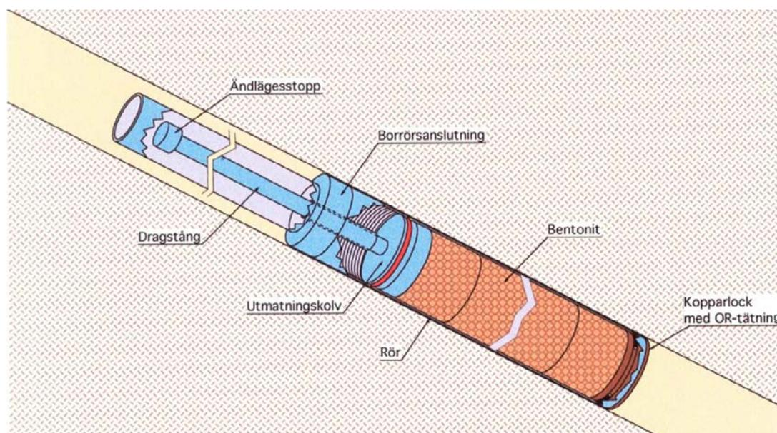
**Figure 7-1.** The “Container” plug equipment placed in a steel tube that is brought into the hole. The brownish clay (or concrete) is contained between a piston (“utmatningskolv”) by which it can be extruded to the desired position. At the outer end of the tube there is tight lid of copper (“kopparlock med OR-tätning”) that moves down with the clay and stays in the hole.
