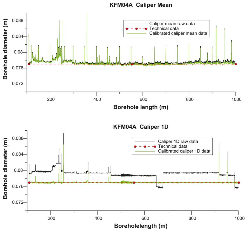
**Figure 2-4.** Example of calibrated caliper measurements in a 1,000 m long, steep borehole. The upper diagram illustrates results from one arm mechanical caliper measurements, whereas the lower diagram illustrates diameter data from acoustic televiewer (Nilsson and Nissen 2007). Thin “spikes” in the diagrams represent single fractures or reference grooves milled into the borehole wall to serve as a means for length calibration.
