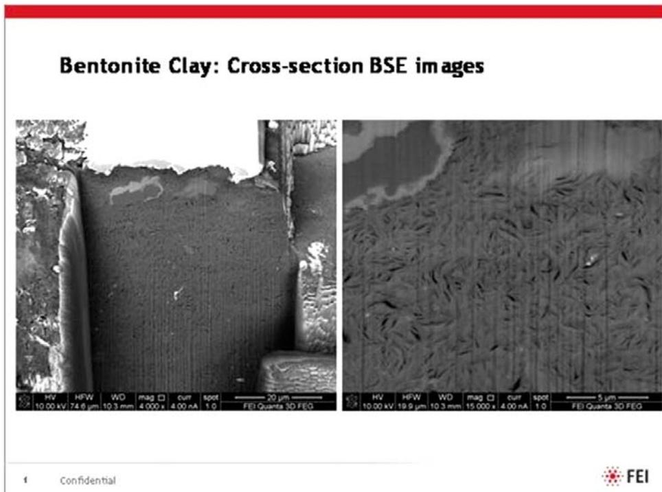
*Figure 5-8. Example of the appearance of the microstructural organization of clay at 0–10 mm distance from the concrete in Disc 7 (Laurence Warr, Greifswald University).*
