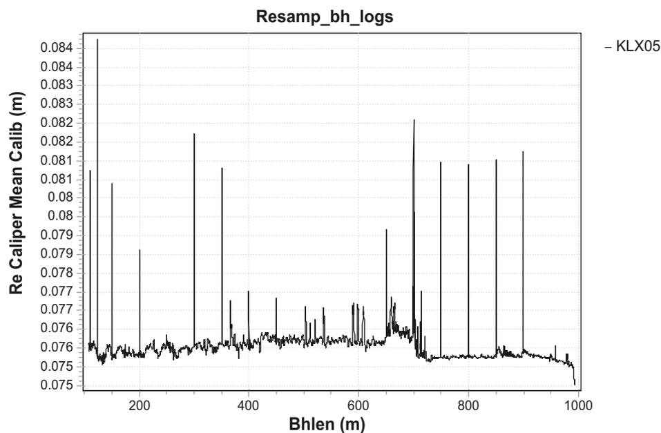
**Figure 2-11. Example of diameter variation in Borehole KLX05.**
