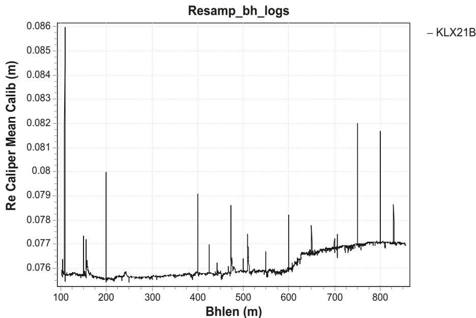
**Figure 2-12.** Example of diameter variation in Borehole KLX21B.
