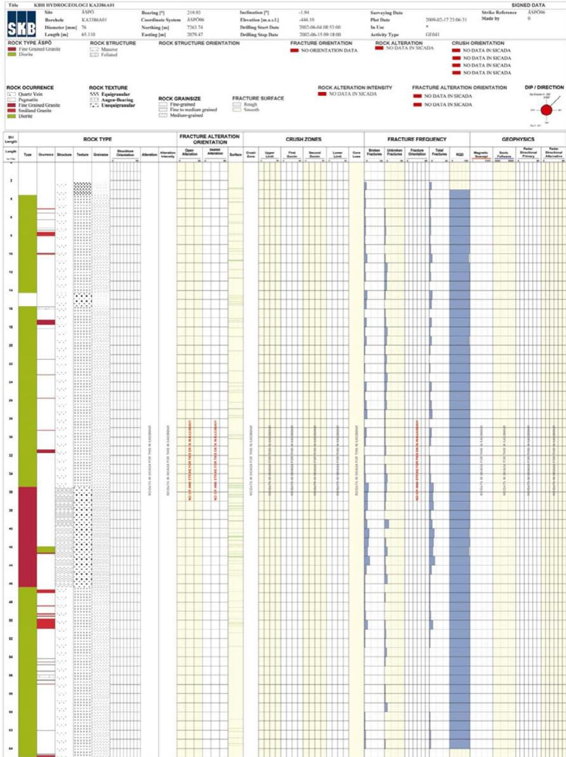
Figure 2-14. Borehole KA3386A01. WellCad-plot showing rock type and fracture distribution.
