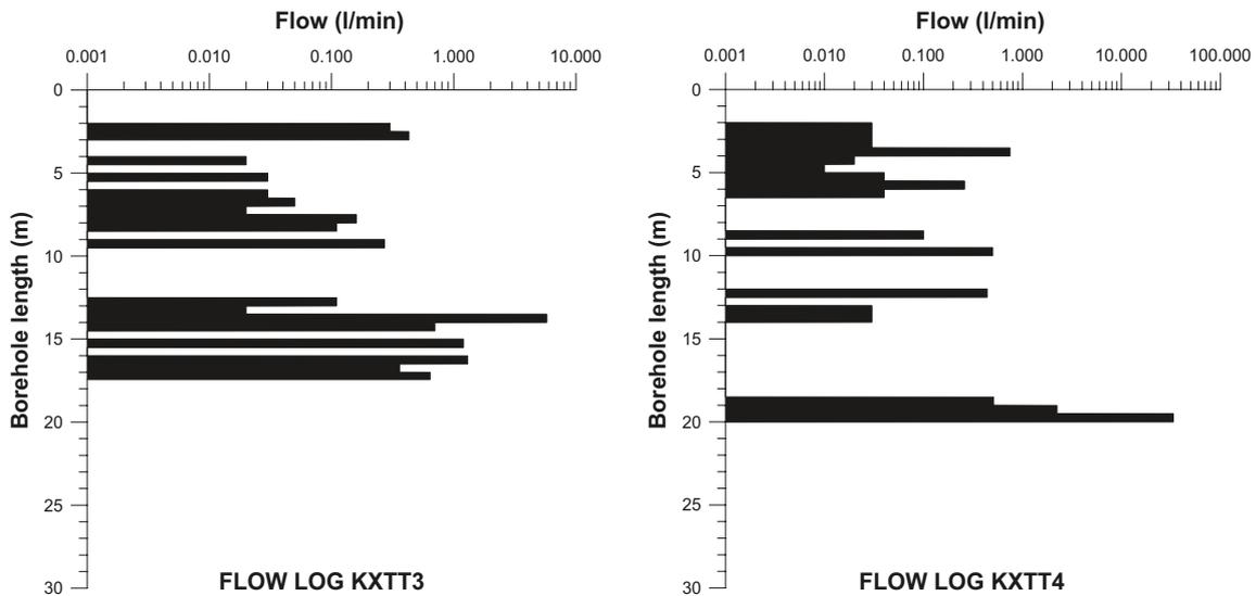
Figure 4-2. Measured inflows in the two boreholes KXTT3 and KXTT4 (Winberg et al. 2000).
