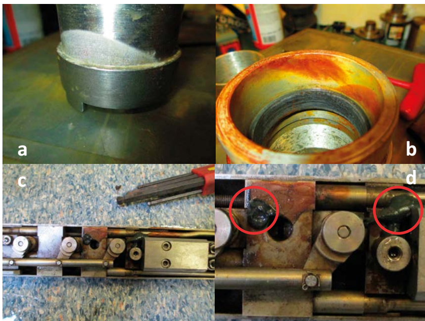
Figure 3-13. Corrosion on downhole equipment after use in borehole KFM08D. a) Precipitates on connection to the umbilical hose b) Surface corrosion on the screw nut to the same connection c) Corrosion on the in situ sampling device placed in the sampled borehole section d) enlargement of c) showing the black material coating parts of the sampling device.
