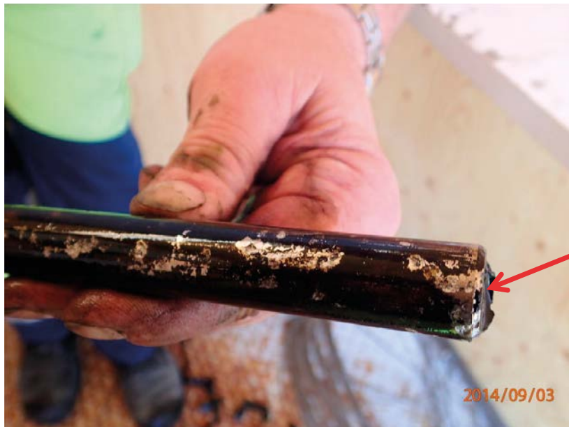
Figure 3-11. Corrosion on sinker in borehole KFM11A. The highest corrosion rate appears on the tip (red arrow).
