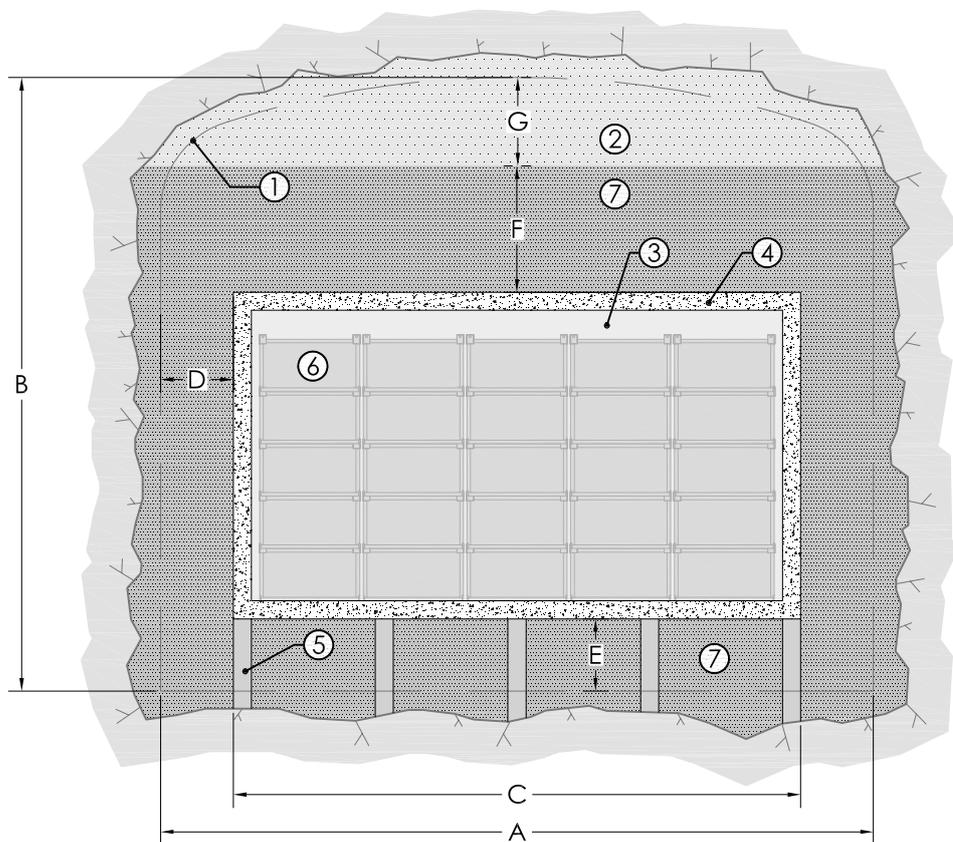
**Figure 2-4.** Schematic cross-sectional layout of BHA from Elfving et al. (2013). Legend: (1) Theoretical tunnel contour; (2) Bentonite pellets, (3) Grout, (4) Concrete structure (0.5 m), (5) Granite pillars, (6) Waste packages, (7) Bentonite blocks. Approximate dimensions:  $A = 20.6$  m,  $B = 18.5$  m,  $C = 16$  m,  $D = 2.3$  m,  $E = 2.4$  m,  $F = 4$  m,  $G = 3.7$  m. The figure is a copy of Figure 5-1 in the *Initial state report*.
