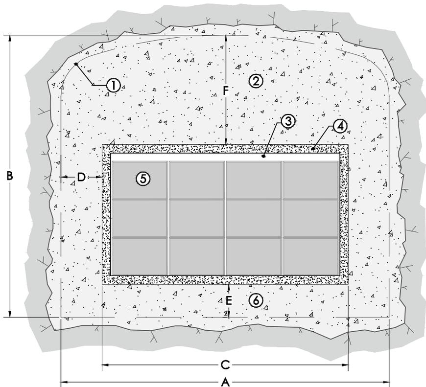
**Figure 2-3.** Schematic cross-sectional layout of BHK from Elfving et al. (2013). Legend: (1) Theoretical tunnel contour, (2) Concrete backfill, (3) Grout, (4) Reinforced concrete structure (0.5 m), (5) Steel tanks, (6) Concrete. Approximate dimensions: A = 20.6 m, B = 19.6 m, C = 15 m, D = 2.8 m, E = 2.4 m, F = 8.8 m. The figure is a copy of Figure 4-1 in the **Initial state report**.
