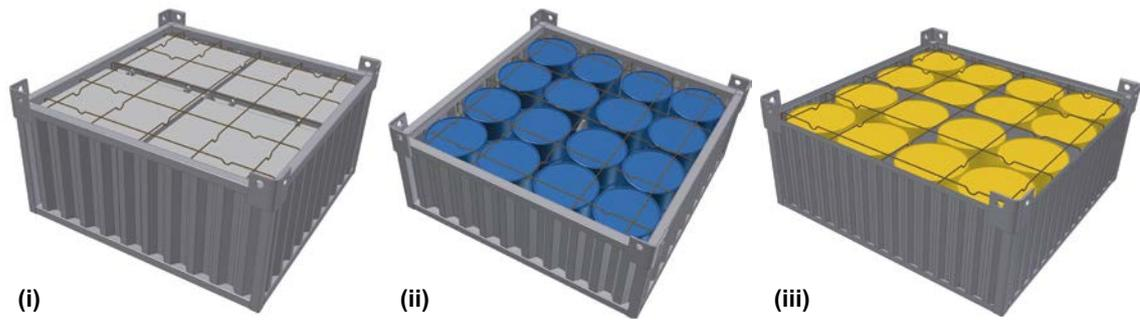
**Figure 2-2.** 3D-view of waste packaging disposed in BHA, loaded with (i) standard moulds, (ii) standard 200-litre drums, and (iii) 280-litre protection drums. Reinforcement bars that will stabilise the future grout on top of the moulds are also shown. The figure is a copy of Figures 3-3 (i), 3-5 (ii) and 3-7 (iii) in the *Initial state report*.
