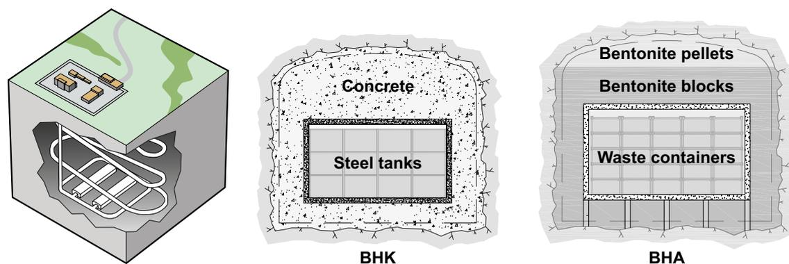
**Figure 1-2.** Preliminary facility layout and the proposed repository concept for SFL (left), one waste vault for metallic waste from the nuclear power plants (BHK, centre) and one waste vault for waste from Studsvik Nuclear AB, Cyclife Sweden AB and AB SVAFO (BHA, right).
