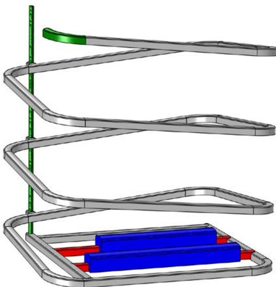
**Figure 2-5.** Schematic illustration of the closure components in SFL: backfill of waste vaults (blue), sealing (red), backfill of access tunnels (grey) and closure plugs (green). The figure is a copy of Figure 6-1 in the **Initial state report**.
