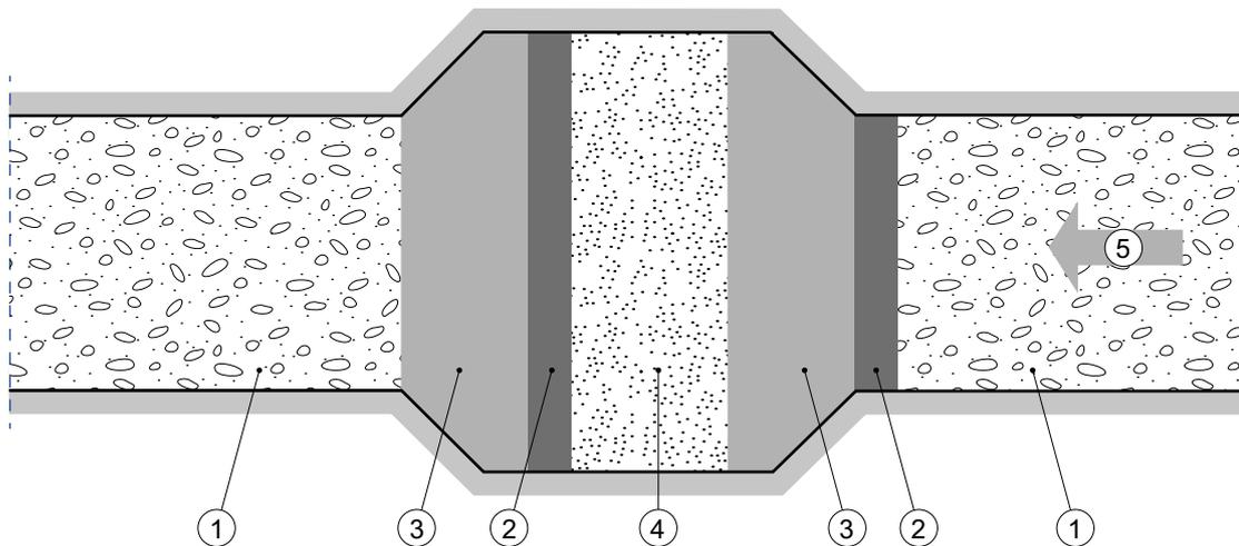
**Figure 2-6.** Schematic design of a sealing plug in the repository main tunnel (Luterkort et al. 2014).
