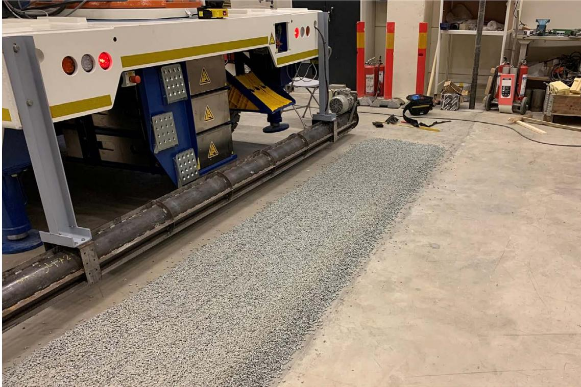
*Figure 4-4. Equipment for installation of pellets on the tunnel floor.*
