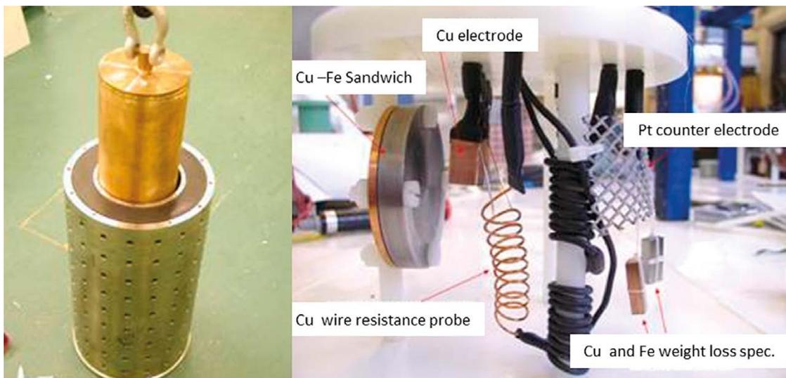
**Figure 3-28.** Model canister being lowered into support cage containing bentonite pellets in annulus (left). Test electrodes inside support cage around model canister experiments (right).
