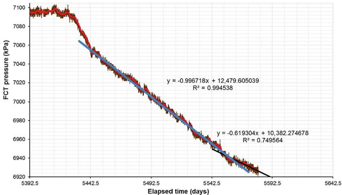
**Figure 3-14.** Pressure decay in the Lasgit FCT.
