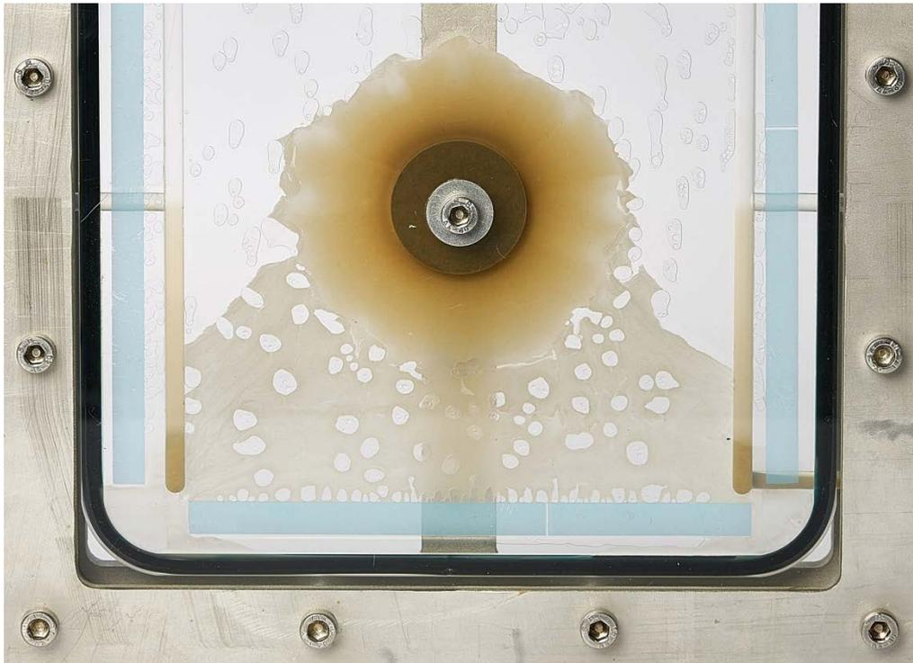
**Figure 6-2.** Experimental cell for measuring of chemical erosion of swelling clays. In this case the clay used is dialysed Nanocore at very low ionic strength in a 0.2 mm vertical fracture. The vertical placement show the impact from gravity on the sedimentation.
