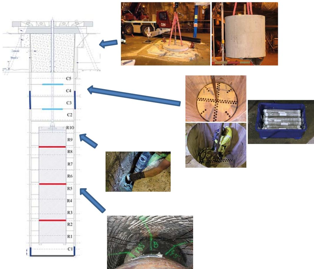
Figure 3-15. Lasgit deposition hole with activities during dismantling and sampling.
