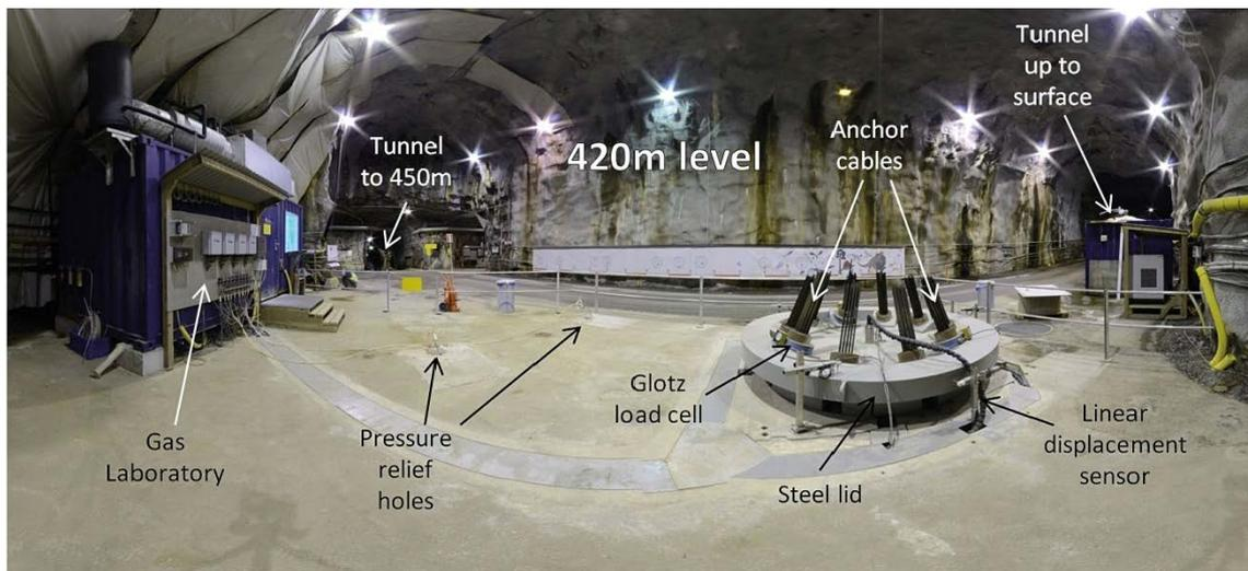
**Figure 3-13.** The Large scale gas injection test at the -420 m level in Äspö HRL.
