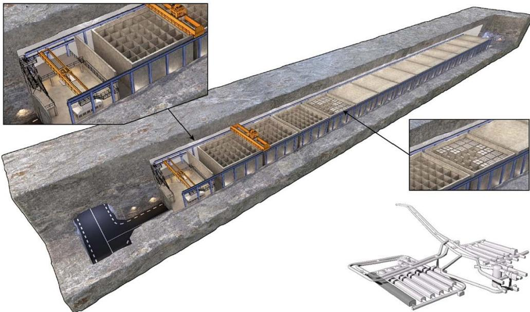
*Figure 3-7. The waste vault for intermediate level radioactive waste, 2BMA.*
