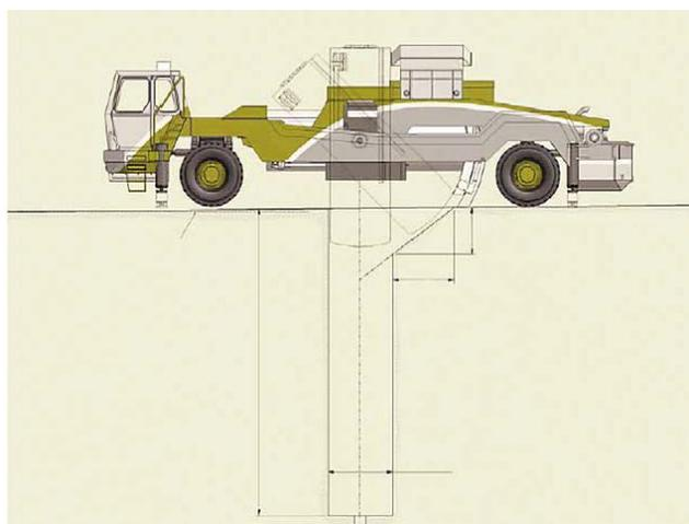
*Figure 5-1. Cross section of a reference design KBS-3 deposition hole.*
