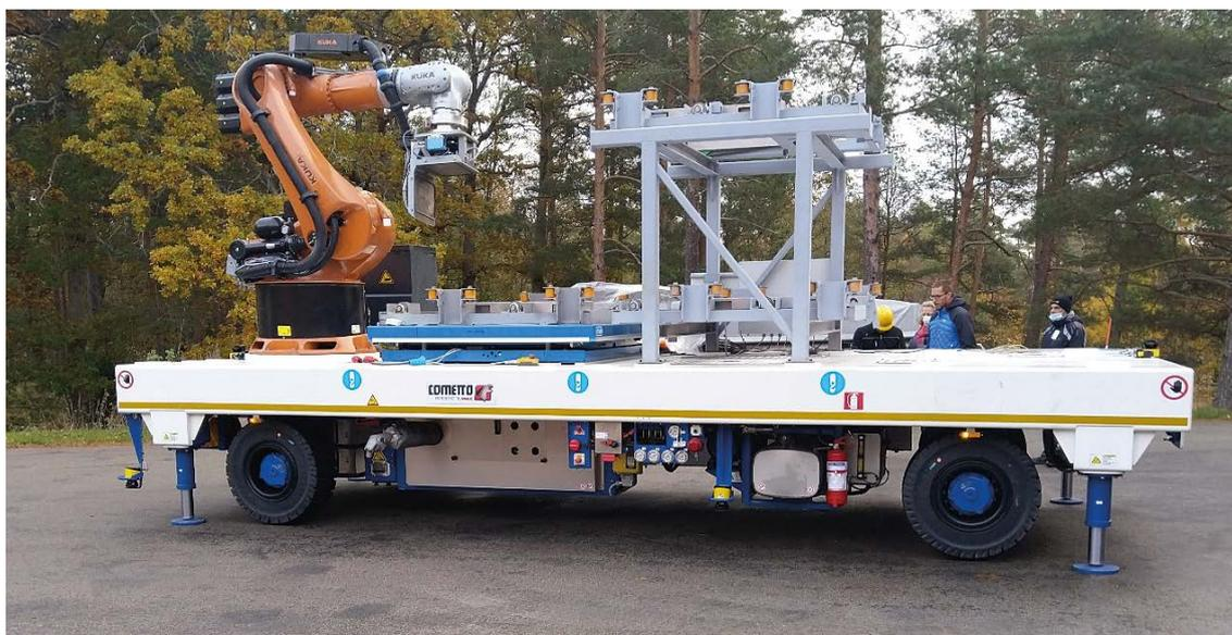
*Figure 4-1. Prototype equipment for installation of backfill.*
