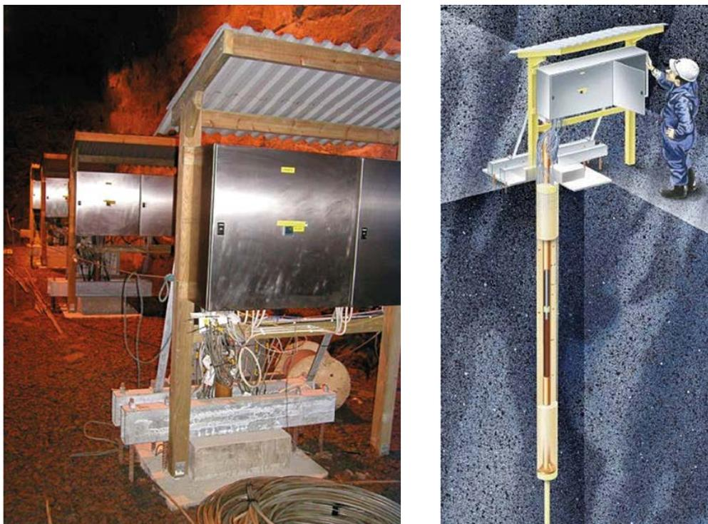
**Figure 3-16.** Left: Photo of the test site in the Äspö HRL. Right: Schematic drawing of a LOT test parcel after installation. Reproduced from Sandén and Nilsson (2020).
