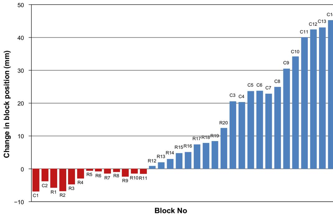
Figure 3-3. The average displacement of the different block layers. The measurements were made in 8 positions.
