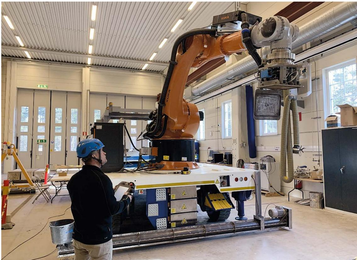
*Figure 4-5. Equipment for installation of backfill. The chassis with the robot, the vacuum tool for handling of blocks, the transporters and the equipment for the installation of a pellet bed on the tunnel floor mounted. Mainly the comprehensive work with converting, integrating and developing the different software to make it compatible.*
