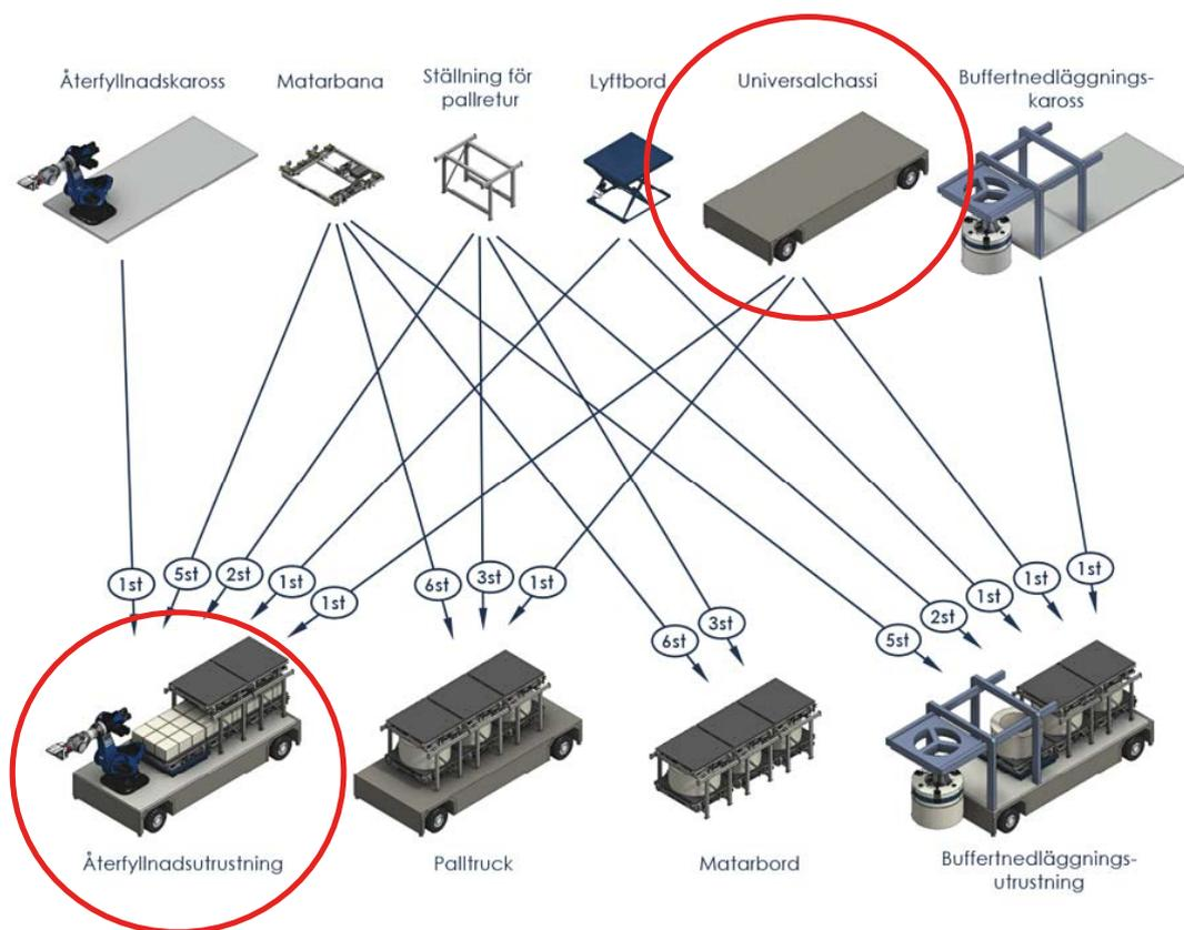
Figure 4-2. Modular chassis concept, with parts used for installation of backfill circled.
