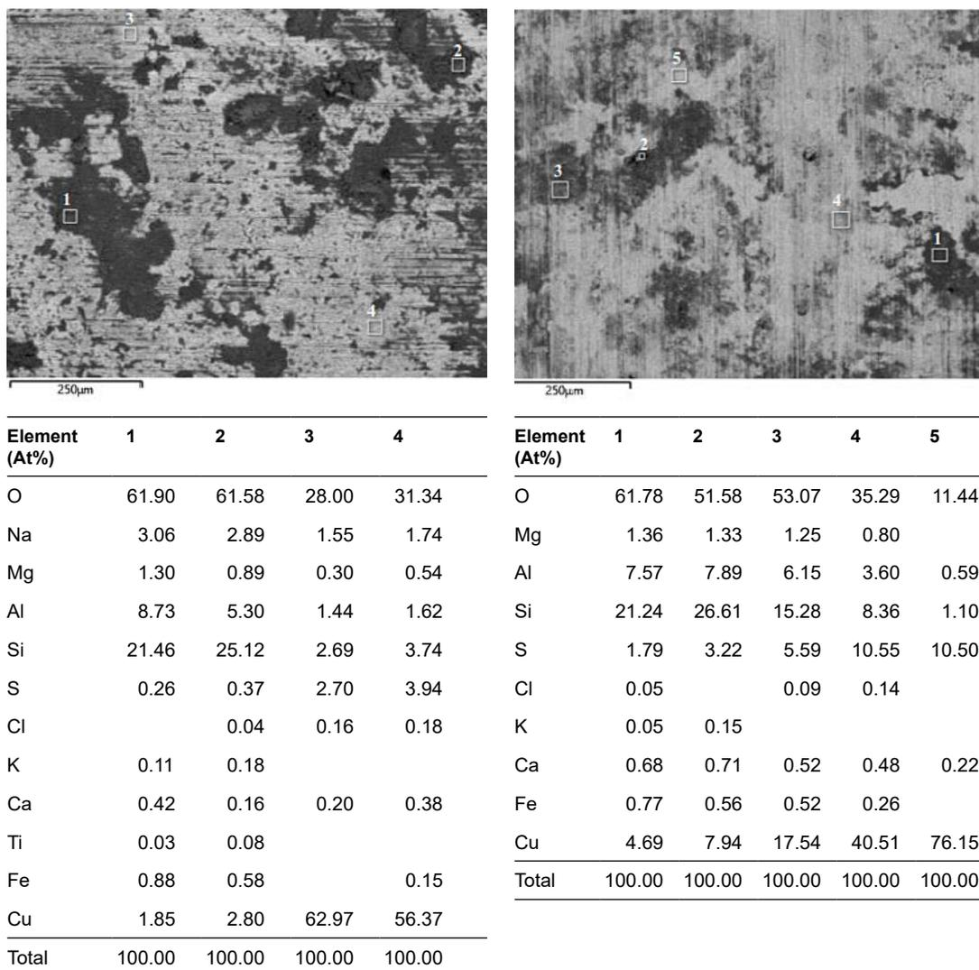
**Figure 3-18.** SEM micrographs with associated EDS analysis results. Copper coupons A3/I (left) and S2/P (right). Magnification x300 (reproduced from Figure 3-10 in Johansson et al. 2020).
