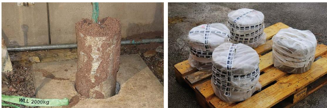
**Figure 3-22.** *Lifting of the concrete cylinder with metallic specimens (left) and the specimens prior to shipping (right).*
