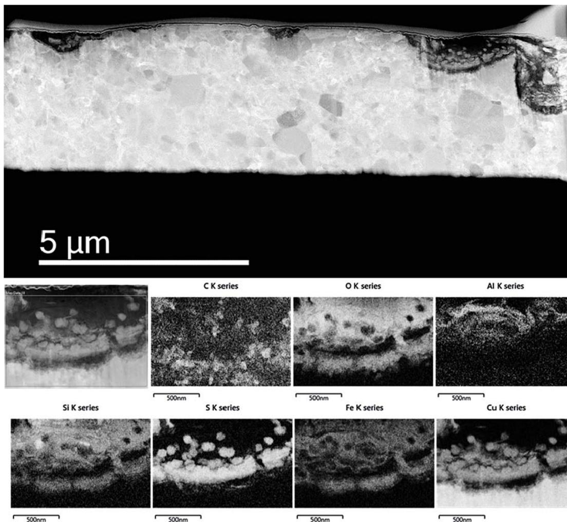
**Figure 3-20.** EDS maps of FIB cut lamella from coupon A3/K (reproduced from Figure 3-15 in Johansson et al. 2020).
