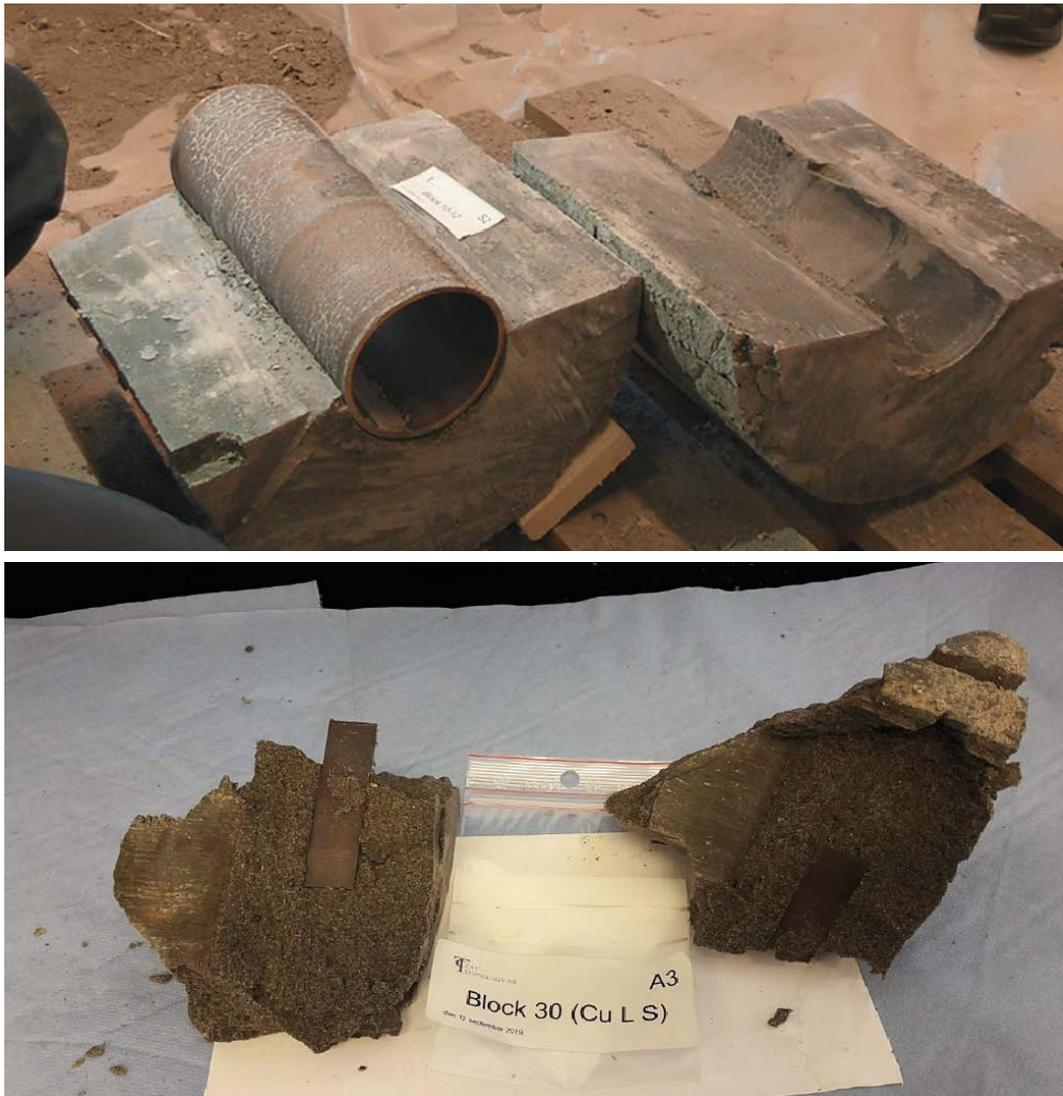
**Figure 3-17.** Upper picture, a piece of the extracted copper pipe. Lower picture, an example of the extracted copper coupons.
