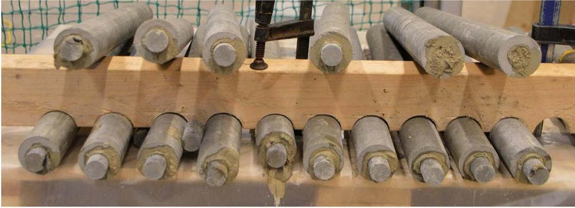
*Figure 3-8. Grout-filled concrete tubes from the initial laboratory investigations.*
