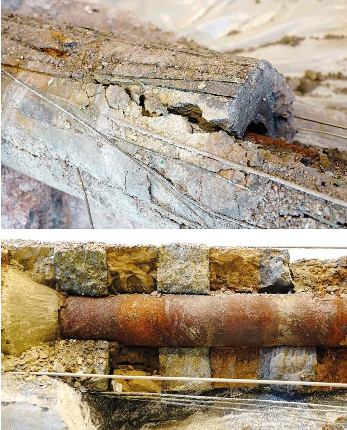
**Figure 3-26.** Highly fractured bentonite blocks from the very high temperature experiment ABM5 excavated in 2017.
