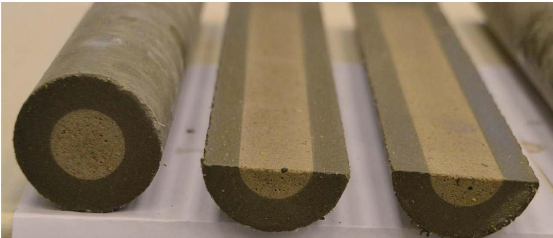
*Figure 3-9. A grout-filled concrete tube after segmentation.*
