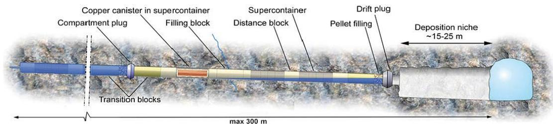
**Figure 3-27.** KBS-3H reference design DAWE with its main components; the plugs with their transition zones, the Supercontainers, and the distance and filling blocks. The illustration shows an ongoing artificial water filling procedure of the second compartment.
