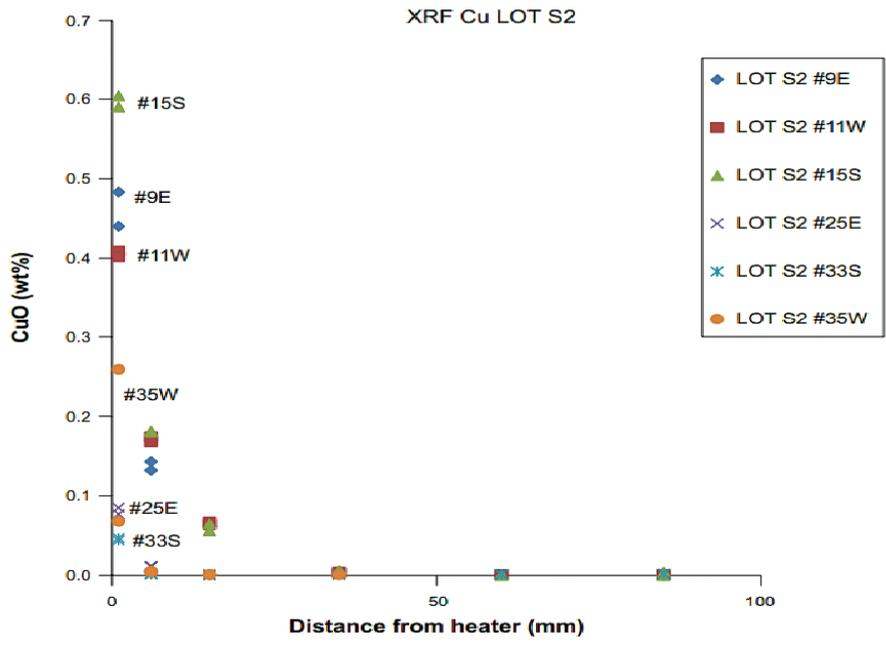
**Figure 3-21.** Upper A3 and lower S2, “CuO” (wt%) as a function of the distance (mm) from the heater pipe in LOT, (reproduced from Figures 3-33 and 3-34 in Johansson et al. 2020).
