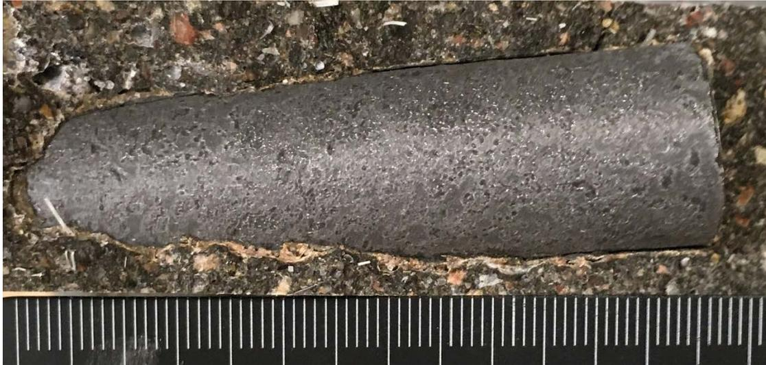
*Figure 3-23. The surface of an aluminium rod which has been deposited in the bedrock under wet conditions for a period of about 10 years showing the presence of a thin crust of whitish corrosion products extruding into the concrete (Kalinowski 2020).*
