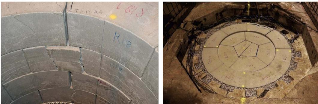
**Figure 3-2.** Observed cracks. Left: Cracks in the buffer surrounding the canister. Right: View of buffer above the canister.
