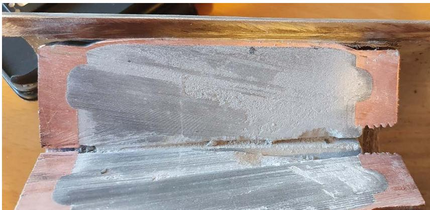
**Figure 3-12.** A cross-section of the self-inflating bridge plug for borehole sealing. The new bridge plug is shaped similar to a conventional packer, though it's made from copper rather than rubber. The bridge plug is not inflated by the use of a fluid or a gas, but rather uses a non-exploding demolishing agent. This produce a solid high pressure that deforms the copper wall to seal against the wall of the borehole, in the picture simulated with a steel pipe.
