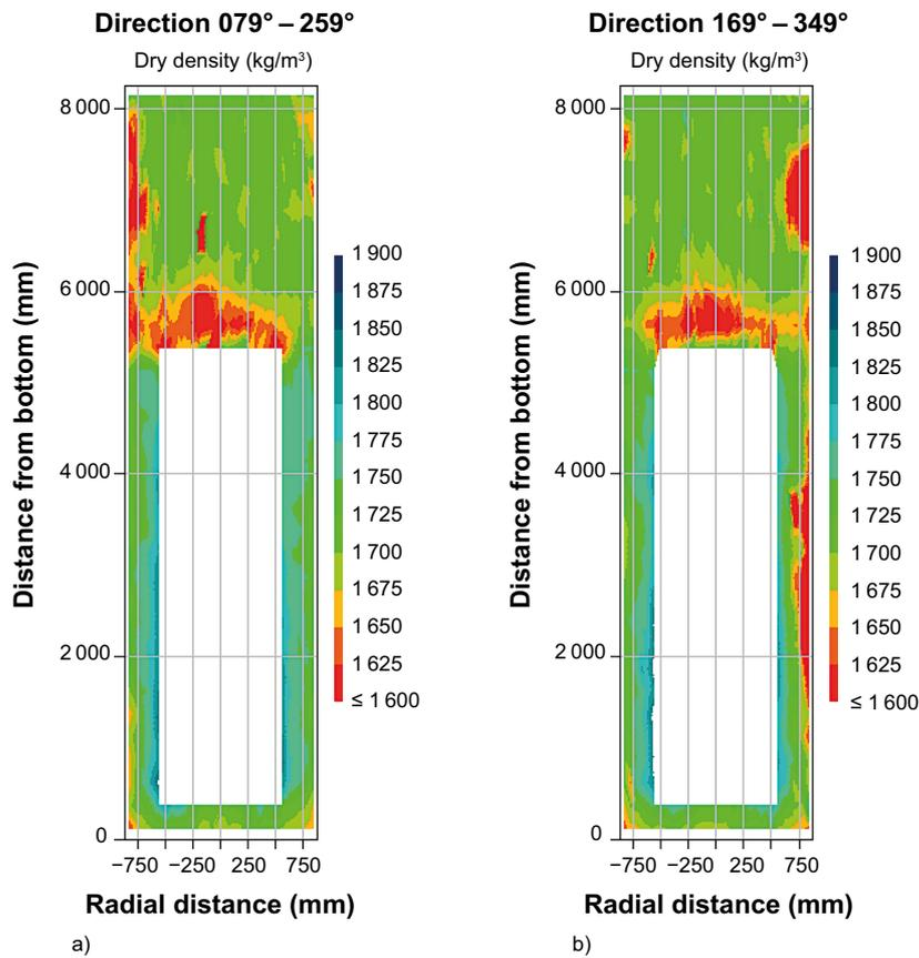
Figure 3-5. Dry density for the buffer a) in section 079°–259° and b) in section 169°–349°.
