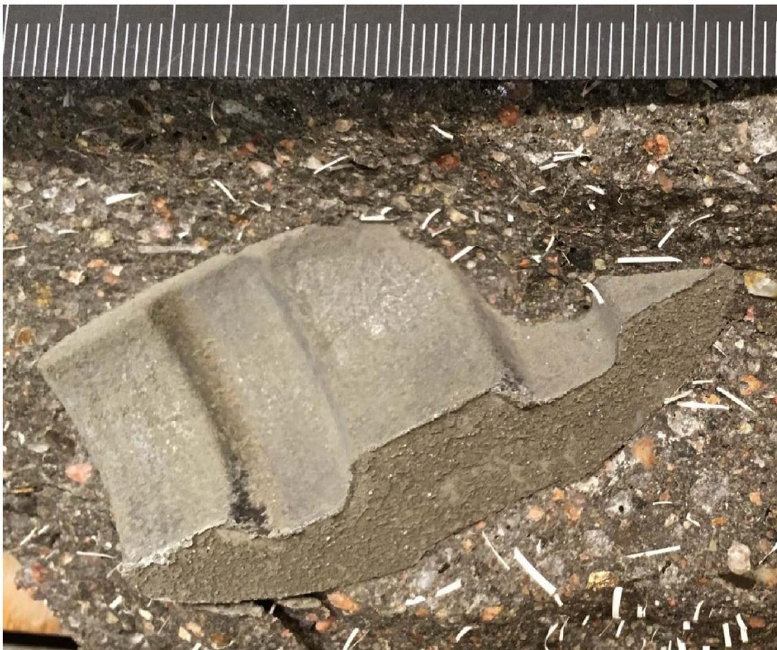
*Figure 3-24. The surface of a zinc specimen which has been deposited in the bedrock under wet conditions for a period of about 10 years (Kalinowski 2020).*
