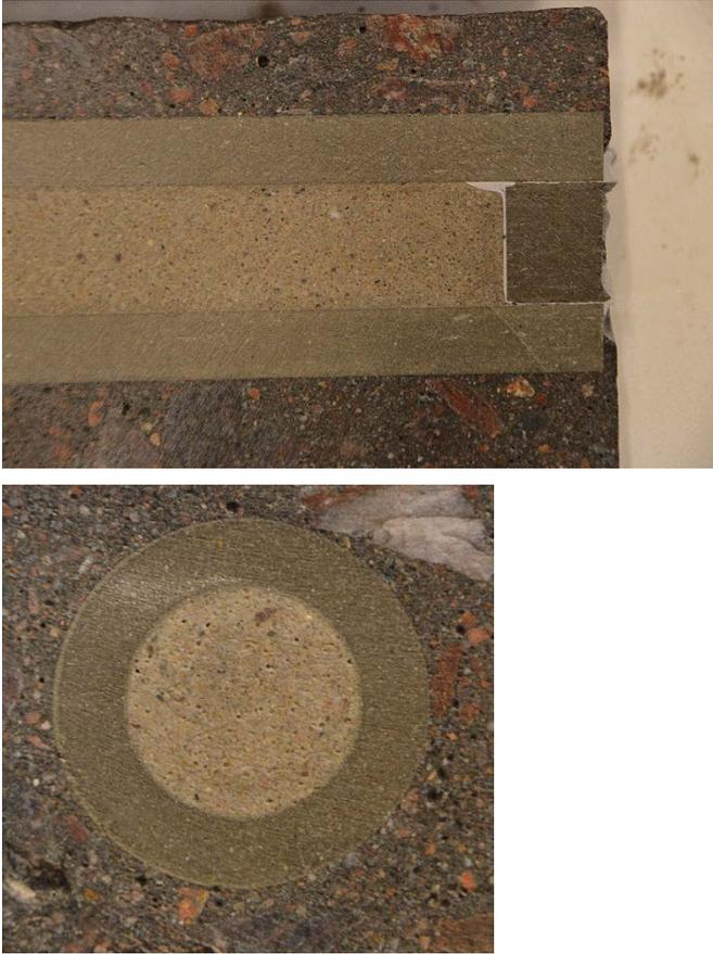
*Figure 3-11. Inner part of grout-filled tube, also showing the cement plug (top image) and cross section of a grout filled tube inside the concrete core.*
