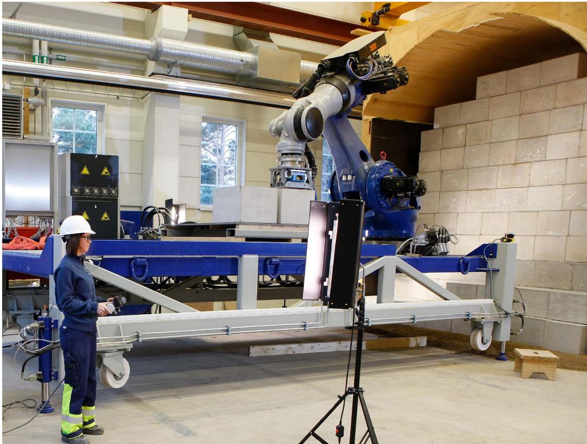
**Figure 4-3.** Earlier version prototype stacking blocks in a full scale test in the Multipurpose test facility. Tests were also performed in the underground laboratory.
