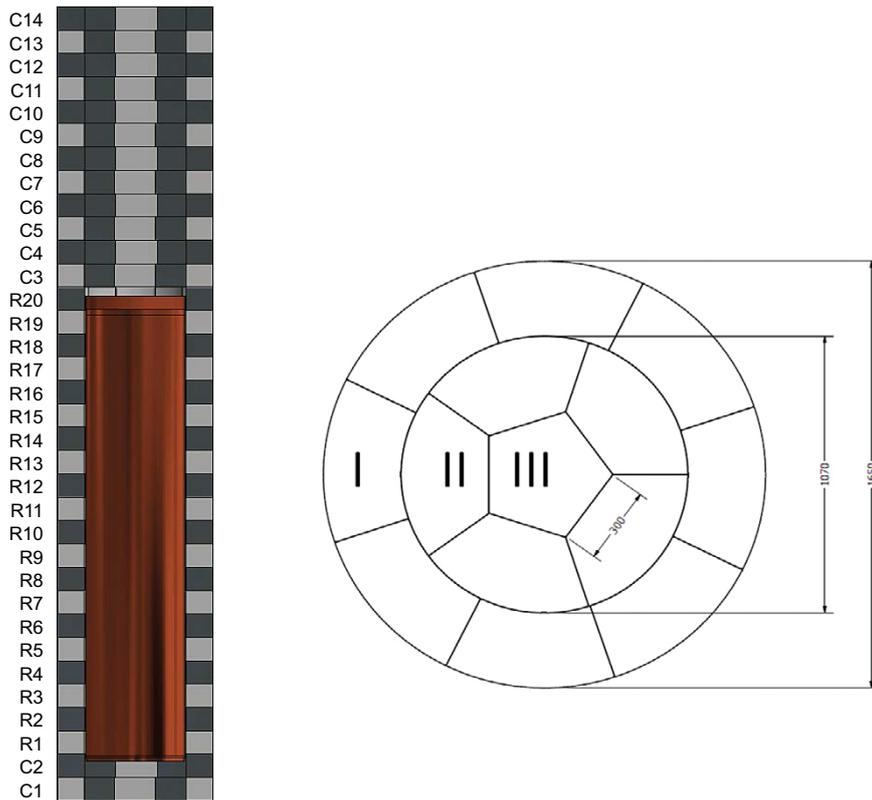
**Figure 3-1.** Test design. Left: Block layers and canister. Right: Block layer design Type (I) Outer block, (II) Inner block and (III) Centre block.
