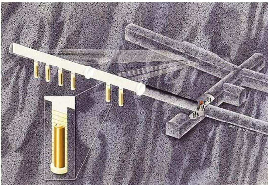
**Figure 3-25.** Schematic view of the layout of the Prototype Repository (not to scale).
