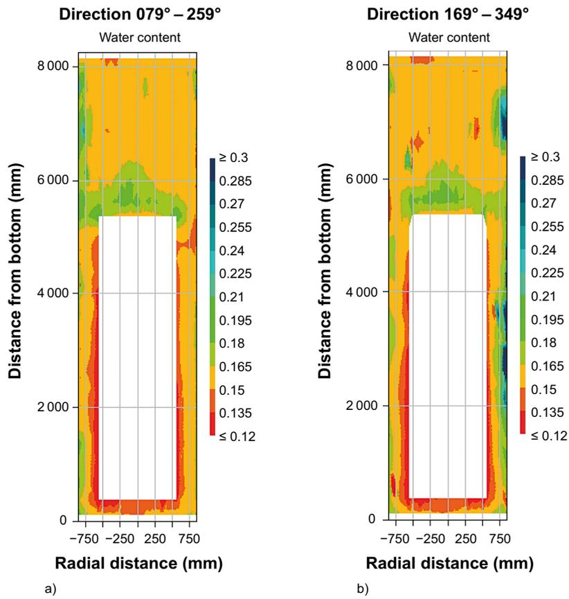
Figure 3-4. Water content for the buffer a) in section 079°–259° and b) in section 169°–349°.
