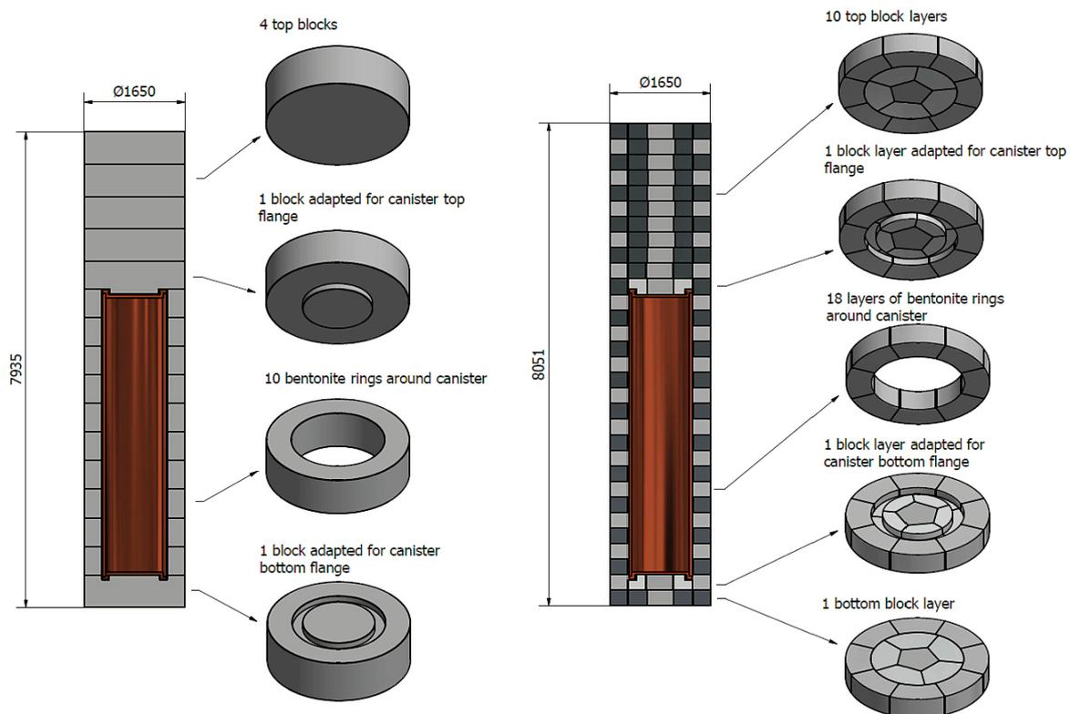
Figure 3-6. Illustration of the differences between the two test designs.
