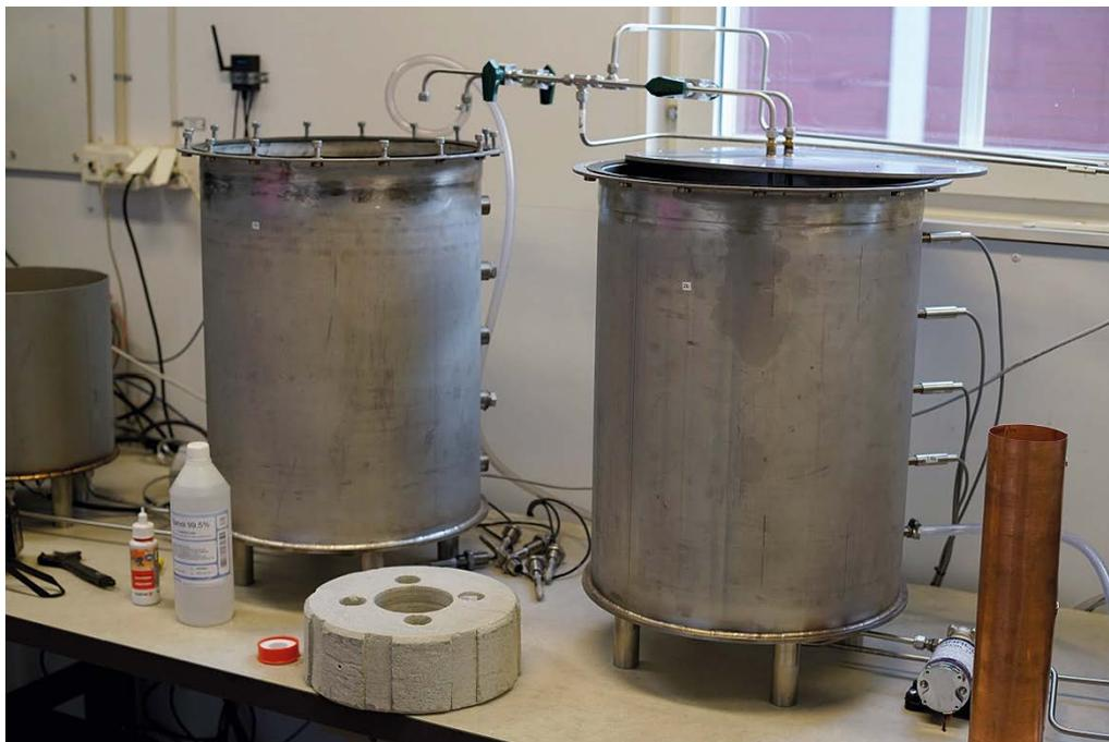
*Figure 6-1. Deposition hole atmosphere test. Bentonite blocks, pellets and a copper heater are placed in a confined volume while oxygen, hydrogen and hydrogensulfide gases are monitored with time.*
