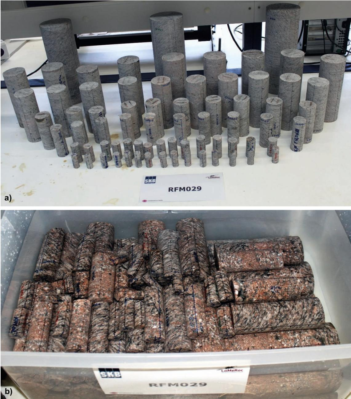
**Figure 4-12.** Samples from rock type 101057 which is the most common rock type at Forsmark, dominating in domain RFM029. The smallest samples are 16 mm in diameter and the largest are 100 mm. b) The same samples as in a) but wet surfaces, which makes the grain size and typical foliated character of the rock type clearly visible.
