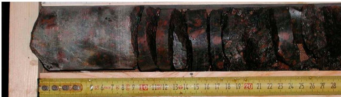
Figure 3-12. Example of core diskings at the TASQ tunnel site in Äspö Hard Rock Laboratory, from a borehole in a point where stresses were elevated due to the excavations (Sjöberg et al. 2007).
