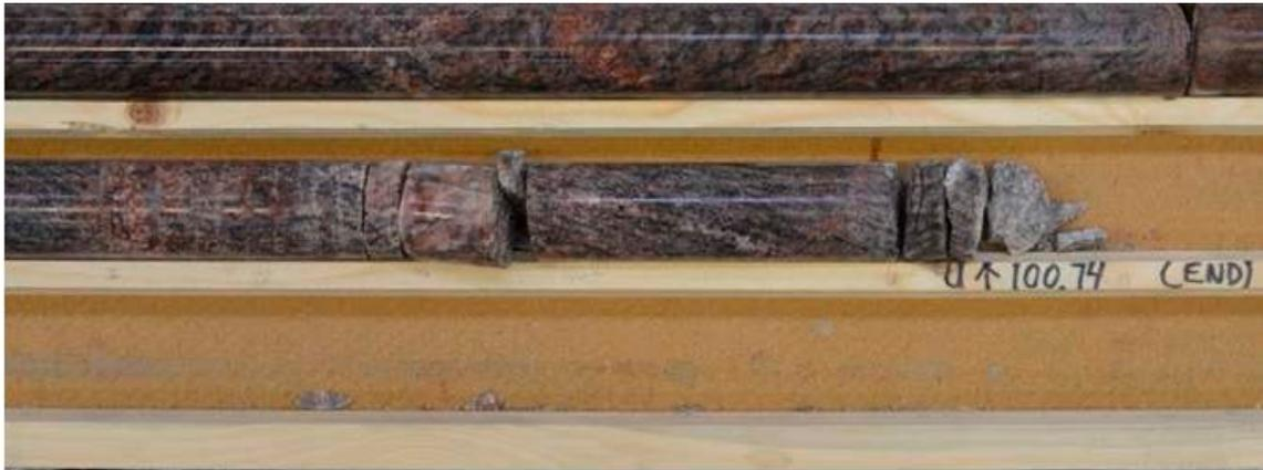
Figure 3-11. Example of core diskings observed on drill core from borehole KFM26 at about 100 m depth, Forsmark site. These core diskings fractures have not all propagated through the whole core, the fractures to the left (white lines) are still connected at the centre of core.
