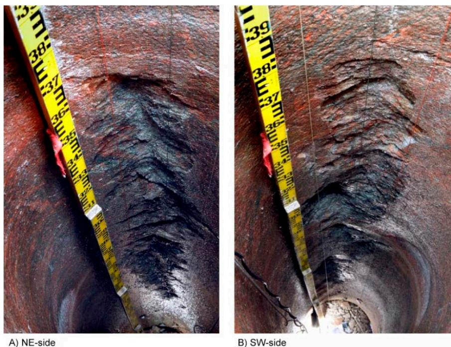
**Figure 2-15.** Example of spalling developed in a ca 490 mm diameter borehole in an experiment (CAPS) with applied thermal loading at the Äspö Hard Rock Laboratory. The two photographs are from the same borehole showing the two opposite sides of the hole. This occurrence is typical for the spalling phenomenon because the stress increase develops on both sides of the created opening, with the orientation depending on the direction of the major stress (Glamheden et al. 2010).
