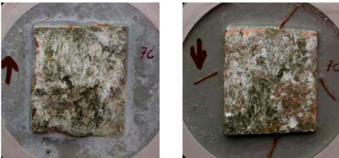
**Figure 6-1.** Example of sealed fracture tested in the laboratory. The lower images are the fracture surfaces after the shear test has broken the sealed fracture (Jacobsson and Flansbjer 2006).
