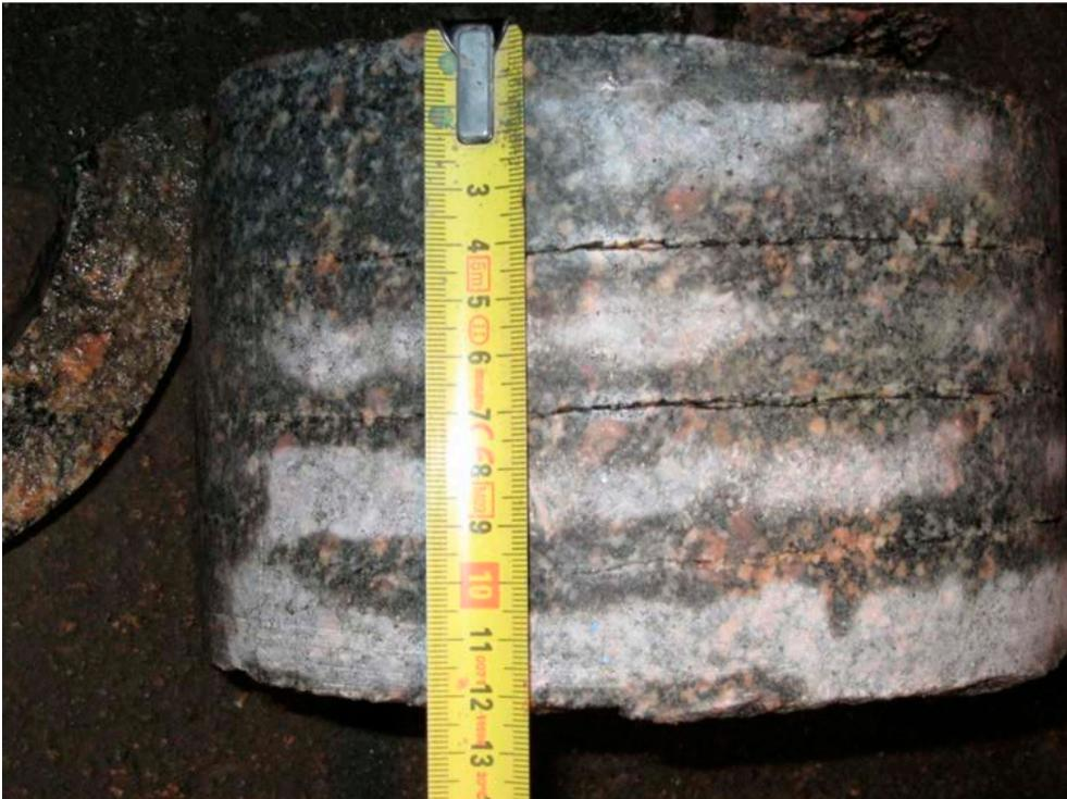
**Figure 3-4.** Ring dishing of a cylinder of Äspö diorite during overcoring of LVDT-cell. The inner diameter is 127 mm and the outer 200 mm (Hakala et al. 2013).
