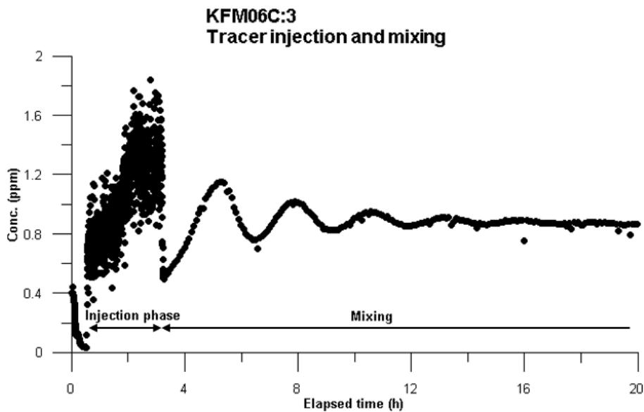
*Figure 4-1. Injection phase and mixing in KFM06C:3.*
