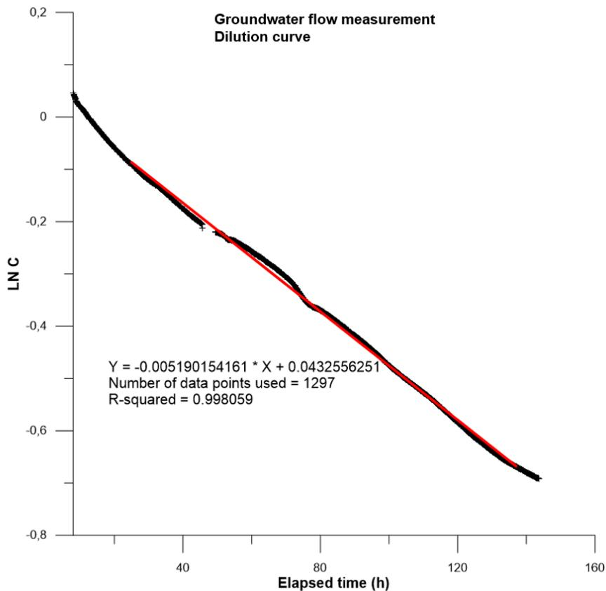
**Figure 3-7.** Example of a tracer dilution graph (logarithm of concentration versus time), including straight-line fit. The used interval is chosen by eye assessment as the injection and start-up effects varies from section to section (Andersson et al. 2018).
