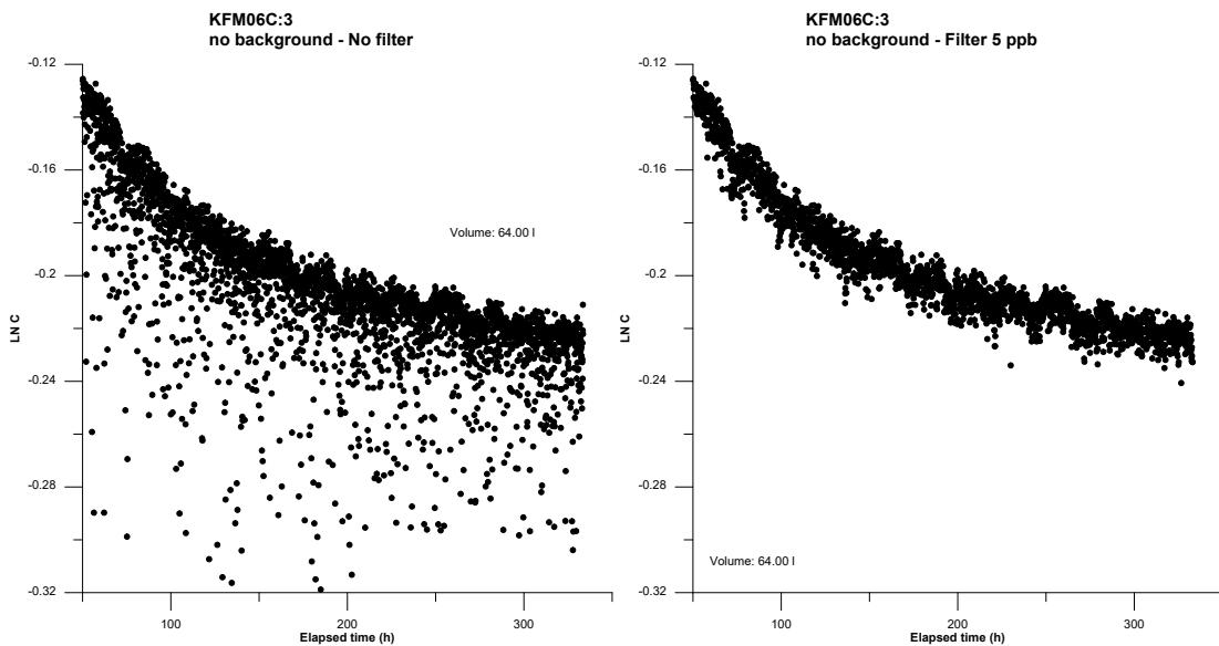
**Figure 4-2.** Unfiltered and filtered data. Fluctuations are due to gas bubbles.
