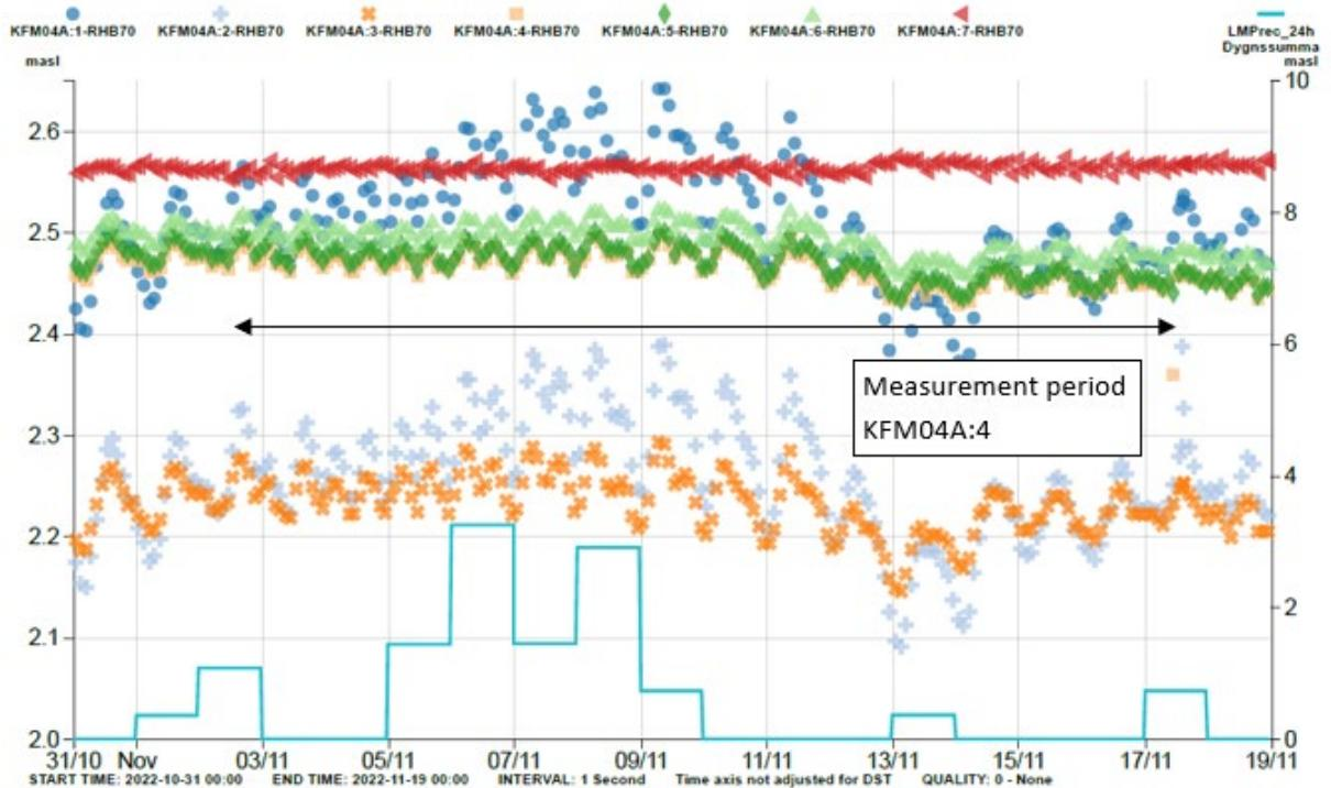
Figure A2-5. Measured section: KFM04A:4 (pale orange, mostly hidden behind section 5, dark green).
