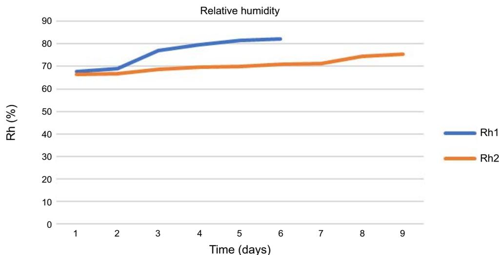
**Figure 4-13.** The evolution of relative humidity in the buffer layer R20. The Rh1 sensor stopped working after six days, probably due to it being exposed to free water.
