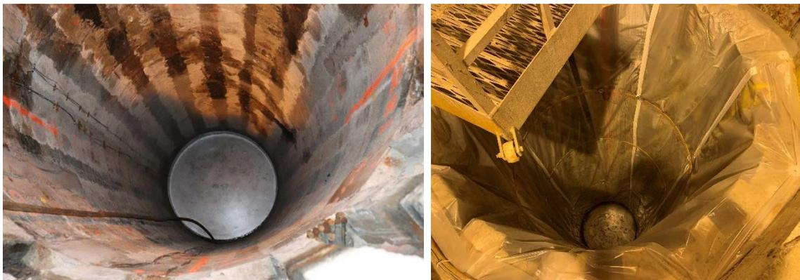
*Figure 3-5. Left: The stainless plate in place in the bottom of the test hole. Right: Plastic tube attached to the plate and the test hole.*
