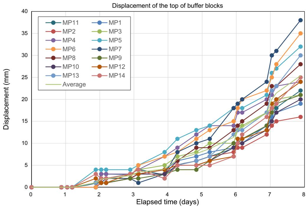
Figure 4-15. Displacement of all of the top buffer blocks.
