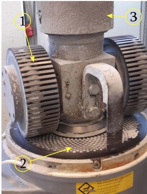
**Figure 2-8.** The extrusion unit: 1) roller, 2) extruder matrix, 3) hydraulic ram.
