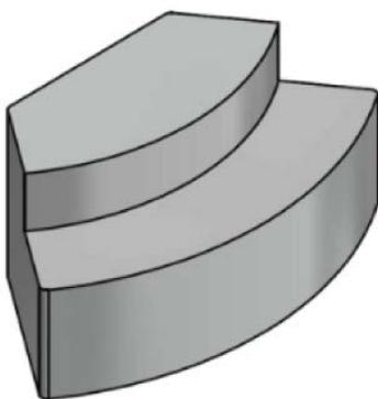
**Figure 2-2.** Machined slot for canister in a type II<sub>1</sub> block to get a type II<sub>2</sub> block.
