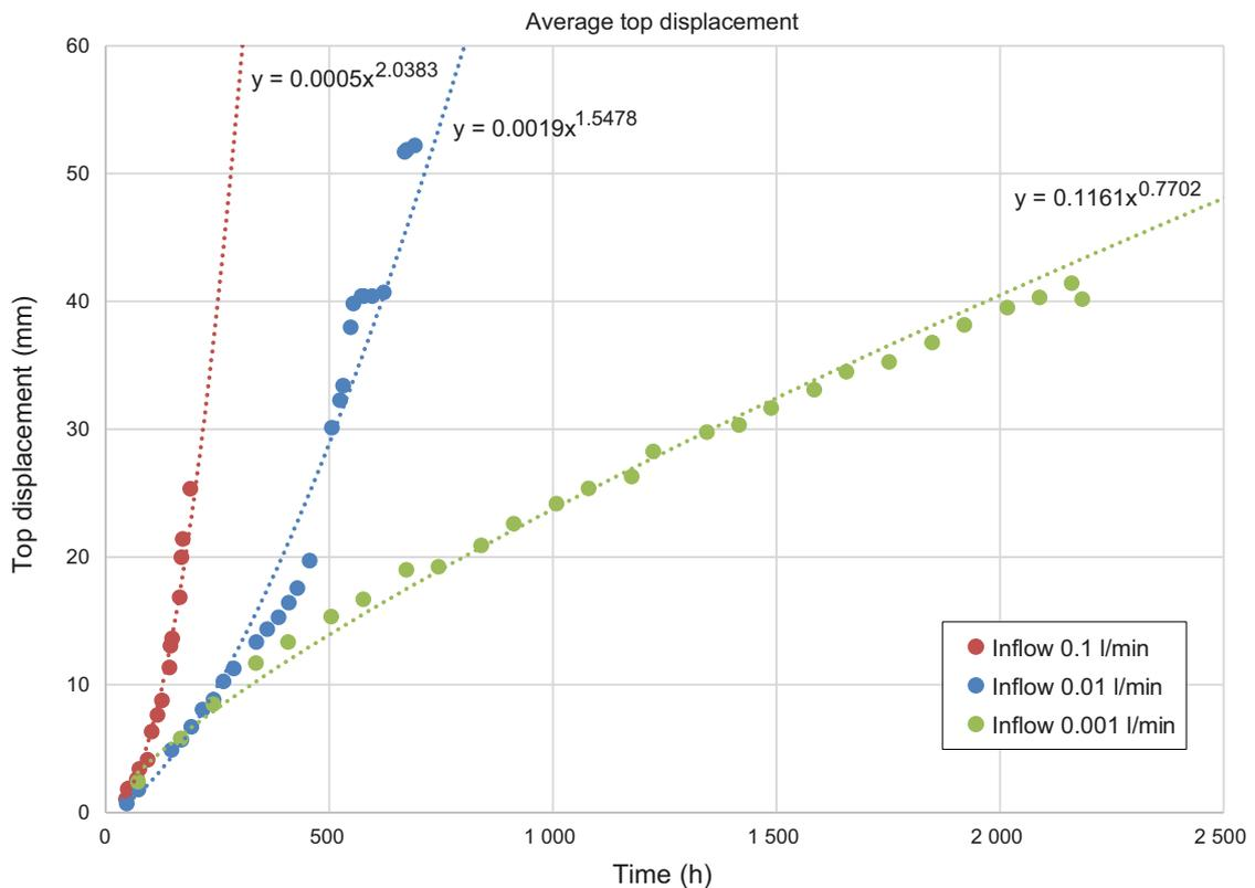
Figure 6-9. The average upwards swelling in the three tests done with segmented buffer blocks.
