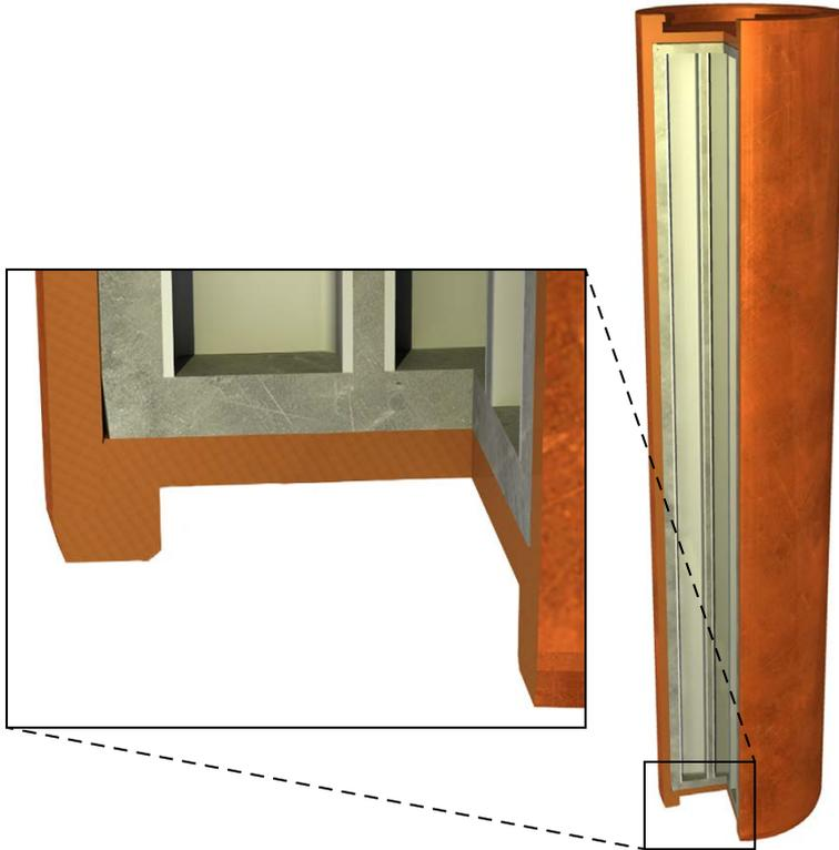
*Figure 4-3. Cross section of canister showing the bottom flange.*
