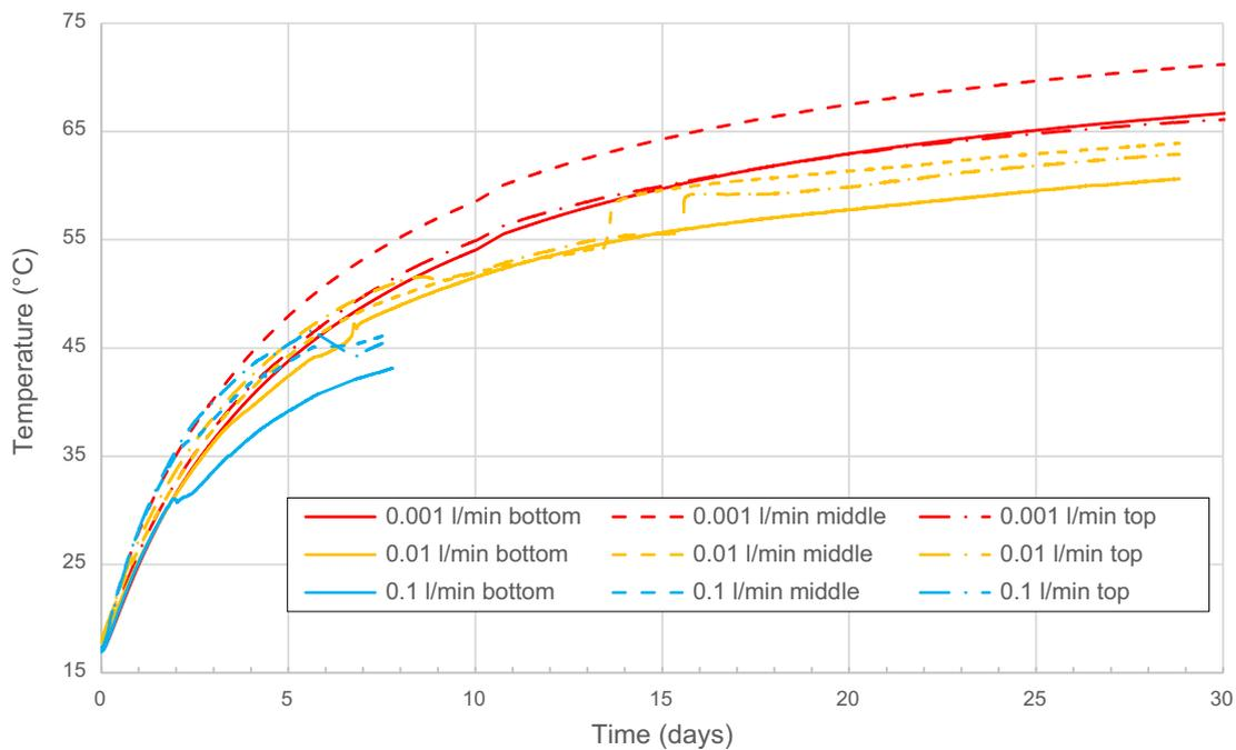
**Figure 6-2.** Temperature measured at the bottom, mid height and top of the canister.
