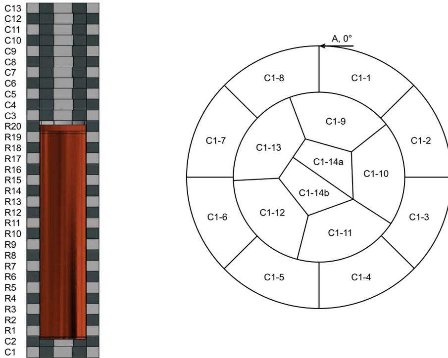
**Figure 3-1.** Example of numbering of individual blocks in one block layer, in this case block layer C1.
