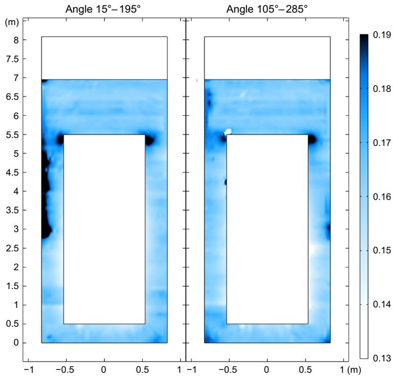
**Figure 6-5.** Water content in the buffer blocks in Test\_Solid\_N with solid blocks and a natural inflow. The scale has been cut of at 13 % and 19 % to be able to see the wetted areas.
