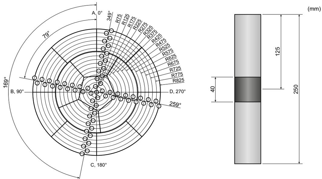
**Figure 3-7.** Left: radial sampling pattern. Right: axial core drilled sample from one block in one position.
