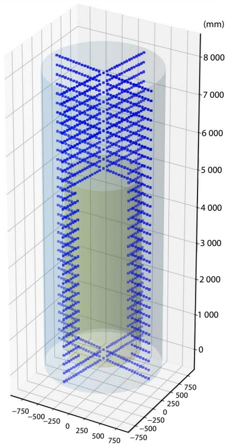
**Figure 3-8.** 3D Visualisation of the sampling done. Blue dots represent the sampling points.
