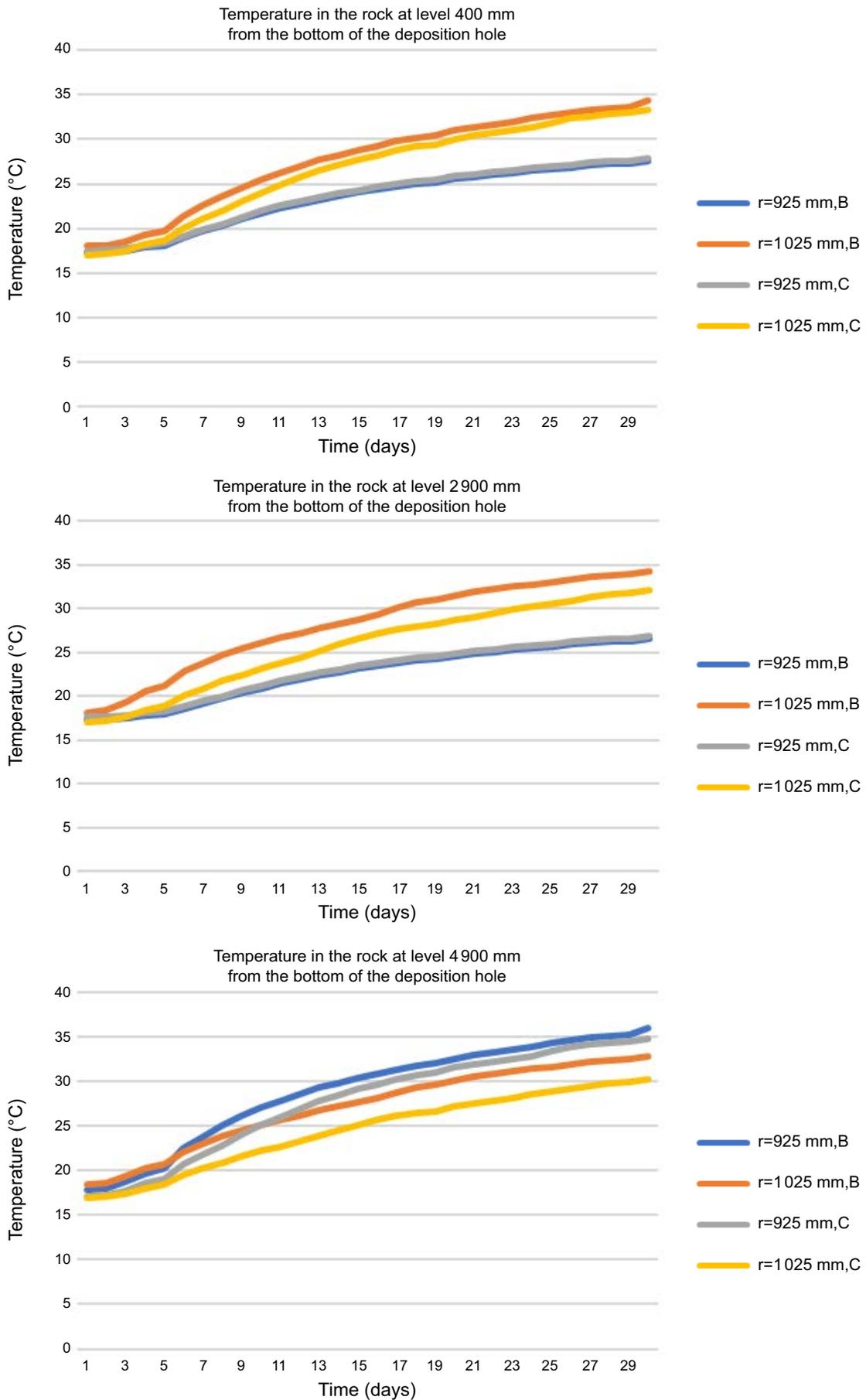
**Figure 5-6.** The temperature evolution in the surrounding rock at three different levels in the deposition hole Top graph 400 mm, middle graph 2900 mm and lower graph 4900 mm from the bottom.
