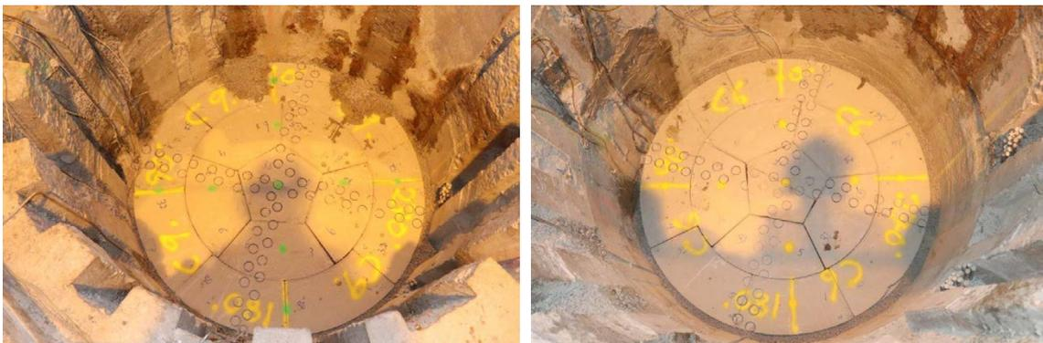
*Figure 5-11. Dismantling and sampling from layer C9 (left) and C6 (right).*
