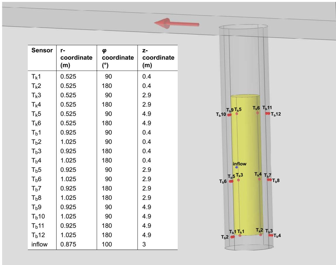
**Figure 3-3.** Placement of the temperature sensors used in the test.  $\varphi = 0$  is towards the tunnel end (red arrow) and  $z$  is calculated from the bottom of the deposition hole.
