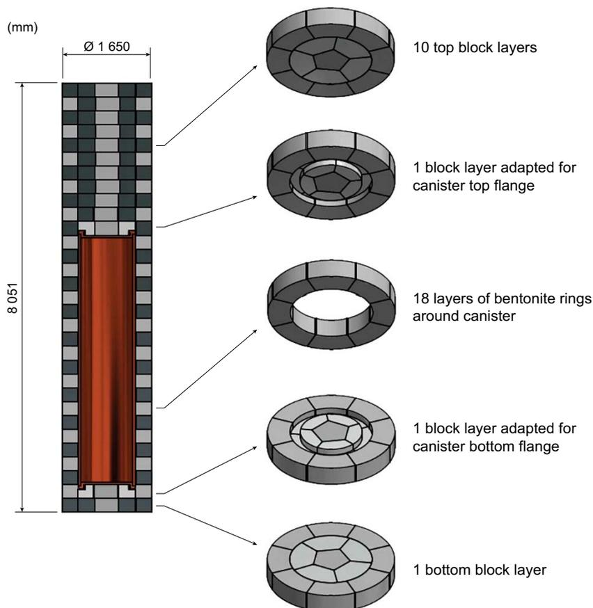
*Figure 1-1. Design of a segmented buffer.*
