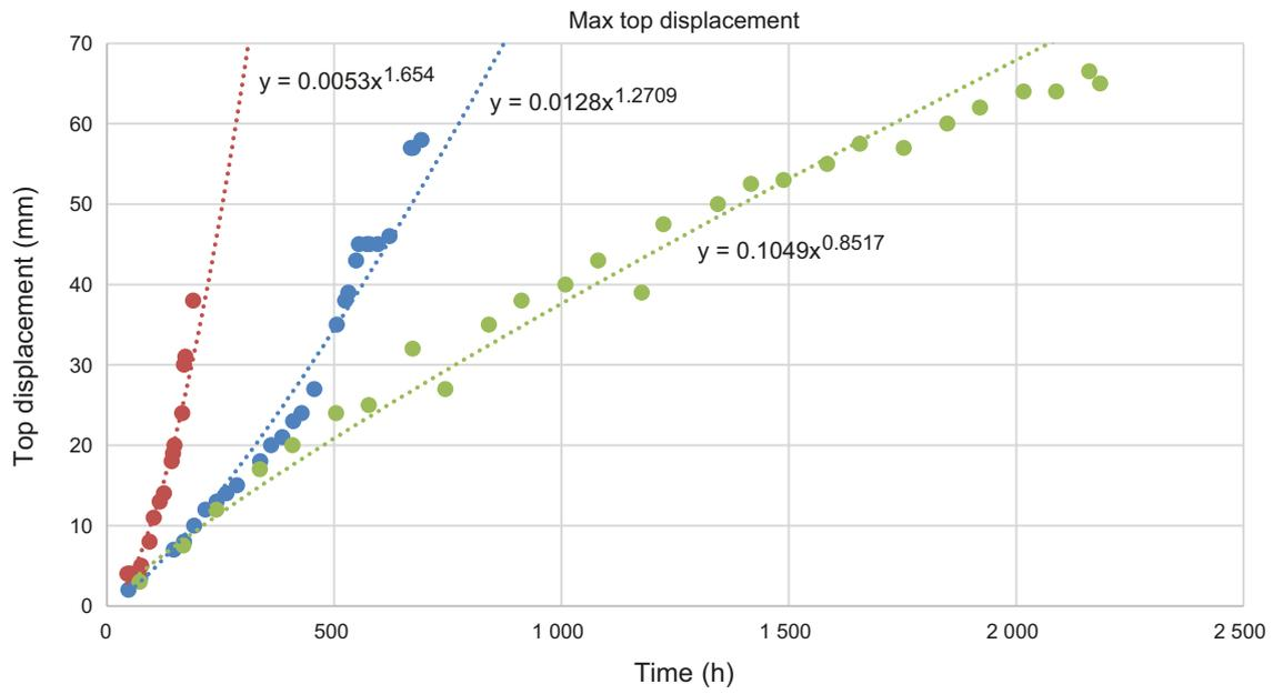
**Figure 6-10.** The maximal upwards swelling in the three tests done with segmented buffer blocks.
