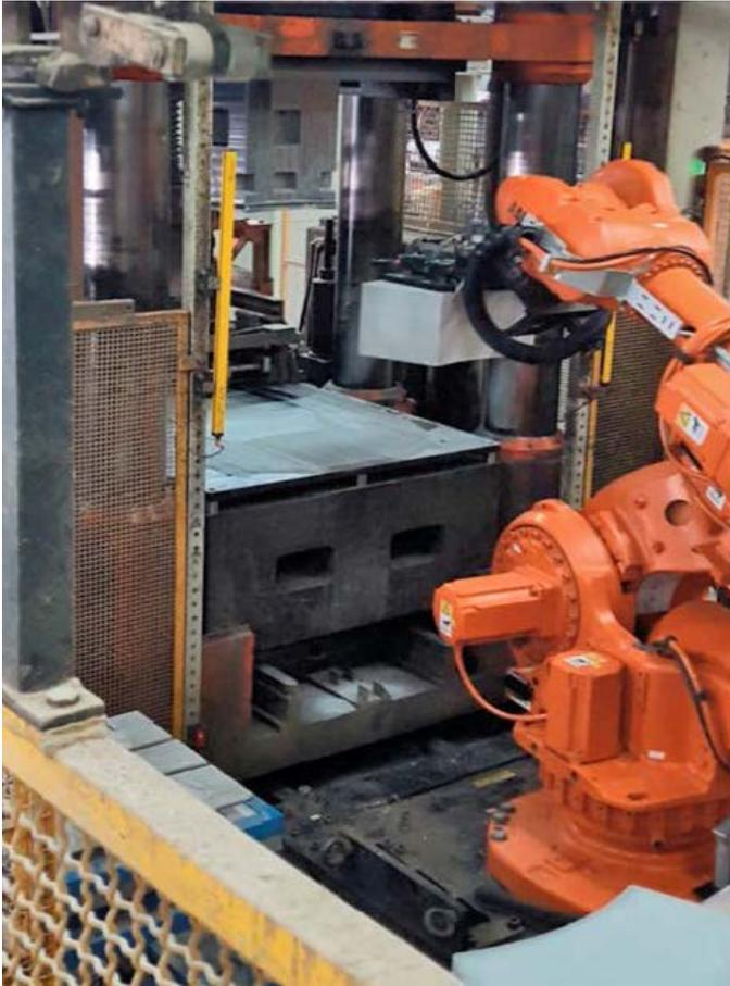
*Figure 2-3. The industrial robot grabbing a finished block from the SACMI press.*
