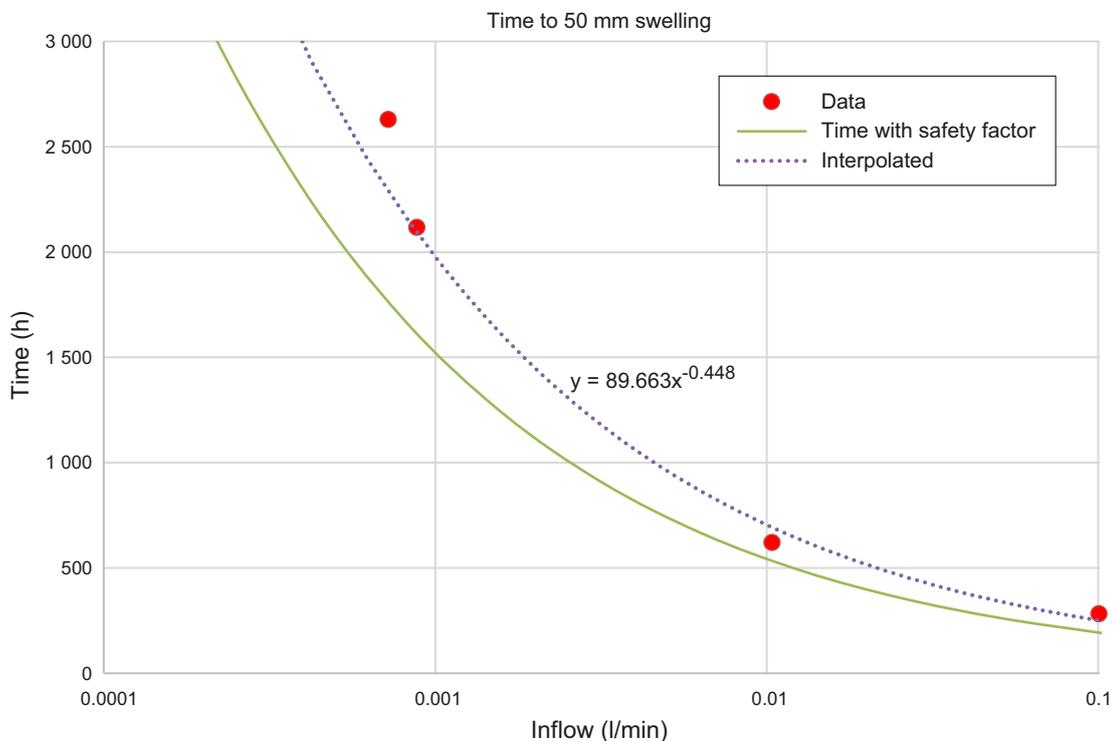
**Figure 7-1.** Estimation of the time before the buffer swells 50 mm upwards for different inflows and interpolation between these points.
