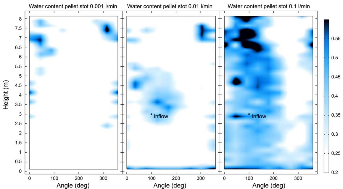
**Figure 6-3.** Water content in the pellet slot for the three tests done with segmented buffer. Left: Test\_Seg\_N, middle: Test\_Seg\_0.01, right: Test\_Seg\_0.1.
