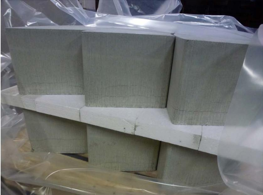
*Figure 2-4. Pallet with 6 blocks separated with Styrofoam and the transparent plastic film.*
