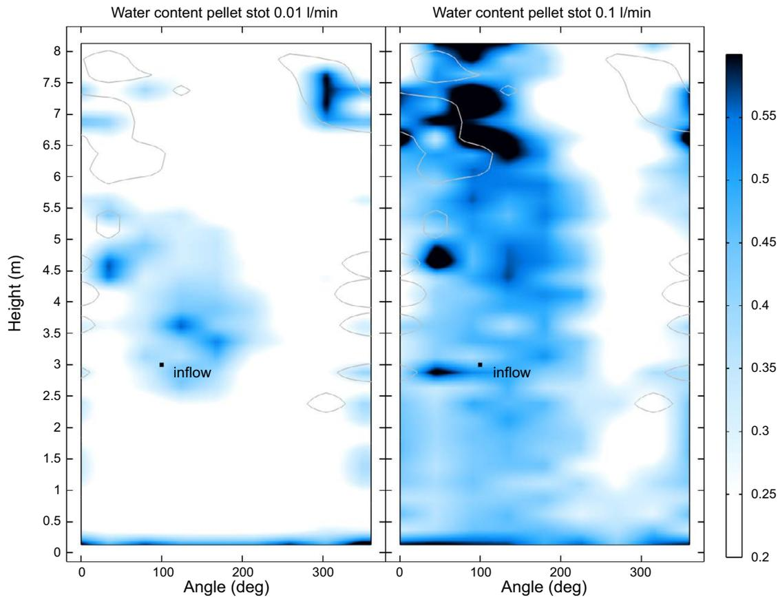
**Figure 6-4.** Wetting of the pellet slot, the areas with natural inflow is indicated with grey isocurves. Left: Test\_Seg\_0.01, right: Test\_Seg\_0.1.
