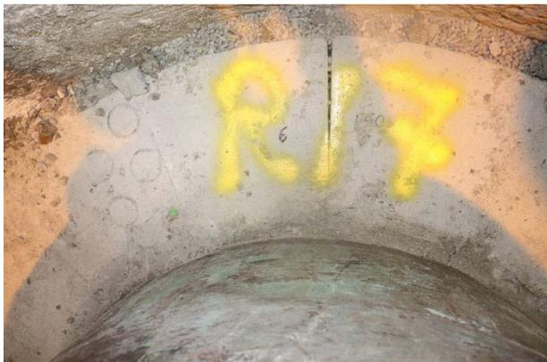
***Figure 4-20.*** Sampling of layer R17 between the canister and the rock surface.
