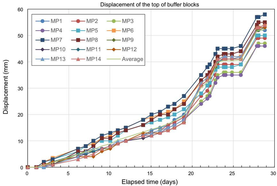
Figure 5-9. Displacement of all of the top buffer blocks.
