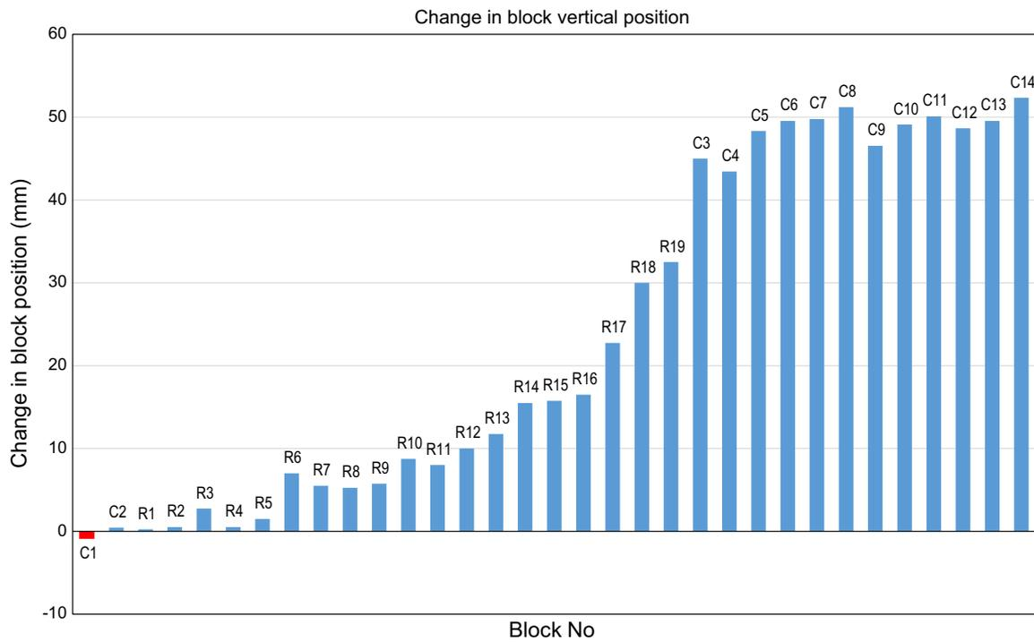
**Figure 5-15.** Changes in block position between installation and dismantling. The naming of layers differs slightly from Test\_Seg\_0.1, see Section 5.1.2.
