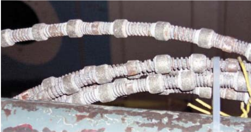
Figure A1-19. Close up of diamond wire saw blade.
