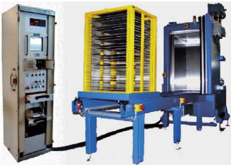
Figure A1-25. RADOS Mobile Clearance Measurement Station.
