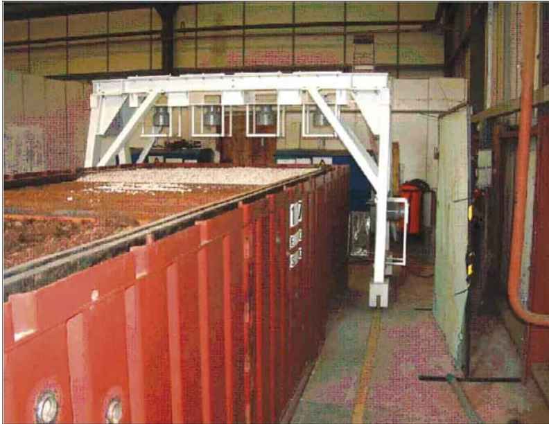
Figure A1-27. Container Monitor for Bulk LLW.
