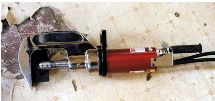
Figure A1-12. Mega-Tech Services Inc. blade plunging cutter.
