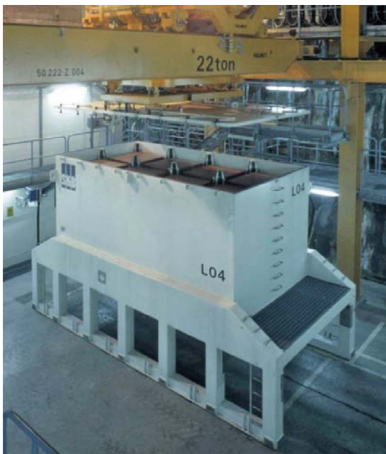
Figure 3-13. Swedish shielded transport container (Photo: Bengt O Nordin, SKB).
