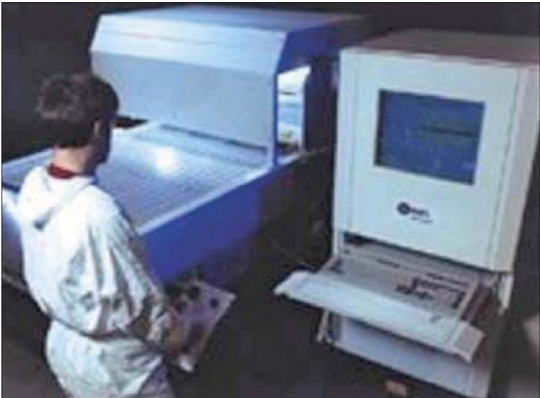
Figure A1-26. IonSens Conveyorised Survey Monitor.
