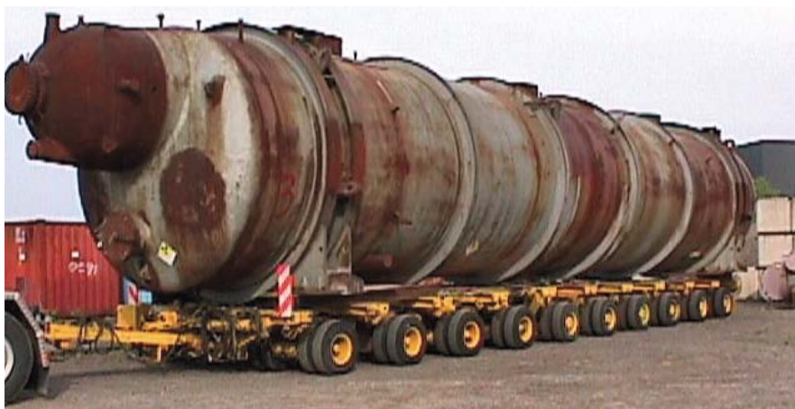
Figure A1-30. Re-heater transported from Oskarshamn 2.
