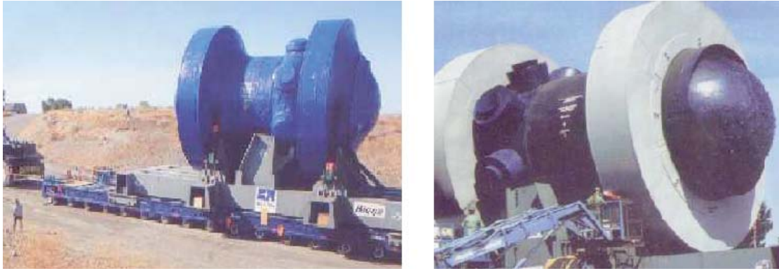
Figure 3-5. Views of Trojan Reactor Vessel with the radiation shield and impact reducers during transport.
