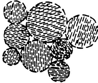
FIG. 2. Schematic microstructure of air-dry MX-80 bentonite powder.
