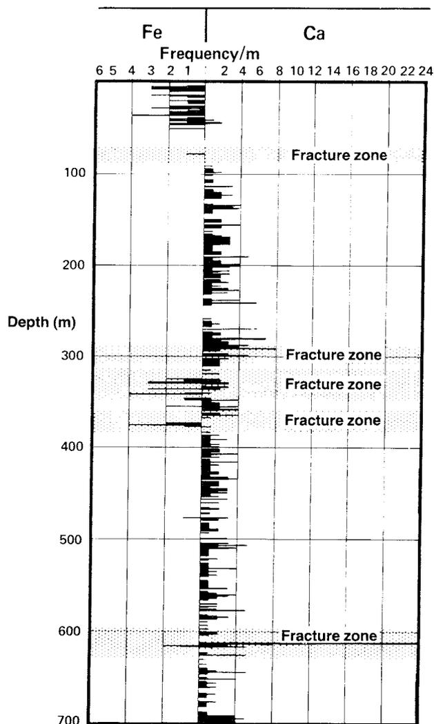
Figure 5-2. Iron oxide hydroxide (rust) and calcite (calcium carbonate) in fracture minerals from drill cores, Klipperås, borehole Kl 12. Oxidizing conditions (rust) and calcite dissolution in the upper 100 m are followed by reducing conditions and calcite precipitation further down. Traces of oxidation are also found in the fracture zones.
