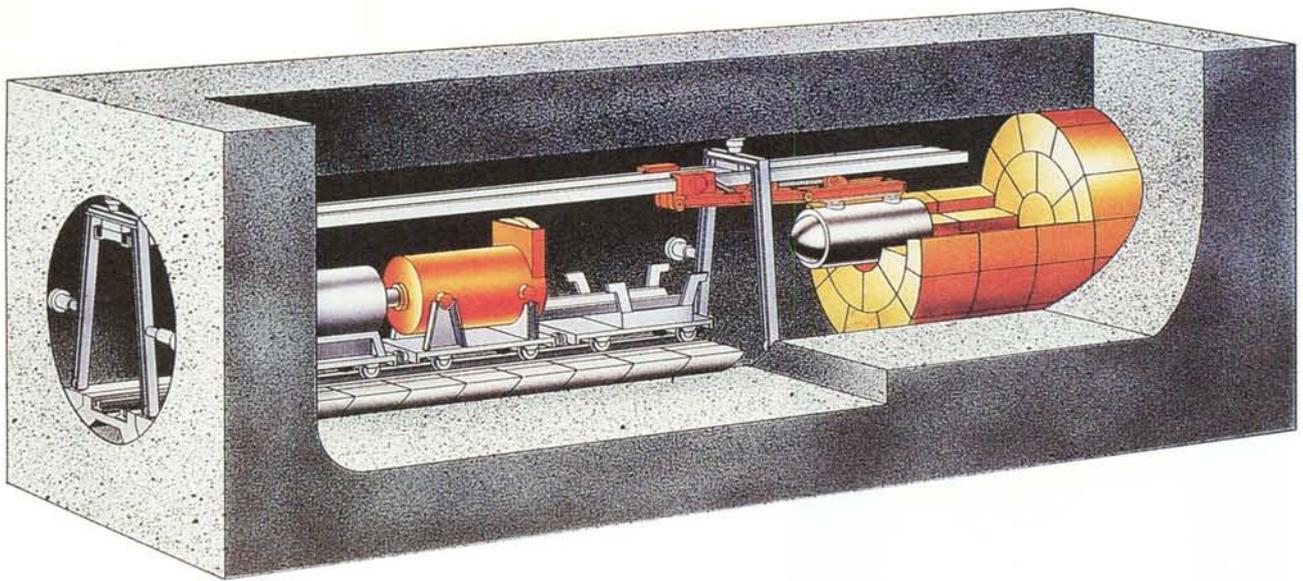
Figure 2-2. According to the NAGRA Gewähr project 1985, canisters and highly compacted bentonite blocks are placed in full-face driven tunnels.
