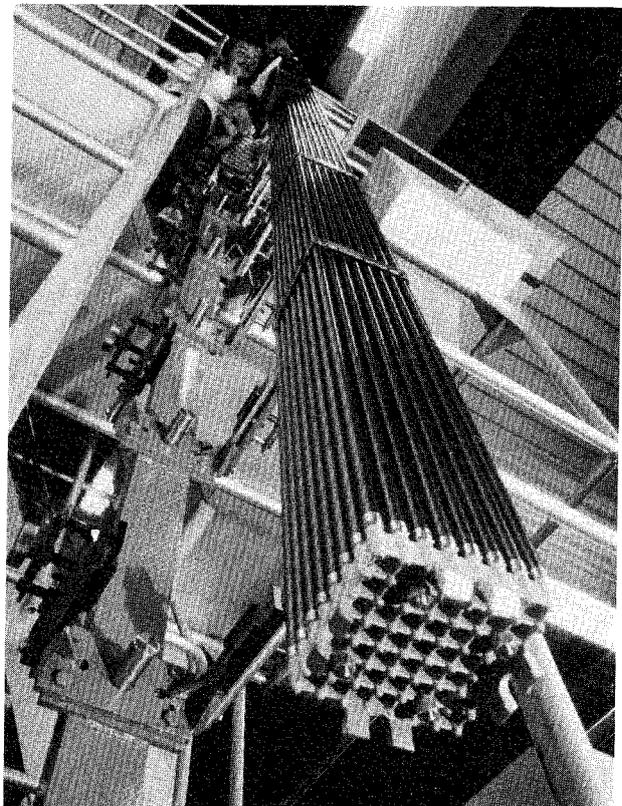
Figure 2-2. Fuel assembly for boiling water reactor.
