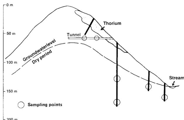
Figure 7-7. Schematic illustration of the planned sampling in boreholes and tunnel in Morro do Ferro, Brazil.
