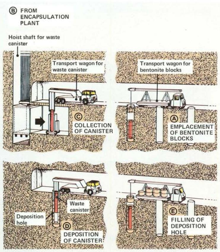
Figure 2-1. According to KBS-3, canisters and blocks of highly compacted bentonite are deposited in holes drilled in the rock underneath the tunnel. The tunnel is then filled with bentonite/sand mixture.
