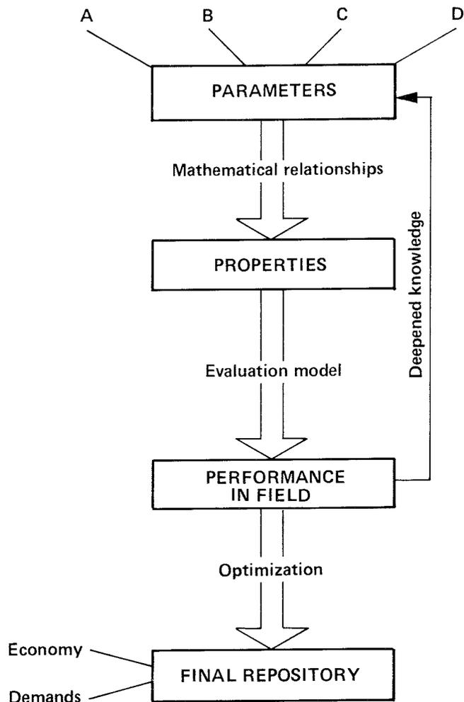
Figure 2-8. General scheme for investigation of buffer material.
