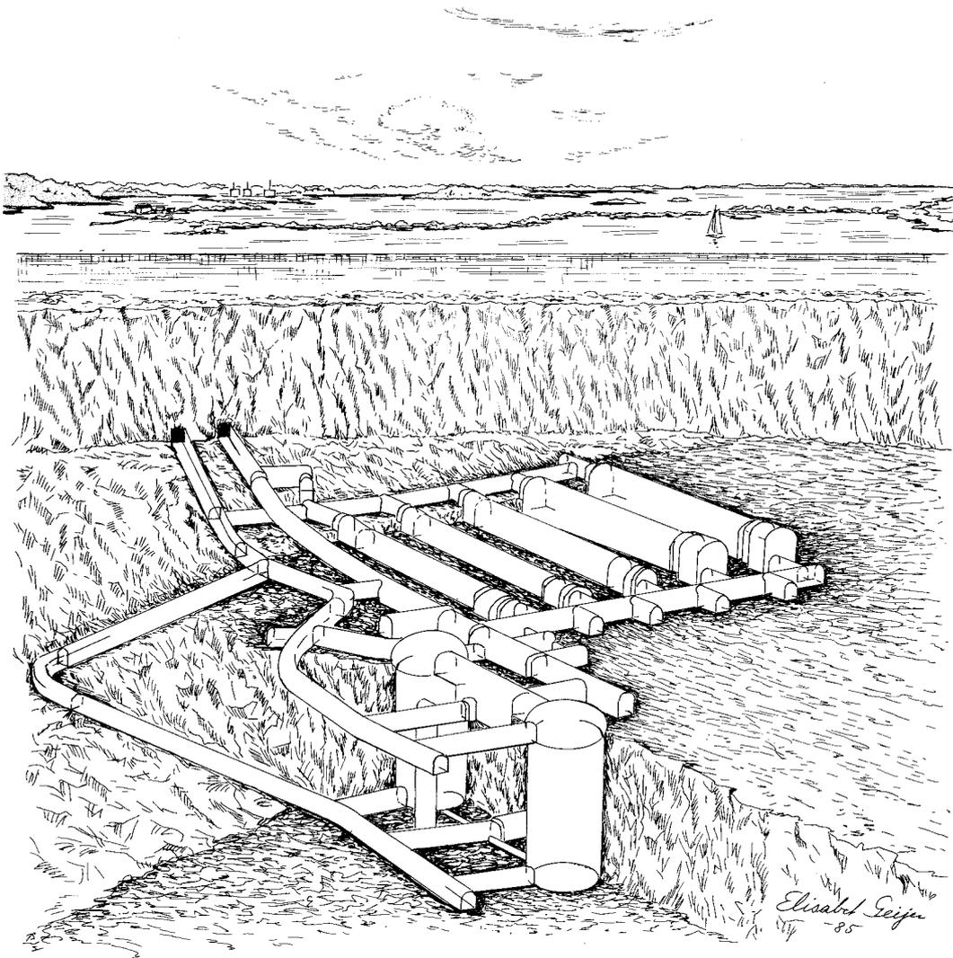
Figure 3-3. Final repository for reactor waste (SFR).
