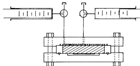
Figure 5-4. Equipment for measuring hydrogen production in alpha-irradiated wet compacted bentonite. The radiation source contains <sup>241</sup>Am and gives 30 MBq (nominal activity). The diameter of the active surface is 25 mm.
