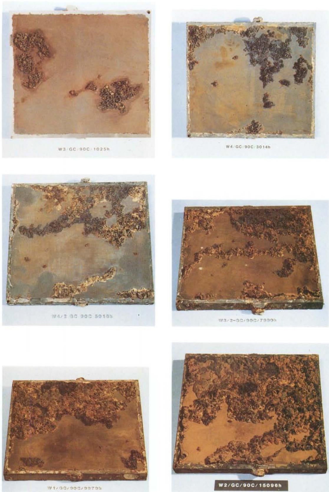
**FIGURE 8** THE DEVELOPMENT OF LOCALISED CORROSION IN PLATES CONTAINING A PENETRATION AUTOGENOUS ELECTRON BEAM WELD
