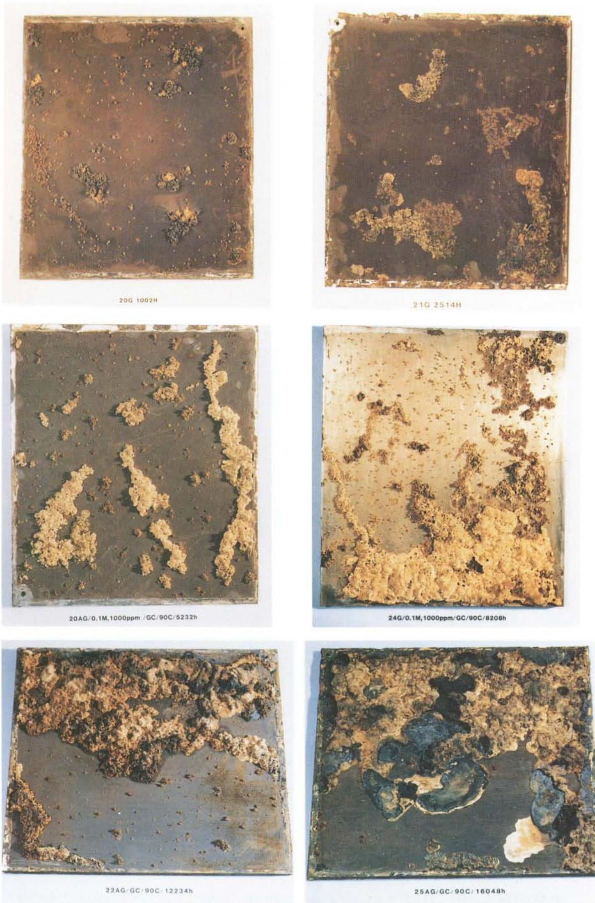
**FIGURE 7** THE DEVELOPMENT OF LOCALISED CORROSION WITH EXPOSURE FOR THE TESTS AT 90C
