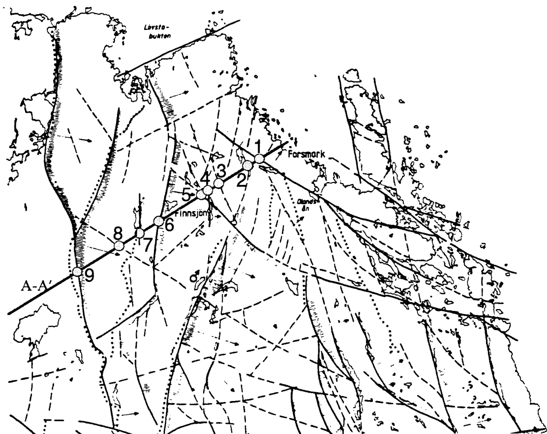
Figure 2.1 Lineament map of northern Uppland with the Finnsjön area. Location of A–A' and fracture zones [Ahlbom, et al., 1987]. The circles 1–9 indicate the intersection between the modelled cross section and assumed vertical fracture zones.
