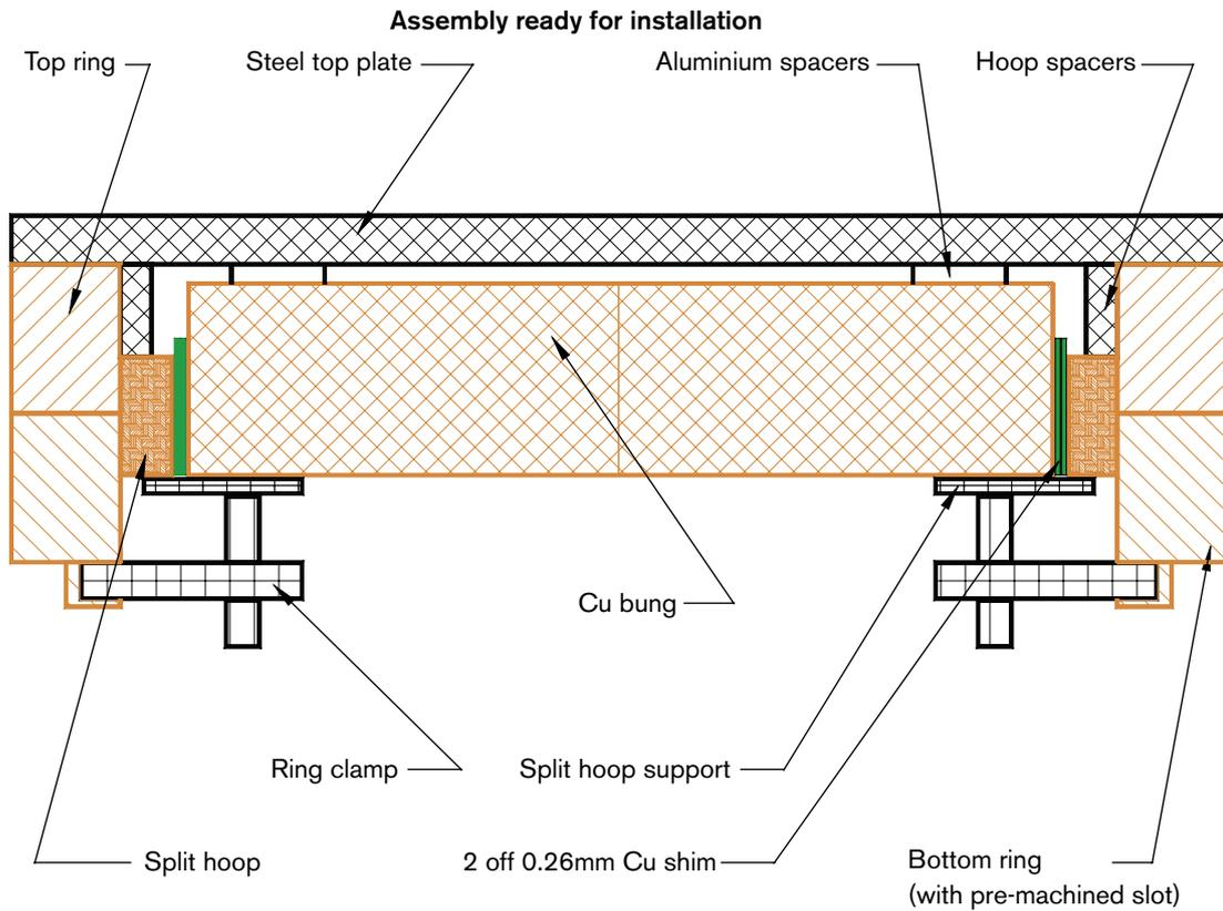
**Figure 6-18.** Cross-section through the full penetration weld set up.
