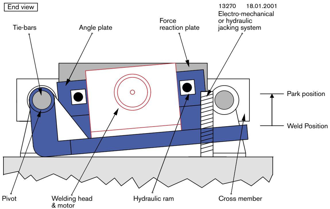
**Figure 8-2.** Scheme of a tool probe exit hole parking system.
