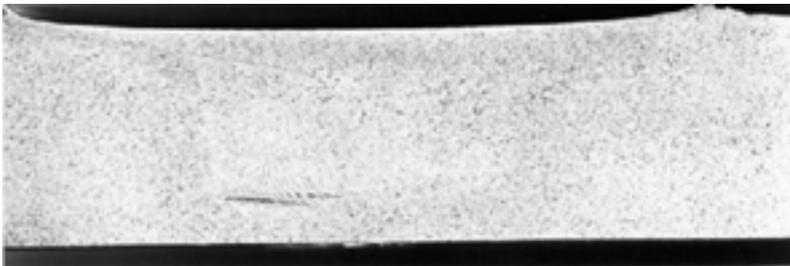
**Figure 4-5.** Transverse metallurgical section cut through an FSW in 10 mm copper plate.
