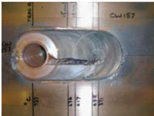
*Figure 10-2. An extreme example of a surface breaking void (CW157).*
