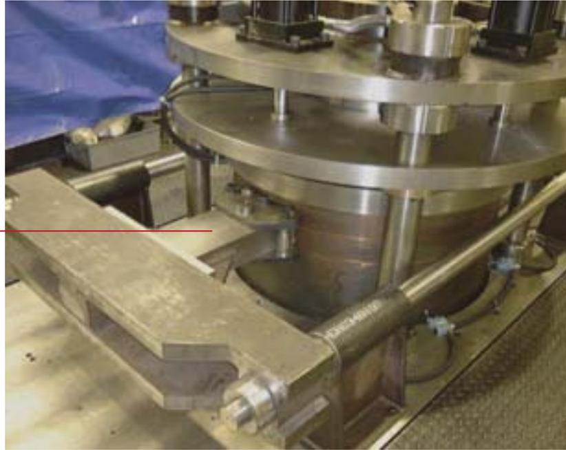
*Figure 5-8. The experimental canister base welding machine showing the roller backstop.*
