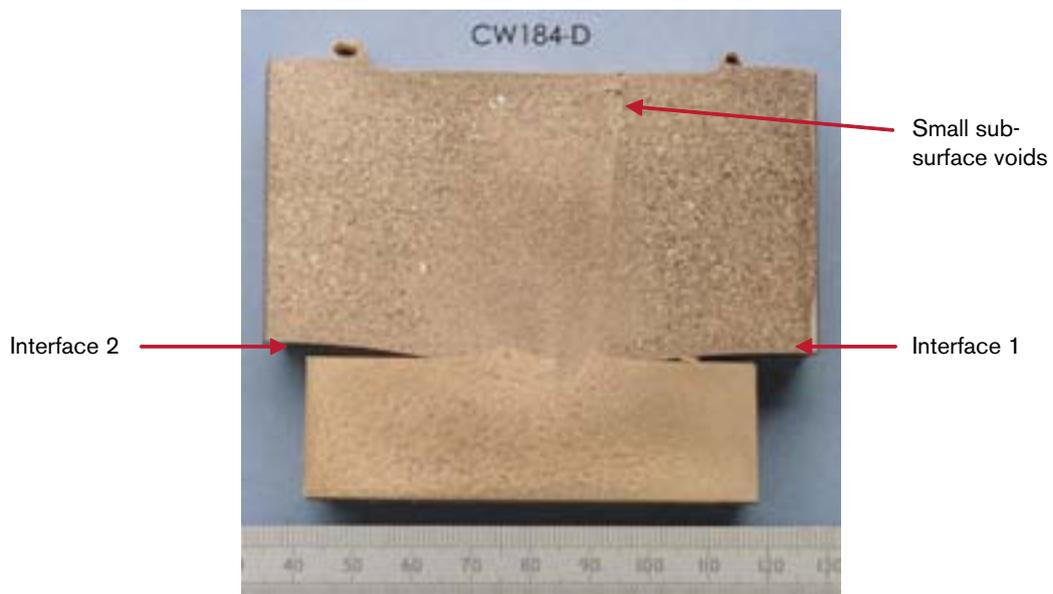
*Figure 10-3. Typical sub-surface void size associated with large fit up gap.*
