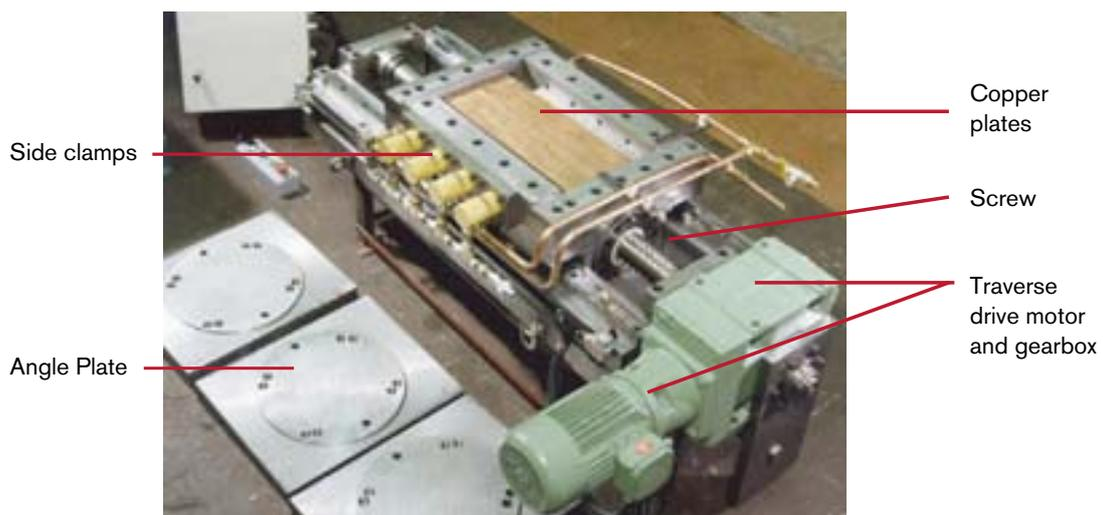
**Figure 4-8.** The purpose-built linear traversing table.
