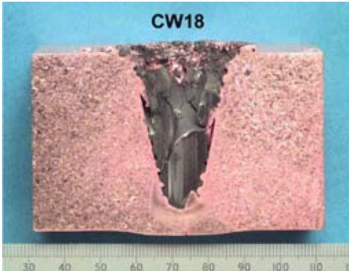
**Figure 7-9.** A cemented carbide MX Triflute™ probe that fractured during the plunge sequence.
