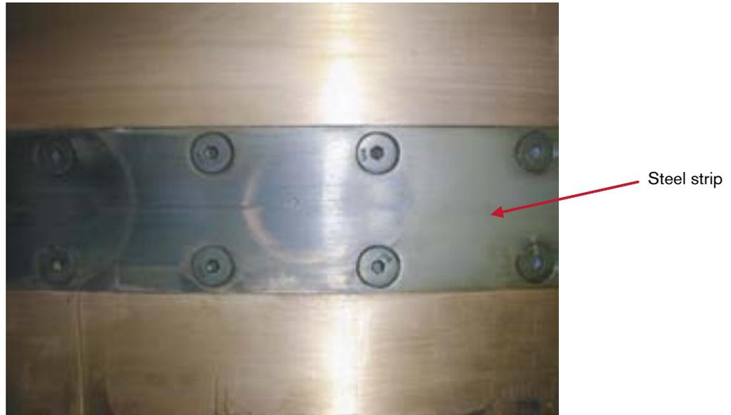
**Figure 5-12.** The steel strip bolted into a slot directly opposite the axis of the FSW tool probe.
