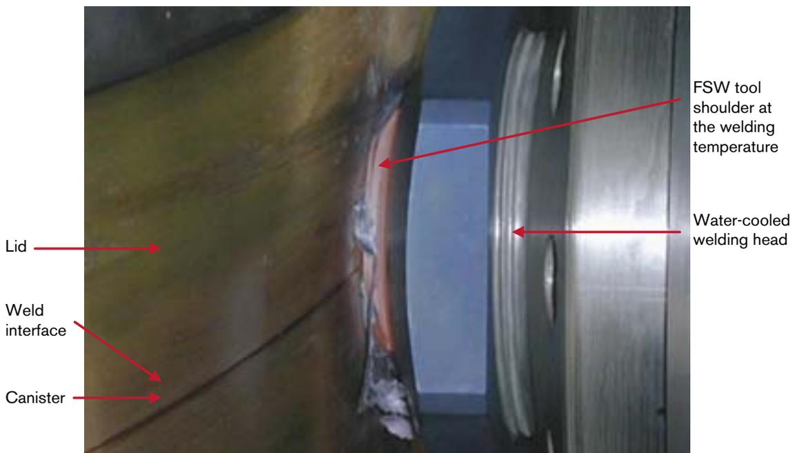
**Figure 9-5.** Weld No. CW189 being made in the steady state condition.
