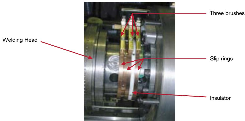
*Figure 6-12. Three brush/slip ring assembly.*
