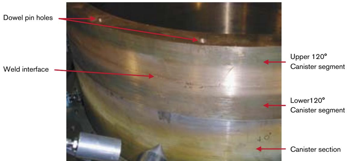
**Figure 6-14.** Location of the canister segments on the canister section in preparation for welding trials.
