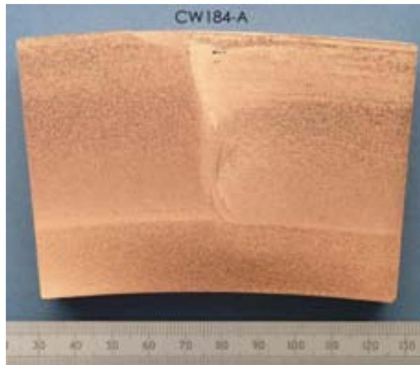
**Figure 10-4.** A longitudinal section through the start region of Weld No CW184.
