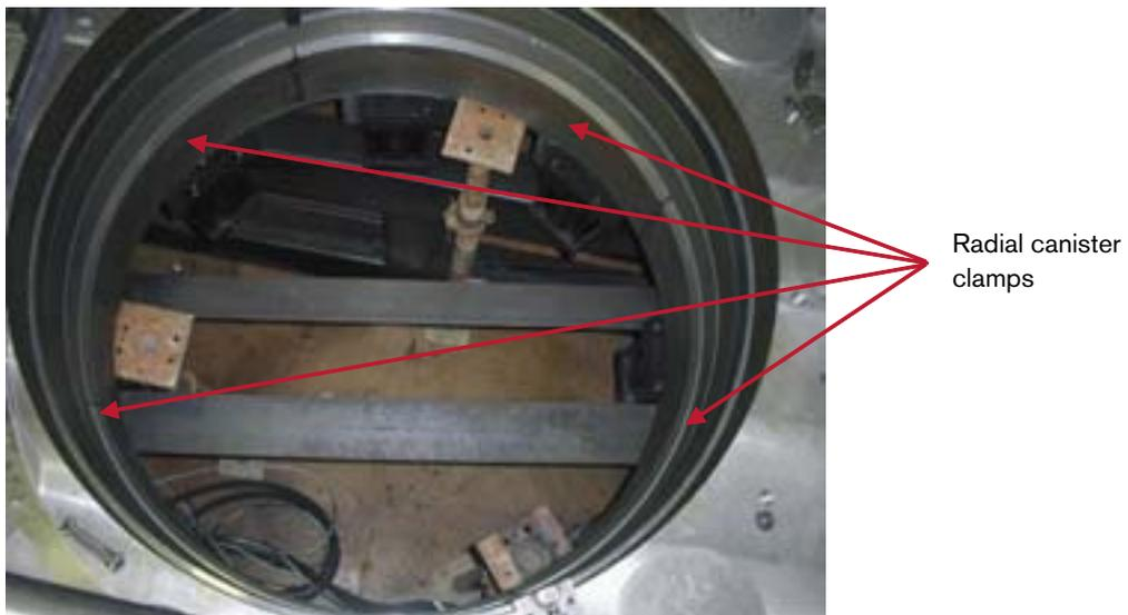
*Figure 5-5. The circumferential canister clamp.*
