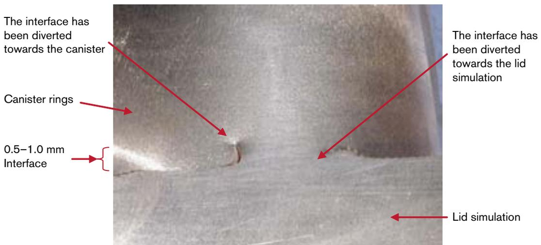
**Figure 10-5.** Weld interface deformation.
