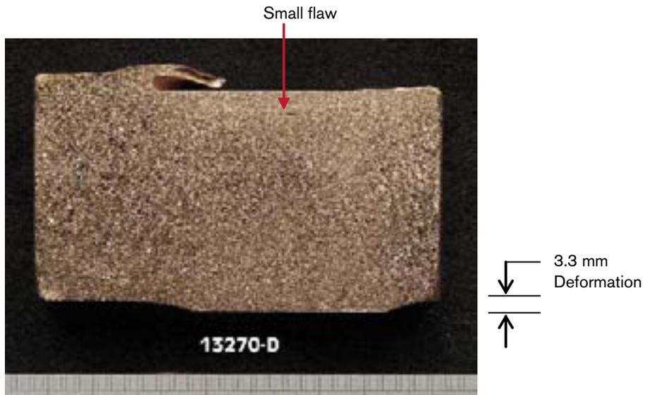
*Figure 8-4. Weld No CW100. Section D.*
