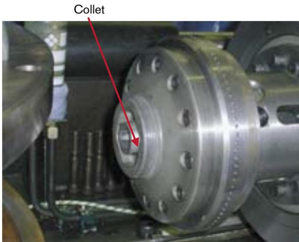
**Figure 6-5.** The tooling flange with the collet in position.
