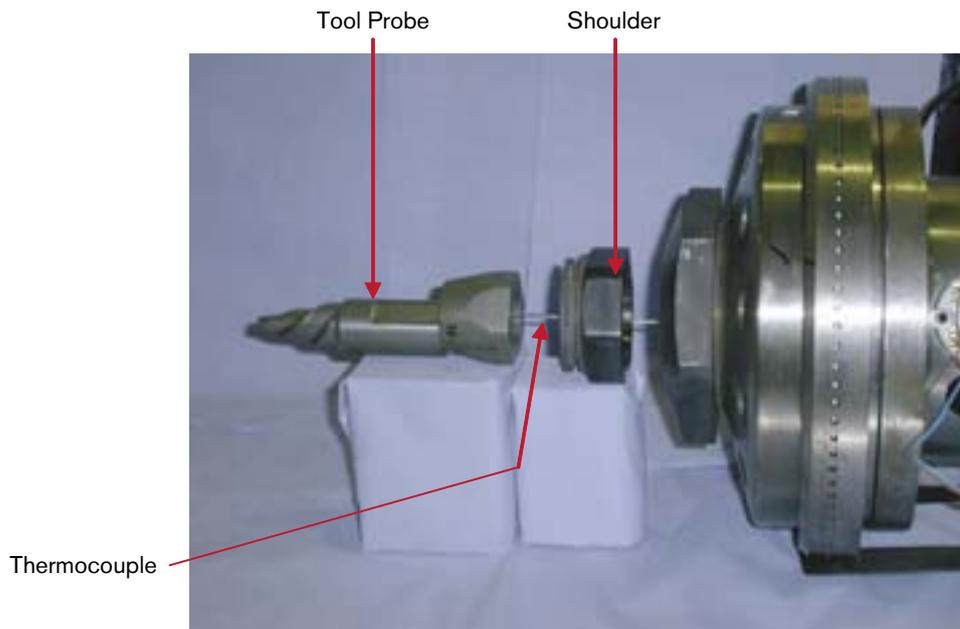
**Figure 6-9.** Thermocouple passing through water-cooled head.
