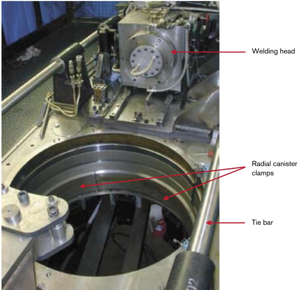
*Figure 5-4. View of the canister clamp showing two of the four circumferential clamps.*
