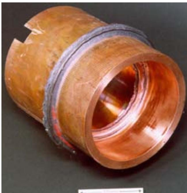
**Figure 1-1.** Friction welded copper tube.
