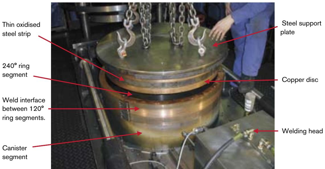
**Figure 5-13.** The lid simulation being lowered into the canister section.
