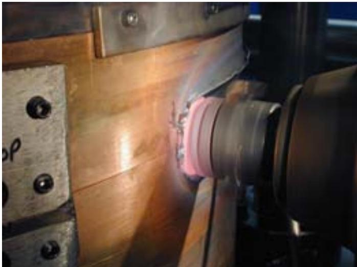
*Figure 6-2. The original experimental FSW canister welding machine's welding head operating at a temperature between 800–900°C.*
