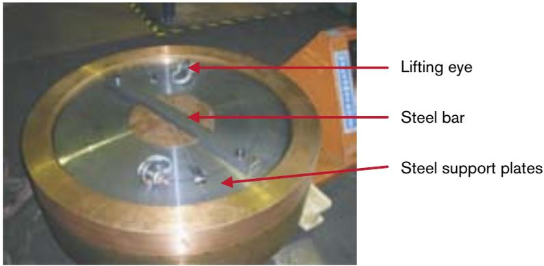
**Figure 6-20.** The steel support plate located in the lid recess.
