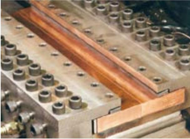
*Figure 4-2. Water-cooled clamping fixture for 10–25 mm plate.*
