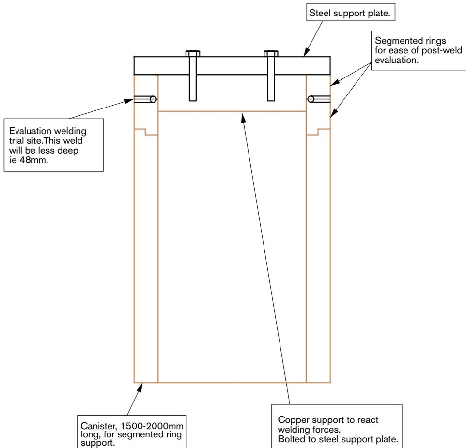
**Figure 5-9.** The lid to canister weld simulation.
