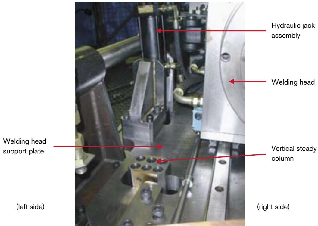
**Figure 8-1.** The hydraulic jack assembly.
