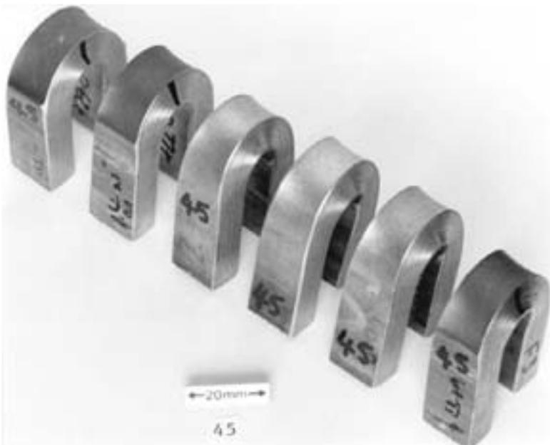
**Figure 4-6.** Root and face bend test specimens.
