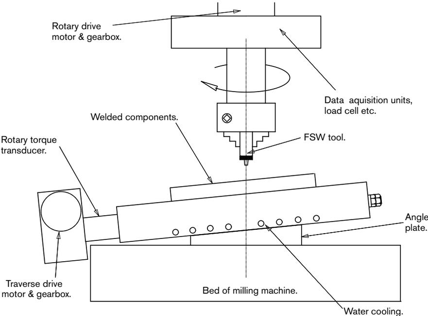
Figure 4-7. General arrangement of the linear traverse unit.
