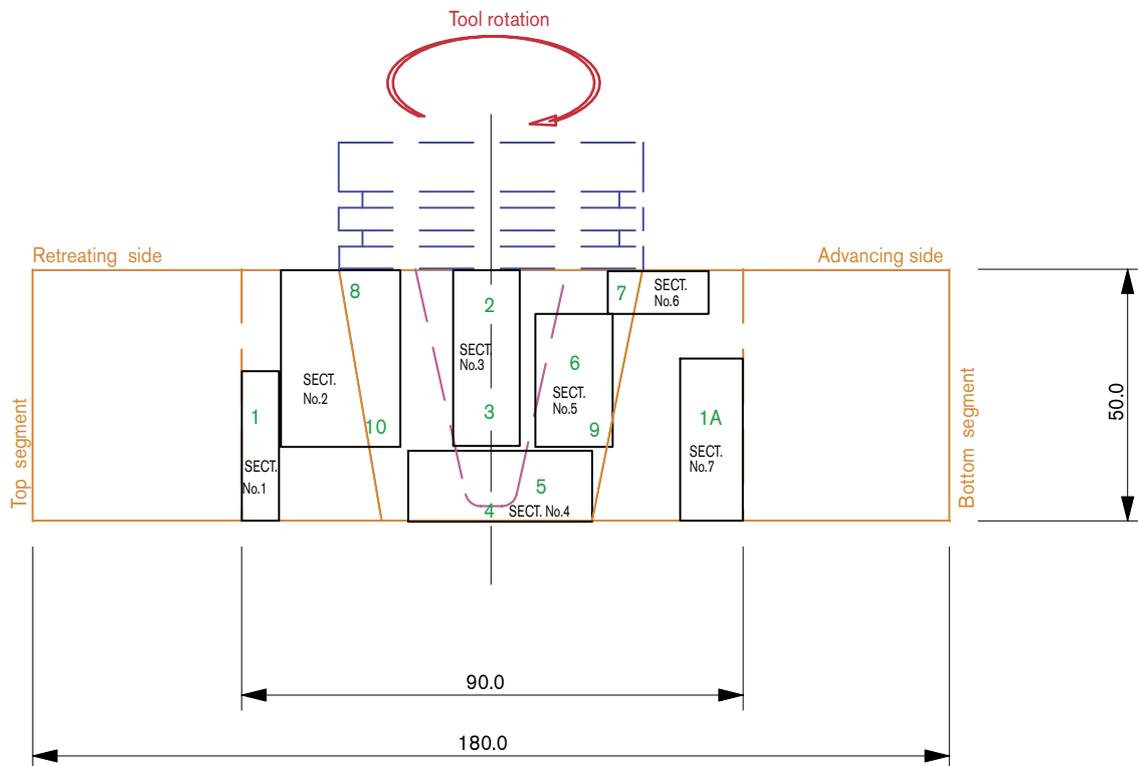
**Figure 10-8.** Metallurgical section cutting plan through a transverse section cut through Weld No. CW32, Section C.
