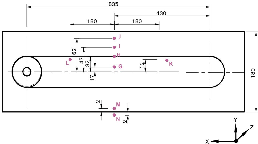
**Figure 4-13a.** Positioning of thermocouples in thermal field measurement tests, not to scale, all dimensions in mm.
