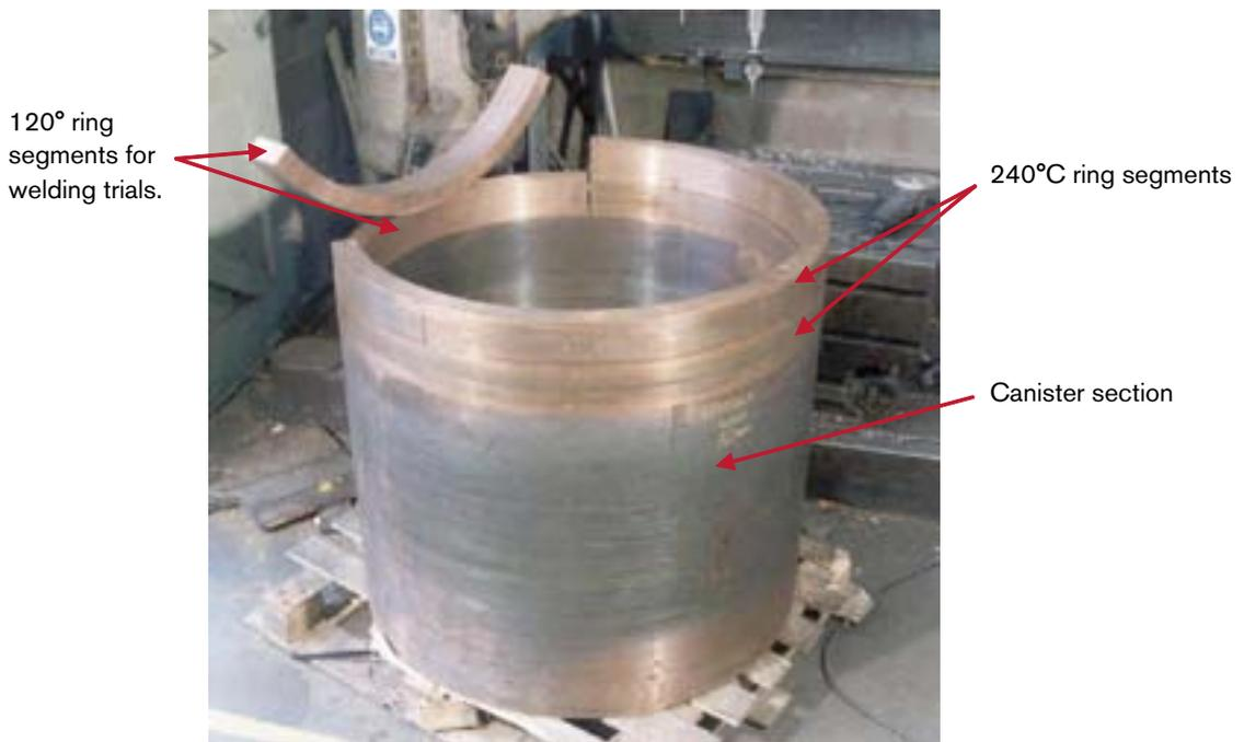
**Figure 5-10.** Canister Simulation.
