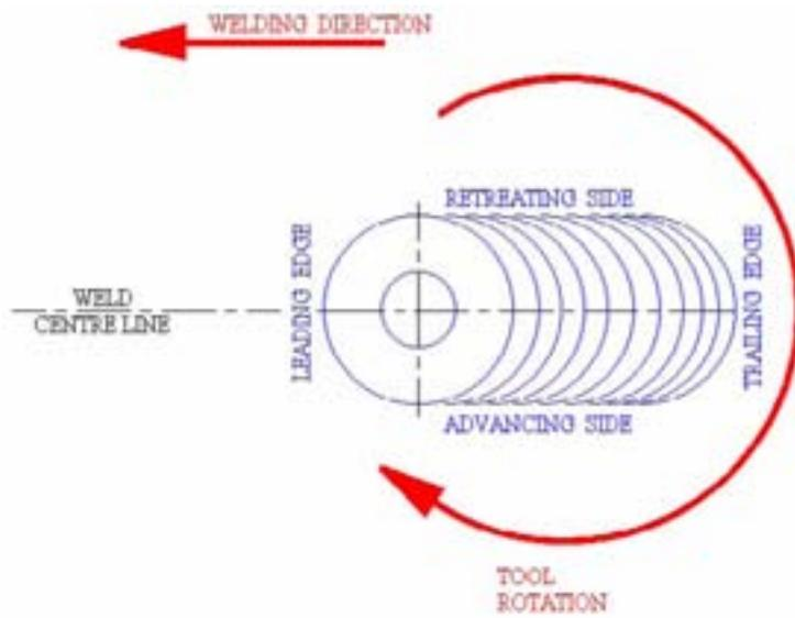
*Figure 4-9. The major features of a friction stir weld.*
