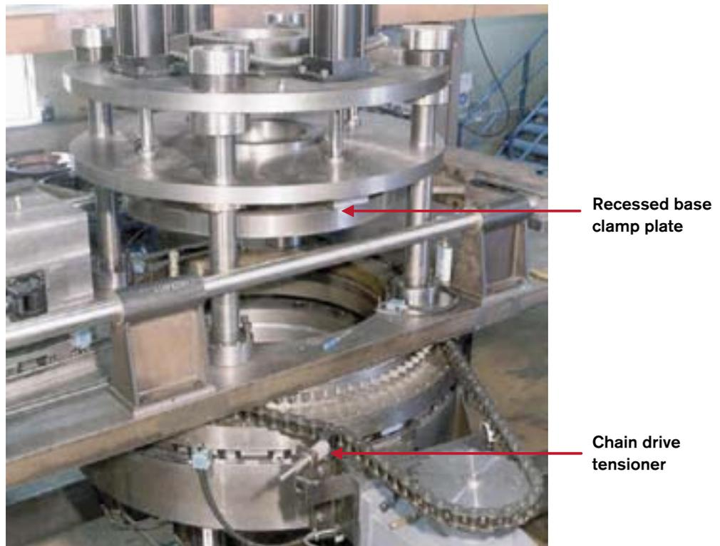
**Figure 5-3.** The experimental canister/base welding machine showing the canister clamp drive system.
