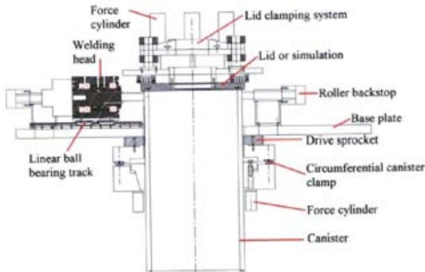
*Figure 5-1. Section through the experimental base welding machine.*
