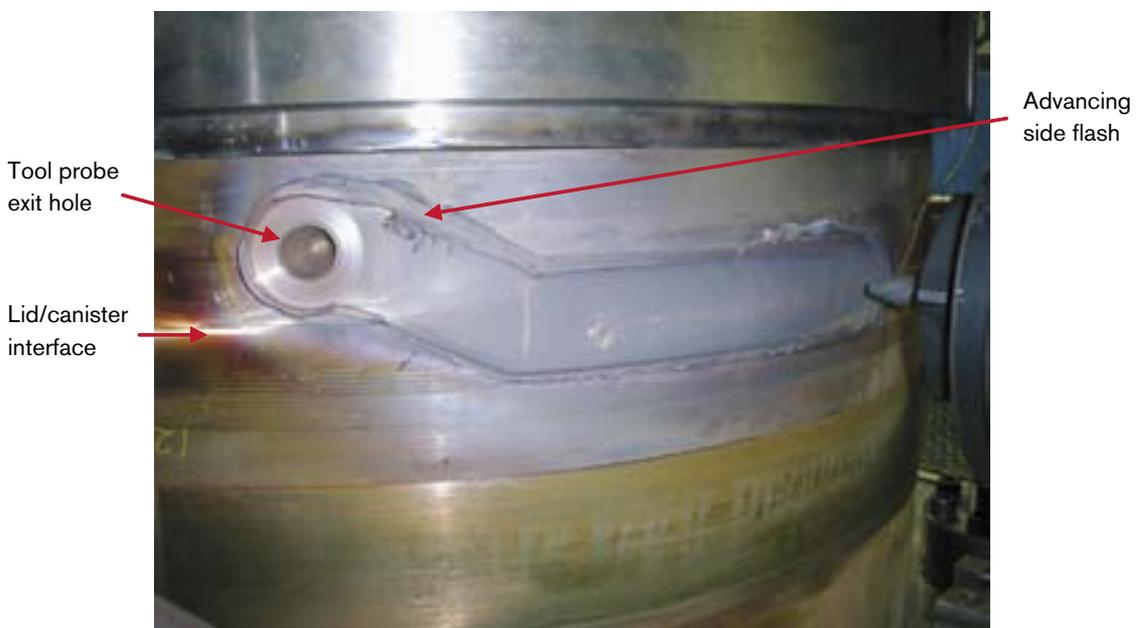
**Figure 8-3.** A tool probe exit path at 25° to the lid/canister interface.
