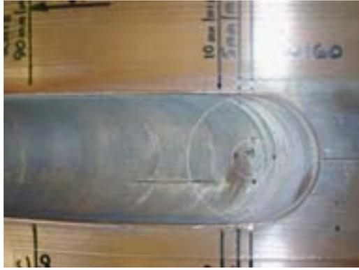
*Figure 10-1. A surface breaking void at the start of the weld (CW160).*
