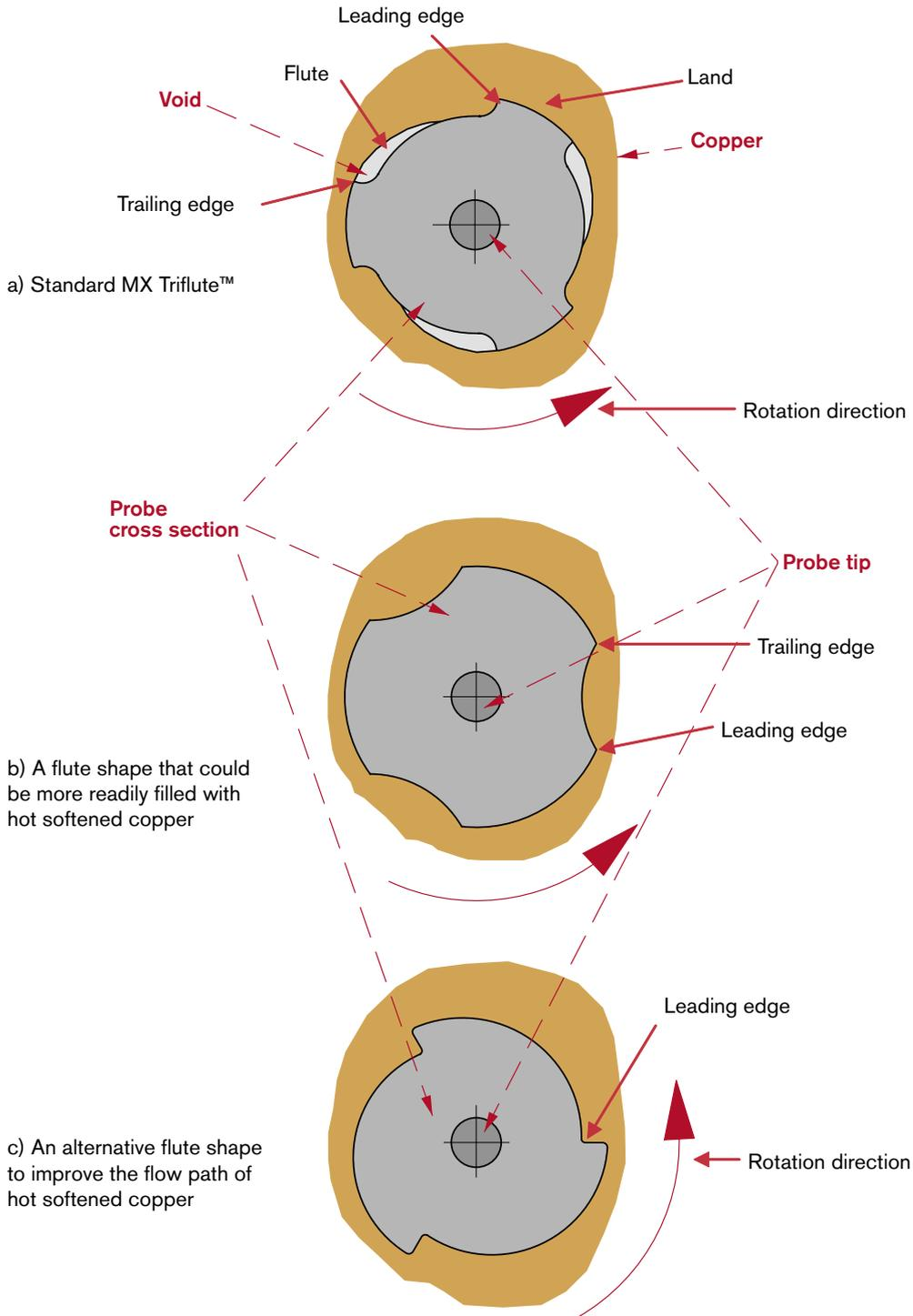
**Figure 7-6.** Illustrations of a cross section through FSW Triflute™ tool probes showing concepts to eliminate voids.
