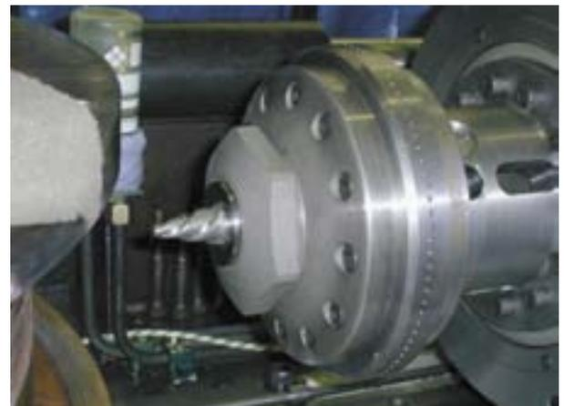
**Figure 6-8.** The shoulder retaining nut screwed up against the tool shoulder and probe.
