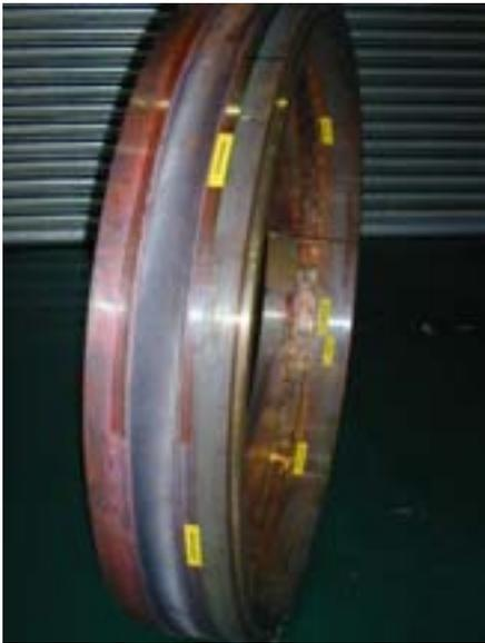
Figure 6-17. CW78 a complete circumferential weld.
