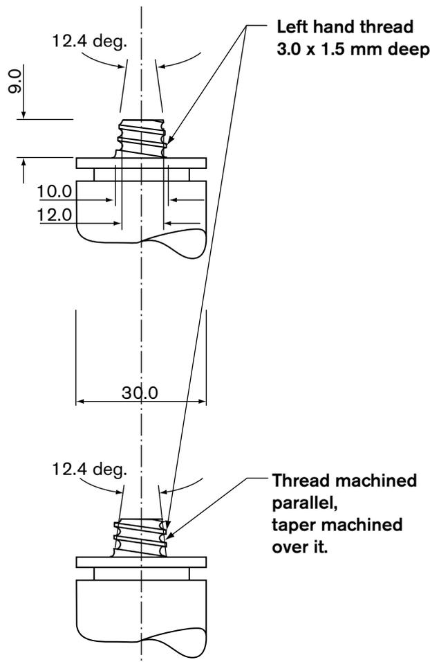
**Figure 7-1.** The 1997 FSW tool probe (Whorl™ type) used for welding 10 mm thick copper plate.
