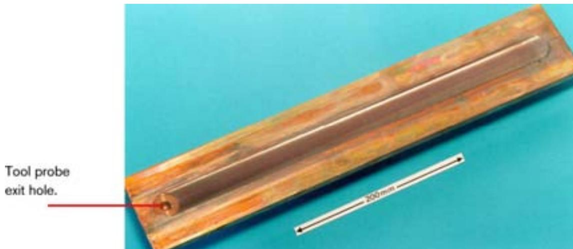
**Figure 4-4.** Completed FSW in copper plate 10 mm thick.
