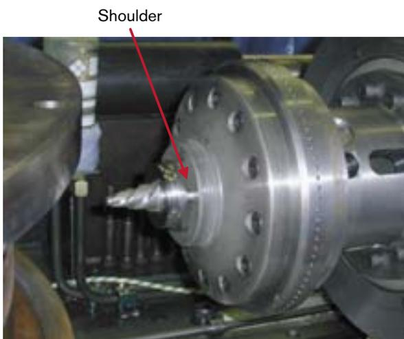
**Figure 6-7.** The Densimet DI76 tool shoulder in position.
