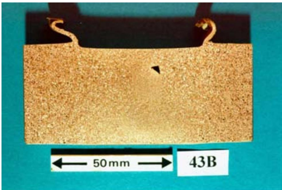
*Figure 4-10. Transverse metallurgical section cut through 40 mm thick weld No. 43B showing triangular shaped flaw on the advancing side.*
