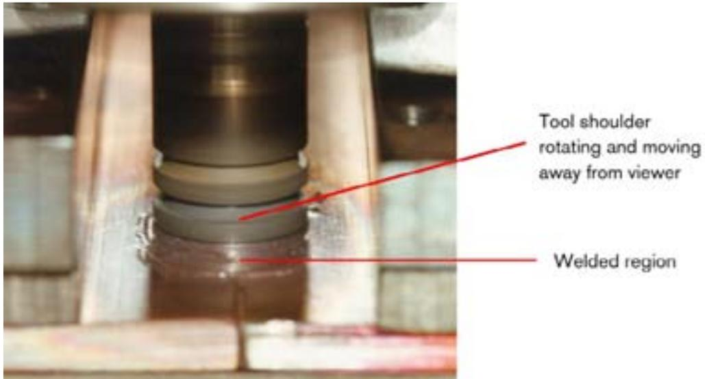
**Figure 4-3.** FSW 10 mm copper plate.
