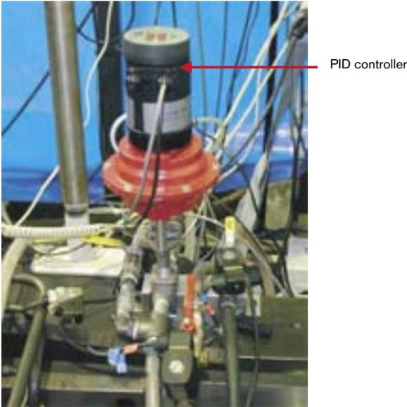
**Figure 9-3.** The Low Flow Valve with an integrated positioner.
