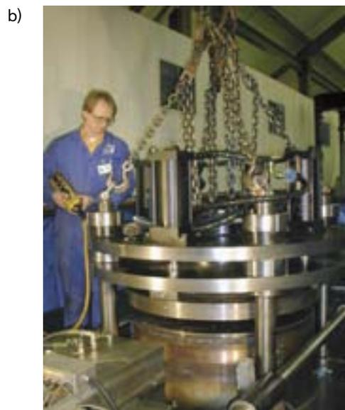
**Figure 6-1.** Lowering the base clamping fixture into position.
