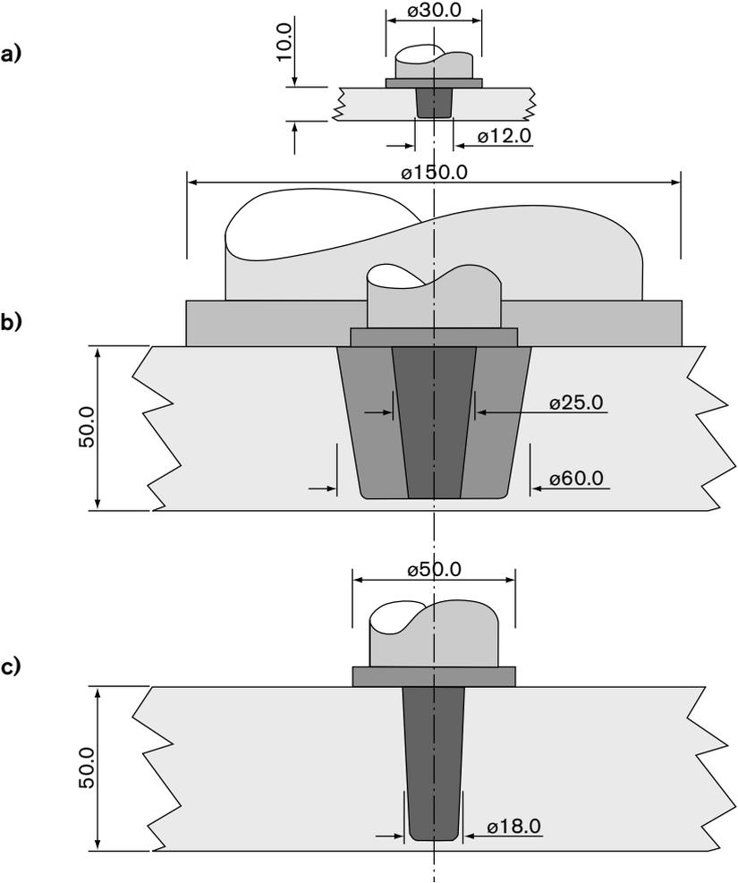
**Figure 7-2.** Sketches showing the tool probe dimensions used to weld 10 mm thick copper plate scaled up to weld 50 mm thick plate.
