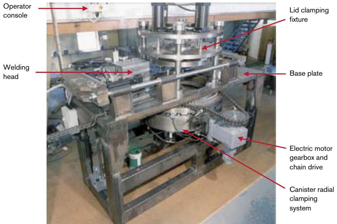
**Figure 5-2.** The general arrangement of the FSW machine before the operator walkway was fitted.
