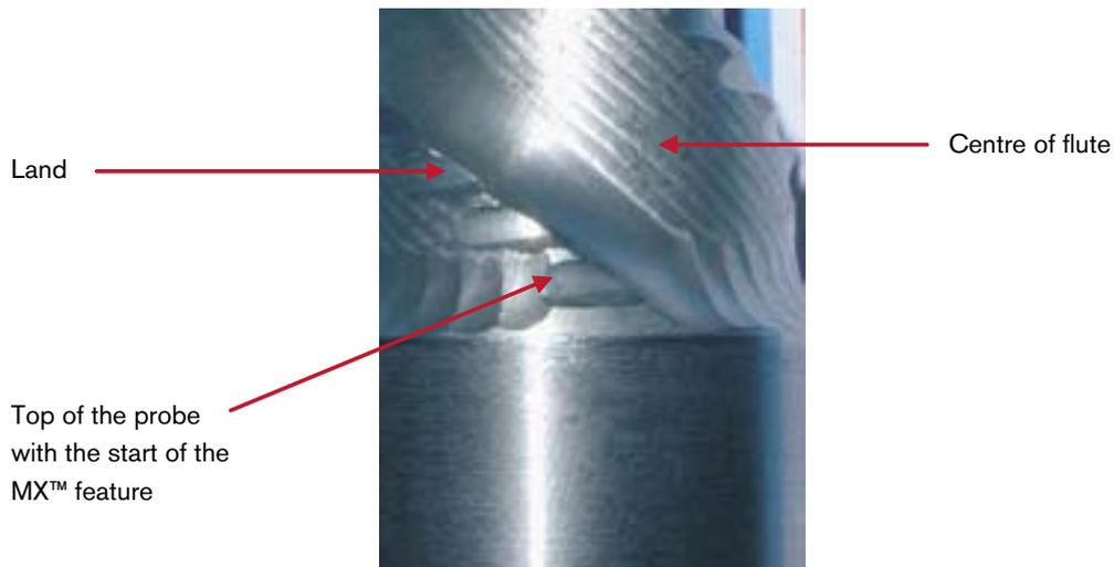
**Figure 7-8.** An A023 MK7 FSW tool probe.
