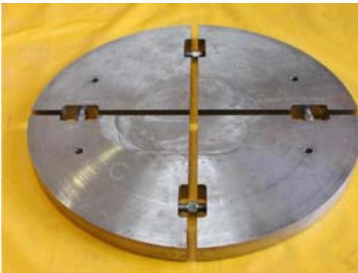
**Figure 6-21.** The lid support plate with four adjustable sections.
