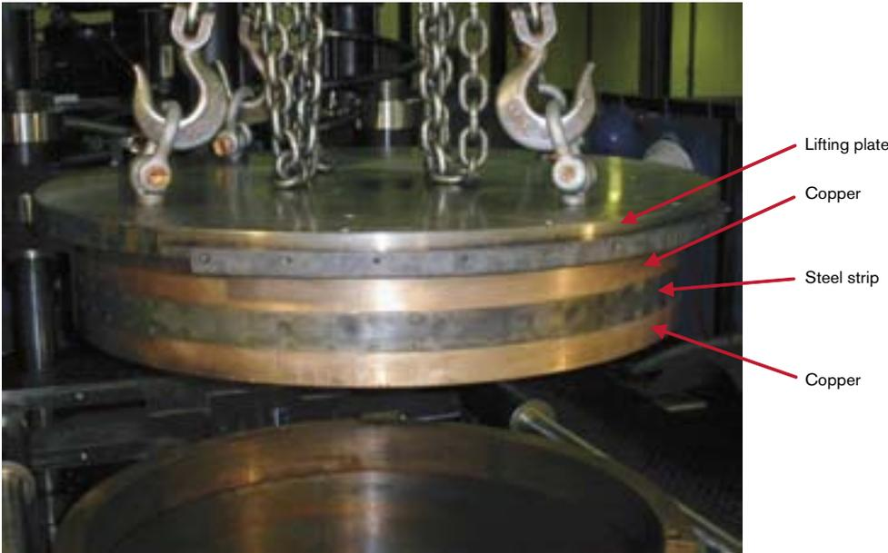
Figure 5-11. The canister base simulation suspended from four lifting eyes.
