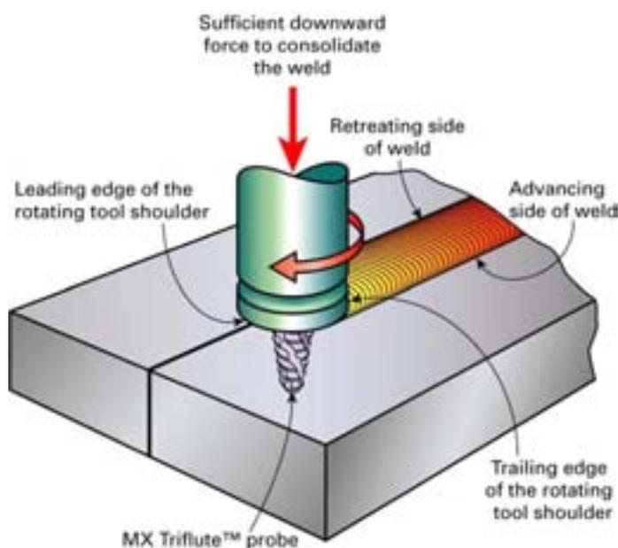
*Figure 2-1. The principle of FSW.*
