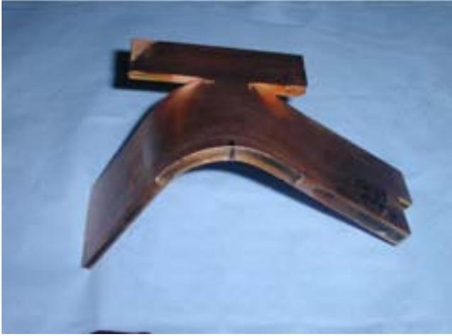
**Figure 10-7.** Weld No.CW160 bent through 130°.
