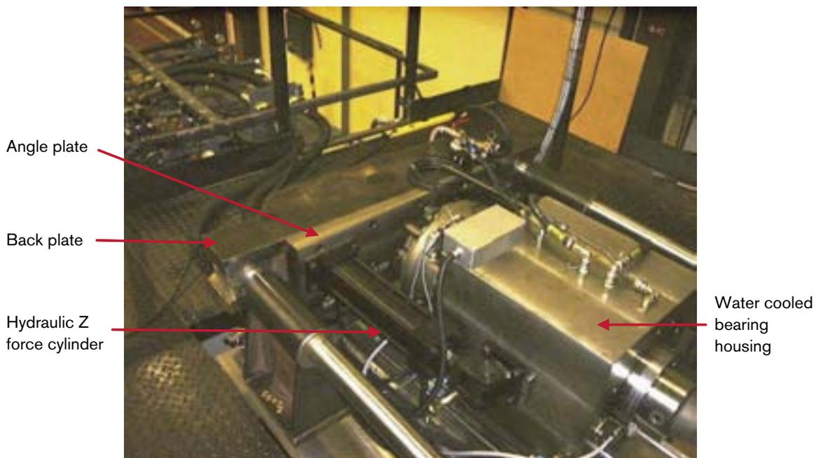
**Figure 5-7.** The experimental canister/base welding machine showing the welding head and angle plate.
