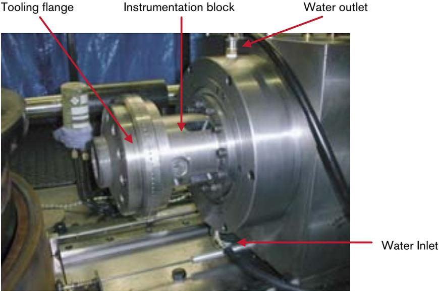
**Figure 6-4.** The instrumentation block and the tooling flange bolted to the water receivers.
