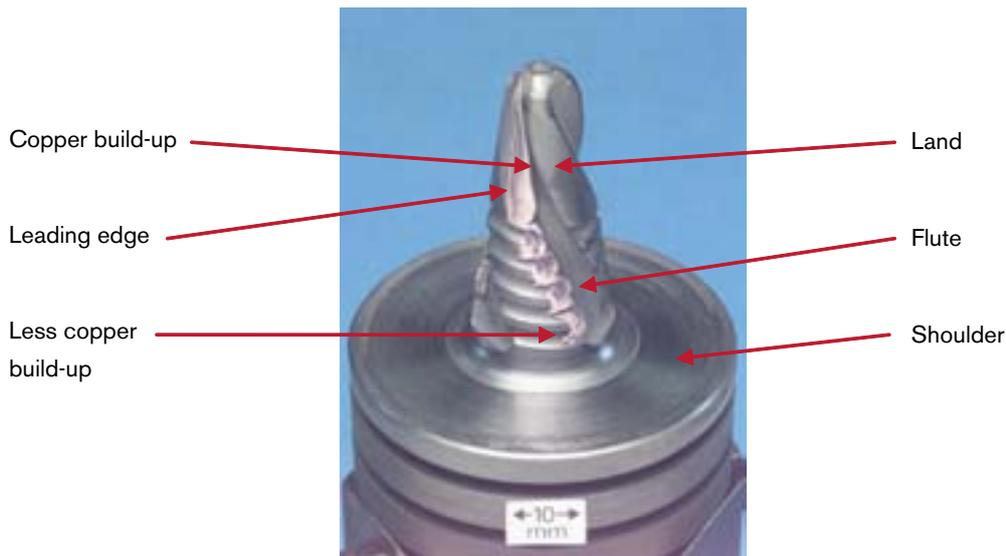
*Figure 7-5. MX Triflute™ probe showing the build up of copper on the leading edge of the flute.*
