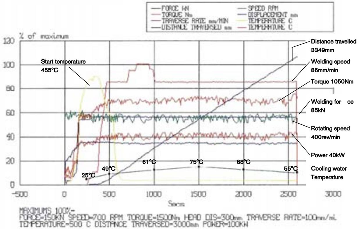
Figure 6-16. CW78 Complete circumferential canister weld.
