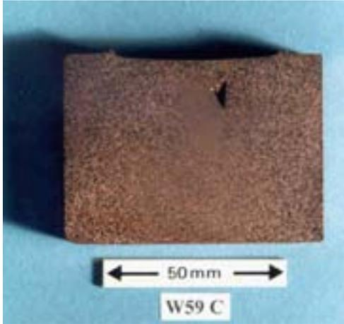
*Figure 7-4. The triangular shaped flaw located on the advancing side, near the top surface of 50 mm FSW copper plates.*
