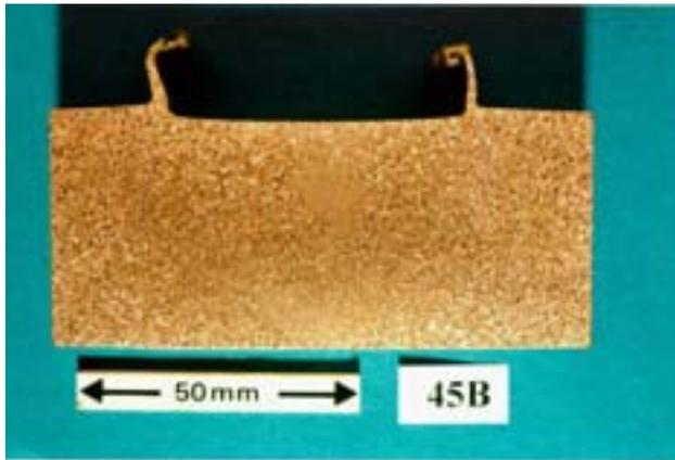
**Figure 4-11.** A transverse metallurgical section cut through weld No. 45B where increased side clamping force was used to eliminate advancing side flaws.
