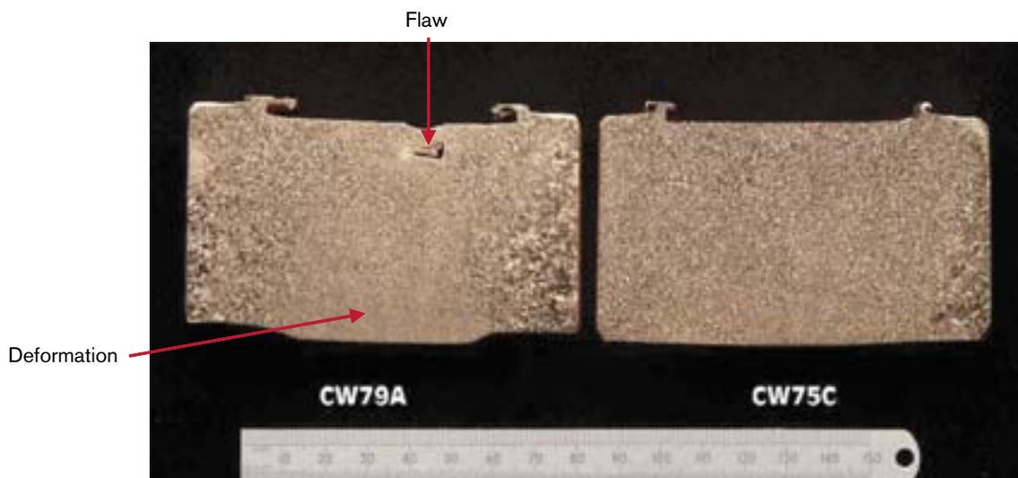
**Figure 9-2.** A comparison of Weld No CW79 (poor fit up and a large flaw) and CW75 (good fit up and no flaw) showing that fit up affects the weld integrity.
