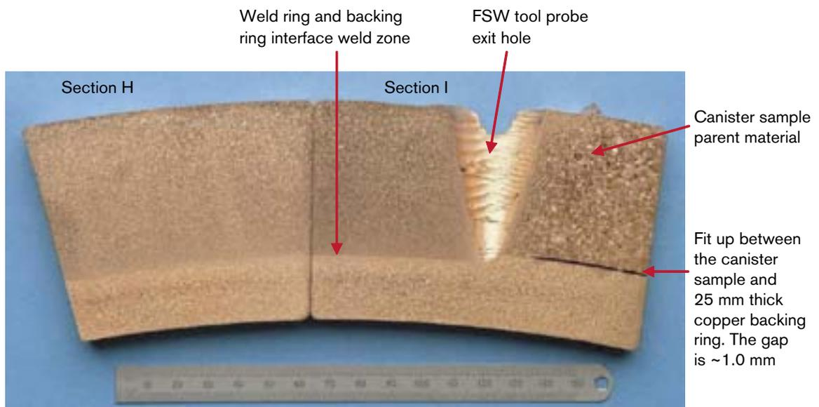
**Figure 6-19.** Canister weld CW136 showing longitudinal metallurgical section.
