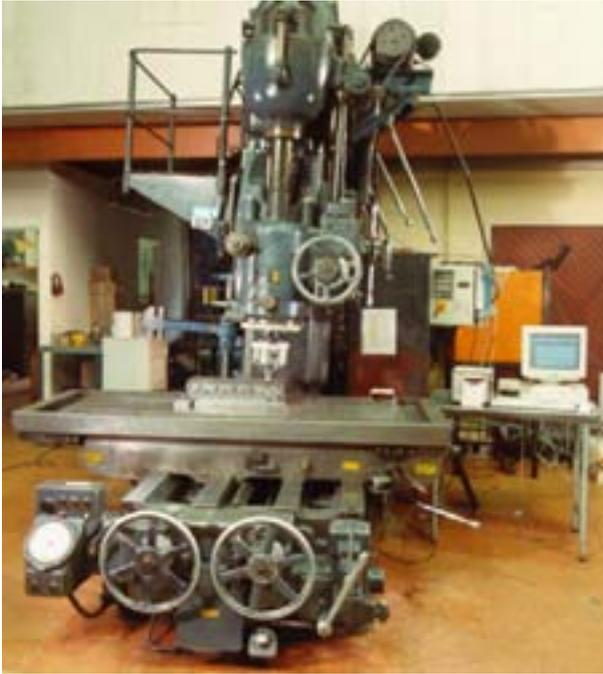
*Figure 4-1. TWI's large milling machine modified for FSW.*
