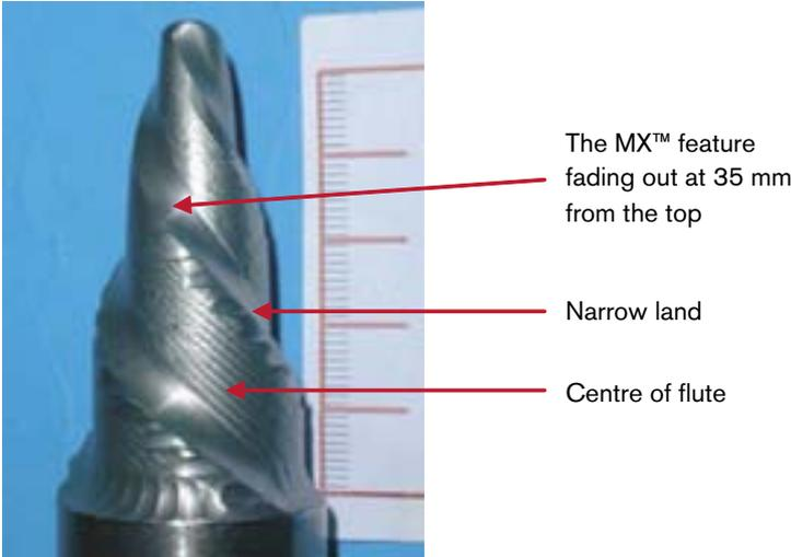
Figure 7-7. An A023 MK7 FSW tool probe.
