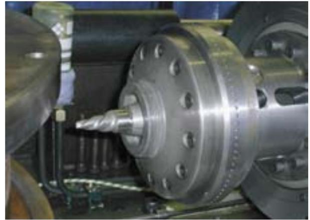
**Figure 6-6.** The FSW tool probe inserted into the collet.
