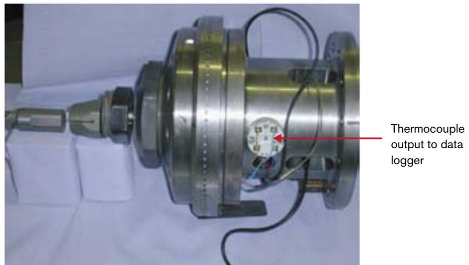
**Figure 6-10.** Thermocouple output into instrumentation block.
