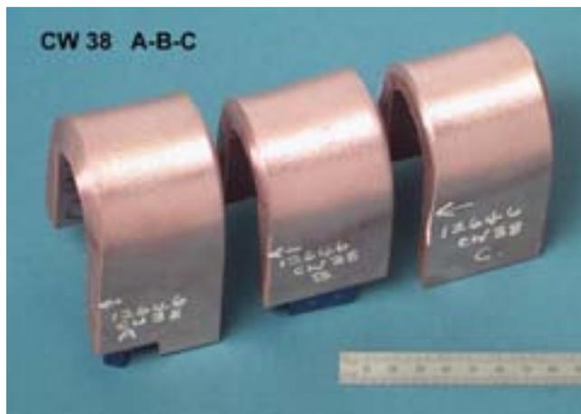
**Figure 10-6.** Side bend test sections A, B and C cut from Weld No. CW38.
