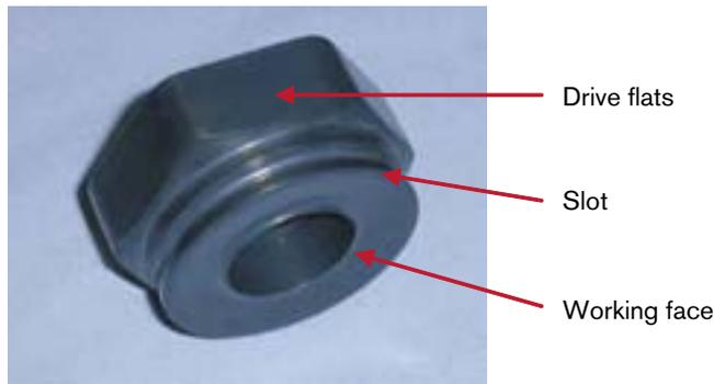
**Figure 7-10.** An FSW tool shoulder.
