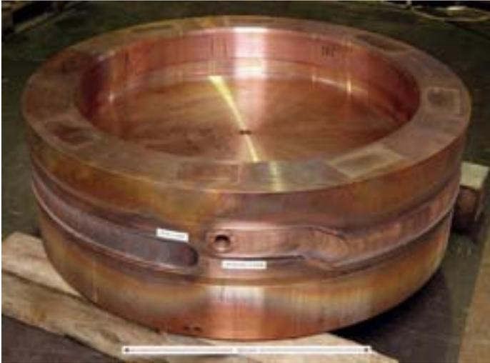
**Figure 6-22.** A lid to canister weld CW189.
