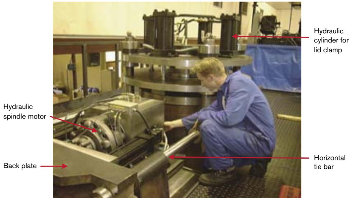
**Figure 5-6.** Location of the welding head and lid clamp.
