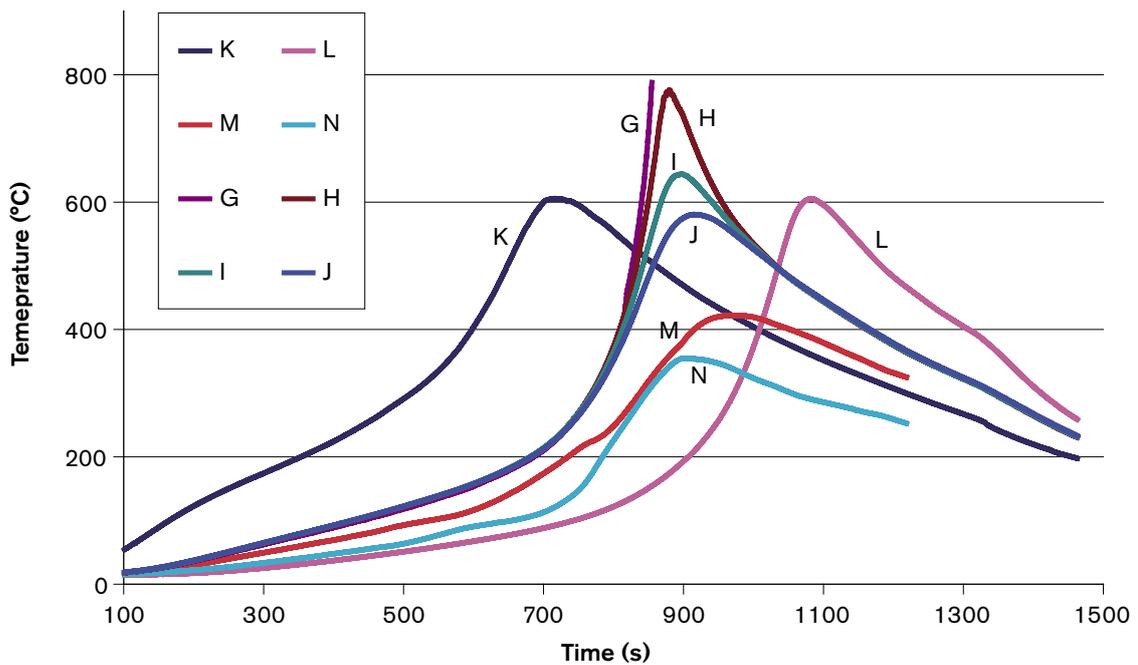
**Figure 4-13b.** Thermal field data obtained for FSW sample shown above.
