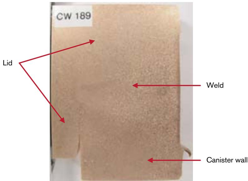
**Figure 6-23.** A metallurgical section cut through a lid to canister weld.
