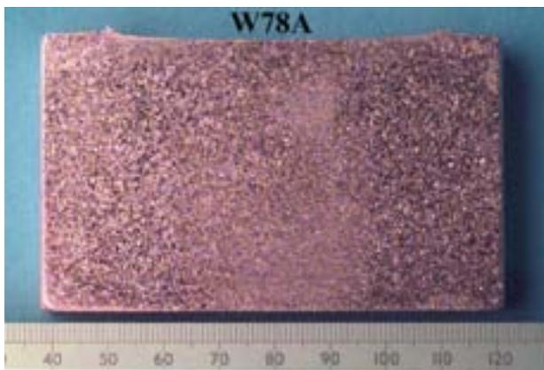
**Figure 4-12.** A transverse metallurgical section cut through weld No. 78A which is free from any major flaws.
